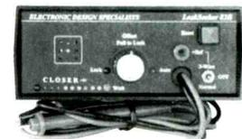
Your DVM shows the same shorted reading all along the pcb trace. LeakSeeker 82B has the resolution to find the defective component. Touch pads along the trace, and LeakSeeker beeps highest in pitch at the defect's pad. Now you can locate a shorted part only a quarter of an inch away from a good part. Short can be from 0 to 150 ohms
