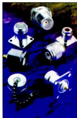
Tru-Connector SC Coaxial Connectors are similar to "C" series bayonet types but are threaded to provide a secure coupling that cannot vibrate loose. Featuring a 5 KV version with overlapping Teflon® dielectrics for a longer electrical leakage path, these connectors can also be supplied in a 1 KV version with high temperature (+165°C) Fluoropolymer dielectrics.
