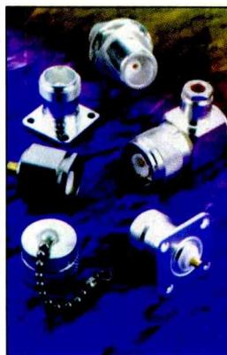
Tru-Connector SC Coaxial Connectors are similar to "C" series bayonet types but are threaded to provide a secure coupling that cannot vibrate loose. Featuring a 5 KV version with overlapping Teflon® dielectrics for a longer electrical leakage path, these connectors can also be supplied in a 1 KV version with high temperature (+165C°) Fluoroloy® H dielectrics.
