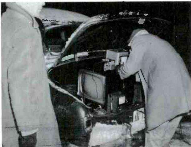
Figure 2. Field Testing UHF Receiver Using Portable Equipment.
