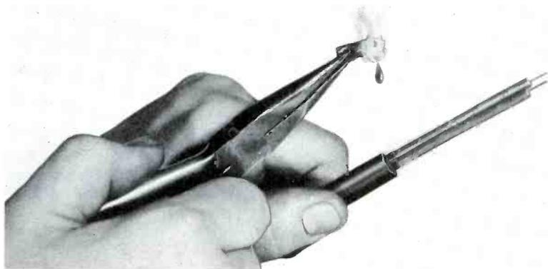
Figure 6. Sealing the Anaconda ATV-270 Line.
