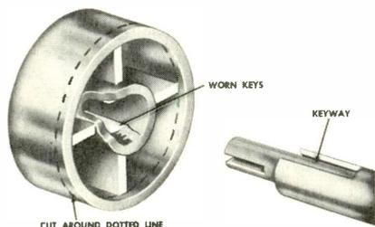
Figure 1. Worn Knob with Dotted Line Marking the Flange Cut.
