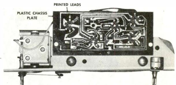
Figure 3. Printed Circuit Leads Formed on Plastic Chassis Plate.
