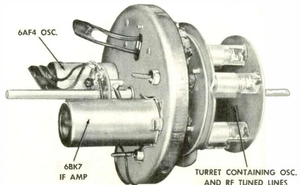
Figure 2. Photo of Tuner Turret with Shield Removed.
