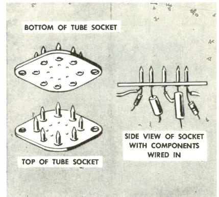
Figure 6. Construction Details of Socket Employing Hollow Tubular Terminals.
