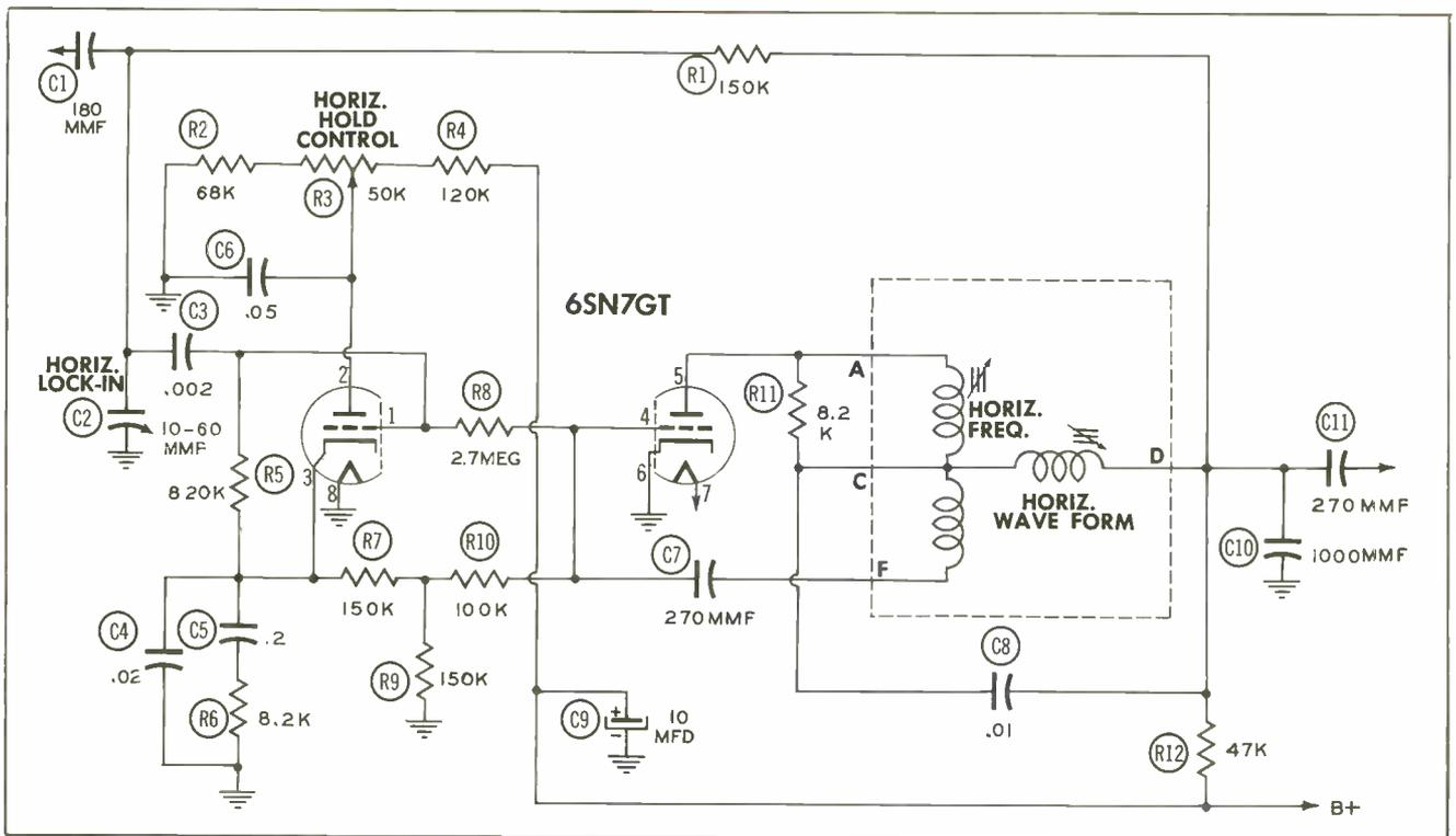
Figure 4. Typical "Synchroguide" Circuit.
