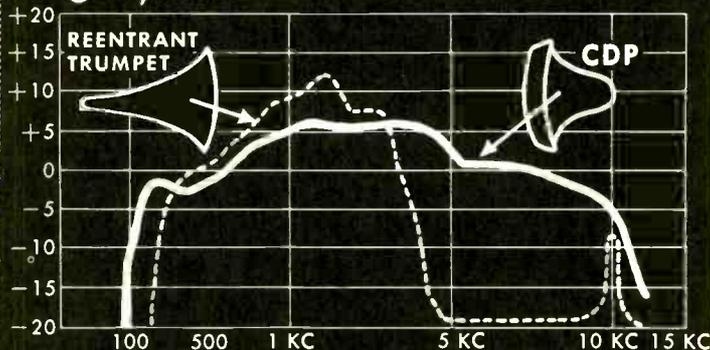
**Model 848 Compound Diffraction Projector\* Loudspeaker System**
