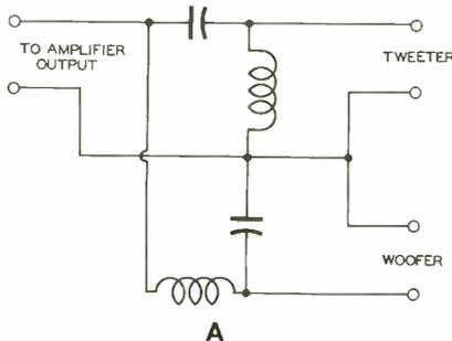
Figure 7. (A) Half Section Network for Two Way System, Parallel Connected.
