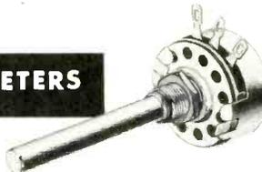
Because the resistance material in these units is solid-molded—not sprayed or painted on—continued use has practically no effect on the resistance. Often, the noise-level decreases with use... and they provide exceptionally long, trouble-free service. Rated at 2 watts, with a good safety factor.
