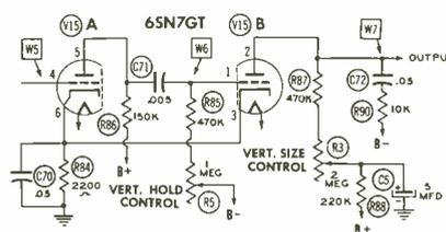
Figure 7-19. A Commercial Type Cathode-coupled Multivibrator.
