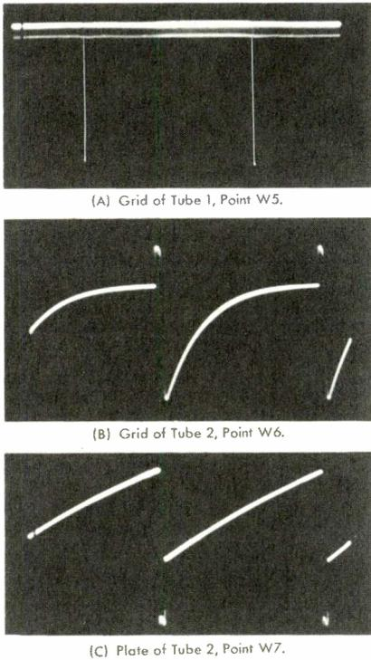
Figure 7-20. Operating Waveform of the Cathode-coupled Multivibrator of Fig. 7-19.
