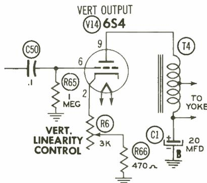
Figure 7-24. Vertical Output Circuit Employing a 6S4.
