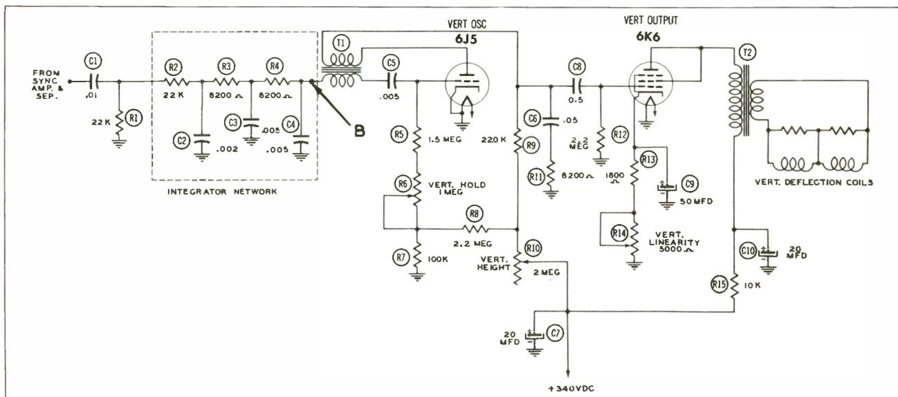
Figure 2. A Typical Vertical Deflection System
