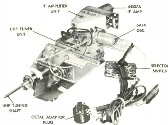
Figure 4. Philco UHF Converter Model UT-21A.
