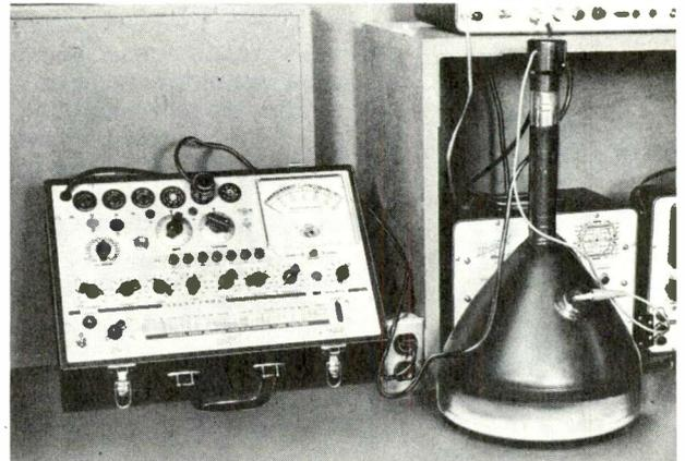
Figure 8. CRT-1 Adaptor Made by Hickok Electrical Instrument Co.
