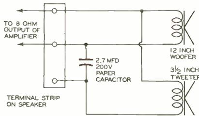
Figure 3. Schematic of Stromberg-Carlson RF-71 Speaker.
