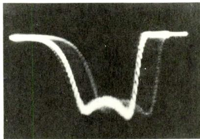
Figure 2. Response Curve with "Ghost" Produced by Horizontal Oscillator Radiation from TV Set.
