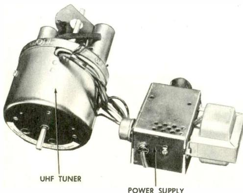
Figure 1. Photo of GE UHF Tuner Model UHF-103 with Included Power Supply.
