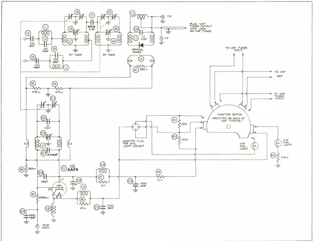
Figure 7. Schematic of Philco UHF Tuner Model UT-20A.
