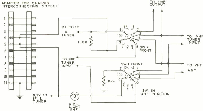
Figure 9. Function Switch and Adaptor for UHF Tuner UT-21.
