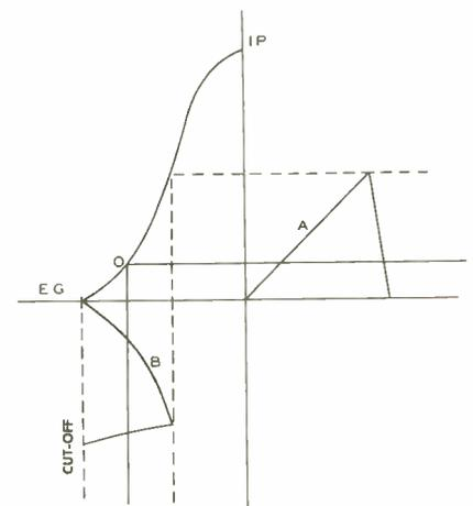
Figure 7-25. Removal of the Non-linearity from the Sawtooth by Operating the Amplifier on the Curved Portion of the Characteristic Curve.
