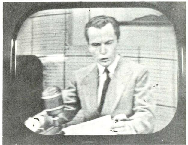
Figure 1. Picture Tube Having Low Cathode Emission. (A) "Zombie" Effect at High Brightness Setting. (B) Normal Shading at Reduced Brightness Setting. (Photographs Reproduced with Permission of CBS Television with Apologies to Winston Burdette.)
