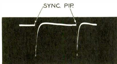
Figure 3. The Incoming Sync Pip as Seen on the Grid Waveform of the Blocking Oscillator.
