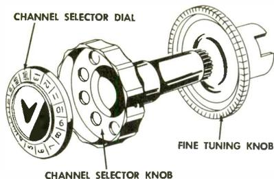
Figure 17. Details of Selector Knob.
