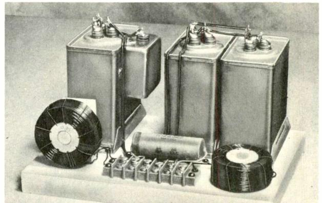
Figure 5. Home-Constructed Divider Network.
