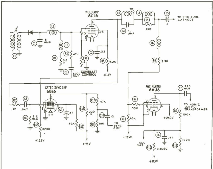
Figure 13. Partial Schematic of Video, Keyed AGC, and Gated Sync Separator Circuits.
