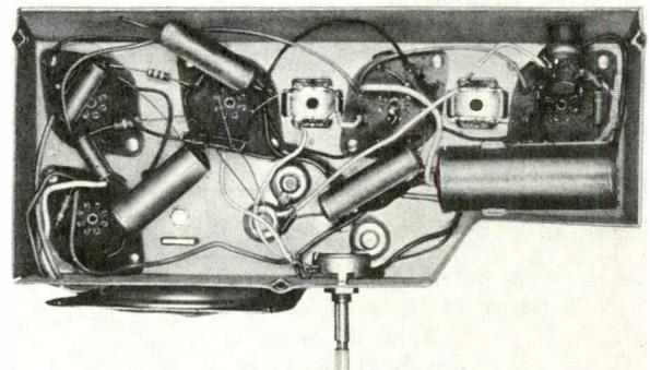
Figure 7. Bottom View of Model 542 Showing Completed Wiring.
