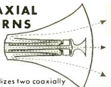
CDP utilizes two coaxially mounted diffraction horns working from both sides of a single diaphragm. Each horn is designed for optimum air loading and reproduction within its own range.
