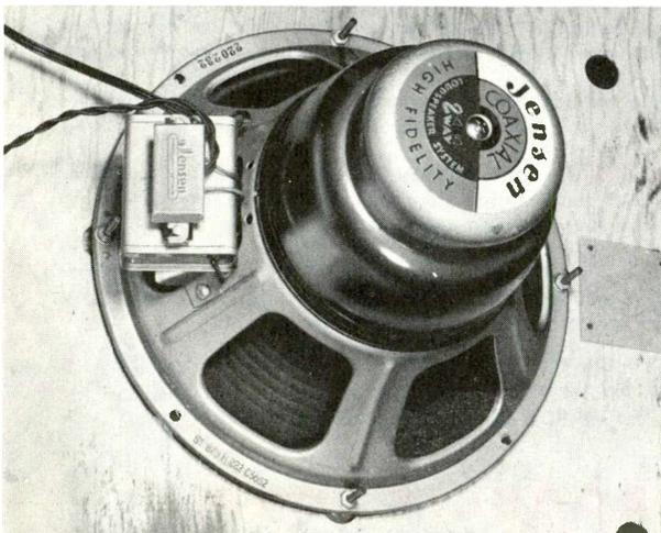
Figure 1. Jensen H-222 Coaxial Speaker with Capacitor Attached to Frame.
