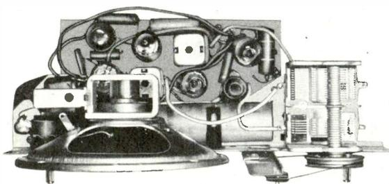
Figure 2. Component Arrangement in Admiral Radio.
