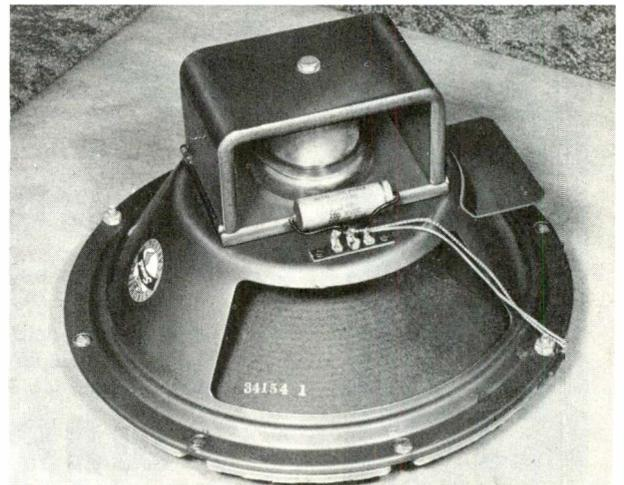
Figure 2. Stromberg-Carlson RF-71, Coaxial Speaker Showing Capacitor in Series with Tweeter.
