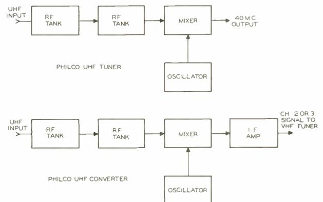
Figure 5. Block Diagram of Philco UHF Tuner and Converter.
