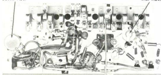
Figure 14. Under Chassis View of KRK-12 Tuner.
