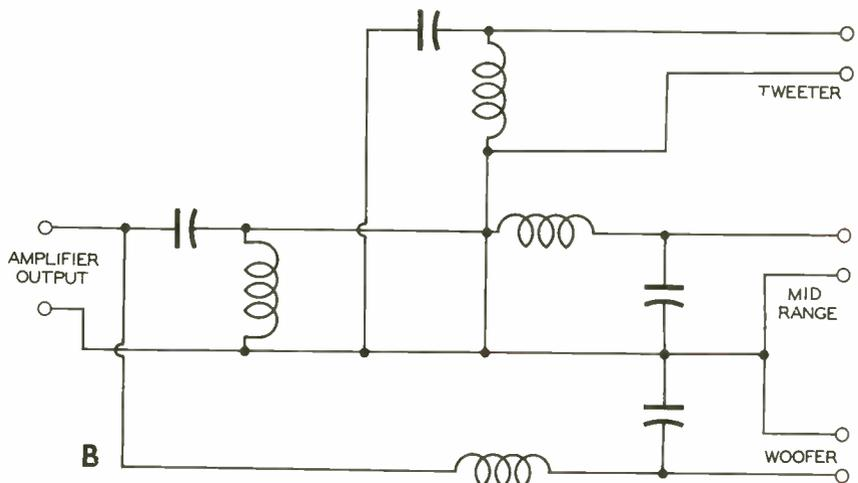
Figure 7. (B) Half Section Network for Three Way System, (B), Parallel Connected.
