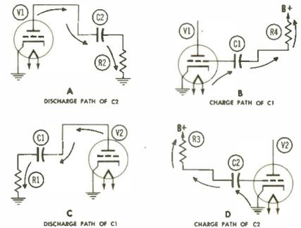
Figure 7-15. Charge and Discharge Paths of the Coupling Capacitors, C1 and C2 of Fig. 7-14.
