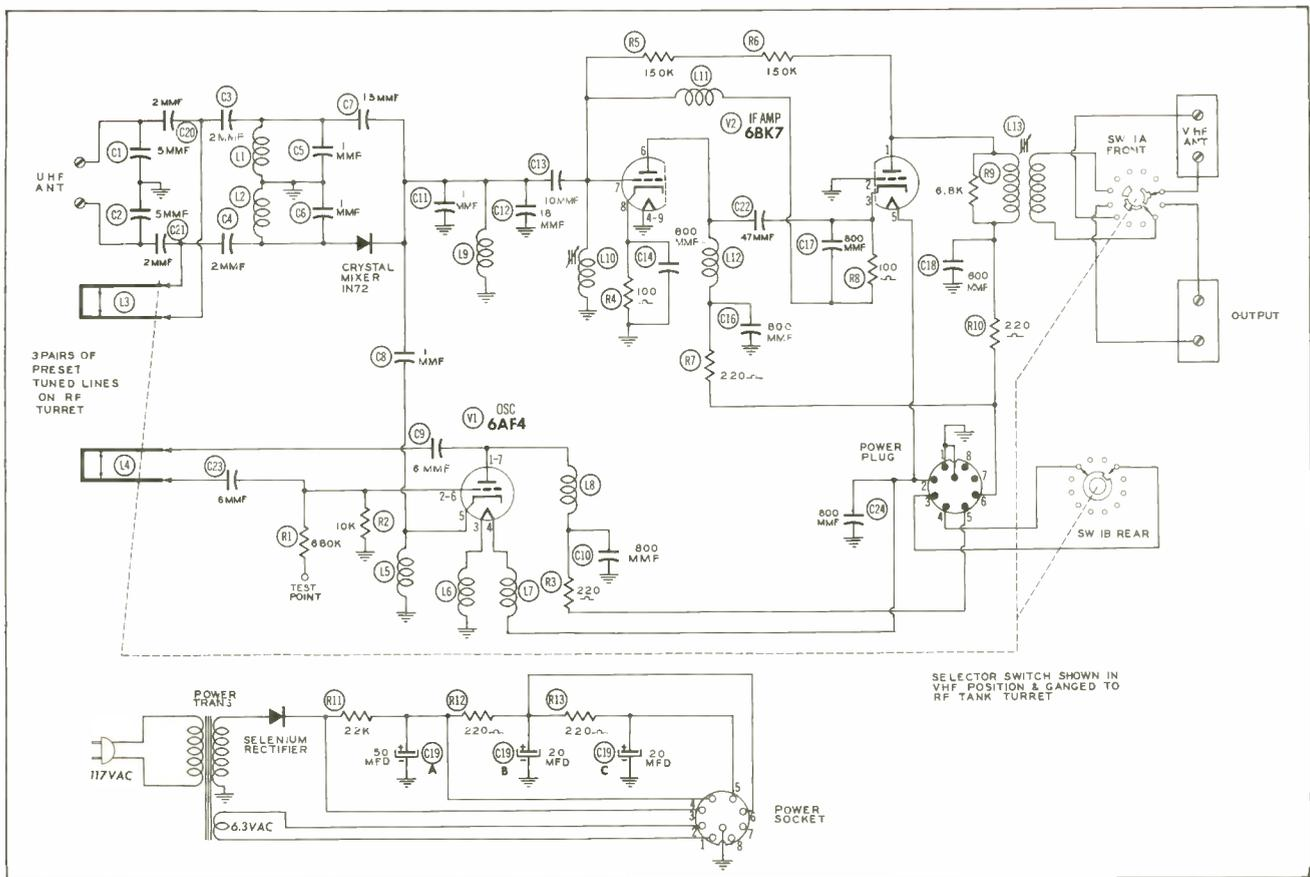
Figure 3. Schematic of GE Model UHF-103.
