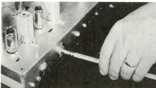
Figure 5. Using a Pencil as a Control Shaft Extension.
