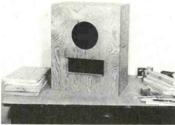
Figure 3. Front View of Reflex Enclosure Discussed in Text. Boards Used to Fill in Cabinet to Reduce Size Are Shown at Left.
