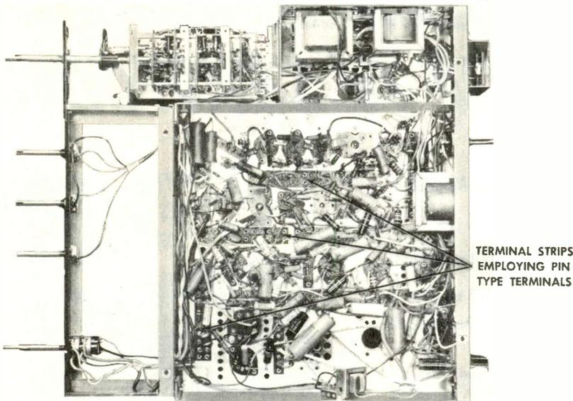
Figure 8. General Electric Receiver Model 21T1 Using Tubular Terminal Strips.
