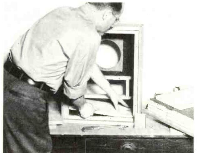
Figure 6. Installing Boards to Reduce Cabinet Size.
