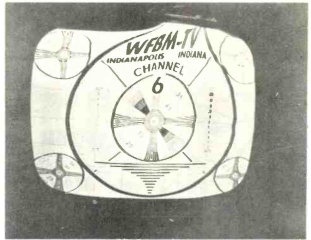
Figure 4. The Effect of a Strong Magnetic Field on a Picture Tube.
