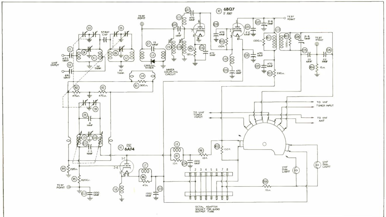
Figure 8. Schematic of Philco UHF Converter Model UT-21B.
