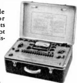
Single composite dynamic test for emission, trans-conductance and relative tube life. Panel-mounted roller-chart; convenient switches; provisions for future tubes. Portable Type 220 has durable metal case and handle; removable cover. Size: 6" x 11¼" x 17". Price: \$114.50.
