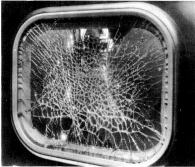
**IMPLOSIONS.** What happens when the expressman drops a television set? The accompanying photo tells the story - - the picture tube implodes and makes pretty patterns on the safety-glass window. Not too clearly shown, though, is the inward bellying of the safety glass toward where the picture tube was. The inrush of air to fill the vacuum of the tube volume sucked the glass inward, proving that these big tubes implode instead of explode.
