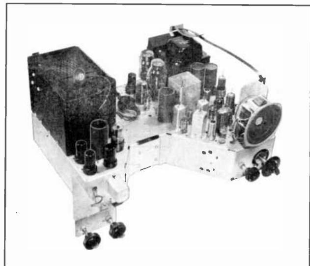
Fig. 1. 630-Type TV Chassis with Deflection Yoke and Focus Coil Removed.
