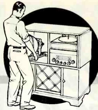
The space available in the Motorola model VF103 (Figure 1) is insufficient to allow the mounting of a 19" rectangular picture tube directly on the chassis, but there is enough room in the phonograph compartment for the tube alone, as shown in Figure 2. A 14" rectangular tube can be mounted on the chassis and such a conversion will be discussed later under cabinet changes. The electrical conversion and chassis changes should be made before the cabinet is altered.
