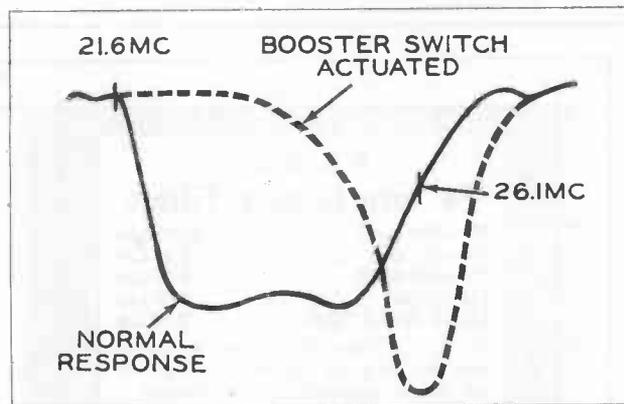
Figure 2. Video IF Response Patterns with Boost Switch "On" and "Off."
