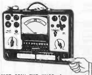
2. JUST SPIN THE KNOB—for correct, last-minute data, on the speed roll chart. Lists 700 tubes.
