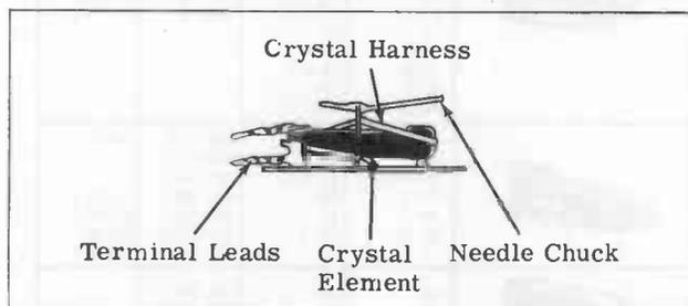
Figure 6. Crystal Harness Coupled to an "Expander" Crystal.
