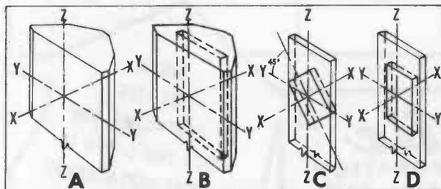
Figure 1. Cutting Angle of Expander and Shear Plate Phono Crystals Showing X, Y, Z Axes.
