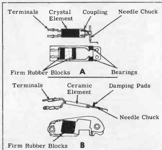
Figure 4. Crystal and Ceramic "Bender" Cartridges.
