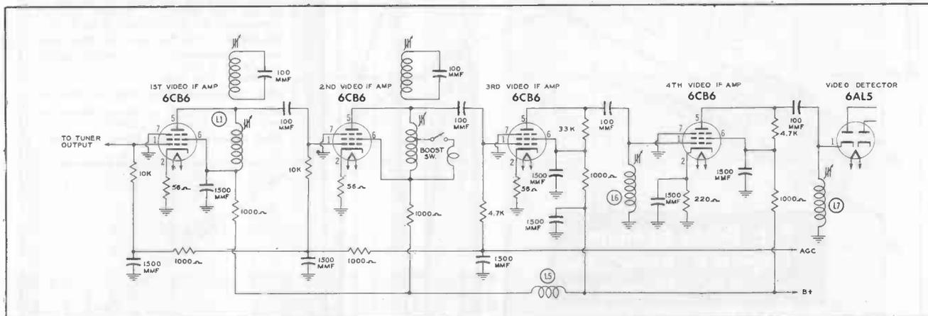
Figure 1. Radio Craftsman Video IF Amplifier Incorporating Boost Switch.
