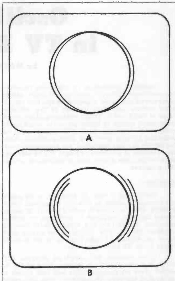
Figure 3. (A) "Ghost" Signal Caused by Reflected Signal. (B) "Echo" Effect Caused by Transient Oscillations.
