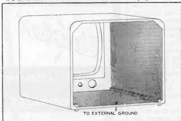
Figure 2. Cabinet with Screen Mounted to Reduce Radiation.
