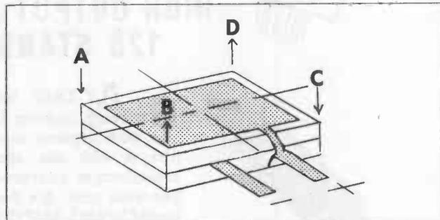
Figure 2. Movement of Corners in a "Twister" Element with a Potential Applied.
