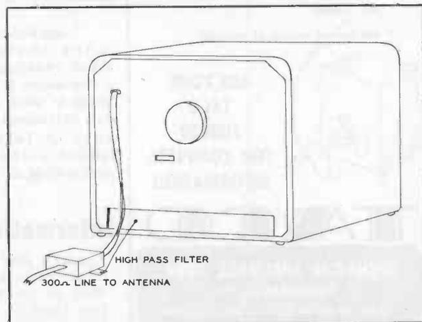
Figure 4. Proper Connection of High Pass Filter to Reduce Radiation from the Antenna.
