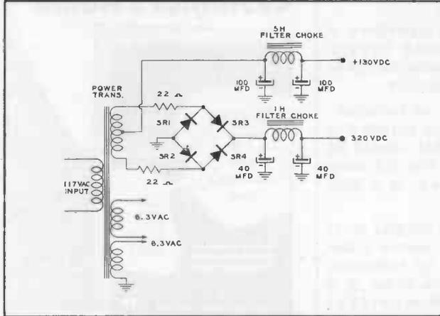
Figure 3. Bridge Rectifier Power Supply Employed in Radio Craftsman.
