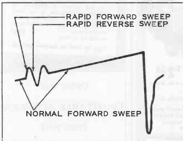
Figure 8. Waveforms of Sweep Voltage Containing Oscillations.
