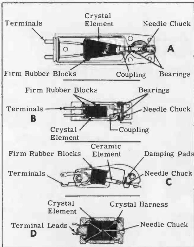
Figure 3. Examples of Various Types of Crystal Harnesses.
