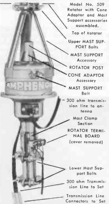
power and torque as a reversible type approximately 40% larger. This affords a stronger, more compact housing that means less weight and wind resistance on the support mast.
