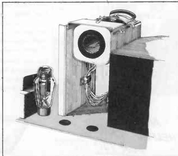
Figure 1. Example of Deflection Yoke Lead Dress to Reduce Radiation.
