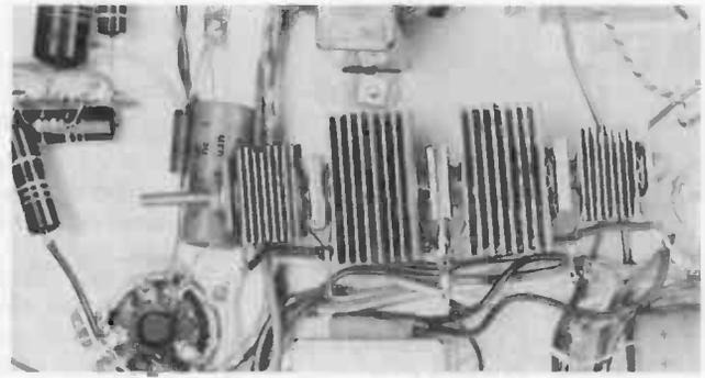
Figure 4. Mounting Detail of Selenium Rectifier.
