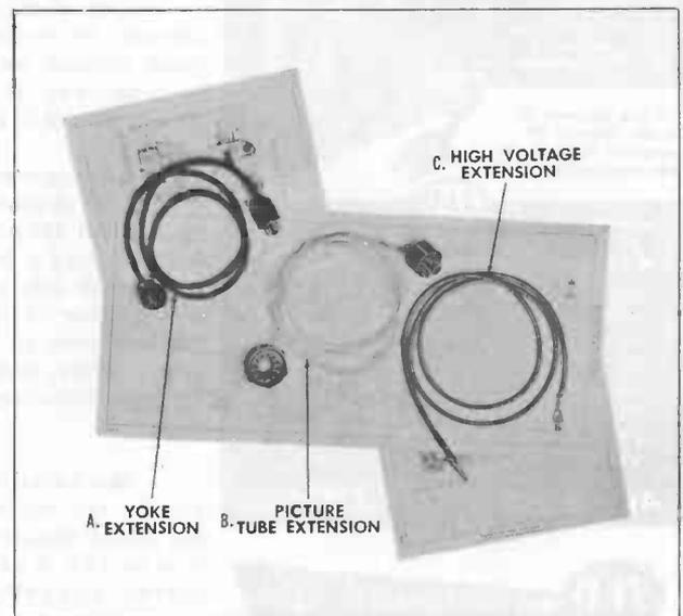
Figure 1. Extension Cables to Aid in Servicing Television Receivers with Cabinet-Mounted Picture Tubes.
