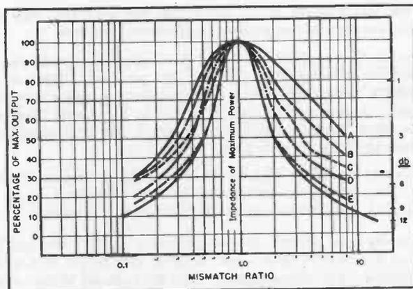
Figure 1. Curves showing the relationship between output power and the load impedance.
