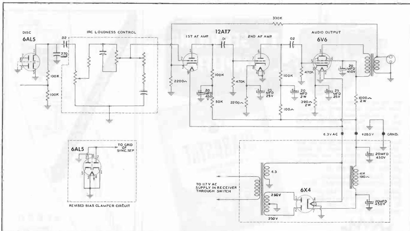
Figure 2. Revised Audio Circuit Showing Connection to Alternate Power Supply.
