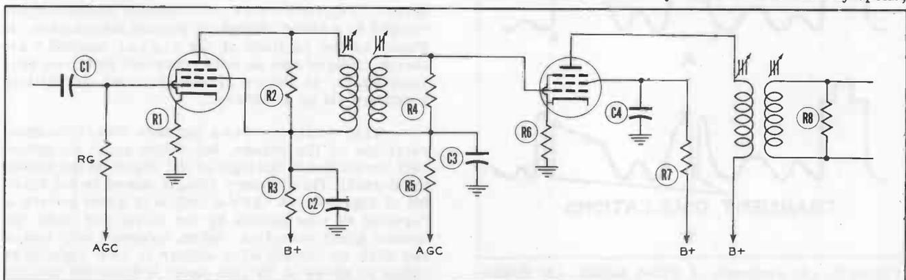
Figure 1. Typical Video IF Amplifier Stages.
