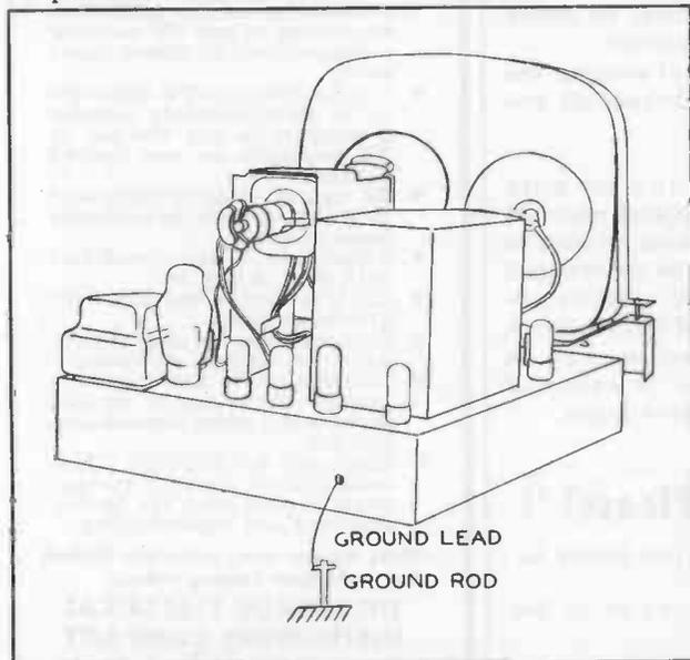
Figure 3. Example of Chassis Grounding Technique to Lessen BC Interference.
