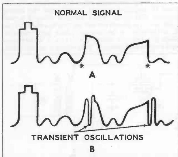
Figure 2. (A) Response of Video Signal. (B) Transient Oscillation in Video Signal.
