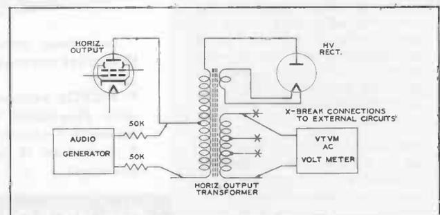
Figure 1. Test Equipment Connections for Checking Horizontal Output Transformer.
