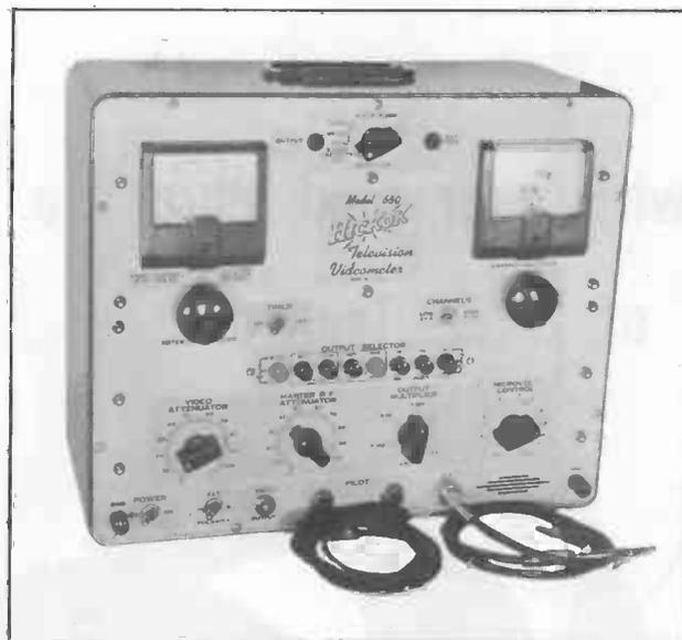
Figure 1. The Hickok Model 650 Videometer.
