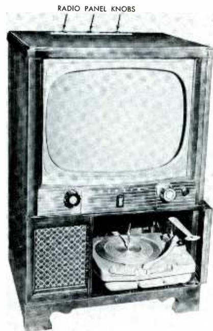
Fig. 12. Front View of Zenith Model L2281 RU Showing Radio Tuning Knobs.
