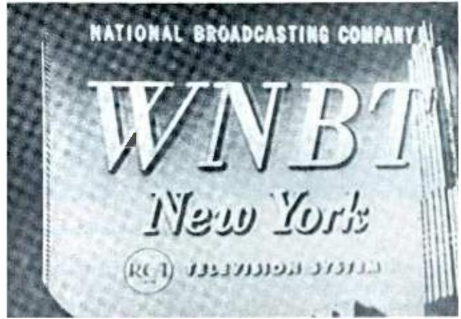
Fig. 4. "Spook" Interference With Signal of Normal Strength.
