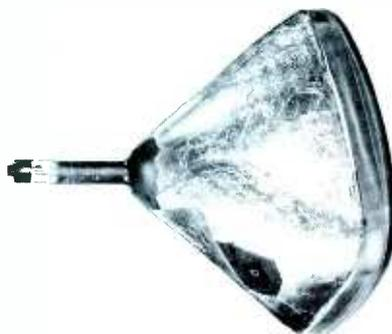
Fig. 4. Picture Tube Which Has Been Shielded With Aluminum Foil.
