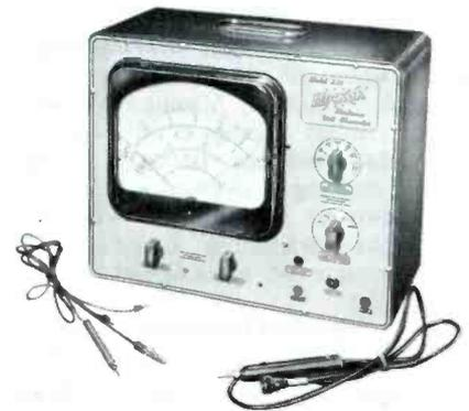
Four panel controls are provided as follows: FUNCTION SELECTOR, RANGE SELECTOR, ZERO ADJ, and OHMS ADJ. The function selector positions are: OFF, +DC, -DC, AC, and OHMS.
