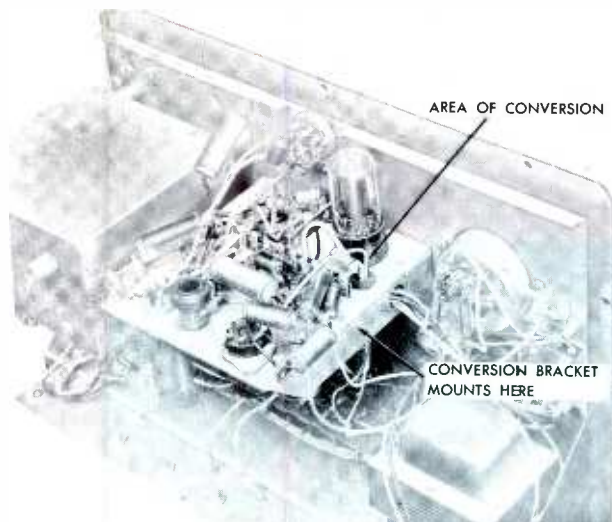
Fig. 2. Two views of the Hickok Model 650 Chassis Showing the Area of Conversion.
