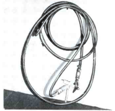
Fig. 4. View of Air Hose Used for Injecting Antistatic Powder Into Tires.
