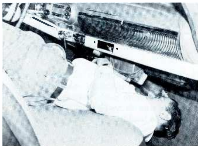
Fig. 7. View of New Radio Being Placed Into Position.
