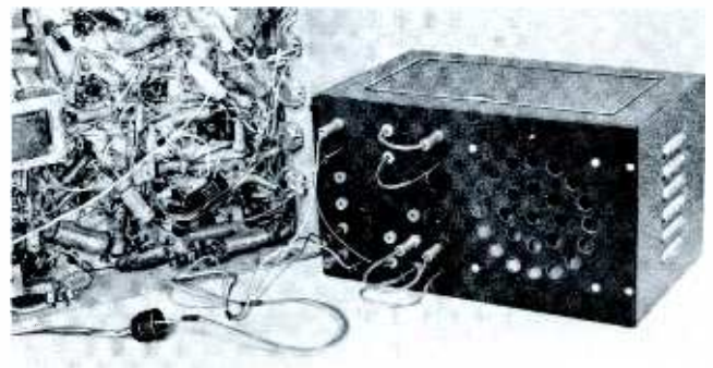
Fig. 5. Test Speaker Connections to RCA Victor Chassis KCS47E.
