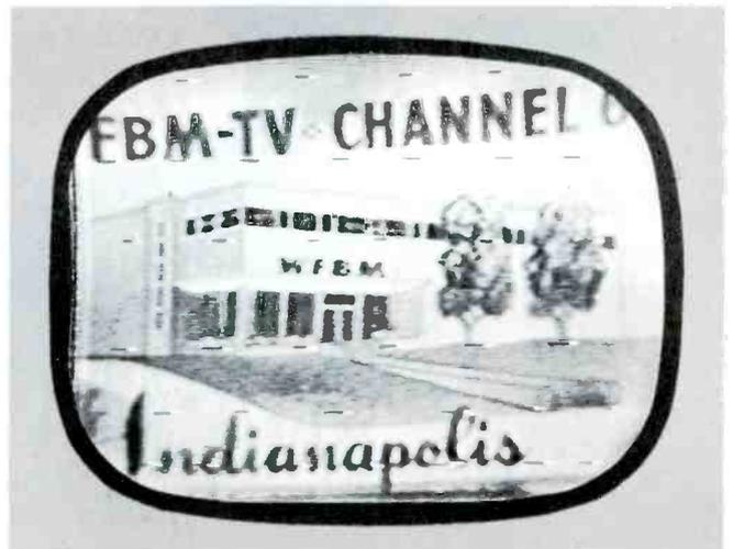
Fig. 6. Ignition Interference.
