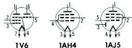
**Fig. 6. Base Diagrams for the Subminiature Tubes Used in the Motorola Model 54L1.**
