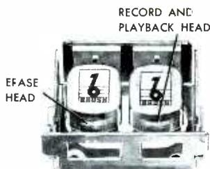
**Fig. 6. Erase Head and Record-Playback Head Used on TDC130 Tape Recorder.**
