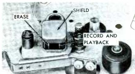
**Fig. 4. Combination Erase, Record, and Playback Head Used on Federal (F-M-E) Model 37-B Tape Recorder.**
