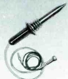
**REMEMBER** that the high voltage (up to 30,000 volts and more) must be set to the specified value before adjusting purity and convergence. The RCA Volt-Ohmysts can be used with the RCA High Voltage Probe (WG-289 and WG-206 Multiplier Resistor) to measure dc voltages up to 50,000 volts.
