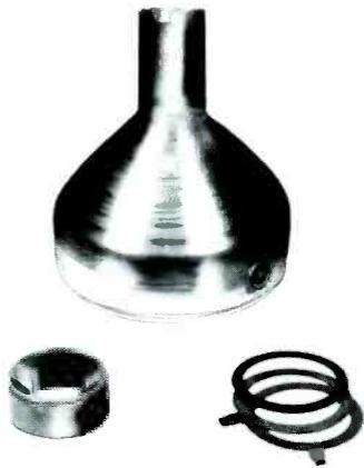
**Fig. 5. A Centering-Magnet Assembly With the Centering Magnets Removed.**
