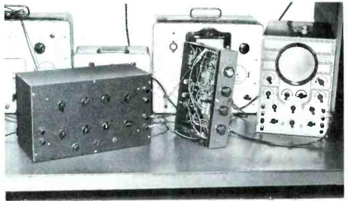
Unfortunately, this requires an extra scope since one is needed to observe the output of the amplifier. If only one scope is on hand, the only alternative is to employ a meter which operates as a VTVM for measuring AC volts. Ordinarily, those meters which use dry rectifiers are not sufficiently accurate at the higher audio frequencies; therefore, a multimeter will not work satisfactorily for monitoring the signal from the audio generator.
