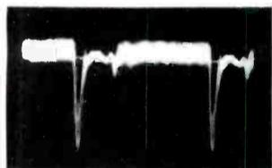
Fig. 6. Q Signal Produced by the Color-Stripe Signal.
