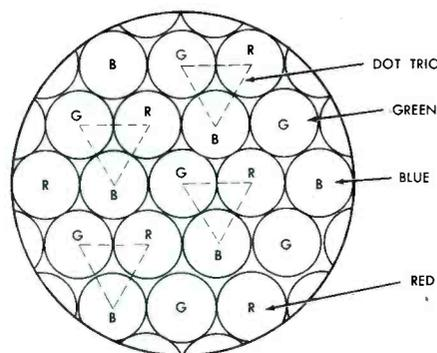
Fig. 9-4. A Portion of the Phosphor-Dot Screen Showing the Arrangement of the Dot Trios.
