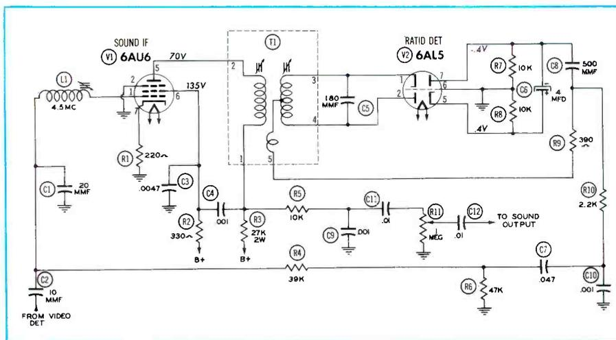
**Fig. 4. Reflex Amplifier Used in Sound Section of Admiral Chassis 18XP4BZ.**
