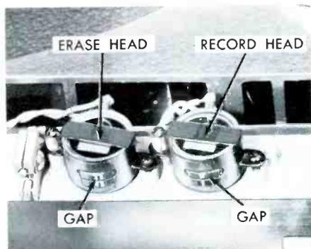
Fig. 1. High-Frequency Erase Head Used in Berlant Model BR-1 Broadcast Recorder.
