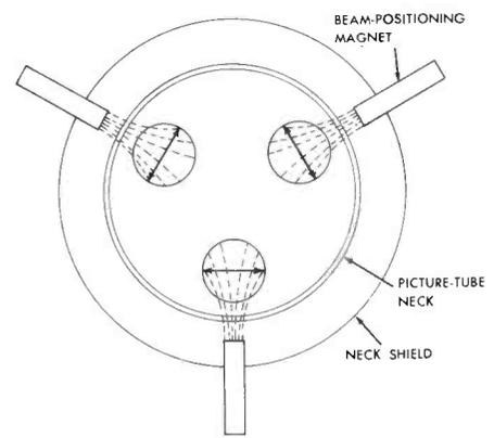
**Fig. 9-16. Arrows Showing Direction of Beam Movement as a Result of the Magnetic Fields Around the Beam-Positioning Magnets.**
