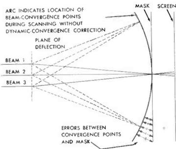
**Fig. 9-11. Drawing from Which the Necessity for Dynamic Convergence Is Apparent.**
