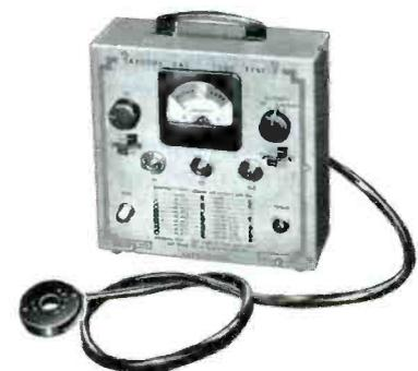
Fig. 4. Authorized Cathode-Ray Tube Tester.
