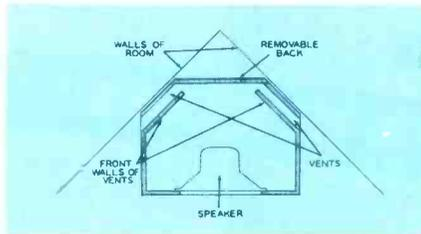
**Fig. 4. "Floor Plan" of Bass-Ultraflex Cabinet.**
