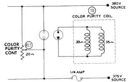
**Fig. 3. Partial Schematic of a Color Receiver Showing Defective Circuit in Case No. 1.**
