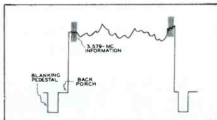
**Fig. 1. Position of Color Information Added to Standard Monochrome Signal.**
