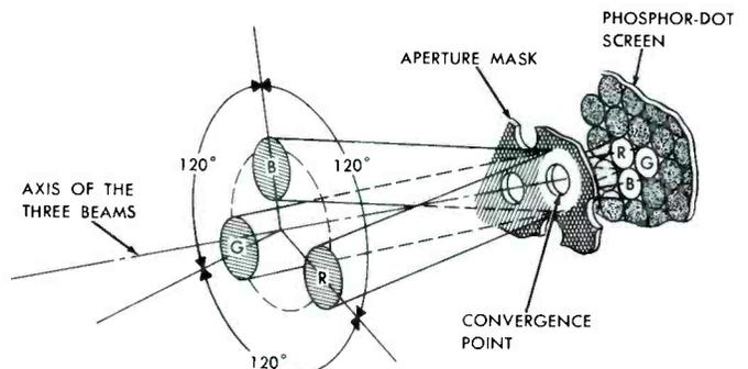
Fig. 9-8. The Relation Between Electron Beams, Aperture Mask, and Phosphor Screen in the Color Picture Tube.
