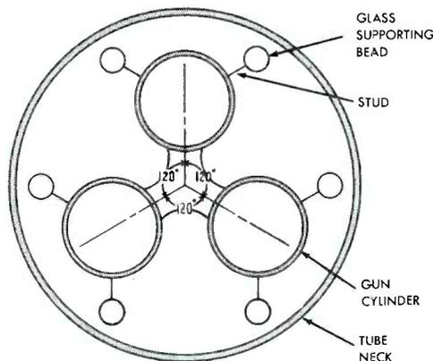
**Fig. 9-9. End View of the Gun Assembly in the Color Picture Tube.**
