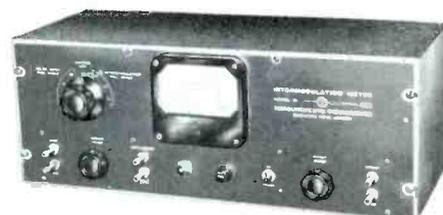
Fig. 4. Intermodulation Meter—Measurements Model 31.
