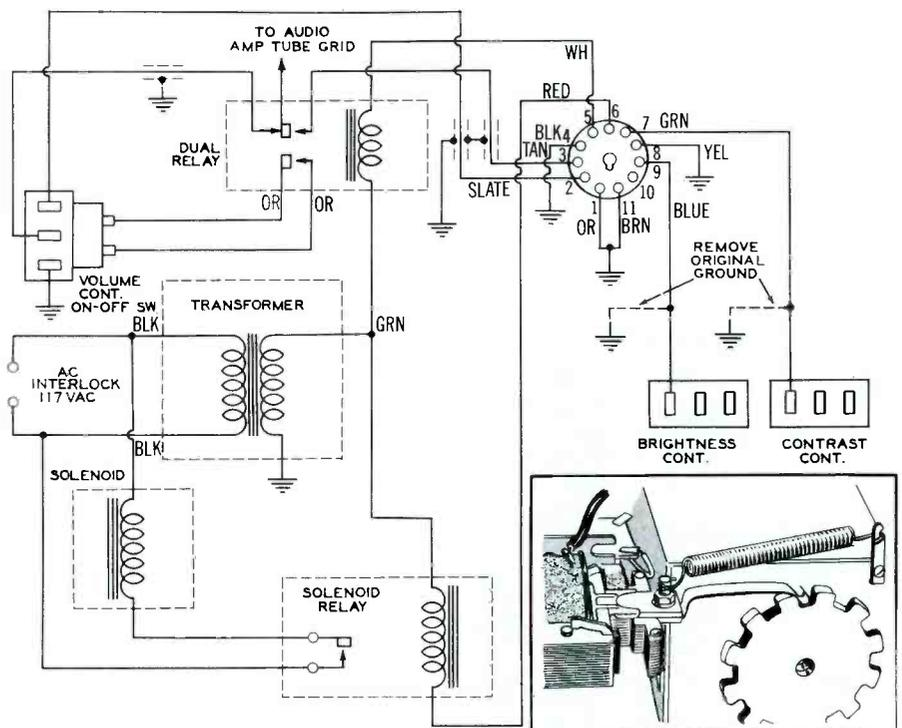
**Fig. 6. Receiver Wiring in the Remot-O-Matic Installation.**
