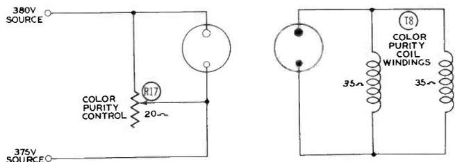
**Fig. 9-17. Schematic Drawing of the Color-Purity Coil and Control Circuit Used in the RCA Victor Model CT-100 Color Receiver.**
