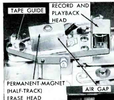
Fig. 4. Permanent-Magnet Erase Head in Wilcox-Gay Recordia Model 4F10.
