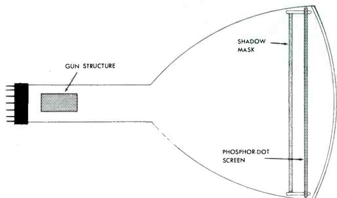
Fig. 9-2. Drawing Showing the Locations of the Three Major Parts in the Color Picture Tube.
