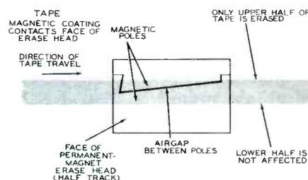
Fig. 6. Drawing Which Shows How Tape Moves in Contact With Face of Permanent-Magnet Erase Head When Recorder Is Operating in the Record Mode.
