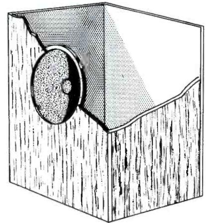
Most totally enclosed units cannot be classed as genuine infinite baffles because their small dimensions do not provide the necessary cubic content. Consequently, the full benefits of the true infinite baffle are not realized when these smaller enclosures are used.
