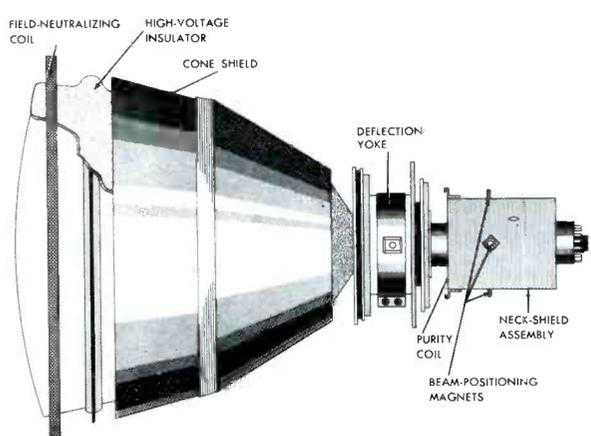
**Fig. 9-14. Auxiliary Components Used with a Three-Beam Color Picture Tube that Employs the Electrostatic Convergence Principle.**
