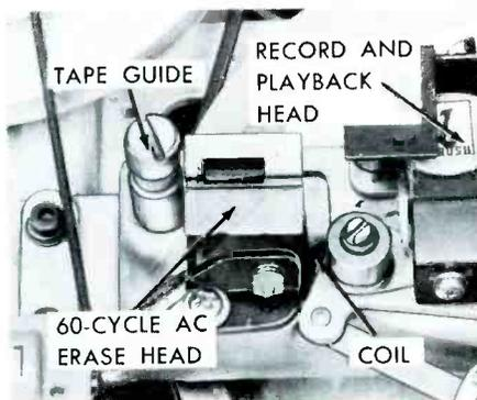
Fig. 3. Erase Head Using 60-Cycle AC in Ampro Model 755 Tape Recorder.
