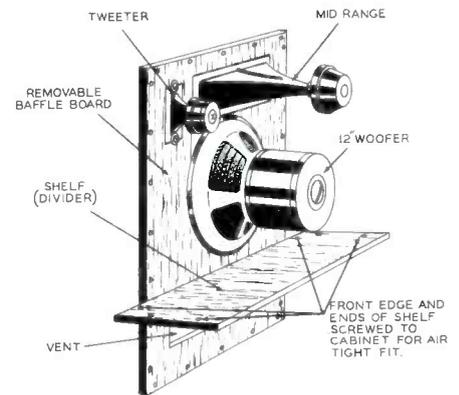
Fig. 1. Baffle-Board Assembly of Home-Constructed Enclosures.
