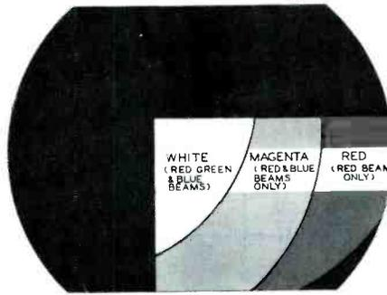
**Fig. 2. Symptoms in Case No. 1 During the Reproduction of a Monochrome Image.**
