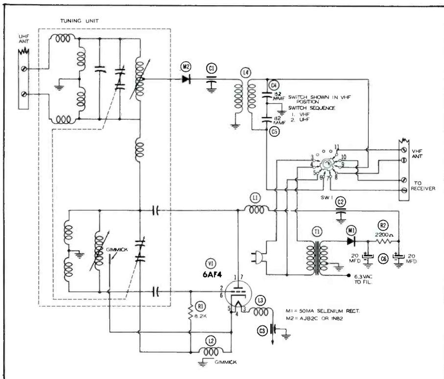
Fig. 6. Schematic of I. T. I. Model IT-150R Ultra-tuner.
