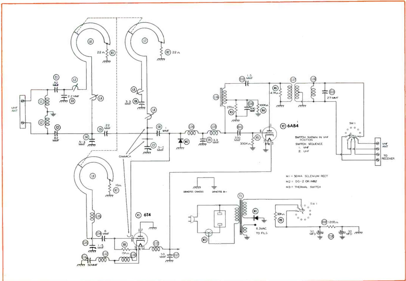
Fig. 2. Schematic of Blonder-Tongue Model BTU-2B UHF Converter.
