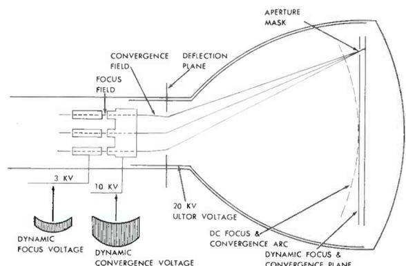
Fig. 9-27. Plane of Convergence and Focus After Application of Dynamic Voltages.
