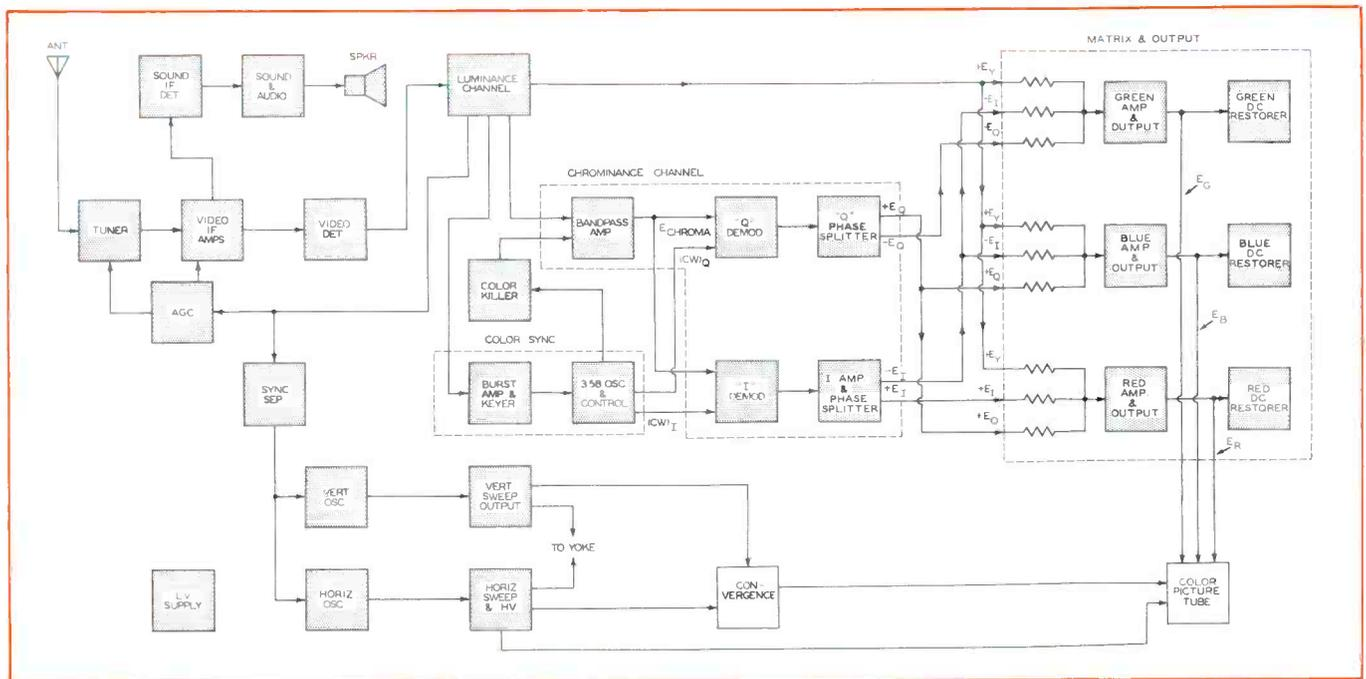
Fig. 9-1. Complete Block Diagram of a Color Receiver Showing Sections Previously Discussed.
