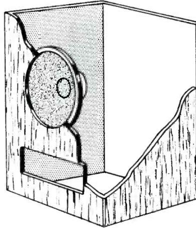
The bass reflex is a totally enclosed unit that is equipped with an opening or vent by which the cabinet is tuned. Very good low-frequency response can be obtained when the enclosure is large, is constructed solidly, and is used with a suitable loudspeaker which has a low resonant frequency.
