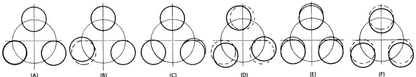
**Fig. 9-10. Drawings Illustrating Misalignment of the Electron Guns. The Dashed Circles Indicate the Correct Position of the Guns. (A) Correct Alignment. (B) One Gun Displaced with Respect to the Other Two. (C) One Gun Tilted. (D) All Three Guns Slightly Rotated. (E) All Three Guns Tilted. (F) Central Axis of the Gun Assembly Displaced from the Central Axis of the Tube.**
