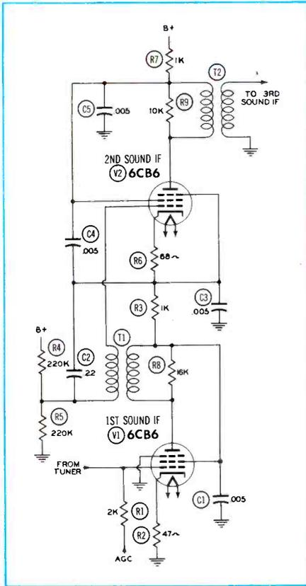
**Fig. 3. Series Type of B+ Supply for Two Video IF Amplifiers in Admiral Chassis 18XP4BZ.**
