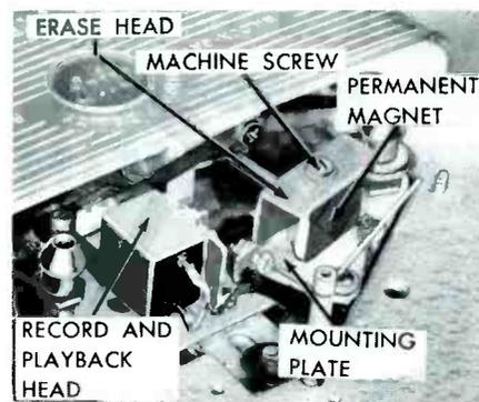
Fig. 5. Another View of Permanent-Magnet Erase Head and Its Mounting Arrangement.
