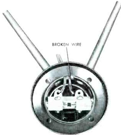
**Fig. 8. Broken Wire in Base of Indoor Antenna.**
