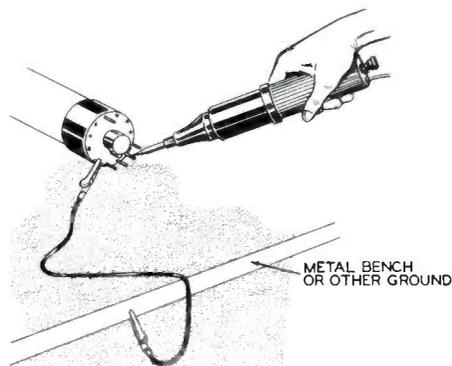
Fig. 2. Using the High-Voltage Coil to Burn Out Shorts.
