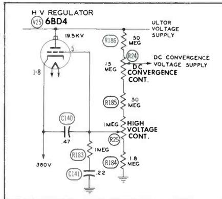
**Fig. 5. Partial Schematic of a Color Receiver Showing Defective Circuit in Case No. 2.**
