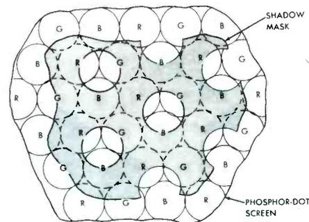
Fig. 9-6. View of Phosphor Screen As Seen Through Aperture Mask.
