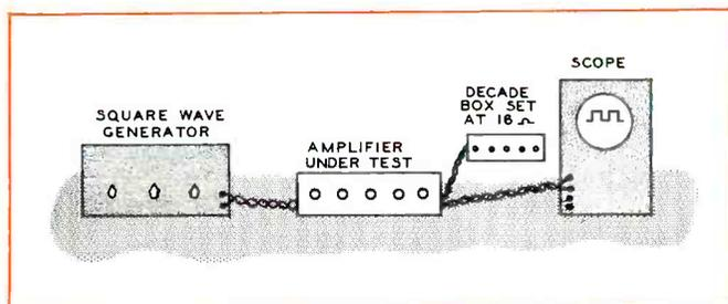
Fig. 1. Diagram of Test Setup Using Square-Wave Generator.
