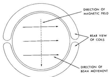
**Fig. 9-18. The Direction of Beam Movement Is Shown to be at Right Angles to the Magnetic Field of the Purity Coil.**
