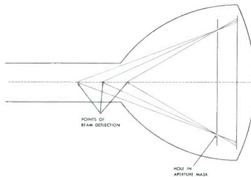
Fig. 9-20. Each Beam Path Through the Holes at the Edges of the Shadow Mask is Shown to be at a Different Angle for Each Position of the Yoke.
