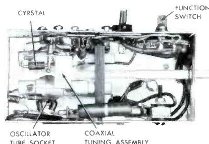
Fig. 7. Tuning Assembly in I. T. I. Model IT-150R Ultra-tuner.
