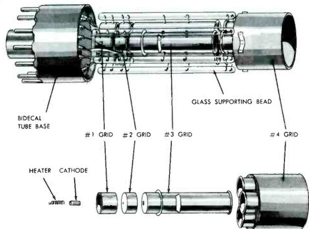
**Fig. 9-12. Three-Gun Assembly with an Exploded View of One of the Guns.**
