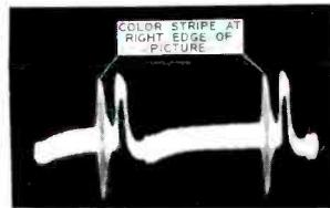
Fig. 3. Color Stripe at Input of Demodulators.
