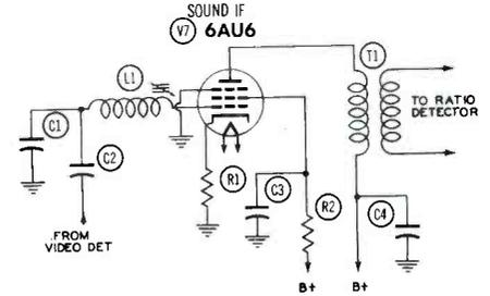
**Fig. 5. Simplified Schematic of Reflex Amplifier Showing Impedances Presented to 4.5-Mc Signal.**
