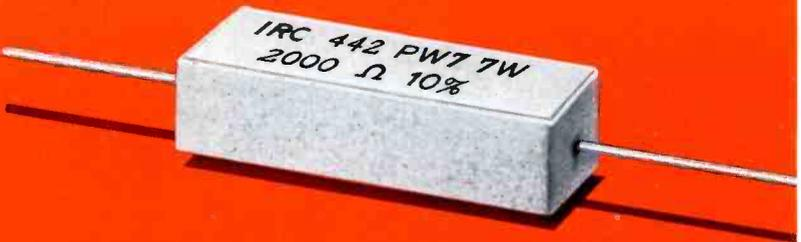
Here are wire wound power resistors designed for today's servicing requirements. New, rectangular design is more compact. Famous IRC element is sealed in ceramic case for complete insulation and protection. Axial leads are easily soldered and speed replacement. Clear, permanent markings give full identification.
