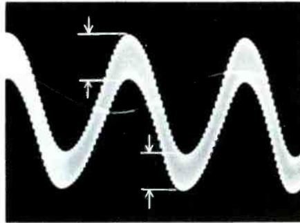
Fig. 5. Waveform Showing Intermodulation Distortion.
