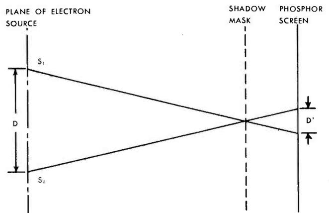
Fig. 9-7. Geometry of Shadow-Mask Principle.
