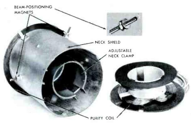
**Fig. 9-15. Physical Appearance of Color-Purity Coil and One of the Beam-Positioning Magnets When Removed from the Neck-Shield Assembly.**
