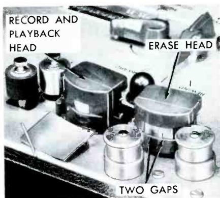
Fig. 2. High-Frequency Erase Head Used in Magnecord Model M30 Tape Recorder.
