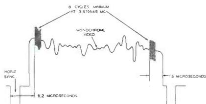
Fig. 1. Transmitted Monochrome Signal with Color Stripe Added.
