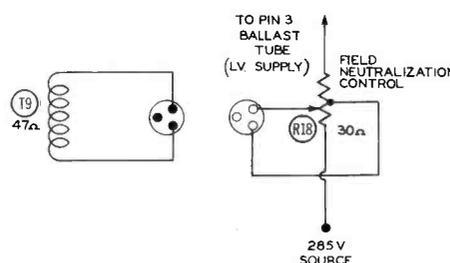
Fig. 9-22. Schematic of the Field-Neutralizing Coil and Its Associated Control Circuit as Used in the RCA Victor Model CT-100 Color Receiver.
