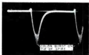
Fig. 7. Signal at the Plate of the Burst Amplifier.
