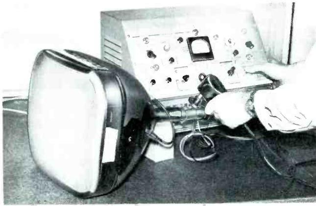
Fig. 3. Method of Applying the Vibrator When Making a Cathode Weld.
