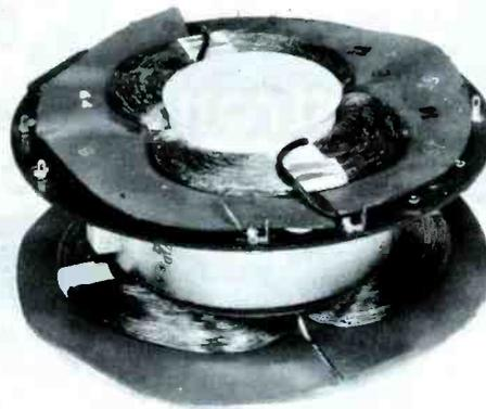
Fig. 9-19. Deflection Yoke Used with a Three-Beam Color Picture Tube.
