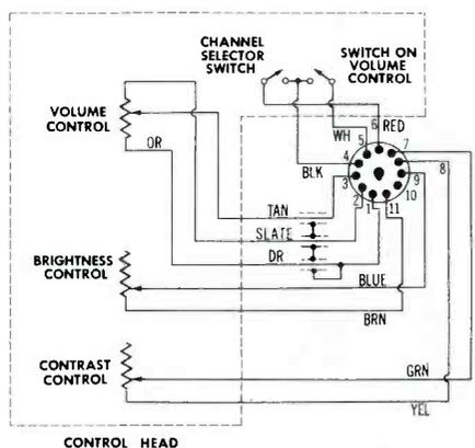
**Fig. 5. Schematic of the Remot-O-Matic Control Head and Connecting Cable.**
