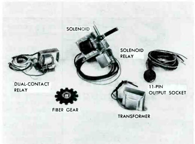
**Fig. 4. Receiver-Mounted Components in the Remot-O-Matic Installation.**
