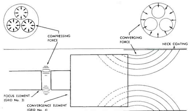
**Fig. 9-13. Drawing Which Shows the Location of the Electrostatic Fields at Each End of the Convergence Element.**
