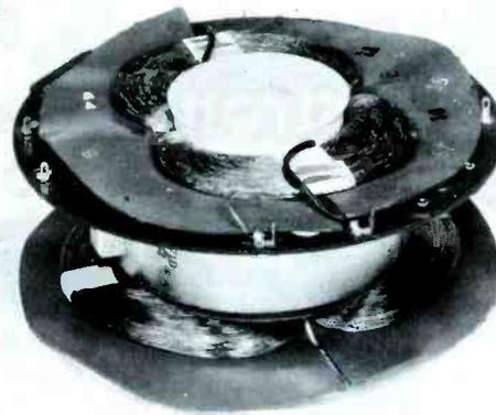
Fig. 9-19. Deflection Yoke Used with a Three-Beam Color Picture Tube.
