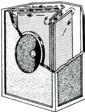
Many horns and curiously shaped things called horns are used in loudspeaker systems. Small horns, in conjunction with diaphragm type speaker units, are used as midrange loudspeakers and tweeters. But here we are more concerned with the necessarily larger horns used with cone type speakers for the purpose of reproducing the low-frequency tones.
