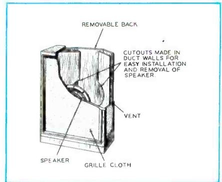
**Fig. 5. Cutaway View of Model BL-220 Bass-Ultraflex Cabinet.**
