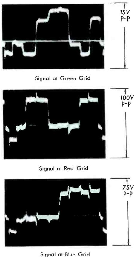
**Fig. 7. Waveforms Observed at the Picture-Tube Grids in Case No. 3 During a Color-Bar Transmission.**
