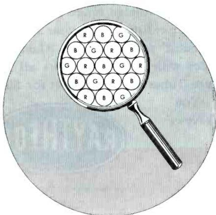
Fig. 9-3. Arrangement of Phosphor Dots on the Screen of the Color Picture Tube (As Seen Under Magnifying Glass).
