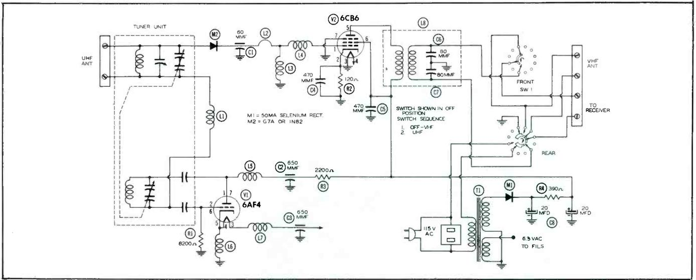
Fig. 4. Schematic of Granco Model SLU UHF Converter.
