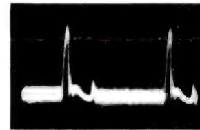
Fig. 5. I Signal Produced by the Color-Stripe Signal.
