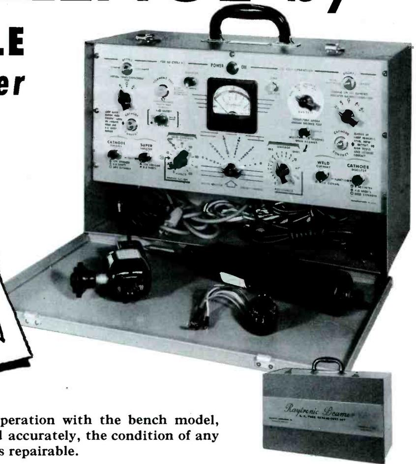
This portable instrument, identical in operation with the bench model, will make 8 tests to show, positively and accurately, the condition of any TV picture tube—and whether or not it is repairable.
