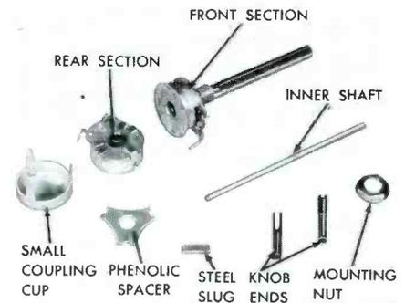
**Fig. 7. Parts Used to Construct a Mallory Dual Control.**
