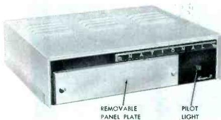
Fig. 1. Front View of National Horizon 20 Amplifier.
