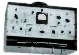
Case cover removed for bench work in horizontal position; rubber base lugs.
