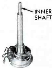
(A) Inner Shaft Inserted Point Downward Into Outer Shaft and Ready for Cutting.
