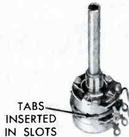
(D) Coupling Cup Fastened to Front Section.
