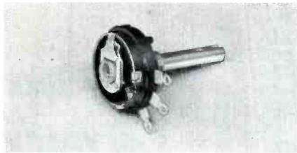
(A) Outer Shaft Inserted in Base Element of Panel Section.
