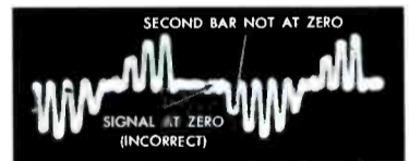
Fig. 14. Signal at Plate of Q Demodulator Illustrates Improper Cancellation of the Second-Bar Signal.
