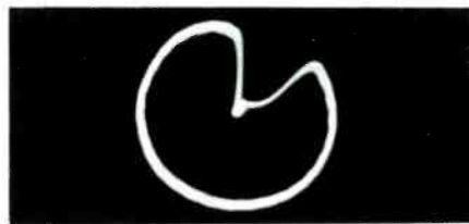
(B) Notched Circle Showing Incorrect Adjustment of the Hue Phase Control.
