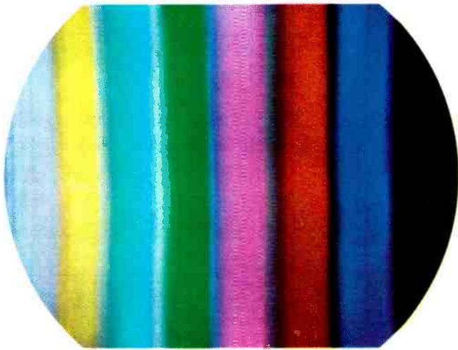
Fig. D7. Color-Bar Pattern in Which Colors Are Normal.
