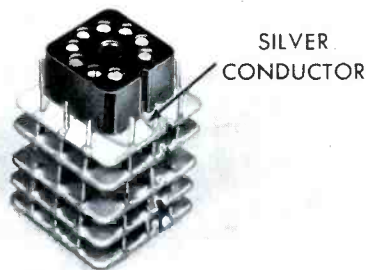
Fig. 9. Silver Conductors on Top of Wafer No. 1.
