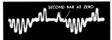
Fig. 13. Signal at Plate of Q Demodulator Illustrates Proper Cancellation of the Second-Bar Signal.
