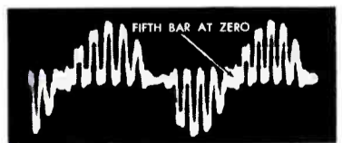
Fig. 11. Signal at Plate of I Demodulator Illustrates Proper Cancellation of the Fifth-Bar Signal.
