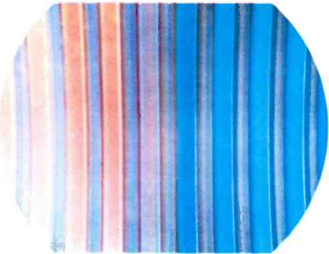
Fig. 2. Pattern Indicating Loss of Q Signal.
