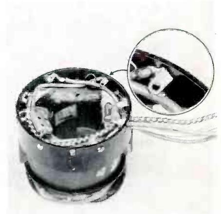
Fig. 2. Short Between Wire and Terminal in Deflection Yoke.
