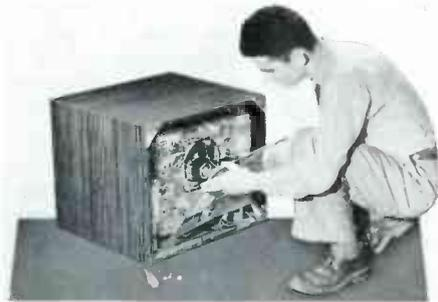
Fig. 7. The CBS-Columbia Model 3T615 Television Receiver With Cabinet Back Removed and With the Fiber Board Which Covers the Wiring Side of the Chassis Partially Removed.
