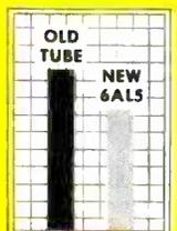
**NEW 6BK7-A, 6BQ7-A, 6BZ7.** *Improved heater design* provides better heater-cathode insulation. Cuts shorts to a minimum, acts to prevent tube burn-outs.
