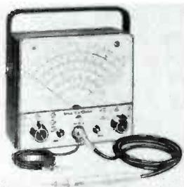
Just announced by Radio Corporation of America is the WV-98A Senior Voltohmyst. This new meter measures DC voltages to 1,500 volts, AC voltages (rms and peak to peak) to 4,200 volts, and resistance to 1,000 megohms.
