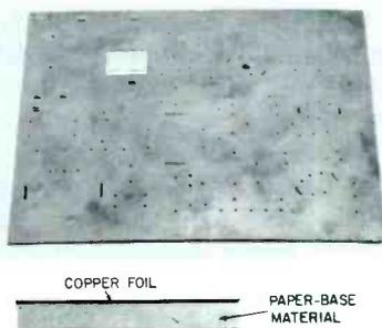
Fig. 1. Prepunched Copper Foil on Paper-Base Material. (inset—Drawing Showing End View of Enlarged Copper-Clad Board.)
