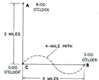
Fig. 6. Sketch of Paths Used As Analogy for Delay Line.
