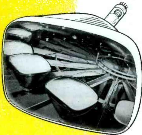
The very latest and up to date manufacturing techniques backed up by modern mass production equipment as illustrated by this mechanized aluminization rack.
