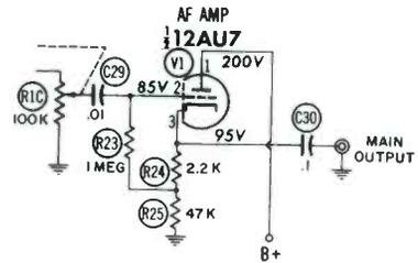
Fig. 2. Cathode-Follower Output Stage Used in Fisher Model 50-C Master Audio Control.
