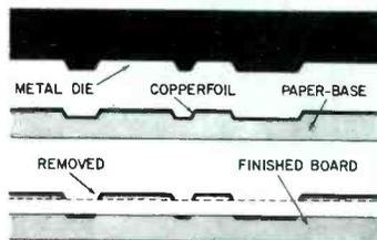
Fig. 5. Drawing Showing Embossed Type of Printed Board and Some Production Details.
