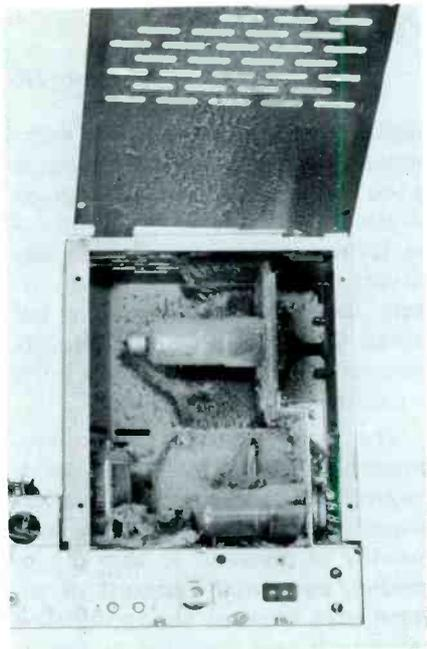
Fig. 2. Dust-Filled High-Voltage Compartment Before Cleaning.
