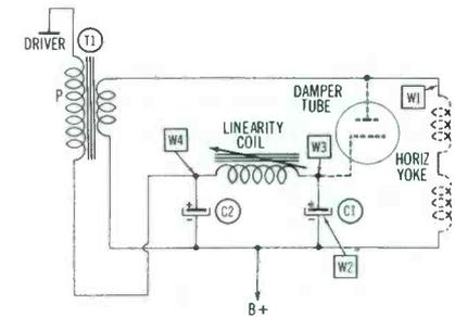
(A) Boost and Linearity-Coil Circuits.
