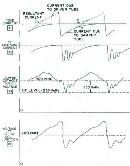
(B) Waveforms of Currents and Voltages.
