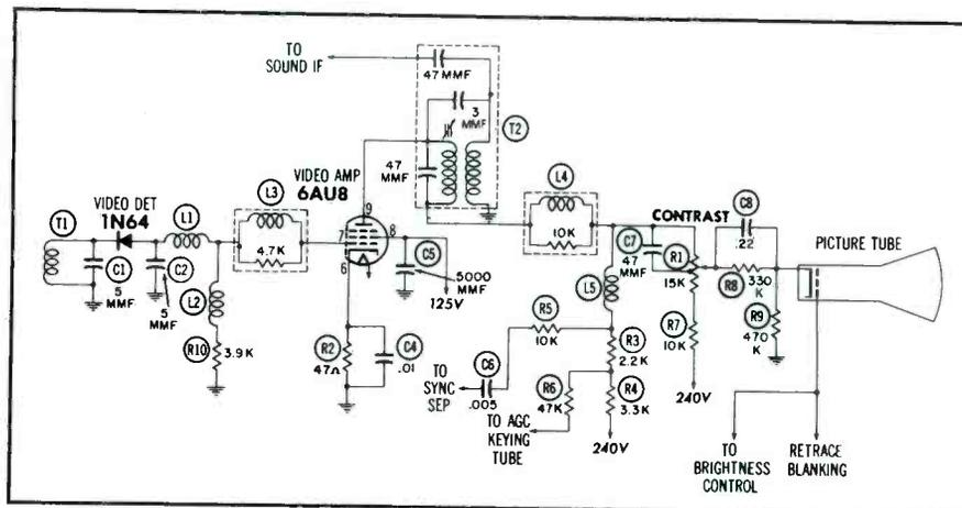
Fig. 3. Schematic Diagram of a Direct-Coupled Video Amplifier.
