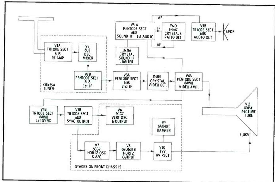
Fig. 3. Block Diagram of the RCA Victor Portable Television Receiver.
