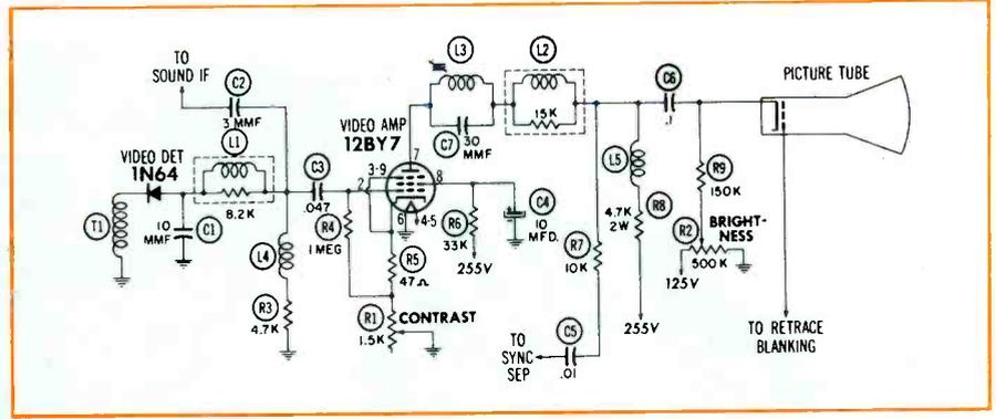
Fig. 1. Schematic of a Typical Single-Stage Video Amplifier Employing AC Coupling.
