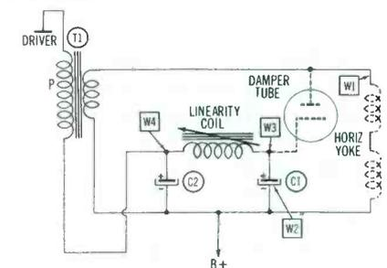
(A) Boost and Linearity-Coil Circuits.
