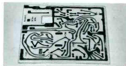
Fig. 2. Etched Board With Resist on Circuit Pattern.
