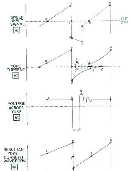
(B) Waveforms of Currents and Voltages.
