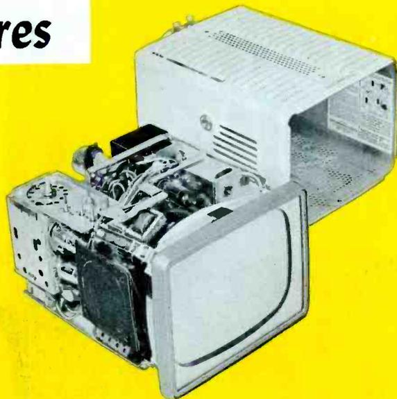
Fig. 1. RCA Victor Portable Television Receiver Chassis and Cabinet.
