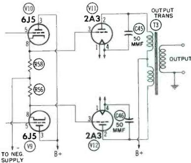
Fig. 4. Cathode-Follower Driver Stage Used in Brook Model 10C3 Amplifier.
