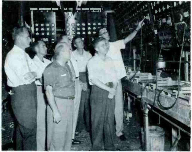
One stop on plant tour was final re-forming operation where completed capacitors are given several-hour final aging.
