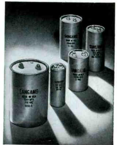
The Sangamo DCM Electrolytic Capacitor is housed in a seamless, drawn aluminum container with gasket-sealed molded alkyd resin base thermosetting plastic cover. Detail of cover construction insures minimum contact resistance in current carrying members and provides an adequate safety vent in case of heavy overload.
