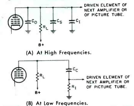
Fig. 2. Equivalent Load Circuits of an RC-Coupled Video Amplifier.
