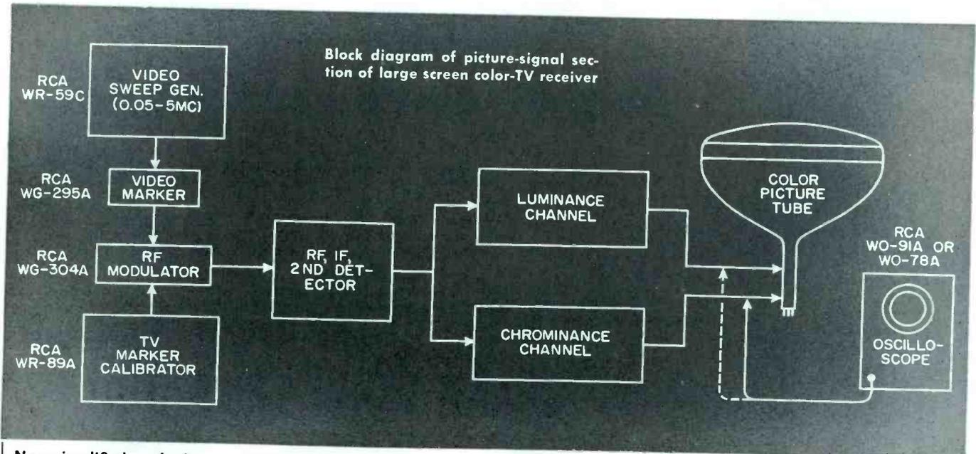
**New simplified method essential for the correct alignment of chrominance circuits and for checking overall frequency response of color-TV receivers from antenna to picture tube—rapidly! accurately!**
