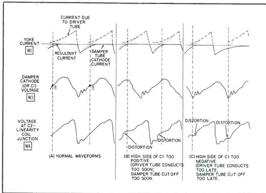
Fig. 3. Waveforms Required to Produce a Linear Yoke Current.
