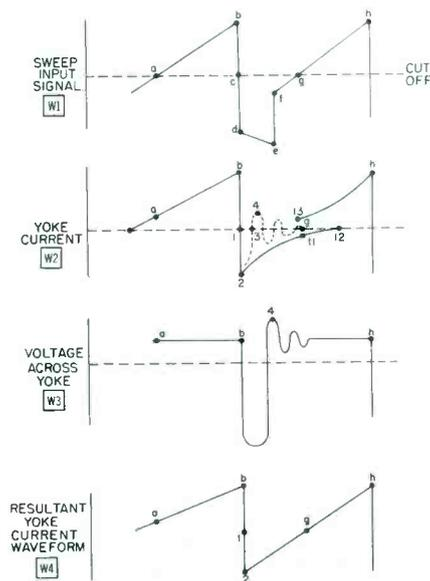
(B) Waveforms of Currents and Voltages.
