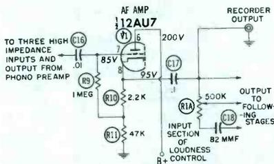
Fig. 3. Cathode-Follower Input Stage Used in Fisher Model 50-C Master Audio Control.
