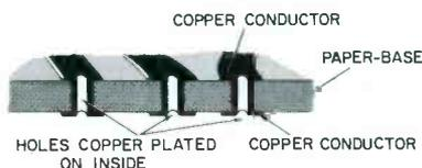
Fig. 4. Drawing Showing Details of Copper Coating on Both Sides of Board and Through Holes.
