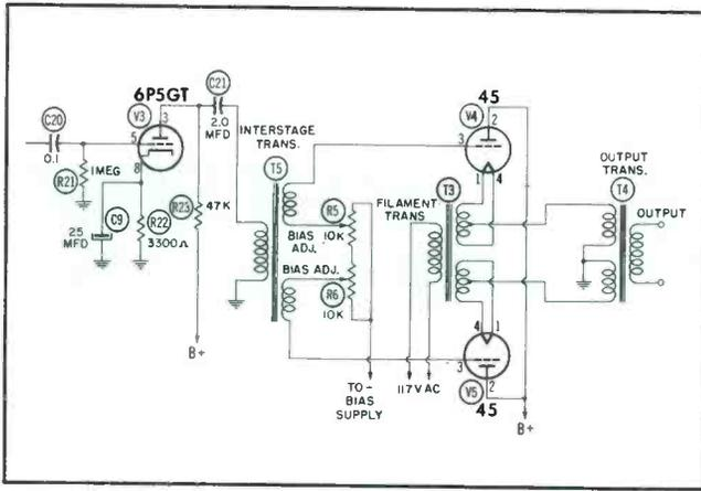
Fig. 5. Cathode-Follower Power Output Stage Used in Experimental Amplifier.
