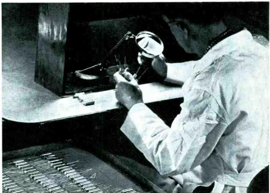
**OIL-FILLED CAPACITORS** are subjected to vacuum under elevated temperatures, then are individually examined to insure complete hermetic seal.
