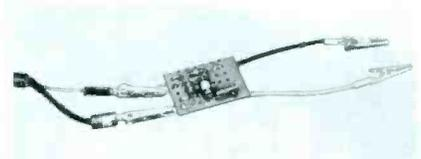
Fig. 11. Small Breadboard Construction of Simple Detector Probe.
