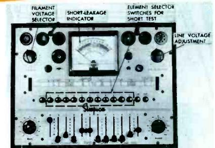
Fig. 2. Typical Tube Tester Which Can Measure Inter-Element Resistances.
