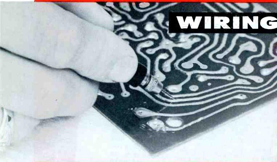
Fig. 1. Using a Sharp Pointed Tool to Locate a Break in the Foil.
