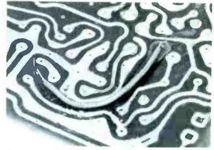
Fig. 4. Conductor Replaced With Wire.
