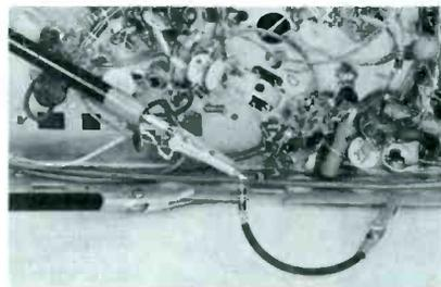
Fig. 5. Pair of Matched Resistors Used in an FM Detector Alignment.
