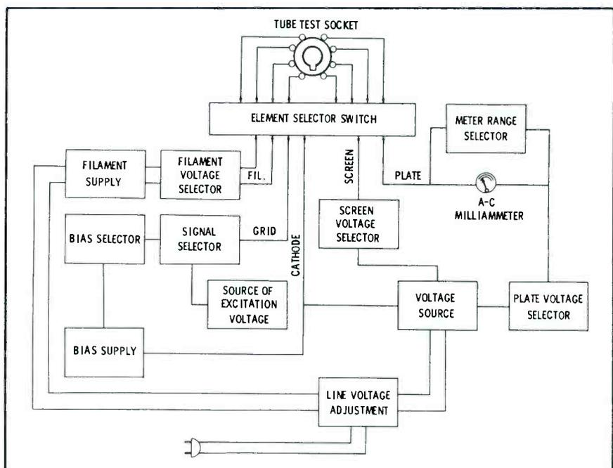
Fig. 5. Simplified Block Diagram of a Transconductance Tube Tester.
