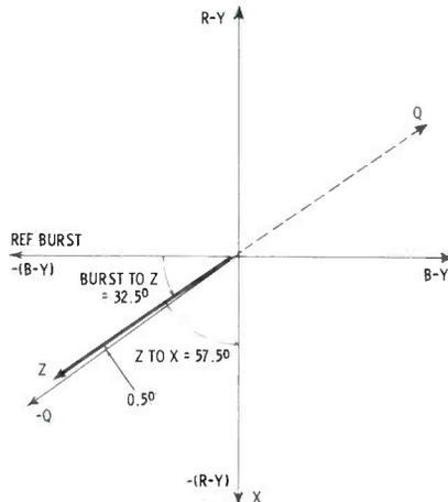
Fig. 8. Phase Relationships Between X, Z, Q, and Burst Axes.
