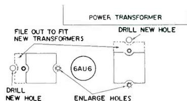
Fig. 4. Metal Work Required.
