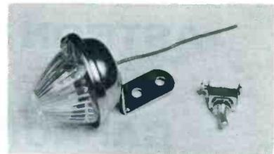
Fig. 3. Small Lamp and Switch for Inside Lighting in Service Truck.
