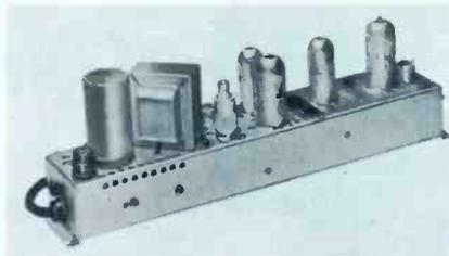
Fig. 4. Single-Channel Amplifier With Gain Between 35 and 38 db and With High Rejection of Adjacent Channels.
