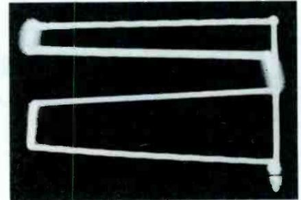
Fig. 2. Square-Wave Presentation Which Was Obtained by Applying Square Wave to Horizontal Input System of Oscilloscope.
