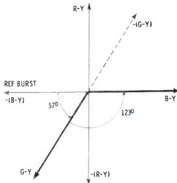
Fig. 7. Phase Relationships Between B-Y, G-Y, and Burst Axes.
