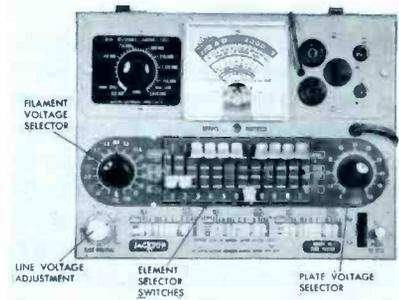
Fig. 4. Commercial Example of an Emission Type Tube Tester.
