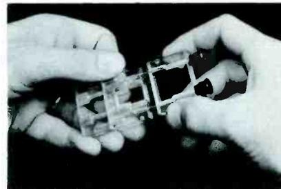
Fig. 3. Hickock Model 75 Impedance-Matching Pad.
