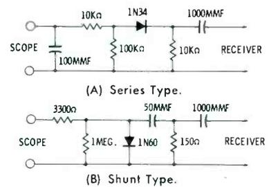
Fig. 10. Two Types of Detector Probes.
