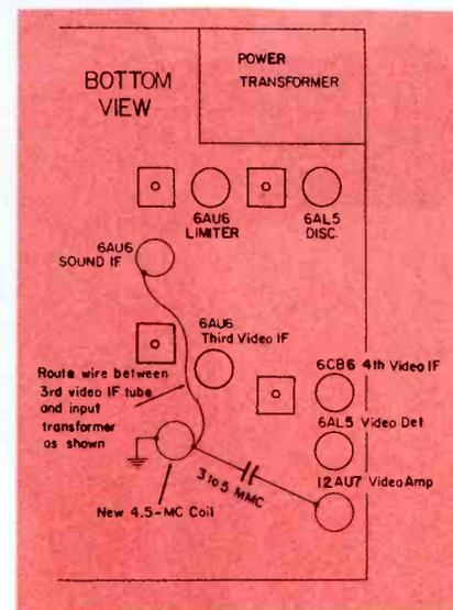
Fig. 2. Chassis Layout Showing Location of New 4.5-mc Coil.
