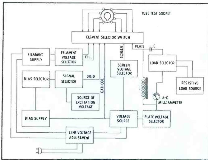
Fig. 7. Block Diagram Showing Basic Setup for Power Output Test.
