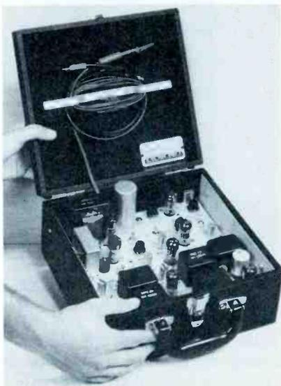
Fig. 8. Hickock Model 660 White Dot-Bar, Color Display Generator.
