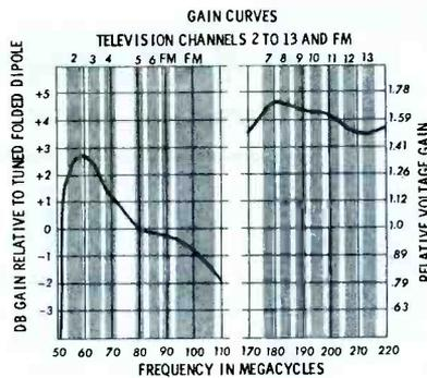
Fig. 3. Mallet Antenna With Separate High Frequency Folded Dipole.
