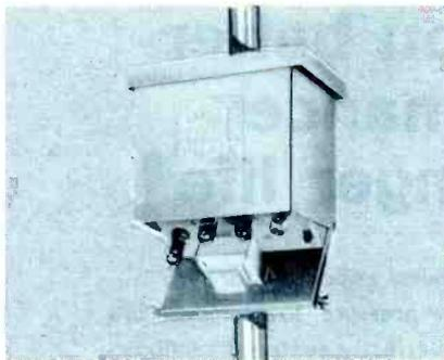
Fig. 1. Antenna-Mounted Booster.
