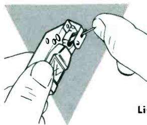
The versatile new Model UX is furnished complete with WEBSTER's WE 122 special, all-speed 2-mil osmium-tipped *push-in* needle. Needle may be removed by pulling out with fingers. Needle may be replaced by placing end in needle chuck and applying light pressure to needle tip (see cut at left).
