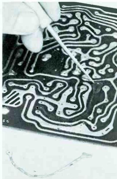
Fig. 3. Conductor Unbonded From Base.
