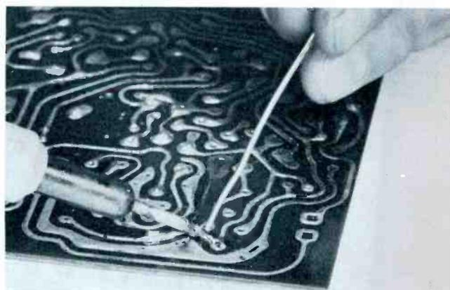
(B) Bonding Wire Bridge to Conductor.
