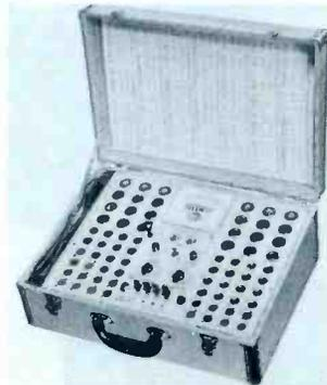
The TeleTest Model T-72 tube tester built by Anko Mfg. Co., Inc., 5042 W. State St., Milwaukee, Wis., checks more than 300 tubes, including series-string types, with a minimum of switching. An array of 72 tube sockets is provided, including 10 spares to allow for future tube designs. A value test is made under full-load conditions, and a test for shorts between adjacent elements can be made without special set-ups. Gas, grid emission, and grid shorts can also be checked.
