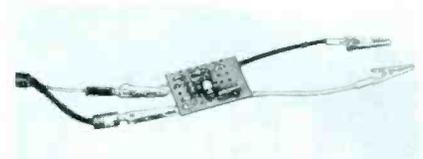
Fig. 11. Small Breadboard Construction of Simple Detector Probe.
