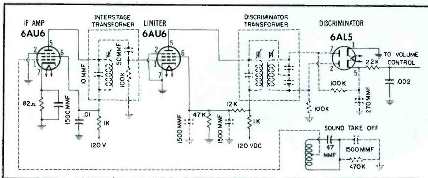
Fig. 1. Schematic of Original RCA Circuit.
