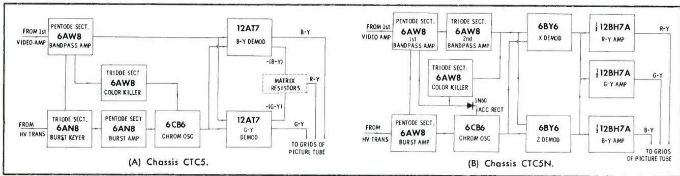
Fig. 6. Block Diagrams of Chrominance Sections of RCA Victor Color Receivers.
