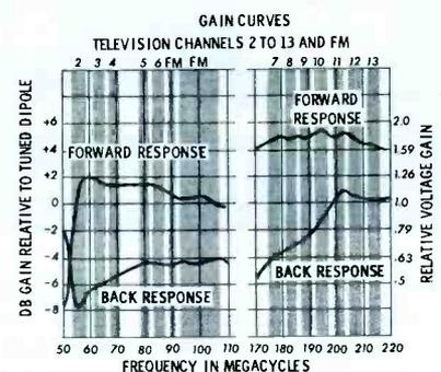
Fig. 4. Conical Antenna.
