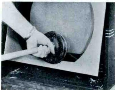
Fig. 1. Plunger Being Used to Remove Safety Glass from TV Set.
