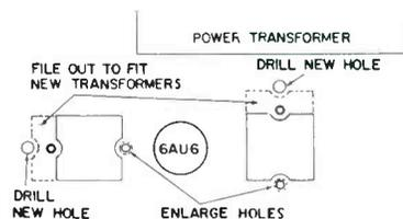
Fig. 4. Metal Work Required.
