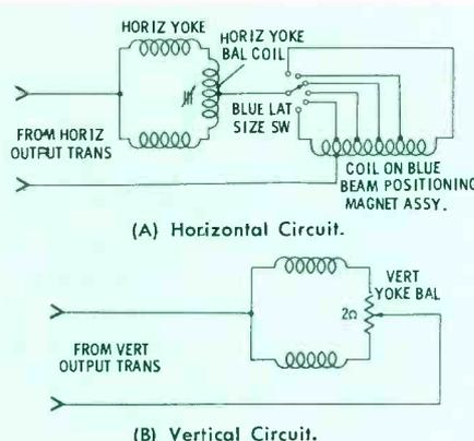
Fig. 2. Simplified Schematic Diagrams of Raster-Size-Correction Circuits.
