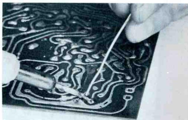
(B) Bonding Wire Bridge to Conductor.
