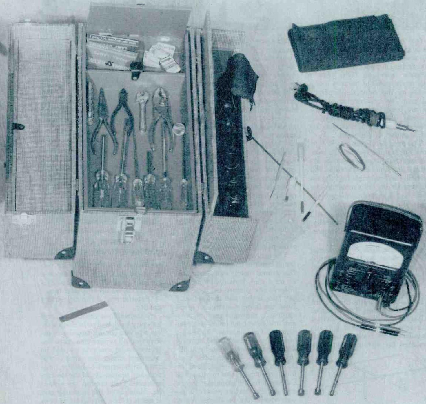
1. Multimeter (sensitivity, at least 20,000 ohms per volt).
