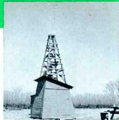
Sample Antenna Under Test. (Rotatable and Tilttable Platform.)
