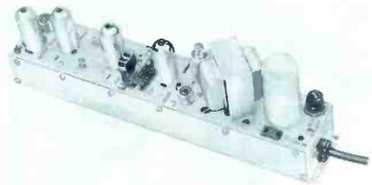
Fig. 2. VHF Converter-Amplifier Which Changes Specified High-Band Signal to a Specific Low-Band Channel. This Unit Provides 33-db Gain.
