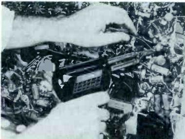
**4 REPAIRING REMOTE-CONTROL TUNING UNITS.** Your Weller Soldering Gun fits neatly into the small spaces between the terminal tabs on telephone-type relay stacks. Also, heat shut-off feature of gun prevents damage to insulation.
