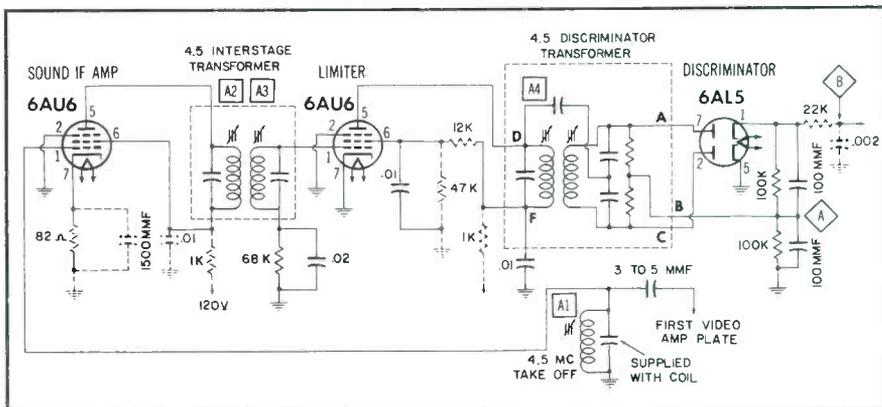
Fig. 3. Schematic of New 4.5-mc Circuit.
