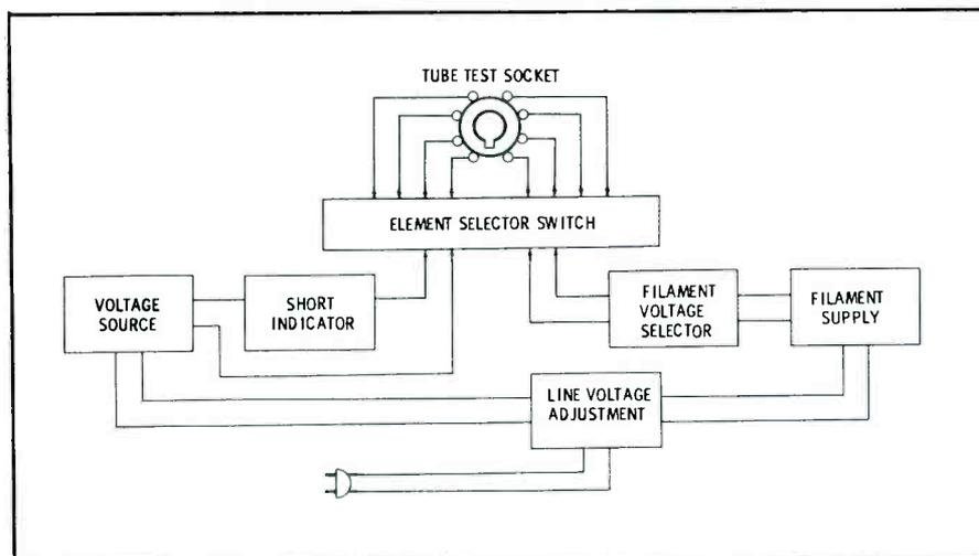
Fig. 1. Block Diagram of Fundamental Short-Circuit Test.
