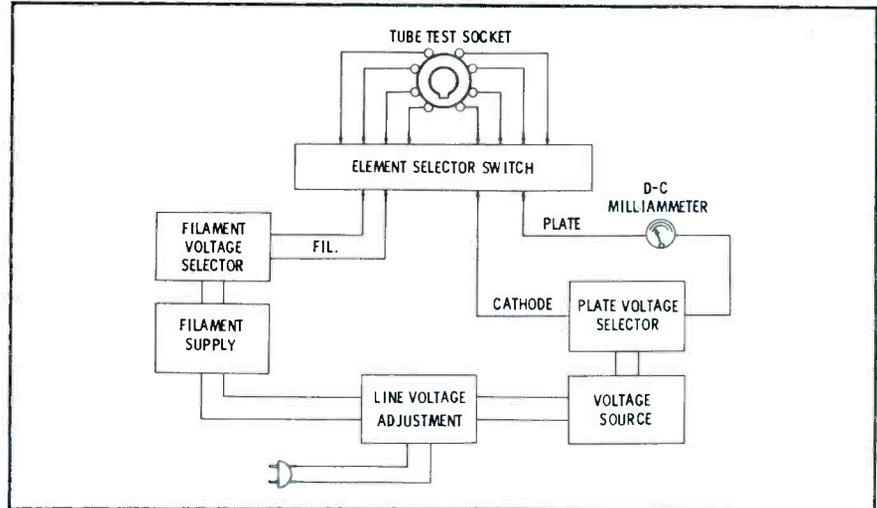
Fig. 3. Simplified Block Diagram of an Emission Type Tester.
