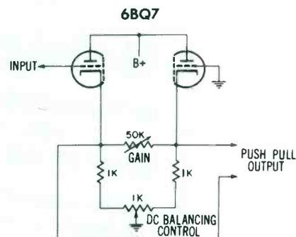
Fig. 4. One Method of Achieving DC Balance for a Push-Pull Output.
