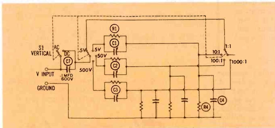
Fig. 1. Typical Attenuator System (with Compensating Adjustments). Found at Input to Vertical Amplifier of Some Oscilloscopes.
