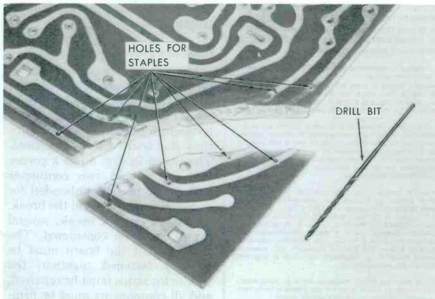
Fig. 6. Holes Drilled to Allow Fastening With Staples.
