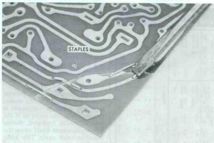
Fig. 7. Uniting the Sections With Heavy Staples.
