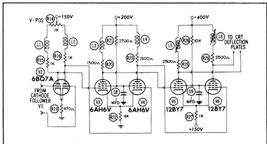
Fig. 3. In This Vertical System, Two Frequency-Governing Adjustments Are Used. These Are L5 and L6.
