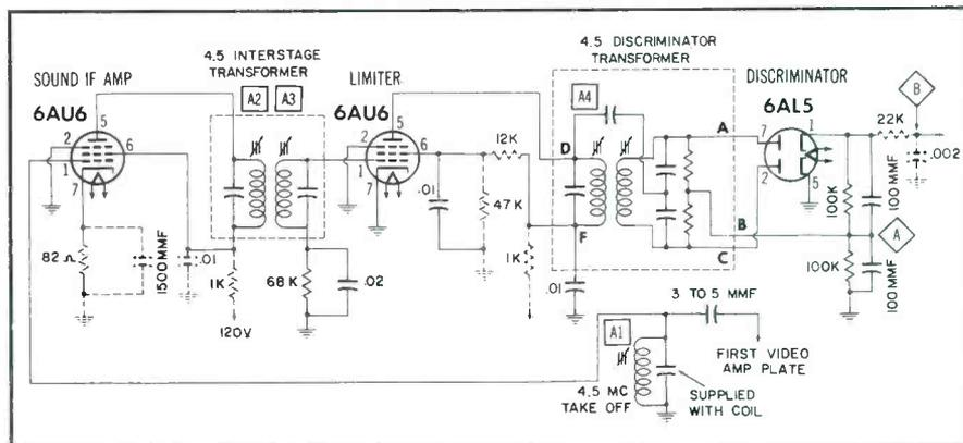
Fig. 3. Schematic of New 4.5-mc Circuit.
