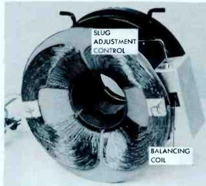
(A) Horizontal Yoke Balancing Coil.
