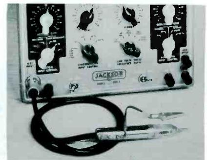
Fig. 9. Detector Probe for Jackson Model CRO-2 Oscilloscope.
