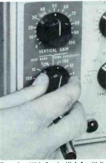
Fig. 1. Wide-Band—High-Sensitivity switch on an oscilloscope.
