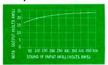
Fig. 1. Input vs. output voltages for a typical 6DT6 detector circuit.
