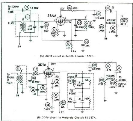
Fig. 2. Schematic diagrams of quadrature-grid detectors.
