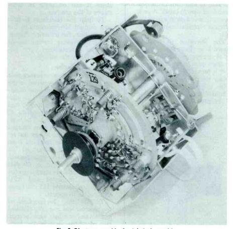
Fig. 2. Disc tuner used in the Admiral portable.
