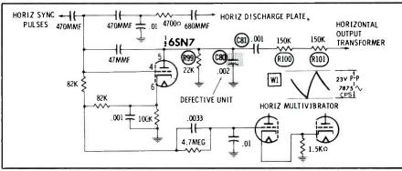
Fig. 2. Triode phase detector for horizontal AFC.
