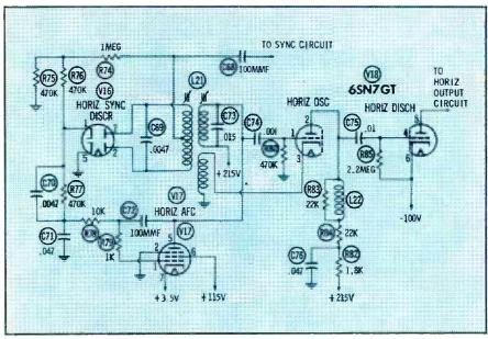
Fig. 1. Circuit diagram of the horizontal-sync stages in George's "tough dog" set.
