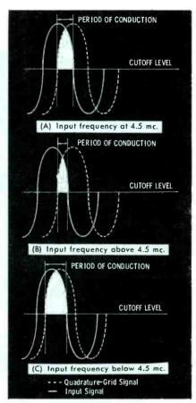
Fig. 3. Plate-current conduction in a quadrature-grid detector.
