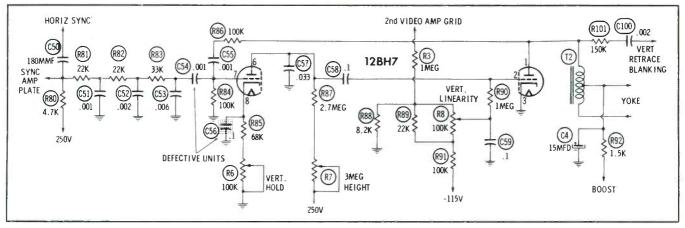
Fig. 3. RC-coupled vertical multivibrator.
