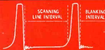
Fig. 3. Positive pulse at color killer plate during monochrome reception.
