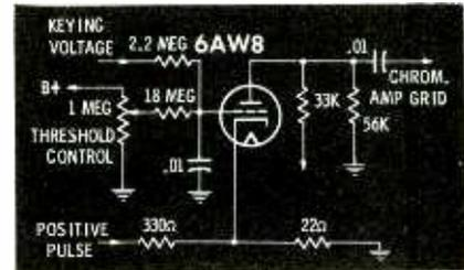
Fig. 6. Color killer circuit used in RCA Victor 21-CS-7815.
