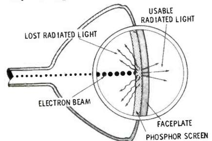
Fig. 2. Light loss in a tube with non-aluminized screen.
