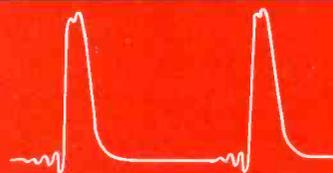
Fig. 2. Negative pulse applied to the grid of the color killer.
