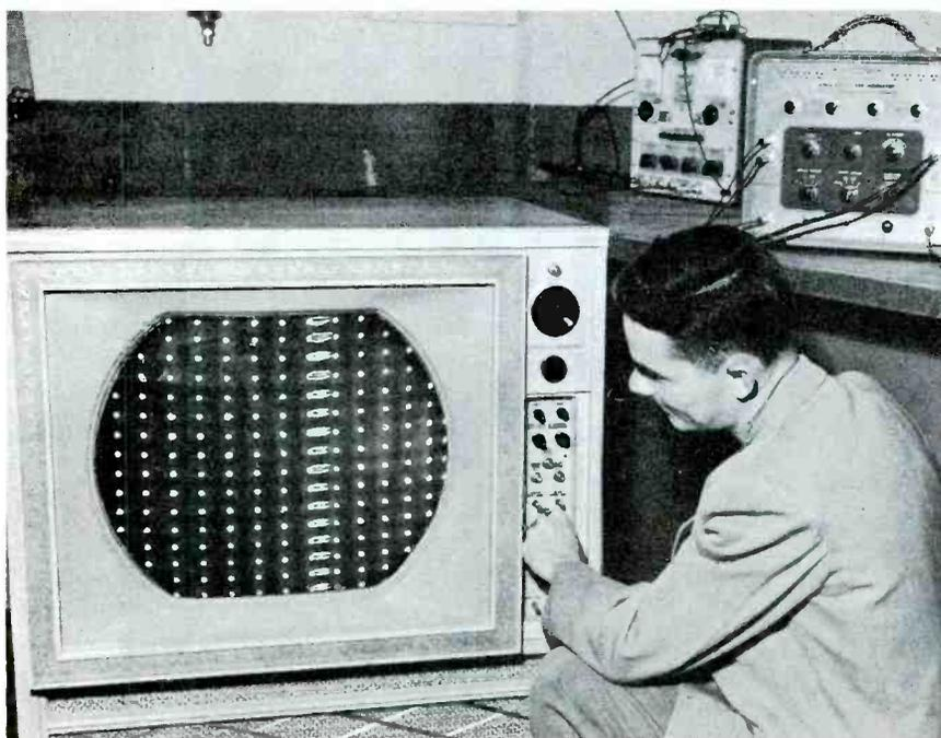
Fig. 6. Dot pattern obtained with Precision Model E-420 generator.
