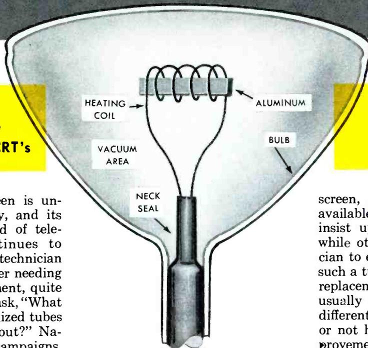
Fig. 1. Vaporizing process used to aluminize TV picture tubes.
