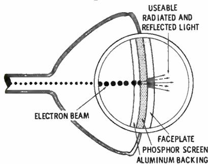
Fig. 3. Aluminized screen reflects light toward TV viewer.
