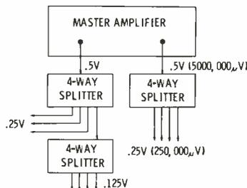
Fig. 2. Four-way splitters connected to provide the necessary number of riser signals. (Actually, 11 outlets are available, but only 10 would be used in our sample installation.)
