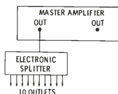
Fig. 3. Splitting arrangement which incorporates a single 10-way splitter.
