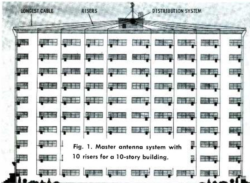
Fig. 1. Master antenna system with 10 risers for a 10-story building.
