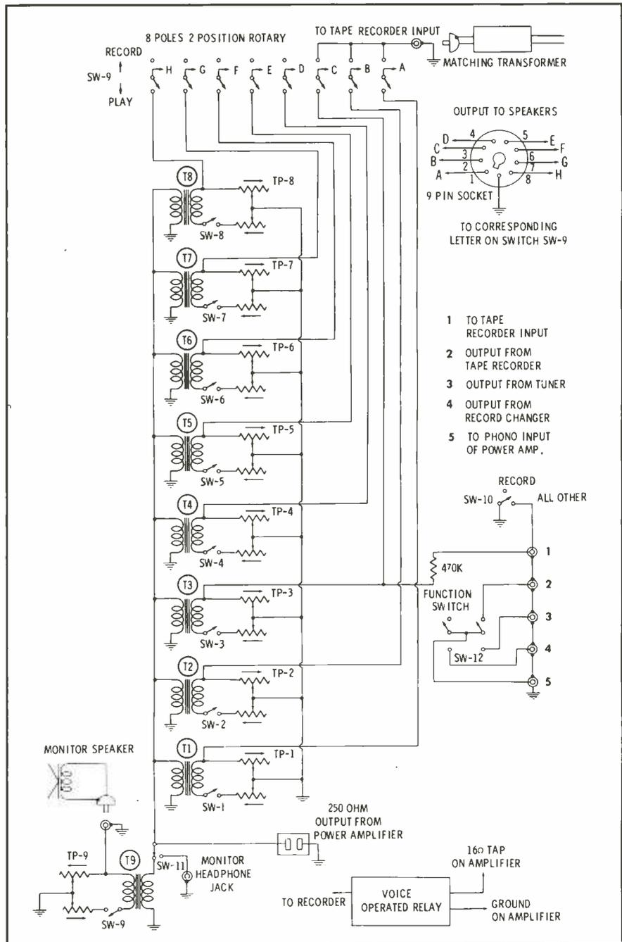
Fig. 2. Schematic diagram of control panel.
