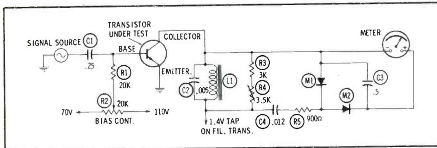
Fig. 1. Simplified schematic of the transistor test circuit in the Triplett Model 3423.
