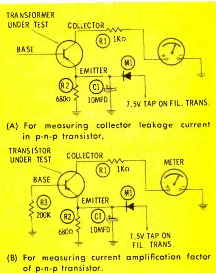
Fig. 2. Simplified transistor-test connections in EICO Model 666 tester.
