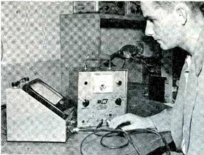
Fig. 3. Checking accuracy of a VTVM by using B & K Model 750 calibrator as a standard voltage source.
