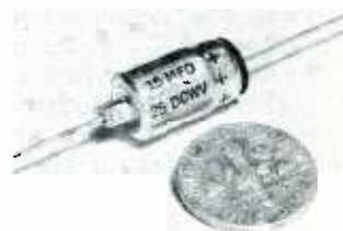
Miniaturized capacitors of the hermetically sealed aluminum-can electrolytic type are being made by Aerovox Corp., New Bedford, Mass. These units, designated Type XPP, are only 3/16" to 3/8" in diameter and 1/2" to 3/4" in
