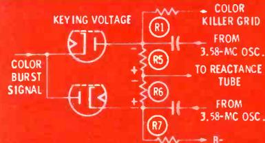
Fig. 4. Typical color phase detector.
