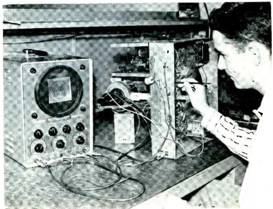
Fig. 8. "Pic-Probe" and scope together substitute for picture tube.
