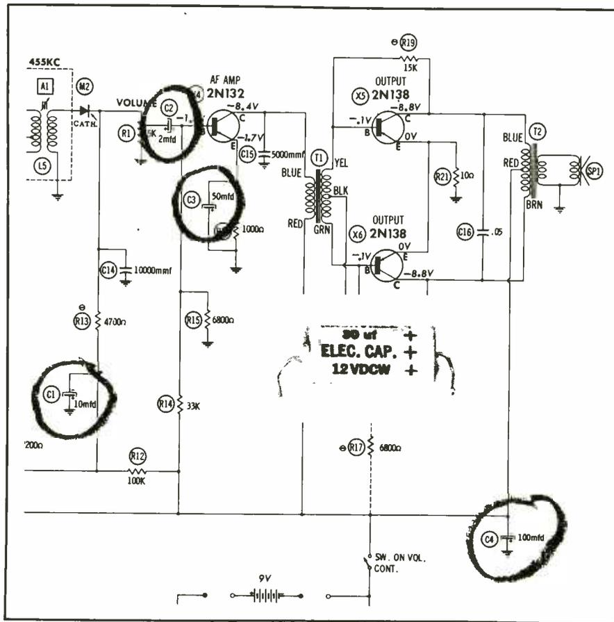
**Fig. 7. Low-voltage electrolytics are found in all transistor portables.**
