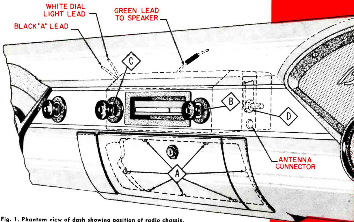
Fig. 1. Phantom view of dash showing position of radio chassis.
