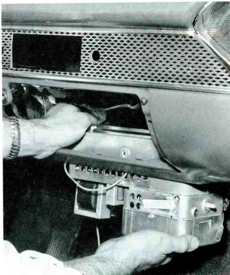
Fig. 2. Removing chassis.
