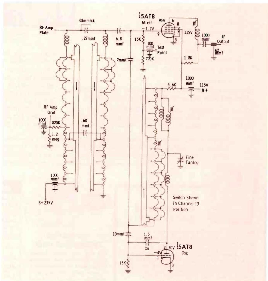
Fig. 1. Mixer and oscillator section of switch-type tuner.
