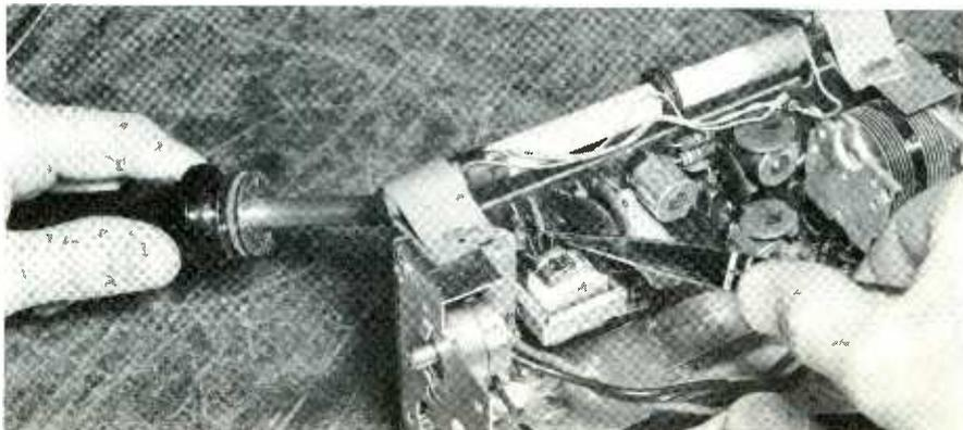
Fig. 8. Use of a heat sink is very important when soldering transistor leads.
