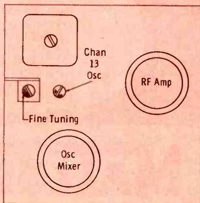
Fig. 3. Channel 13 oscillator adjustment on top of tuner.
