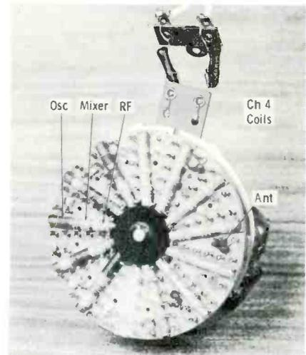
Fig. 2. Bottom view of new tuner showing tuner coils mounted on wheel.
