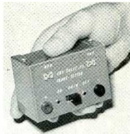
Fig. 5. Eby's new Trans-Tester converts milliammeter to transistor checker.
