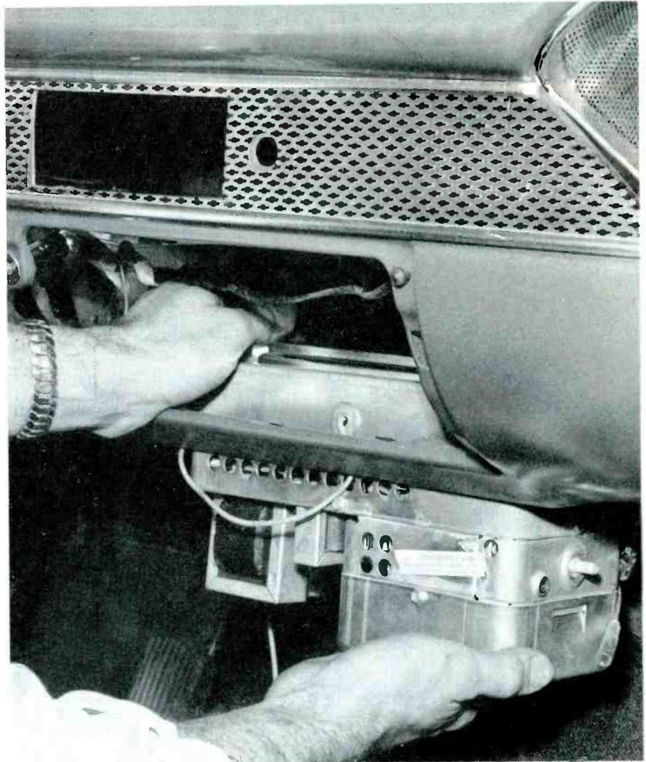
Fig. 2. Removing chassis.
