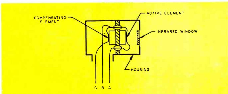
Fig. 4. Internal makeup of a bolometer.
