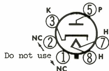
operate at a high potential above ground (in some cases, thousands of volts), extreme arcing may occur within the tube and overload the circuit to the extent that the horizontal output tube can be ruined in a very short time. Some 6W4GT tubes are supplied with pin 1 on the base. When installing such a tube, cut the extra pin off with side cutters rather than risk a recall.
