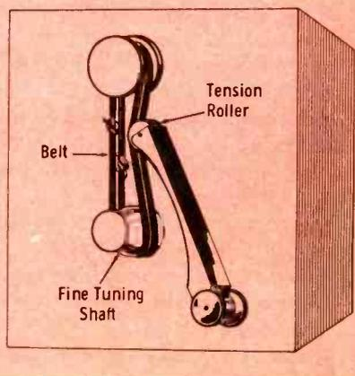
Fig. 4. Belt drive for fine tuning replaced with "treated" shoe strings.
