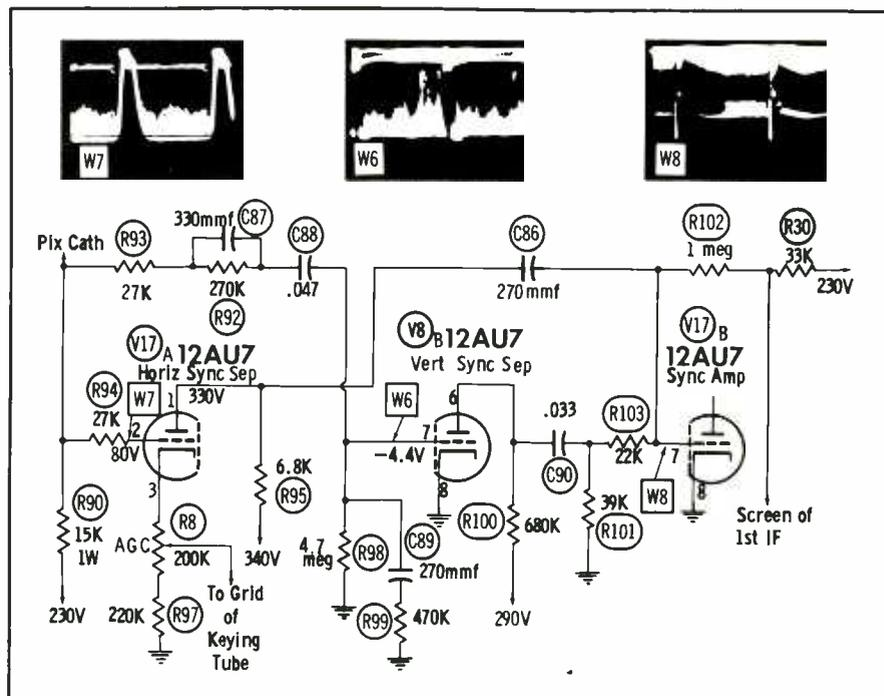
Fig. 5. Separate horizontal and vertical sync separators—ATR Model 26001.
