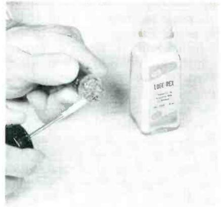
Fig. 4. Putting a thin film of conductive lubricant on tube pins.
