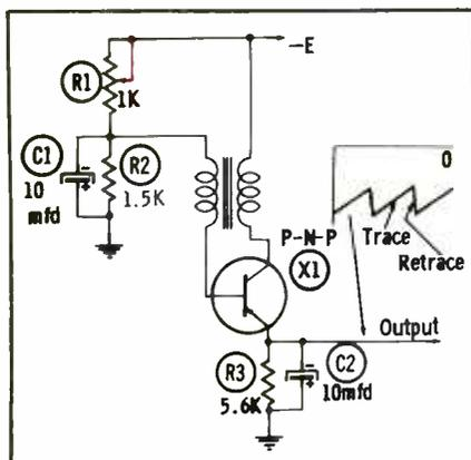
Fig. 5. Development of the sawtooth wave in this circuit differs from Fig. 4.
