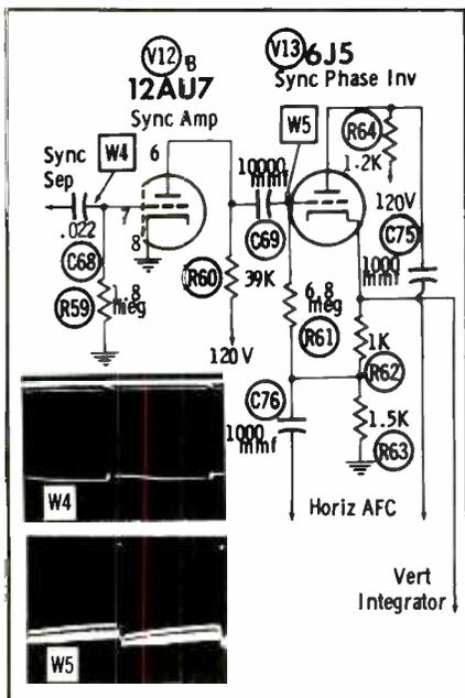
Fig. 3. Intermediate sync amplifier with grid input—Fada Model H274T.
