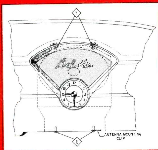
Fig. 3. Phantom view showing position of speaker unit.
