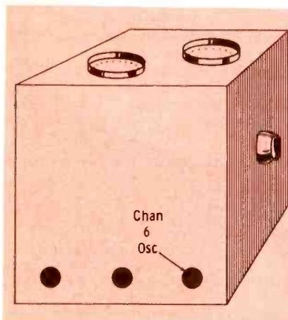
Fig. 2. Left side of RCA Tuner showing location of channel 6 adjustment.
