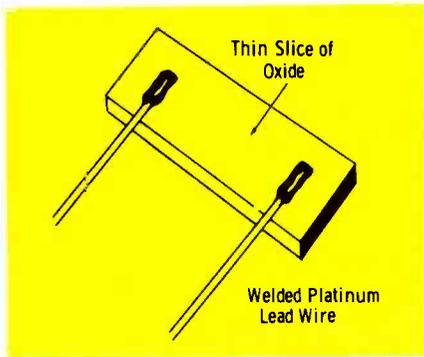
Fig. 3. Simple sketch of a thermistor.
