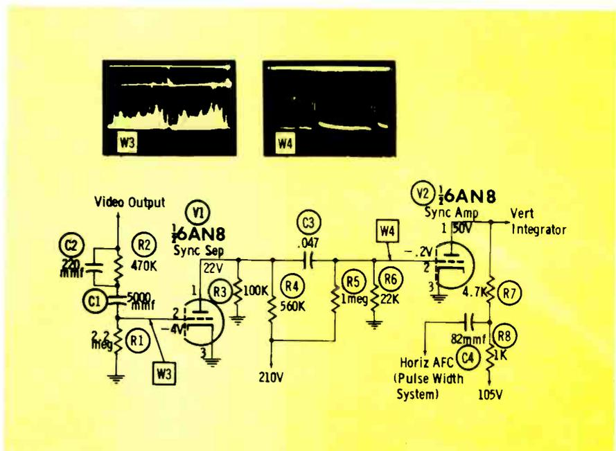
Fig. 1. Typical dual-triode sync section—Truetone Model 2D2423A.
