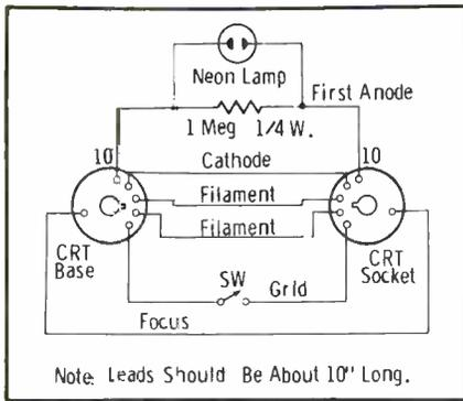
Fig. 2. CRT emission indicator which utilizes a neon lamp shunted by a 1-meg resistor in the first-anode lead.
