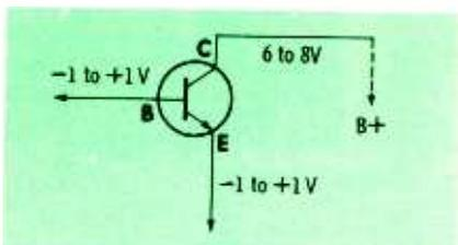
Fig. 6. Typical voltages for audio circuits employing n-p-n type transistors.
