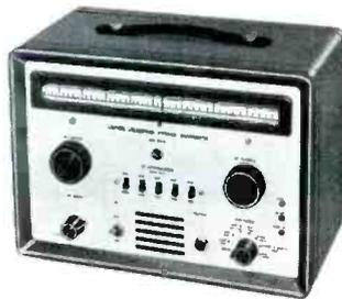
A new crystal-calibrated marker generator, WR-99A, is being produced by RCA Components Division, Camden, N.J. This instrument covers a frequency range of 19 to 260 mc in eight bands, with crystal calibration points at 1-mc intervals.
