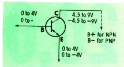
Fig. 4. Typical DC voltages for converter, IF, and some audio circuits.
