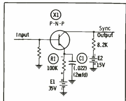
Fig. 2. A single-stage sync separator.
