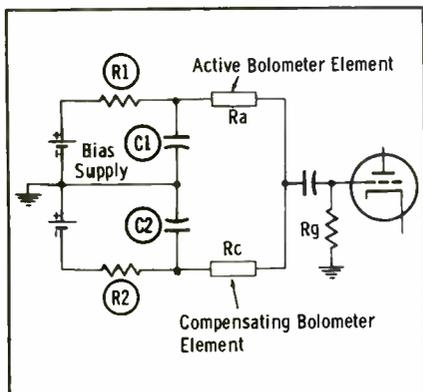
Fig. 5. Typical bolometer bridge circuit.
