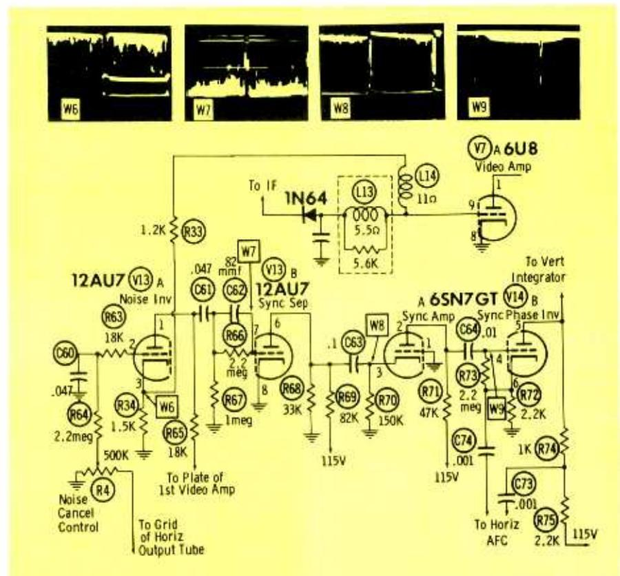
Fig. 2. Sync section plus triode noise inverter—Stromberg-Carlson Model 621.
