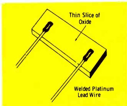
Fig. 3. Simple sketch of a thermistor.
