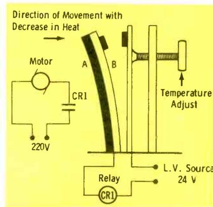
Fig. 2. The contacts of a bi-metal thermostat will open and close over a pre-determined temperature range of 2° to 3°F.
