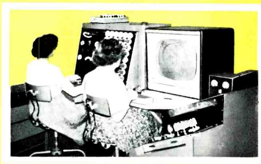
New heater-cathode design helps Sylvania damper types pass this dynamic arc test with flying colors. Dynamic tests such as this have now been instituted by Sylvania on all important types in every
