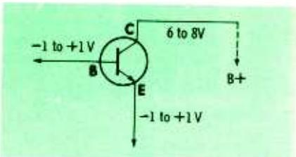
Fig. 6. Typical voltages for audio circuits employing n-p-n type transistors.
