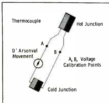
Fig. 6. Structure of a thermocouple.
