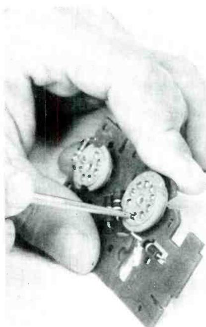
Fig. 3. Using a soldering aid to tighten tube socket contacts.
