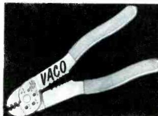
The "Crimcut" combination tool designed by Vaco Products Co., 317 E. Ontario St., Chicago, Ill., features jaws for crimping wire, five holes for shearing common sizes of bolts and screws, wire-cutting edges  $\frac{1}{2}$ " long, and a row of six slots for stripping insulation off various sizes of wire from #10 to #22. The tool is 8" long and is chrome-plated with plastic-covered handles.
