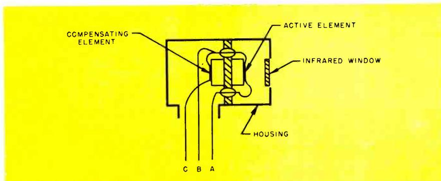
Fig. 4. Internal makeup of a bolometer.
