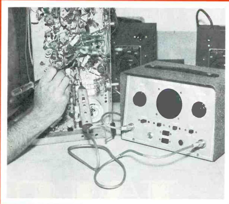
Fig. 1. New Win-Tronix Analyzer aids in quickly isolating intermittents.
