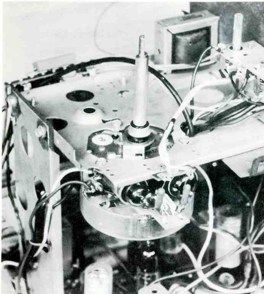
Fig. 1. New compact version of Standard Coil tuner in Airline Model GTM4031A.
