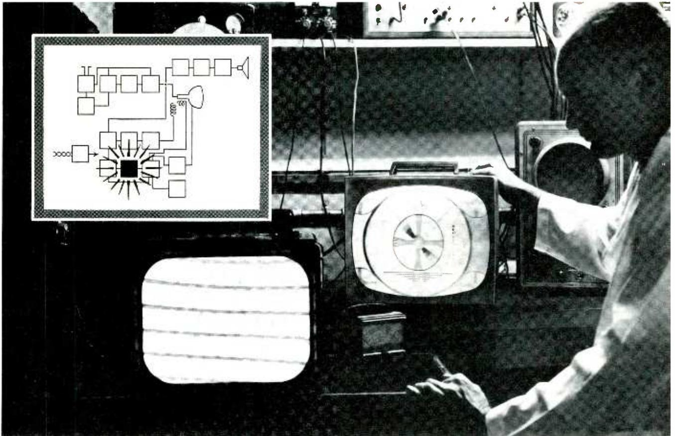
Here General Electric Application Engineer C. L. Taylor shows what can happen when an old-style horizontal-oscillator tube is used in two different TV sets. Image at left is completely
