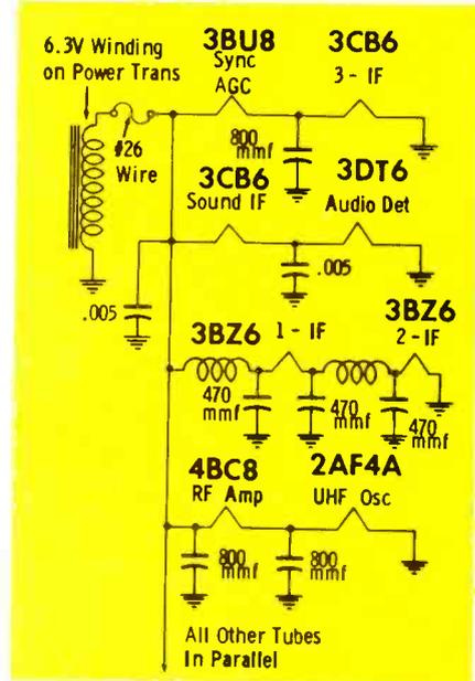
Fig. 6. Series-parallel hookup across 6.3-volt filament supply in Motorola TS-544.
