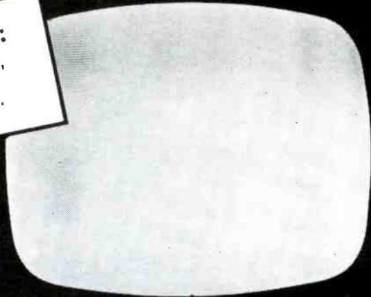
Let's take a look at this problem: A condition such as this can exist only when there is no signal reaching the picture tube or the audio output stage. Using the Tuner Service data (found in every PHOTOFACT TV Folder), first isolate the trouble by connecting an amplitude-modulated signal to the mixer-grid test point "D." The appearance of one or more black bars on the face of the tube would indicate that the trouble is probably in the tuner. So look for the following possible causes:
