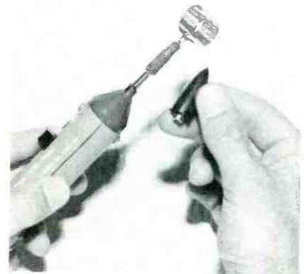
Fig. 2. Attachments for Win-Tronix intermittent probe permit signal sampling without direct circuit contact.
