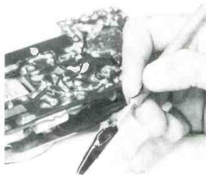
Fig. 2. A needle-point probe is ideal for transistor-radio testing.
