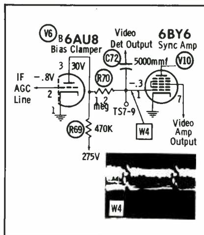
Fig. 6. Bias clamber for pentagrid separator—General Electric "ST" Line chassis.
