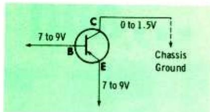
Fig. 5. Operating voltages for a conventional p-n-p audio stage.
