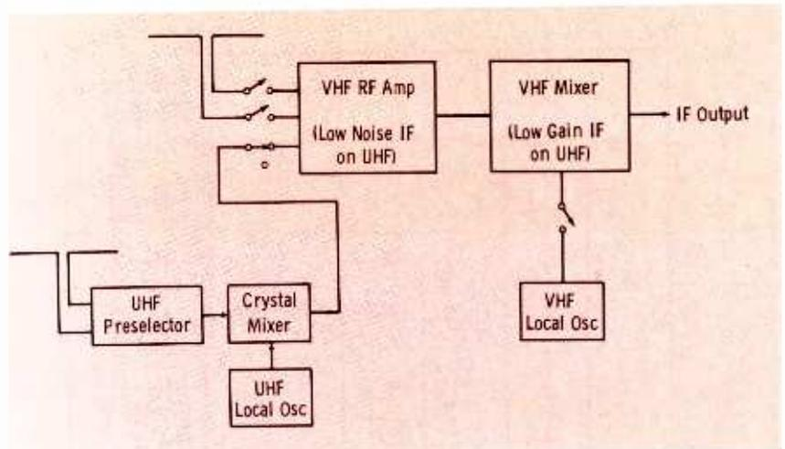
Fig. 2. Block diagram of UHF-VHF tuner.
