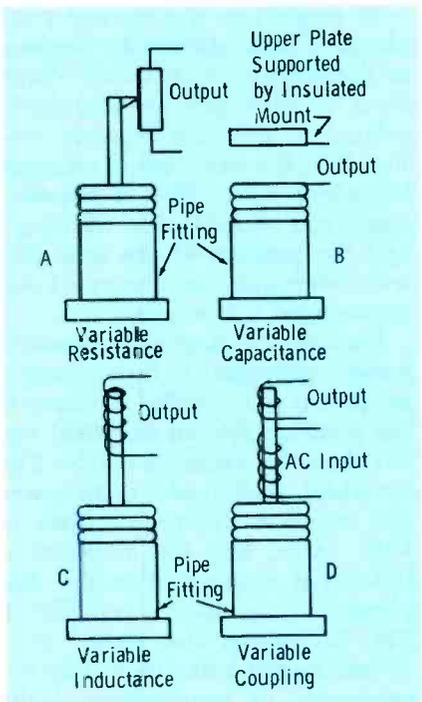
Fig. 3. Linear movement of diaphragm makes conversion more accurate.
