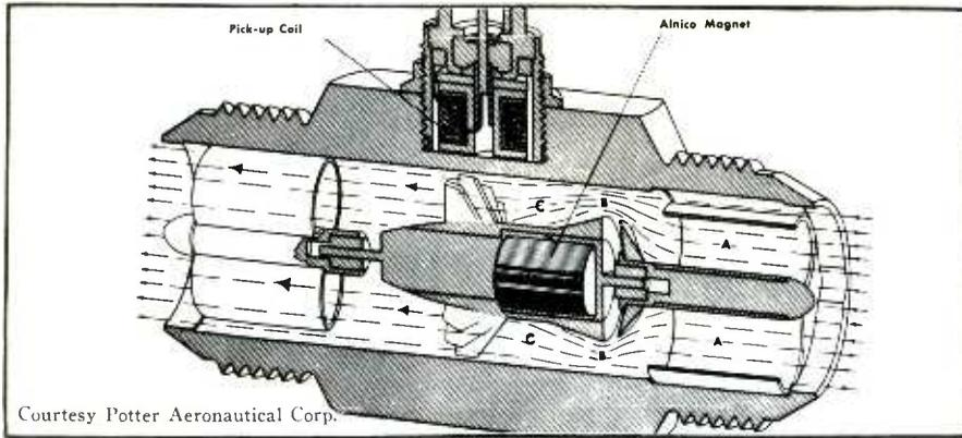
Fig. 10. Rotation of turbine causes the magnetic field to cut the pickup coil, generating an output pulse which varies with velocity.
