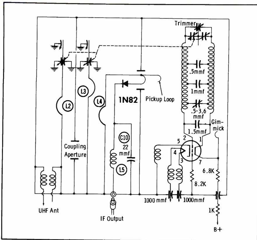
Fig. 4. Schematic of UHF tuner with two stage preselector.
