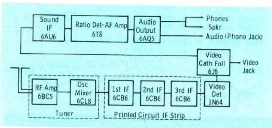
Fig. 2. Block diagram of the circuits used in "Duo-Master" chassis.
