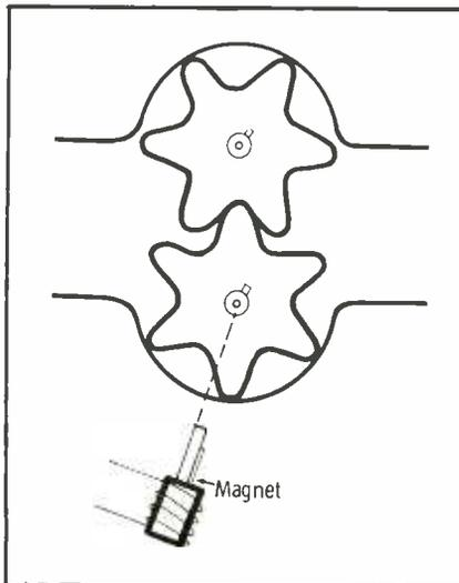
Fig. 8. Positive displacement meter offers direct quantity measurement.
