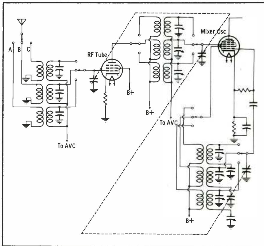
Fig. 5. Input circuits for three-band, triple-tuned superheterodyne.
