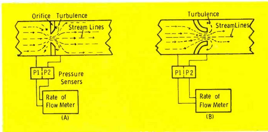
Fig. 6. Pressure difference from P1 to P2 is proportional to velocity.
