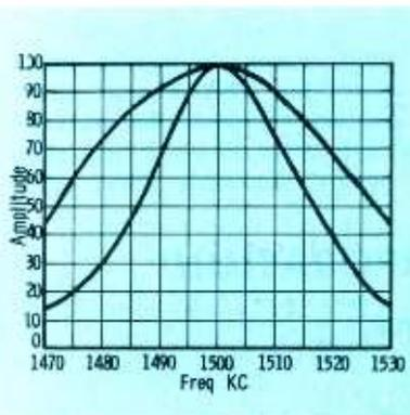
Fig. 9. Resonance curves for tuned circuits of different Q.
