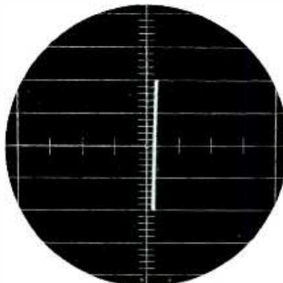
(A) Calibration wave with sweep-width reduced to zero.
