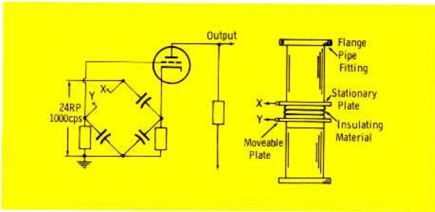
Fig. 5. Deformation of pipe causes capacitor plate separation to vary.
