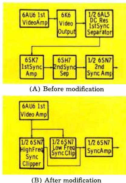
Fig. 1. Block diagram of the sync section of a 630-type chassis.
