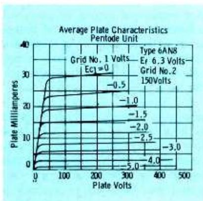
Fig. 5. Characteristic curves of the pentode section of a 6AN8 tube.
