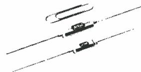
Two new types of subminiaturized electrolytic capacitors for transistor circuits and similar applications have been announced by Astron Corp., East Newark, N. J. Type EE has an epoxy end fill, and Type EM features a "spun" end with rubber bushing. The new units come in physical sizes ranging from 3/16" × 1/2" to 1/4" × 3/4" and in voltage ratings of 1, 3, 6, 8, 16, 26 and 50 volts.
