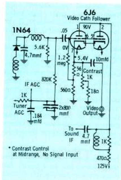
Fig. 3. Details of video cathode follower circuit.
