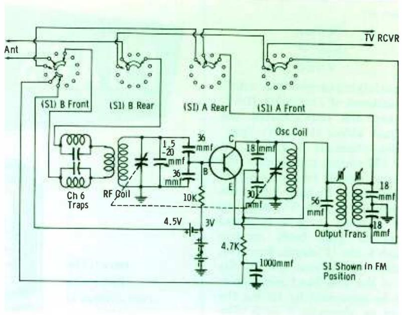
Fig. 6. "TeleVerter" contains SB transistor functioning as mixer-oscillator.
