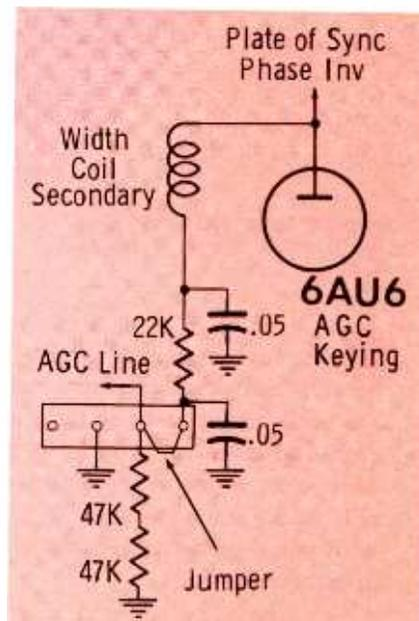
The width coil also supplies a pulse to the plate of a special type of sync phase inverter stage that controls the horizontal oscillator; therefore, any interference with the width-coil circuit would tend to affect horizontal sync. The keying pulses to this circuit would not be entirely disabled, since they would find a return path to ground through the .05-mfd capacitors.
