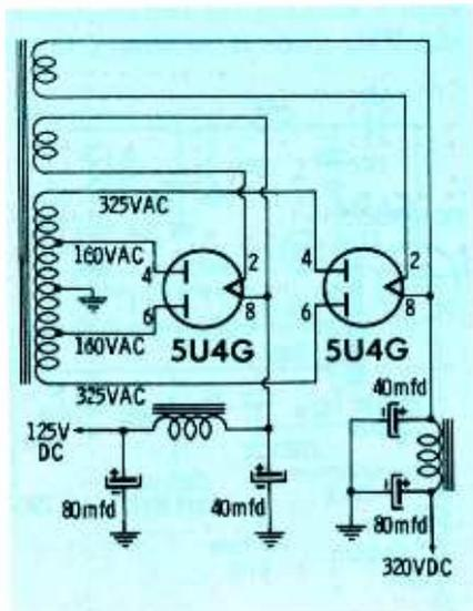
Fig. 3. Power supply circuit with separate high and low voltage rectifiers.
