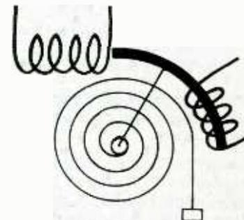
(D) Change of coupling between coils.
