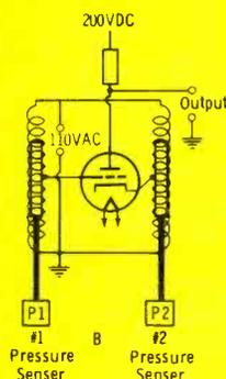
Fig. 12. Differential transformer used in pressure indicating applications.
