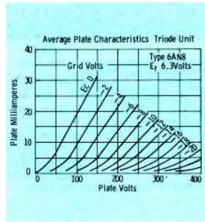
Fig. 6. Characteristic curves of the triode section of a 6AN8 tube.
