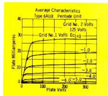
Fig. 3. Characteristic curves of the pentode section of a 6AU8 tube.
