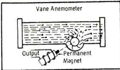
Fig. 9. With anemometer, velocity is measured without being affected by static pressure applied to system.
