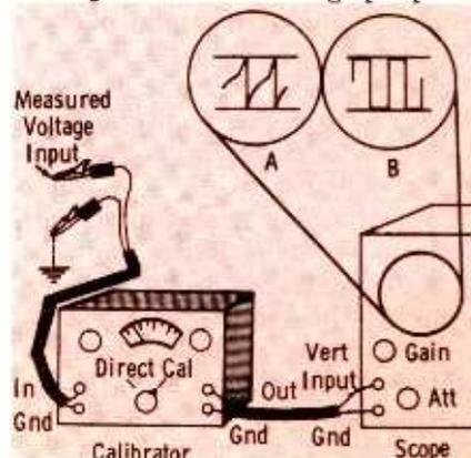
Fig. 1. Oscilloscope-Calibrator arrangement for peak-to-peak measurements.
