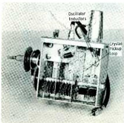
Fig. 5. Crystal injection loop.
