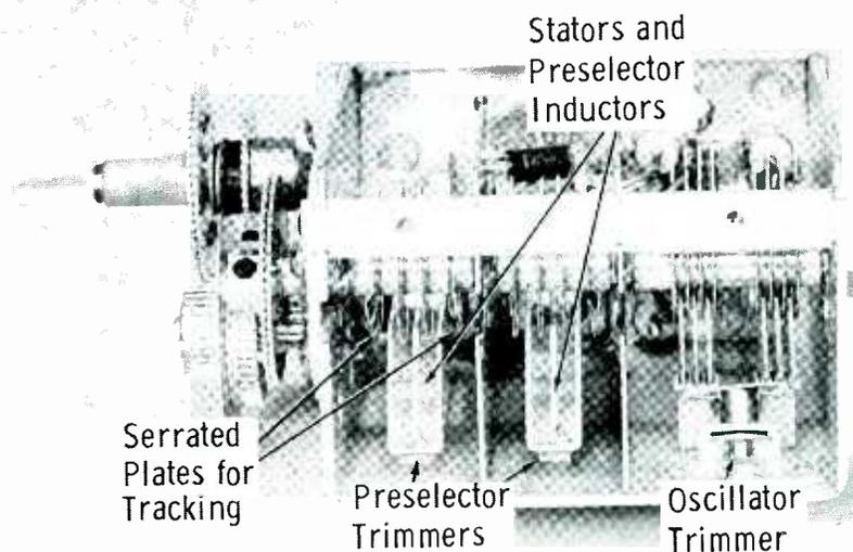
Fig. 3. UHF tuner with shields removed exposing preselector tuning assembly.
