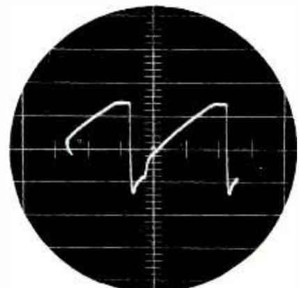
(B) Waveform of horizontal drive voltage.
