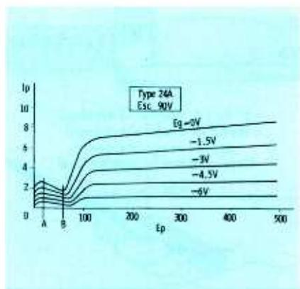
Fig. 7. In tetrode tubes, region A-B represents a negative resistance.
