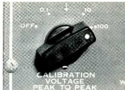
Fig. 5. This scope permits the use of 4 different calibrating voltages.
