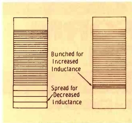
Fig. 6. Principle of coil pruning.
