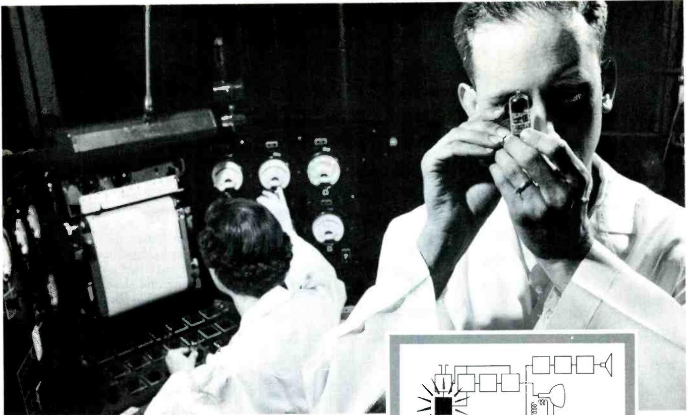
**G-E DESIGN ENGINEER** M. W. LeClear examines the structure of a 6U8 through a magnifier. Characteristics of the tube have been plotted by the two-axis recorder in background. Outstanding quality of G-E oscillator-mixer tubes—consequently, their popularity as replacements—comes from a balanced application of advanced design principles, precision manufacture, and careful testing.
