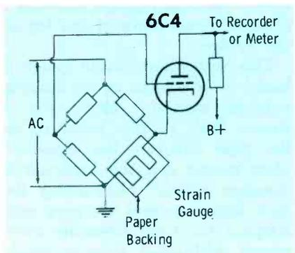
Fig. 4. The strain gauge senses pressure from deformation of pipe.
