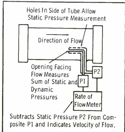
Fig. 11. The Pitot tube measures exact energy due to velocity by compensating for static pressure.
