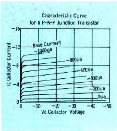
Fig. 4. Characteristic curves for a p-n-p junction transistor.
