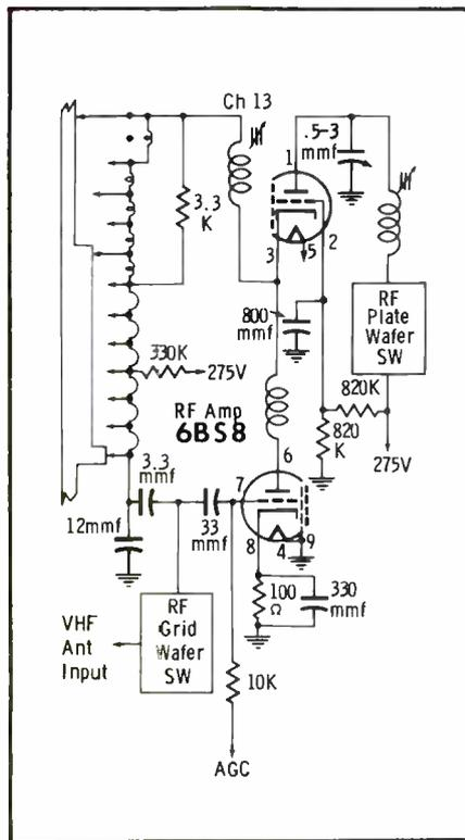
Fig. 7. New GE tuner has variable inductance between halves of RF stage.
