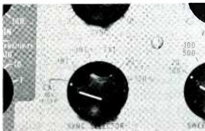
Fig. 4. Sync selector includes CAL. position for internal calibrating voltage.
