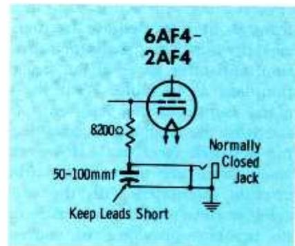
Fig. 6. Modification used in the measurement of oscillator grid current.
