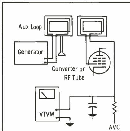
Fig. 3. VTVM monitors AVC and serves as output indicator during alignment.
