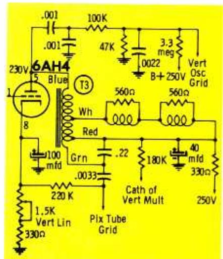
Fig. 4. Zenith vertical output circuit.
