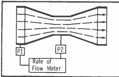
Fig. 7. Pressure loss is kept at a minimum in the venturi nozzle.
