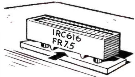
**HANDY TO USE**—Sturdy terminal pins. Simply plug fuse resistor into receptacle. Projections on bottom of case leave air space so receptacle won't overheat.
