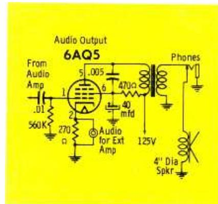
Fig. 4. Plate circuit of audio output tube in "Duo-Master" drives either speaker or phones; cathode circuit furnishes signal for external amplifier.
