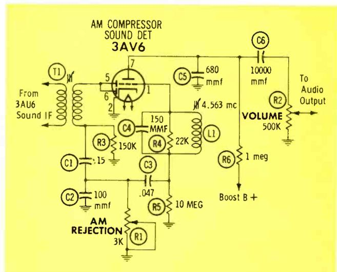
Fig. 2. "Delta" sound detector circuit of latest GE 14" portable TV sets works on the slope-detection principle.
