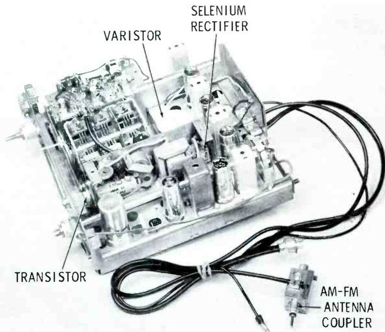
Fig. 4. The Model 88BH FM tuner is an accessory for the 1958 Lincoln.
