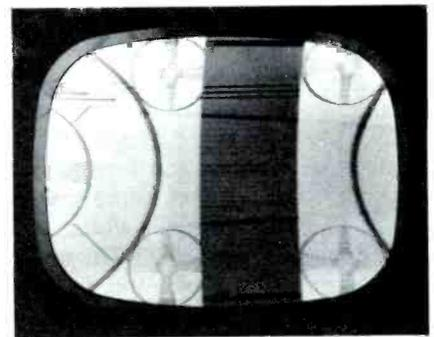
Fig. 3. This out-of-phase condition is due to improper horizontal AFC control.
