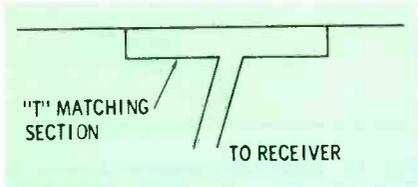
Fig. 17. T-matching section formed between the transmission line and dipole.
