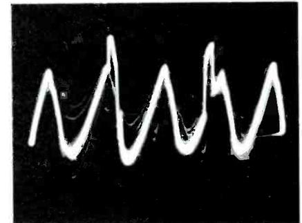
(B) AFC grid waveform.
