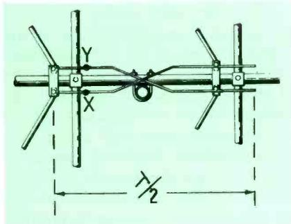
Fig. 18. Two-conductor coupling between T-matched sections. Lead-in goes to X-Y.
