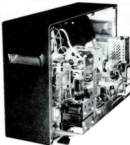
Fig. 1. In new General Electric "Designer" series, most of chassis is exposed when curved back cover is removed.
