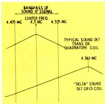
Fig. 3. Frequency response curves of tuned circuits used in sound detectors.
