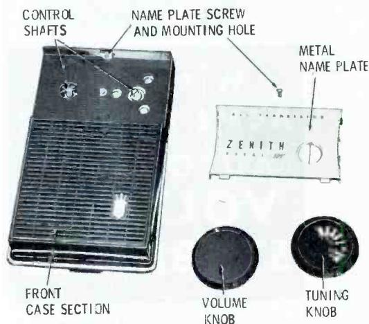
Fig. 5. To remove the chassis of the Royal "300," disassemble the name plate and control knobs.
