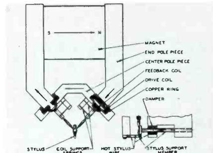
Fig. 2. Basic recording head showing coil placement and attachment to stylus.
