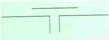
Fig. 9. Parasitic element is placed close to driven element in Finney arrays.
