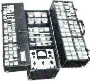
A caddy with built-in tube tester is being marketed by Vis-U-All Products Co., Grand Rapids, Mich. The tester provides checks for quality, grid-cathode or heater-cathode shorts, interelectrode leakage, grid emission, and gas. Sensitivity of the leakage test can be regulated to suit the owner. An adapter is furnished for checking picture tubes. An adapter is also available for checking selenium rectifiers. Dealer net price of the Model V100 Caddy Tube Tester is \$99.50.
