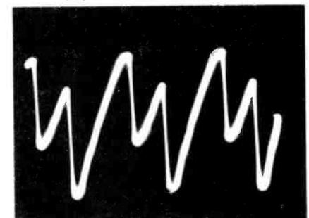
(B) Oscillator plate waveform.
