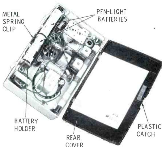
Fig. 2. In the Philco Model T-4, the case can be opened by prying out on clip and separating the two individual sections.
