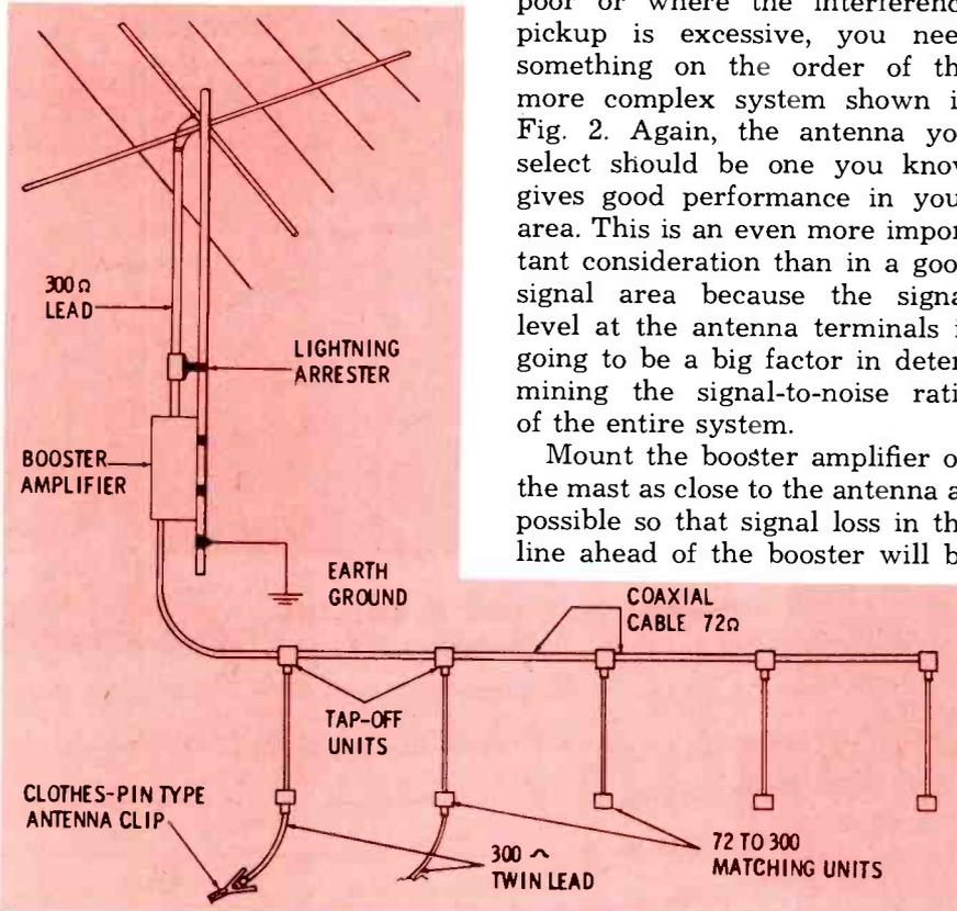
Fig. 2. Shop antenna system for weak signal areas where noise level is high.
