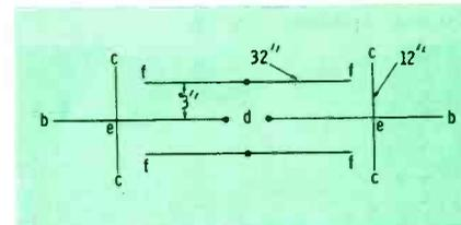
Fig. 3. Geometric characteristics of, and spacing between, "Satellite" elements.
