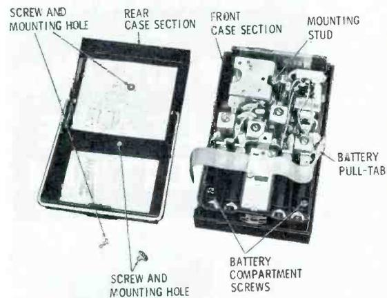
Fig. 4. Zenith portable incorporates a pull-out tape for quick removal of the battery cells.
