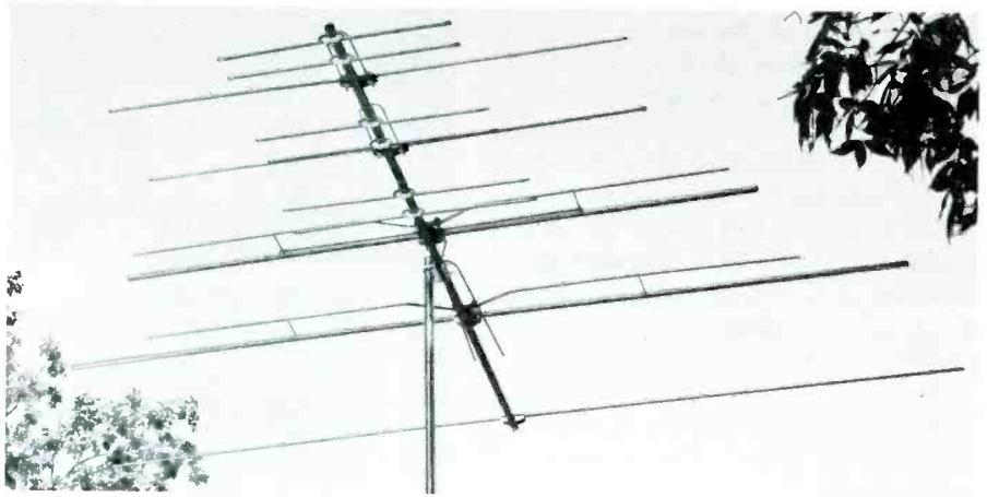
Fig. 14. Basis of Winegard "Color 'Ceptor" is T-matching sections toward rear.
