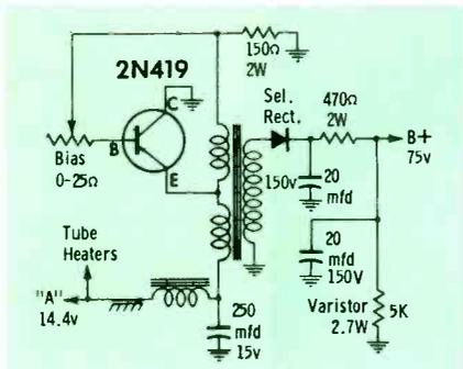
Fig. 5. Power supply of FM tuner uses 2N419 transistor as 400-cps oscillator.
