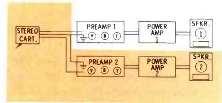
Fig. 5. Block diagram of changes necessary to convert monaural system to stereo.
