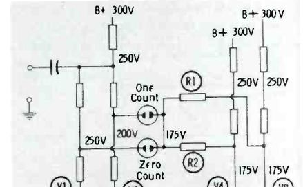
Fig. 6. Method of connecting lamps so they light for only one set of conditions.
