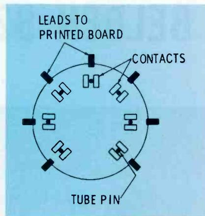
Fig. 5. Details of printed-board type tube socket that caused noisy operation.
