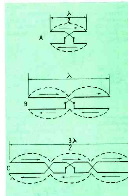
Fig. 4. Steps used in developing broad-band response for Trio's wing dipole.
