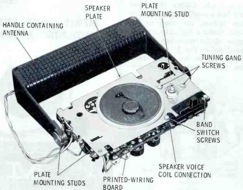
Fig. 10. To give yourself enough room to work on the Motorola Model 6X39A-2, the large speaker-mounting plate should be separated from the main chassis.
