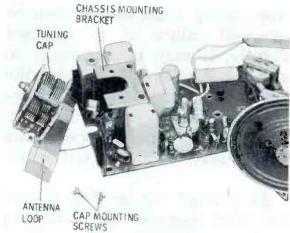
Fig. 9. Servicing Emerson Model 888 may require removal of tuning capacitor.
