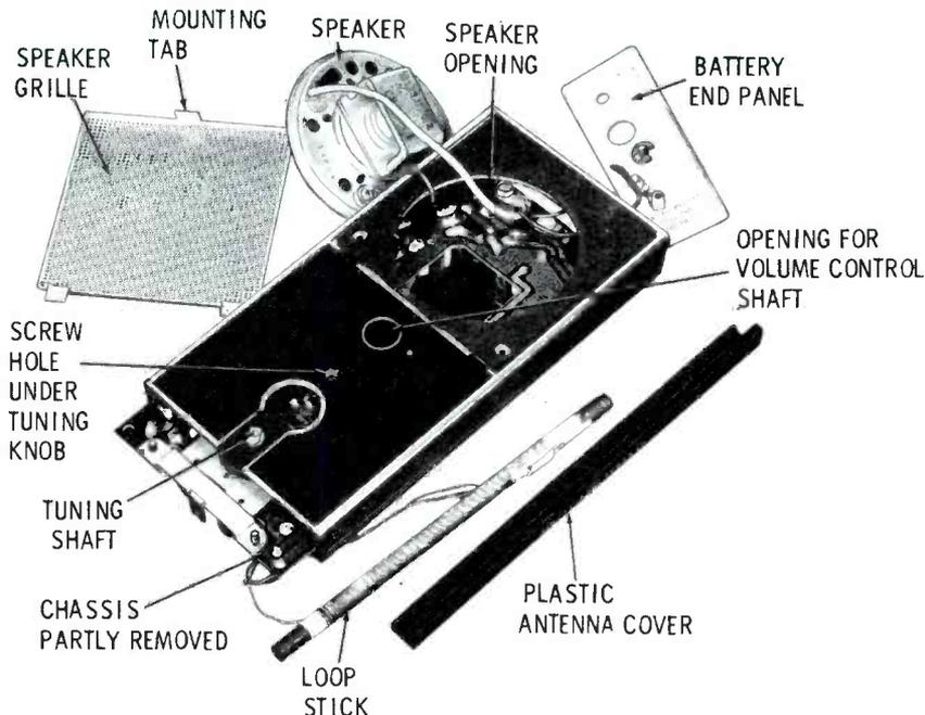
Fig. 7. In this G.E. model, the chassis board slides out one end of the metal case. Be sure to use caution when handling its delicate loop stick and speaker leads.
