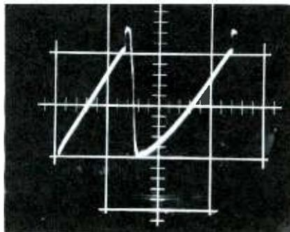
Fig. 13. Normal waveform at horizontal AFC grid after open C84 is replaced.
