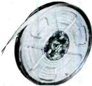
You can clean iron oxide and dust off the heads and capstan of a tape recorder without disassembling the machine, if you use a Walsco "Kleen-Tape." This service aid is a fabric tape which has been impregnated with a solvent and then wound on a standard 5" reel so that it can be played through the machine in the same way as an ordinary recording.
