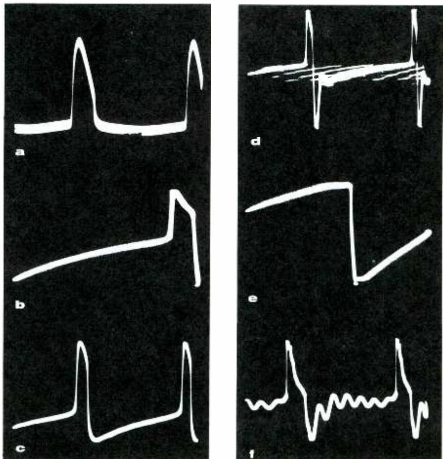
Fig. 4. Waveforms at key points in multivibrator circuit with trouble present.
