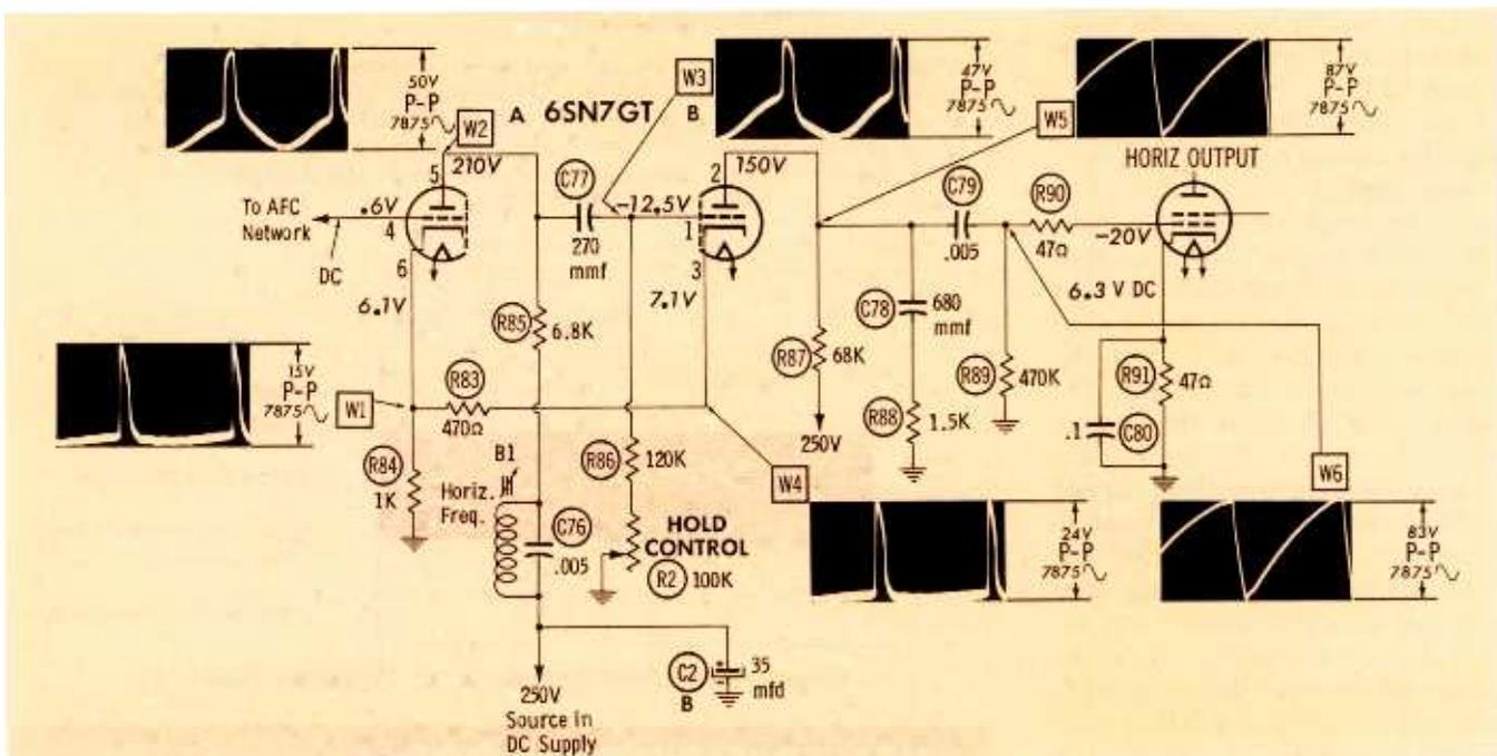
Fig. 1. Schematic of typical horizontal multivibrator circuit and key waveforms.
