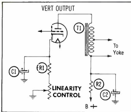
Fig. 7. Diagram of vertical output stage showing probable use of electrolytics.
