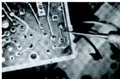
Fig. 5. Easiest way to repair open spot is to bridge break with piece of wire.
