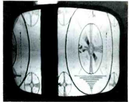
Fig. 5. Split picture is caused when oscillator frequency is reduced by half.
