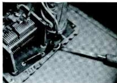
Fig. 4. Conductor sometimes will fuse or rupture as result of current overload.
