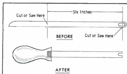
Fig. 5. Old hacksaw blade becomes useful tool for removing "C" clips.
