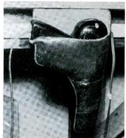
Fig. 6. Holster holds soldering gun and protects case against breakage.
