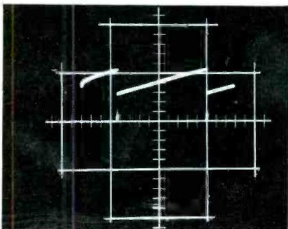
Fig. 15. Waveform at vertical output grid normally has 118V p-p amplitude.
