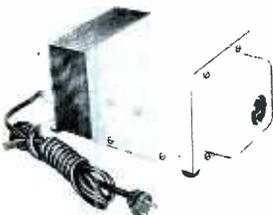
Fluctuations in line voltage within the range from 95 to 130 VAC are corrected by the Acme Electric automatic voltage stabilizer, which furnishes constant 118-volt output to any TV or hi-fi set rated at up to 200 volt-amperes. A relay automatically disconnects the primary circuit of the stabilizer when the load is removed.
