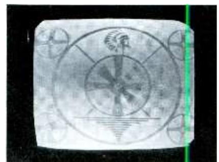
Fig. 3. Leaky B+ filter causes loss of brightness and decrease in raster size.
