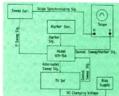
Fig. 2. In setup for IF alignment, the adder receives and delivers all signals.
