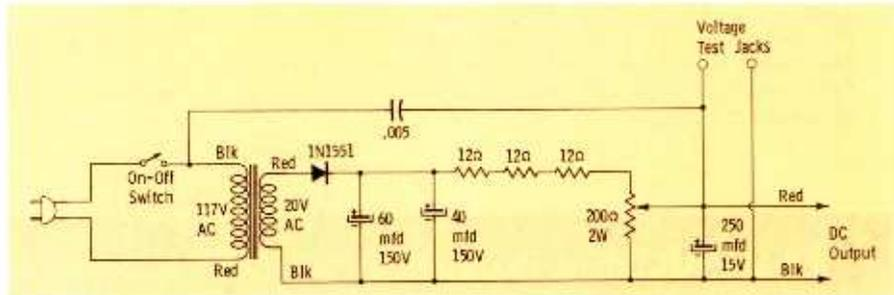
Fig. 5. Schematic of Seco Model PS-2 featuring silicon diode for rectification.
