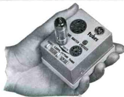
**NEW TUBE-FUSE-LAMP CHECKER (ETR-981A).** Only  $3\frac{1}{2}$ " by  $2\frac{3}{4}$ " by  $1\frac{7}{8}$ ". Can easily be carried in pocket. Powered by 3 "C" flashlight batteries. Will check 7- and 9-pin miniature tubes, also lock-in and octal-base types . . . picture-tube heaters . . . all TV and radio fuses . . . all filament-type pilot lamps. A "must" for technicians.
