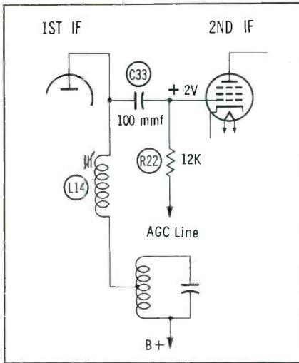
Fig. 10. Grid voltage of second IF stage was +2 volts because of leaky C33.
