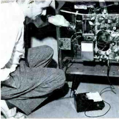
Fig. 9. With an accessory probe, Model 630-PL can be adapted to read KV.
