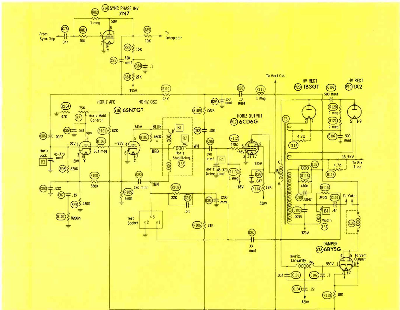
Fig. 5. Schematic of horizontal, high-voltage, sweep, and sync inverter stages.
