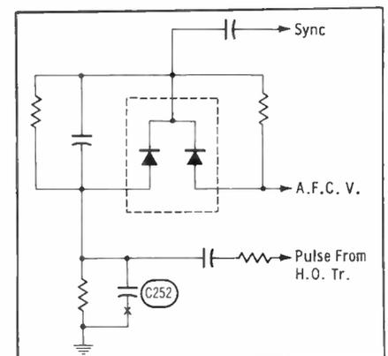
Fig. 3. Bad solder joint at ground end of C252 resulted in double picture.
