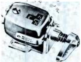
A .7-mil diamond stylus for playing stereo records is mounted on one side of the Recoton RG745-1SD turnover cartridge, and a 1-mil sapphire stylus for monaural LP's is on the other side. A companion model, the RG745-3SD, features a combination of a .7-mil and a 3-mil stylus. The cartridges are magnetic.
