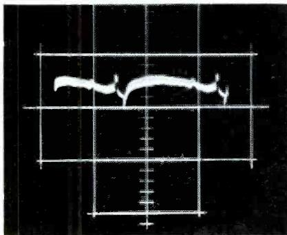
Fig. 11. Normal waveform on plate of second IF stage after replacing C33.
