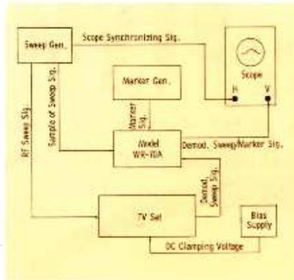
Fig. 3. Typical arrangement for RF sweep alignment with Model WR-70A.
