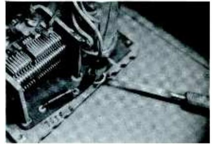
Fig. 4. Conductor sometimes will fuse or rupture as result of current overload.
