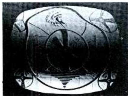
Fig. 4. 60-cps distortion resulting from open electrolytic in the power supply.
