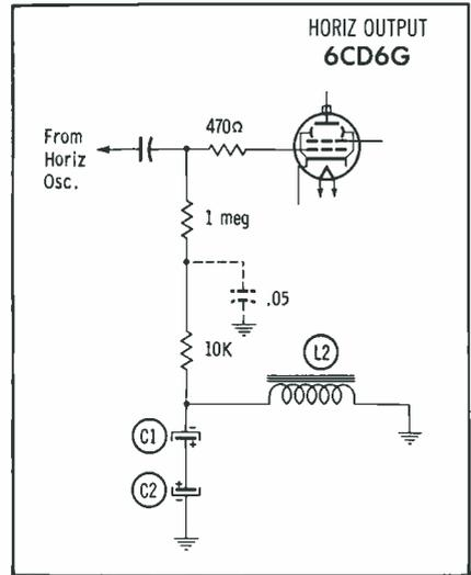
Fig. 7. Horizontal pulse energy across 10K-ohm resistor caused it to burn up.
