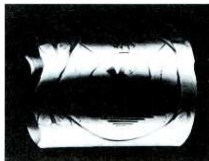
Fig. 2. Two hum bars indicate an open electrolytic in a full-wave supply.
