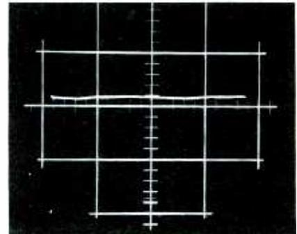
Fig. 9. Absence of a signal at plate of second IF stage indicates trouble.
