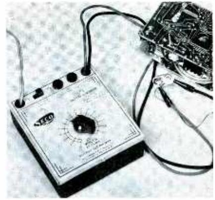
Fig. 4. Seco Battery Eliminator powers pocket-sized transistorized equipment.
