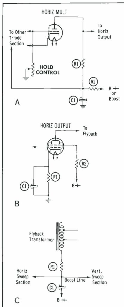
Fig. 9. Schematics showing the use of electrolytics in horizontal sweep stages.
