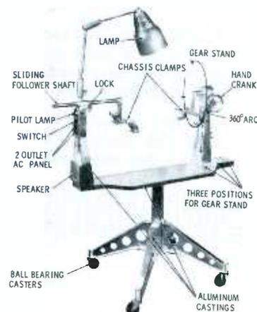
Fig. 3. *Tel-A-Turn* has built-in test speaker, trouble light and AC line cord.
