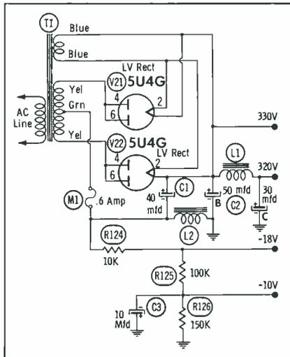
**Fig. 6. Low-voltage power supply includes two taps for negative voltages.**
