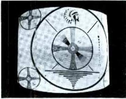
Fig. 10. Nonlinear sweep due to faulty electrolytic in horizontal output stage.
