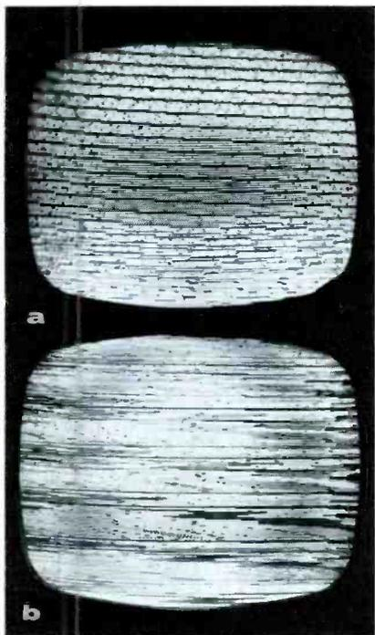
Fig. 3. Too high oscillator frequency causes this "Christmas-tree" distortion.
