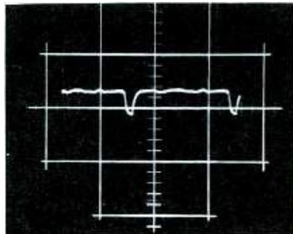
Fig. 8. Normal signal at plate of first IF viewed with demodulator probe.
