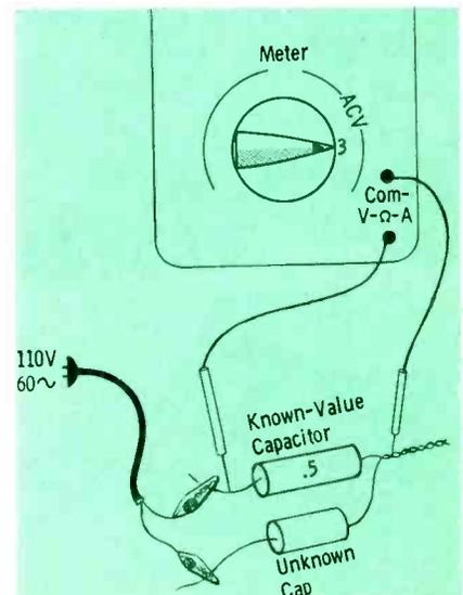
Fig. 8. Simple setup for checking capacity with Triplet Model 630-PL VOM.
