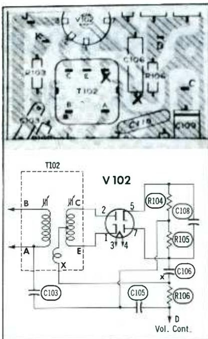
Fig. 1. Break in printed wiring conductor caused intermittent loss of audio.
