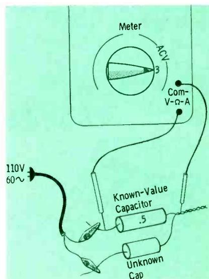
Fig. 8. Simple setup for checking capacity with Triplet Model 630-PL VOM.
