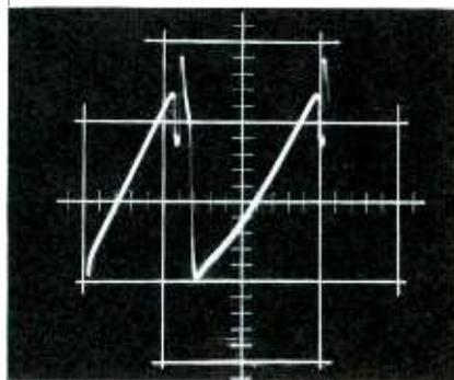
Fig. 12. Distorted waveform on grid of horizontal AFC produced by open C84.
