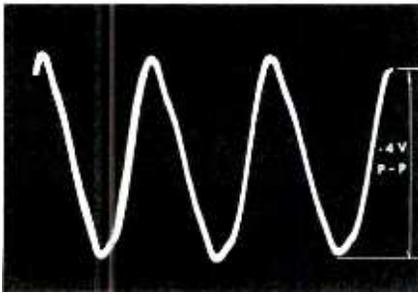
Fig. 6. Waveform of 60-cps hum voltage present in output of Model PS-2.
