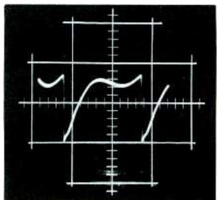
Fig. 4. Horizontal oscillator slugs are adjusted for equal peaks on waveform.
