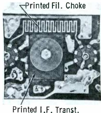
**Fig. 6. Inductors such as IF transformers may be printed directly on board.**
