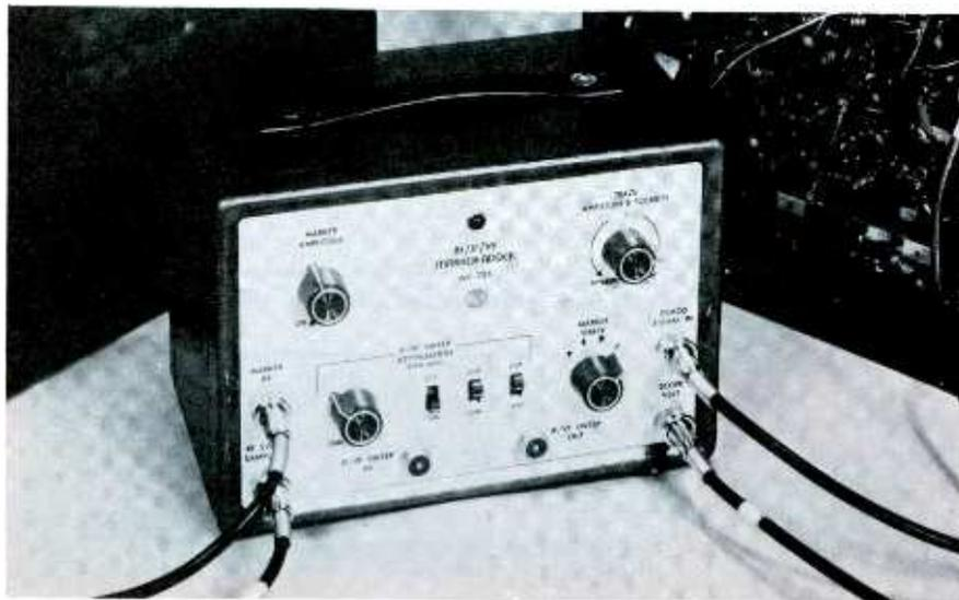
Fig. 1. RCA's Model WR-70A Marker-Adder injects markers between set and scope.
