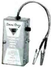
Selenium and silicon rectifiers can be tested under load with the Hallmark Model OC-1 "Omni-Chex," a battery-operated rectifier tester. This unit will also check other components such as crystal diodes and power transistors. Dimensions are 4" x 1½" x 2", and the net price is \$5.95 including batteries.
