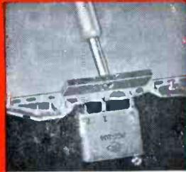
Bar Type De-Soldering Tiplet removes solder from all straight line component junctions at one time.
