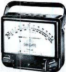
Temperatures of gases, liquids and solids can be measured within  $\pm 3^\circ$  F with the Simpson Model 389-3L "Dual Range Therm-O-Meter." The 7" meter face has two scales covering  $-50^\circ$  to  $100^\circ$  F and  $100^\circ$  to  $250^\circ$  F. Price is \$62.50, including a 15' lead with a thermistor tip for sensing. The meter has jacks for two extra leads (\$3.95 each) and a switch that allows readings to be taken individually from up to three leads.
