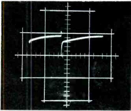
Fig. 14. Normal waveform at grid of vertical oscillator measures 105V p-p.
