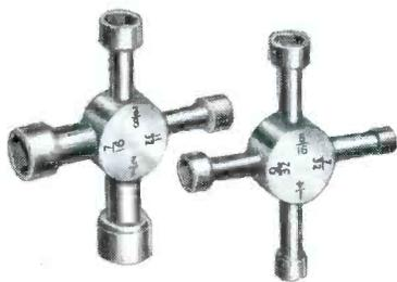
**TWIN-X WRENCH SET (ETR-752)**—designed and built expressly for TV-radio repairwork. Replaces eight hex-head socket wrenches  $\frac{3}{16}$ " to  $\frac{1}{2}$ ". Sizes are clearly marked for quick selection. Hollow shafts permit wrench to grip the nut over protruding end of bolt. Chrome-plated case-hardened steel—will stand up in long, hard service.
