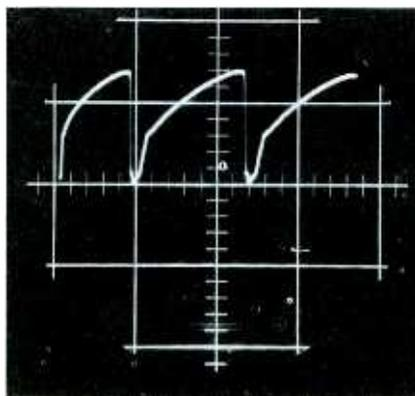
Fig. 3. Horizontal output grid driving signal is 140V p-p in normal operation.
