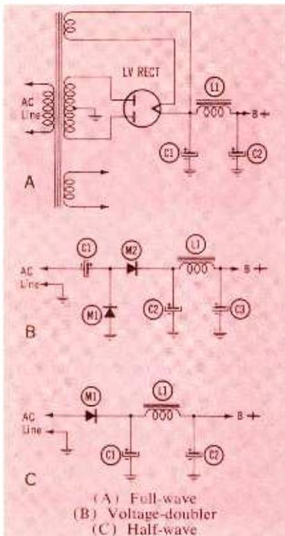
Fig. 1. Partial schematics of typical TV low-voltage power supply circuits.
