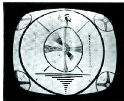
**Fig. 11. Horizontal foldover resulting from a defective boost filter capacitor.**
