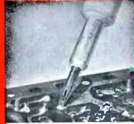
Slotted De-Soldering Tiplet straightens bent tabs and removes solder in one easy motion.
