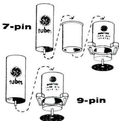
**PIN-LOCATOR FOR MINIATURE TUBES (ETR-1540).** Use it to place miniatures in hard-to-reach sockets. Centering plug positions the locator above pin holes. Magnets then hold locator while tube is turned till pins drop into socket.
