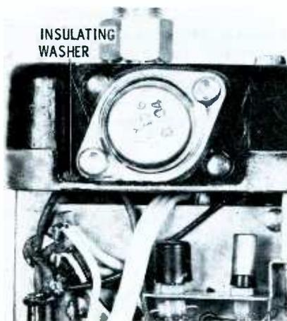
Fig. 1. Insulating washer is coated with silicone compound to aid heat transfer.
