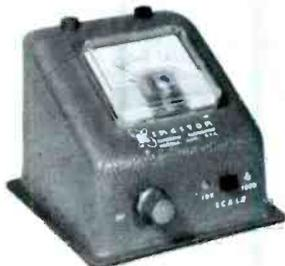
A continuously variable DC voltage from 0 to 67.5 volts, useful in receiver alignment or AGC troubleshooting, is provided by the battery-operated Kingston Model BB-1 "Variable DC Source." A built-in meter indicates output in two ranges (0-10 and 0-100V) with 5% accuracy. The battery employed is a standard radio "B" type. Net price is \$14.95, less battery.
