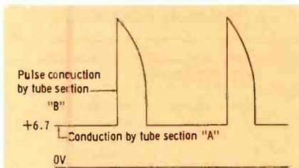
Fig. 2. Analysis of cathode waveform showing conduction of tube sections.
