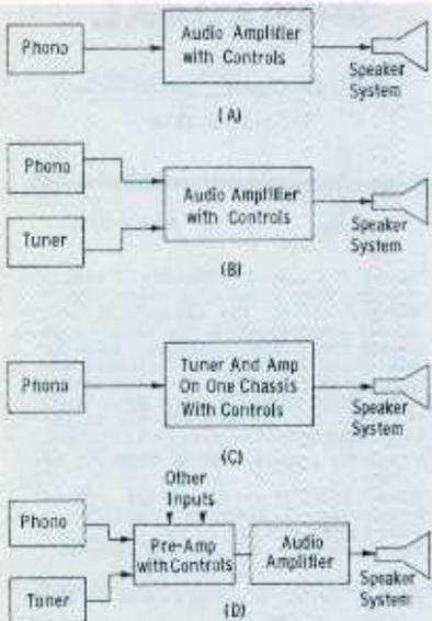
Fig. 1. Block diagrams showing components used in various hi-fi systems.
