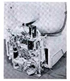
Fig. 2. Chassis can be operated while upended on bench behind the cabinet.
