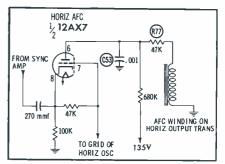
of the signal at the transformer winding was 450 volts p-p. R77 and C53 in series act as a load across this winding; and, since the impedance of C53 at 15,750 cps (in ohms) is equal to only about one-fifth of the ohmic value of R77, about fourfifths of the pulse voltage will appear across the resistor.
