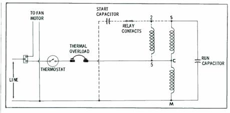
Fig. 6. Permanent split-capacitor motor does not need special start circuit.
