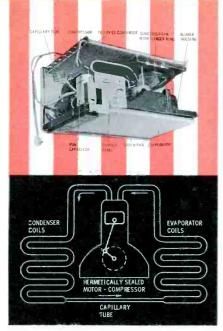
Fig. 1. Diagram showing the flow path of refrigerant used in air-conditioners.
