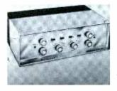
The Arkay CS-28 incorporates dual 14-watt stereo amplifiers and a pair of control preamplifiers, all on a single chassis. A reverse-stereo switch (for interchanging channels) and a balance control are included. Output taps are provided for speaker impedance of 4, 8, 16 and 32 ohms. Price is 664,95 (kit) or \$99.95 (wired).
