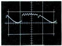
Fig. 18. Transients in the signal at screen grid of horizontal-output tube.
