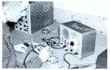
Fig. 1. Signal-tracing, substitution, and alignment of transistor radios is easy with Hickok's Model 810, which also featuers a test circuit for transistors.
