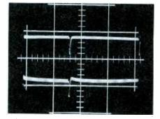
Fig. 4. Normal separation between the waveforms when C60 has no leakage.
