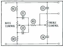
Fig. 4. Tone control circuit provides bass and treble boost and attenuation.
