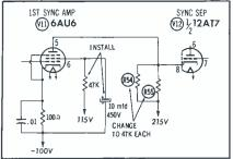
Fig. 12. Schematic showing sync-circuit changes to improve picture stability.
