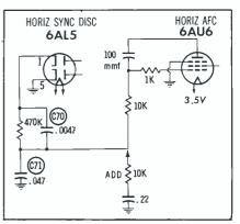
Fig. 11. Horizontal-AFC circuit showing changes to prevent bend in picture.
