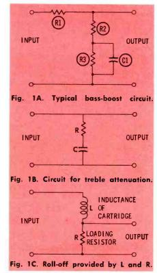
latter case, however, signal amplitude is decreased below its normal level. If C1 is open, the impedance across the output is considerably higher, resulting in greater voltage output, but there is a loss of bass boost. If R3 should open, boost will be excessive and hum level will increase.
