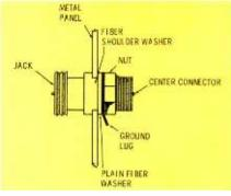
Fig. 1. Installation of miniature microphone connectors improves VTVM value. luck obtaining capacitors with special temperature characteristics from your local distributor. About the only ones I've been able to get consistently are zero and N750 types.
