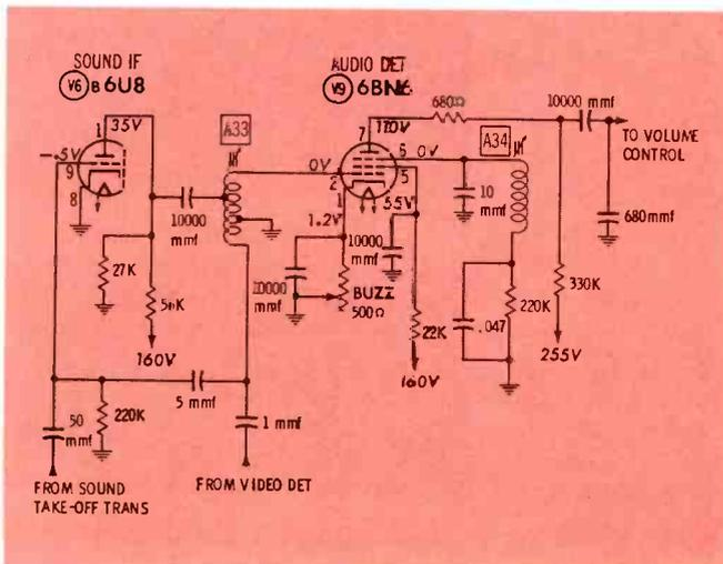
Fig. 2. Buzz control adjusts operating point of tube.
