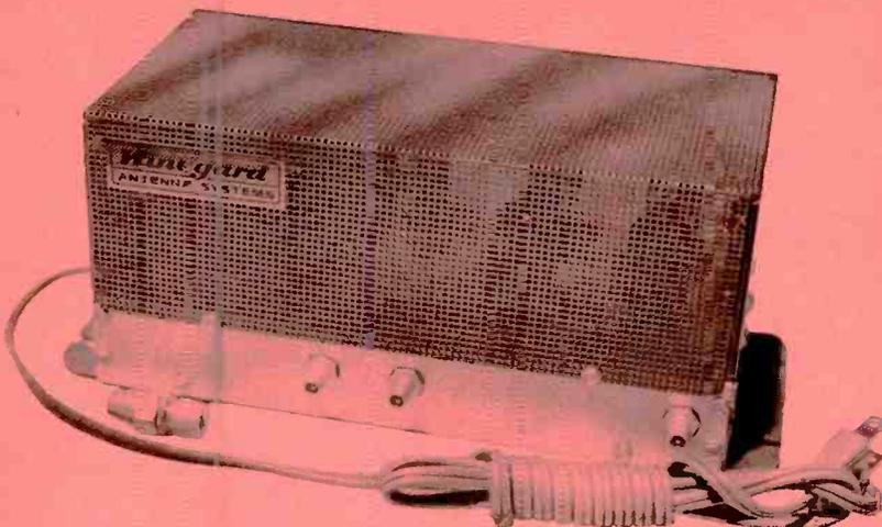
The heart of most master antenna systems is the broad-band distribution amplifier, which may be the only amplifier in the system. Its purpose is to provide signal amplification over the entire VHF band at a low noise level, with sufficient isolation between the various outputs to prevent interaction. Normal gain figures range from 15 to 25 db.
