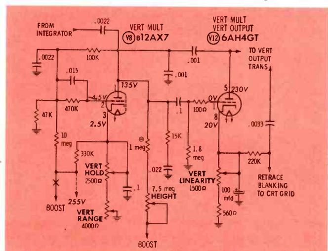
Fig. 3. Output tube is second half of multivibrator.
