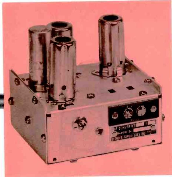
Live in a UHF area? Units such as this are used to convert any given UHF channel to a VHF channel of your choosing. Although each UHF channel requires its own converter, use of this type of unit eliminates the need for individual converters at each set.
