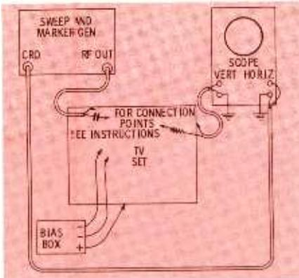
Fig. 2. Basic test equipment hook-up for performing a sweep alignment.
