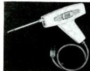
A new addition to the *Shop-mate* line of soldering guns and irons by Portable Electric Tools, Inc., is the Model SG-125 *Shop-Shooter* — a transformer-type gun with white nylon housing, a trigger extending the full length of the handle, and a screw-in 5" tip. Extensions and special tips are also available. Heating time is 2 1/2 sec; input current is 1.3 amps at 115 VAC; weight is 1 3/4 lb; and price is \$6.95.
