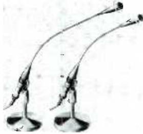
Long, slender necks of semi-rigid tubing are attached to the Electro-Voice Model 652 and 652A dynamic microphones in order to bring them close to the user's face without creating a "hiding behind the mike" effect. A clear plastic baffle, encircling the mike head, increases directivity and slightly boosts frequencies in the 6000-cps region for greater "brilliance" of sound.
