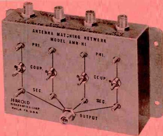
Some sort of mixing or matching unit must be used when two or more antennas are connected to the same "down line." If additional signal strength is required, you can get it from a mixer amplifier — if not, a low-loss, non-amplifying coupler (as shown) can be used.
