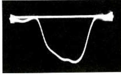
Fig. 8. Radiation from horizontal sweep circuit causes "hash" on curve.
