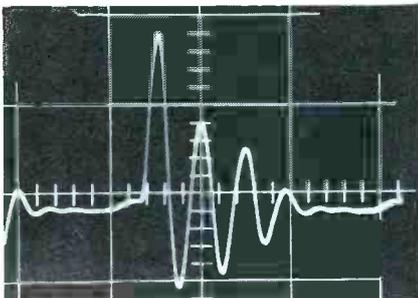
Fig. 3. Ringing in waveform taken from 1B3 lead pointed to damper trouble.
