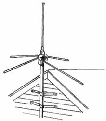
Base stations generally use a ground-plane antenna mounted in the same manner as a TV antenna. List prices for the antenna range from \$25 to \$50.
