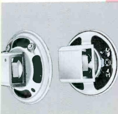
Transistorized portable radios, with outputs of only .25 to 1.5 watts, have 2" to 3" speakers with extremely shallow frames. When you're selecting a replacement, pay particular attention to the output circuit of the set. Some designs use a transformer and require speakers with 3.2-ohm voice coils, while others have direct-drive circuits and demand special speakers with an impedance of 100 ohms or more.
