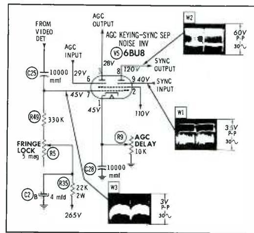
Fig. 4. Zenith Chassis 16F25 has a typical 6BU8 noise limiter circuit.
