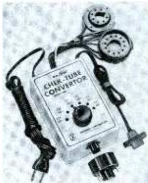
A multipurpose adapter newly introduced by Antronic Corp., the Anchor Model TC-438 "Chek-Tube Converter," permits connecting either the 90° or 110° type of 8" check tube to a CRT socket designed for either the conventional 12L duodecal base or the 8HR standard 110° miniature 8-pin base. In addition, a selector switch sets up the proper base connections and power ratings for substitution testing of five groups of CRT's having unusual filament characteristics. Price is \$11.95.
