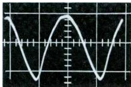
Fig. 5. Linearity-coil setting affects the phase of 15,750-cps boost waveform.
