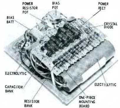
Fig. 6. Note the ease of accessibility to components on the Model 500 chassis.
