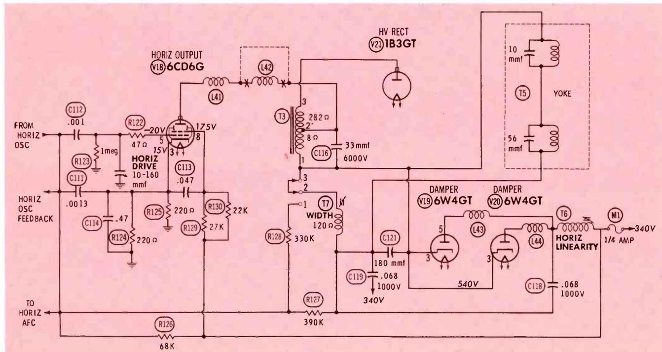
Fig. 1. Schematic of direct drive horizontal sweep circuit used in RCA Chassis KCS81F.
