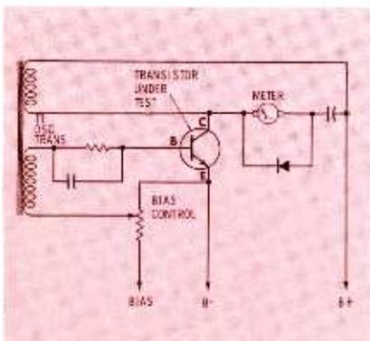
Fig. 2. NPN transistor connected into the oscillator circuit of Model TR110.
