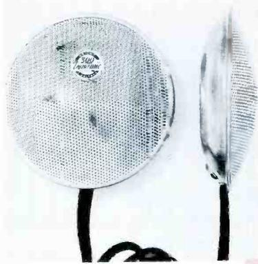
Although "personalized listening" once meant "ear-phones," accessory speakers are now available which can be slipped under a pillow or placed right next to the listener's ear. These units can be connected directly into the speaker circuit of home-entertainment equipment, and also used as a microphone.
