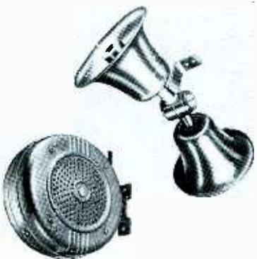
Paging speakers can also serve as microphones. Frequency response may be broad enough to permit use in combined intercom and background-music systems. Power ratings vary from 5-40 watts—depending on size. Most are single re-entrant horns, but special units may be used for bi-directional coverage.
