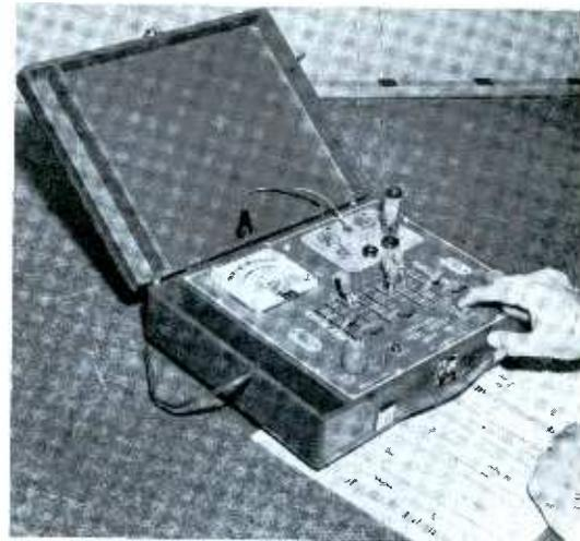
Fig. 7. Superior Model 85 checks the tubes for shorts, leakage, and quality.
