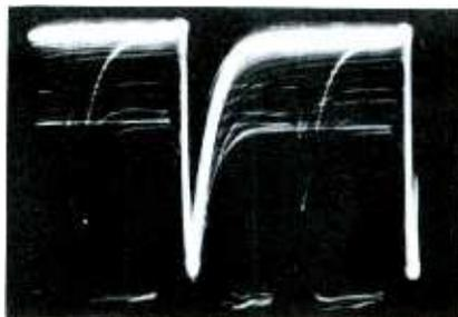
(A) Normal sync-pulse waveform.
