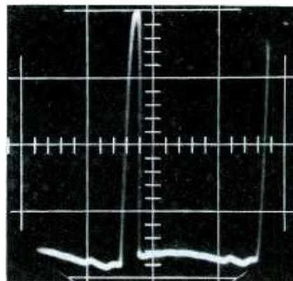
Fig. 4. Waveform normally obtained when scope probe is attached to 1B3.
