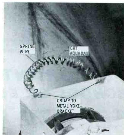
Fig. 2. Improvising a ground for the aquadag coating is no real problem.
