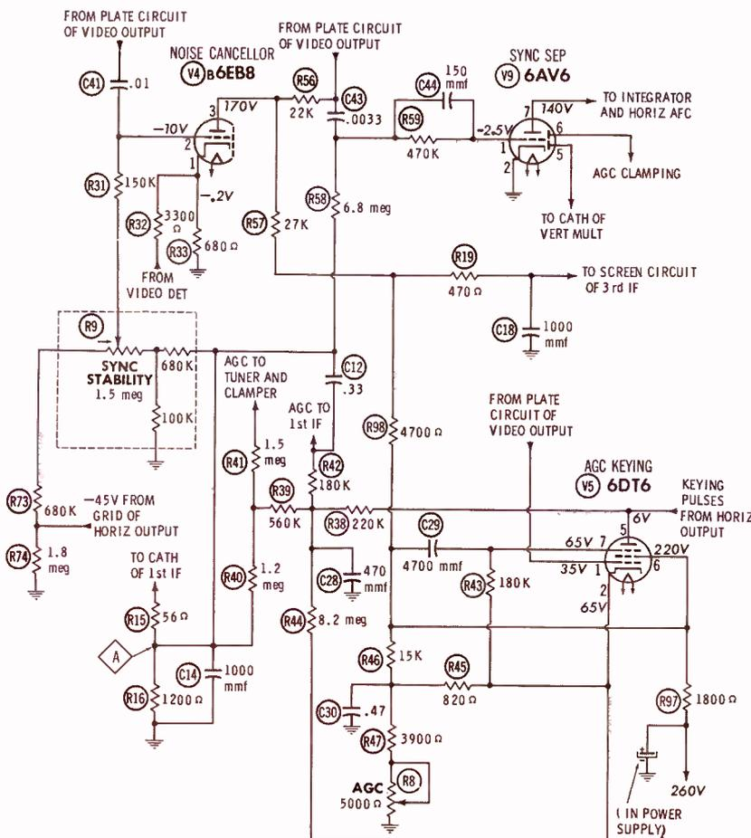
Fig. 1. RCA Chassis KCS131 has noise-inverter triode and 6DT6 AGC tube.
