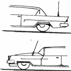
Special "loaded" antennas for mounting to fender, trunk, or roof are available for mobile use and list for around \$25 complete.
