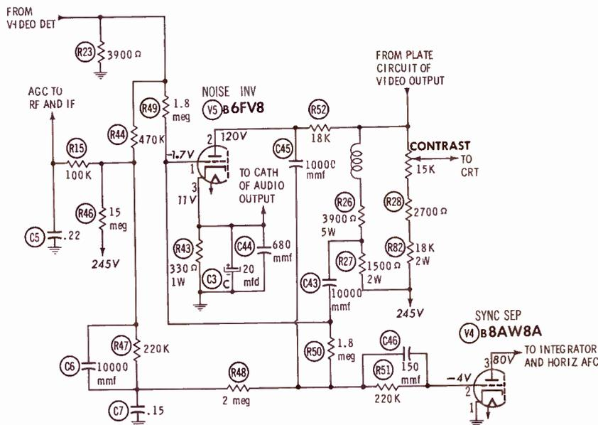
Fig. 3. Westinghouse V-2384-15 has different version of triode circuit.
