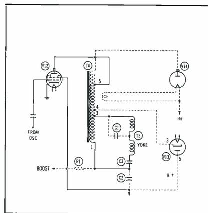
Fig. 2. The horizontal sweep and high-voltage circuit reduced to essentials.
