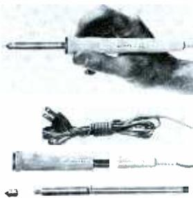
Different models in the Ungar "Imperial" line of soldering irons are assembled from the following assortment of interchangeable, individually-available components: 25-, 30-, and 40-watt heat cartridges; polycarbonate-resin "Perma-Cool" handles with patented heat-sink design, in three pastel colors; 42 threaded "Mini-Tips" in a choice of three materials; and three types of power cords, including two designs for use with grounded three-terminal outlets.
