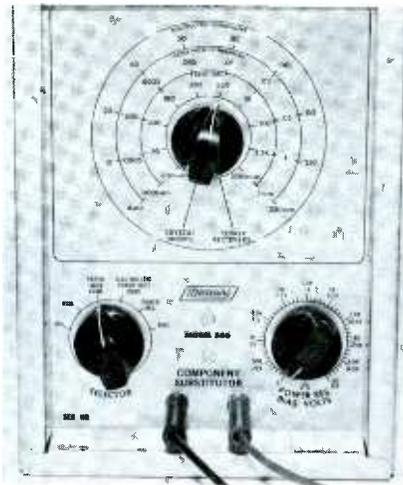
Fig. 5. Two switches and one control select all functions of the Substitutor.
