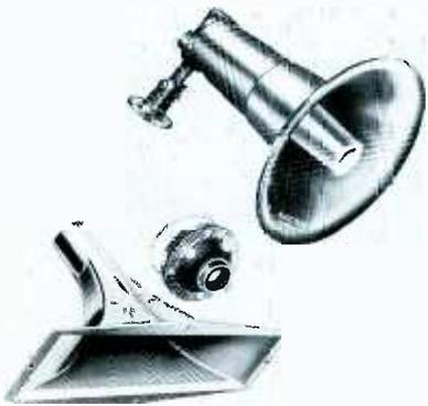
Many horns used in public address applications are two-piece units, with the voice coil and magnet housed in a detachable driver. However, one-piece horns are gaining popularity because of advantages such as lower price. Both integrated and two-piece types have similar electrical ratings—for example, outputs of 10-100 watts and frequency response of 75-7000 or 100-10,000 cps.
