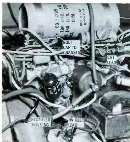
Fig. 1. CRT substitution may involve the addition of a high-voltage filter.
