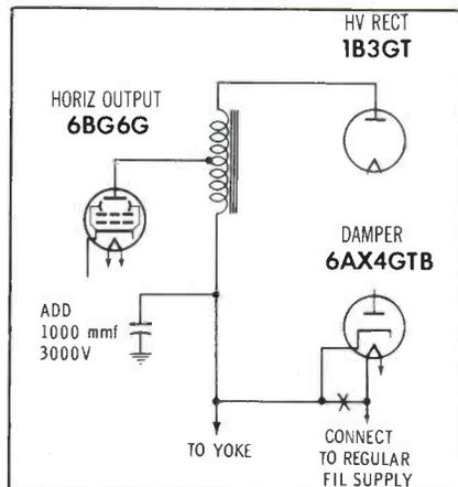
ment to the other filaments. However, I couldn't hold a yoke in the set until I bypassed the damper cathode to ground with a 1000-mmf, 3000-volt capacitor. The set would operate for an hour or two, and then the horizontal yoke winding would start arcing to the vertical winding. Since I installed the bypass capacitor, it has held up.
