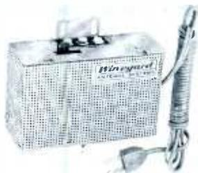
The amplifier circuit in the Winegard AT-6 "Booster-Pack" broadband TV-FM amplifier, using a low-noise MADI transistor, develops a gain of 16 db on the low VHF band and 14 db on the high band. A three-position switch selects full gain, reduced gain, or amplification of signals picked up on the line cord in strong-signal areas. The unit obtains AC power through an isolation-transformer supply. List price is \$34.95.
