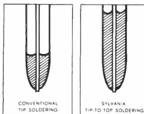
"Tip-to-top" soldering is what Sylvania calls their newest improvement in picture tube manufacturing. It involves use of tapered socket pins with solder extended throughout the entire length. The new technique will result in more firmly seated sockets, and will minimize service callbacks for cracked picture tube bases and open or intermittent base pin connections.
