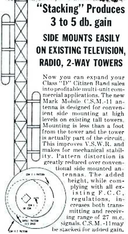
Two C.S.M.-11 Units stacked on opposite sides of the tower produce 3 db. gain . . . stacking two units on the same side of the tower produces a directional pattern with 5 db. gain!
