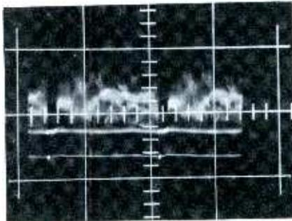
Fig. 4. Normal signal at control grid of video output tube (30 cps; 14V p-p).
