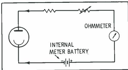
Fig. 6. Phototube can be checked by ohmmeter if proper polarity is used.
