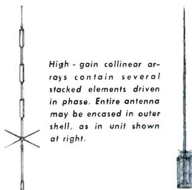
High-gain collinear arrays contain several stacked elements driven in phase. Entire antenna may be encased in outer shell, as in unit shown at right.
