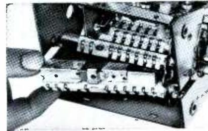
**6.** Tuner designed for quick, easy UHF conversion on the spot. You can convert tuner to take up to 4 UHF stations, *switch strips without disassembling tuner or drum.*
