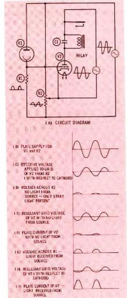
Fig. 3. Operation of a photoelectric control amplifier supplied with AC.
