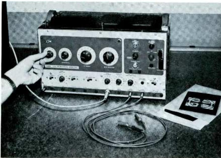
Fig. 1. The *Analyst*—a complete TV generator to save troubleshooting time.
