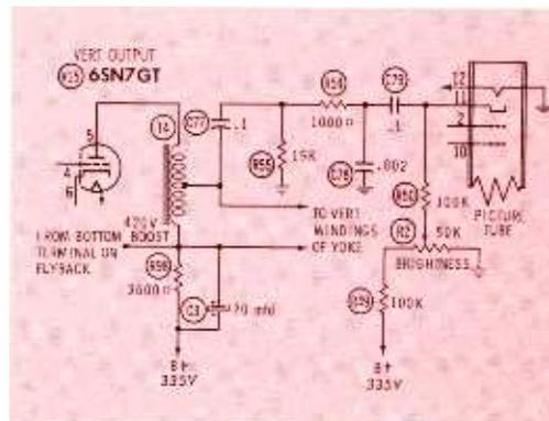
Fig. 2. Interfering signal can reach the CRT through retrace-blanking circuit.
