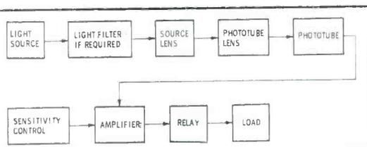
Fig. 5. Block diagram of photoelectric system is aid in troubleshooting.
