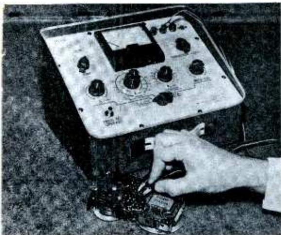
Fig. 4. The new Hickok Model 890 tests transistors either in or out of circuit.
