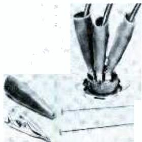
The tip of the Mueller "Micro-Gator" test clip has jaws 1/32" wide, with a 7/32" maximum spread. This clip, available in cadmium-plated steel or solid copper, can be soldered onto #20 or smaller wires and crimped in place with strain-relieving ears. Sold separately are skin-tight, flexible vinyl insulators, which cover the entire clip, but are split at the tip to allow the jaws to open.
