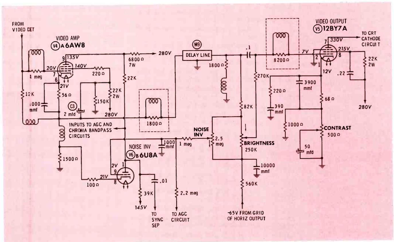
Fig. 3. Video amplifiers and noise-inverter stage of the RCA Chassis CTC7A.
