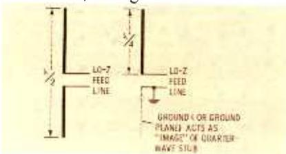
This drawing shows similarities between half-wave dipole (Hertz) and quarter-wave (Marconi) antennas.
