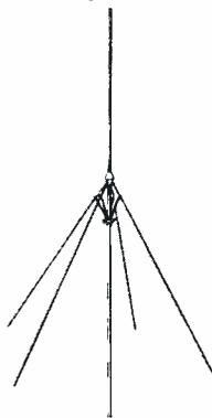
Quarter-wave antennas mounted high in air use ground plane to stabilize operating characteristics.
