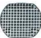
**Crosshatch Pattern...**A crosshatch of thin sharp lines for adjusting vertical and horizontal linearity, raster size and overscan. **Dot Pattern** (not illustrated) permits accurate color convergence.
