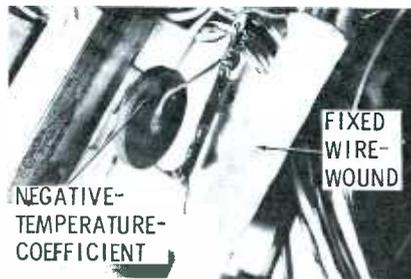
Fig. 1. Combination of two resistors protecting a series filament circuit.
