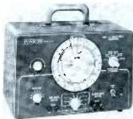
The **Paco Model G-34** generates both sinusoidal and square waves at any frequency between 6 cps and 750 kc. Maximum output obtained across a 600-ohm load is 10V rms for sine waves, or 18V p-p for square waves; amplitude is controlled by an attenuator switch and potentiometer. Rise time of square waves is less than .15 usec. Frequency accuracy is  $\pm 5\%$ .
