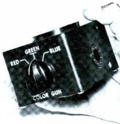
Fig. 4. Test head eliminates the need for additional test-socket adapters.
