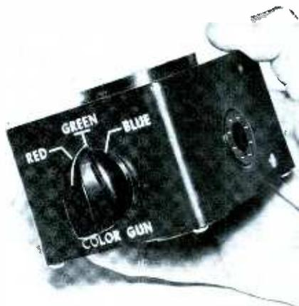
Fig. 4. Test head eliminates the need for additional test-socket adapters.
