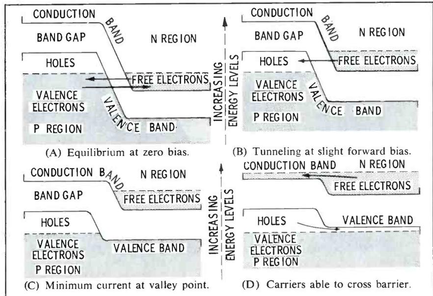
Fig. 5. Current across junction in a typical General Electric tunnel diode.
