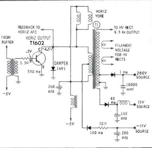
Fig. 5. Flyback circuit produces several rectified voltages, but no boost.
