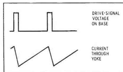
Fig. 6. Square drive pulse is needed to produce a sawtooth current in yoke.
