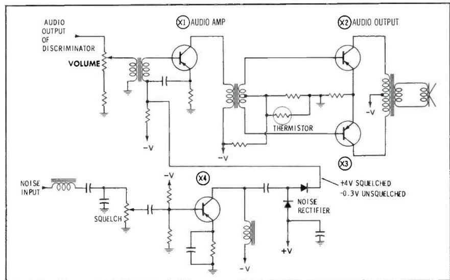
Fig. 4. Audio section with adjustable squelch and stabilized output circuit.
