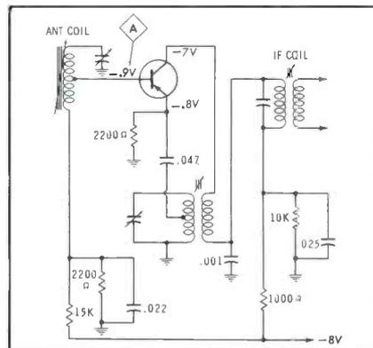
**Fig. 7. Converter circuit combines the functions of the oscillator and mixer.**
