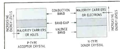
Fig. 3. Current carriers in a diode occupy two different energy levels.
