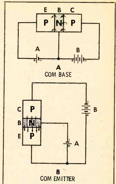
Fig. 5. Bias voltages for PNP transistor are opposite to those of an NPN.
