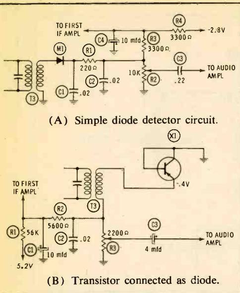
Fig. 12. Detectors in transistor radios.
