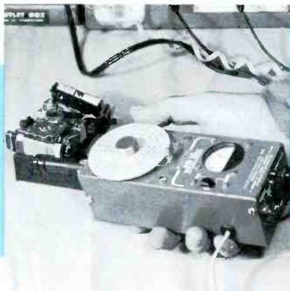
Asked if there were any other tools or instruments he found useful in minimizing trouble-diagnosis time, Wayne replied, "Sure is—a low-frequency grid-dip meter. I use mine to inject alignment signals, to substitute for the local oscillator, and to check the resonance of loopstick and oscillator coils. Since it also supplies higher frequencies, I find it useful for checking short-wave and FM bands, too."
