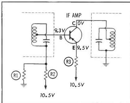
Fig. 2. DC voltages in transistor circuit are valuable troubleshooting aid.
