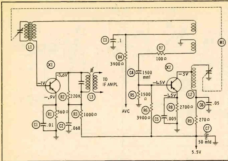
Fig. 17. Oscillator-mixer-RF stage uses coil for feedback and mixer injection.
