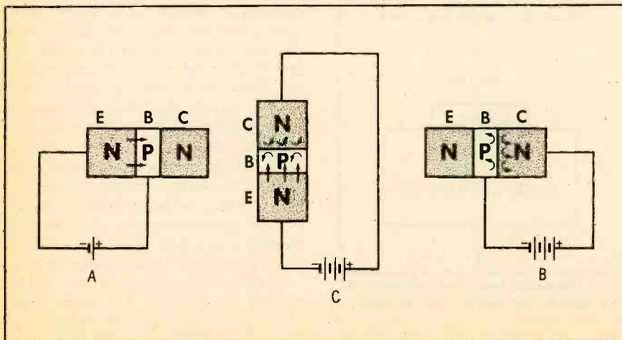
Fig. 3. Transistor bias arrangements show how junctions conduct or block.
