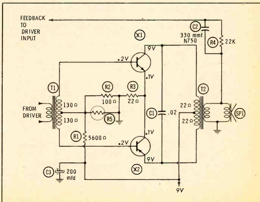
Fig. 11. Matched transistors add to balance in push-pull output stages.
