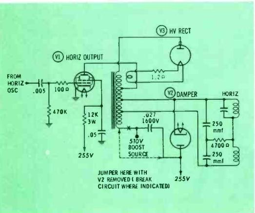
Fig. 2. Substituting B+ in place of boost voltage isolates faulty component.
