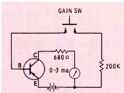
Fig. 1. A method for obtaining leakage and transistor relative-gain checks.
