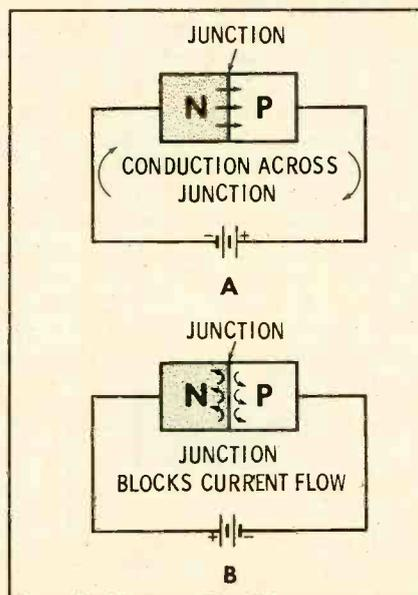
Fig. 1. Forward bias and reverse bias of a simple NP diode semiconductor.
