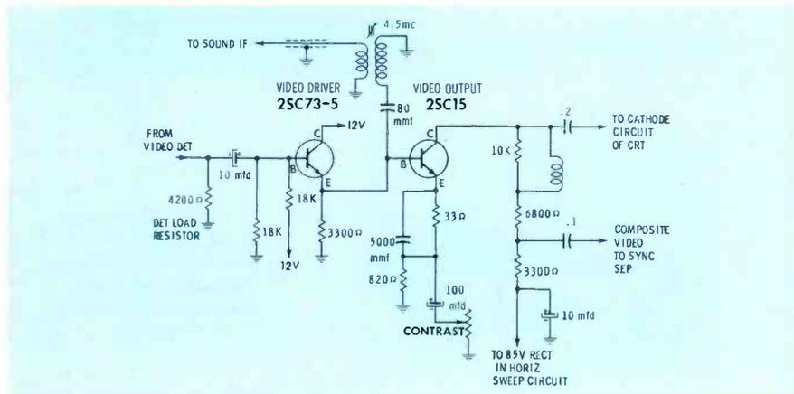
Fig. 2. Driver couples video signal to the output stage without amplification.
