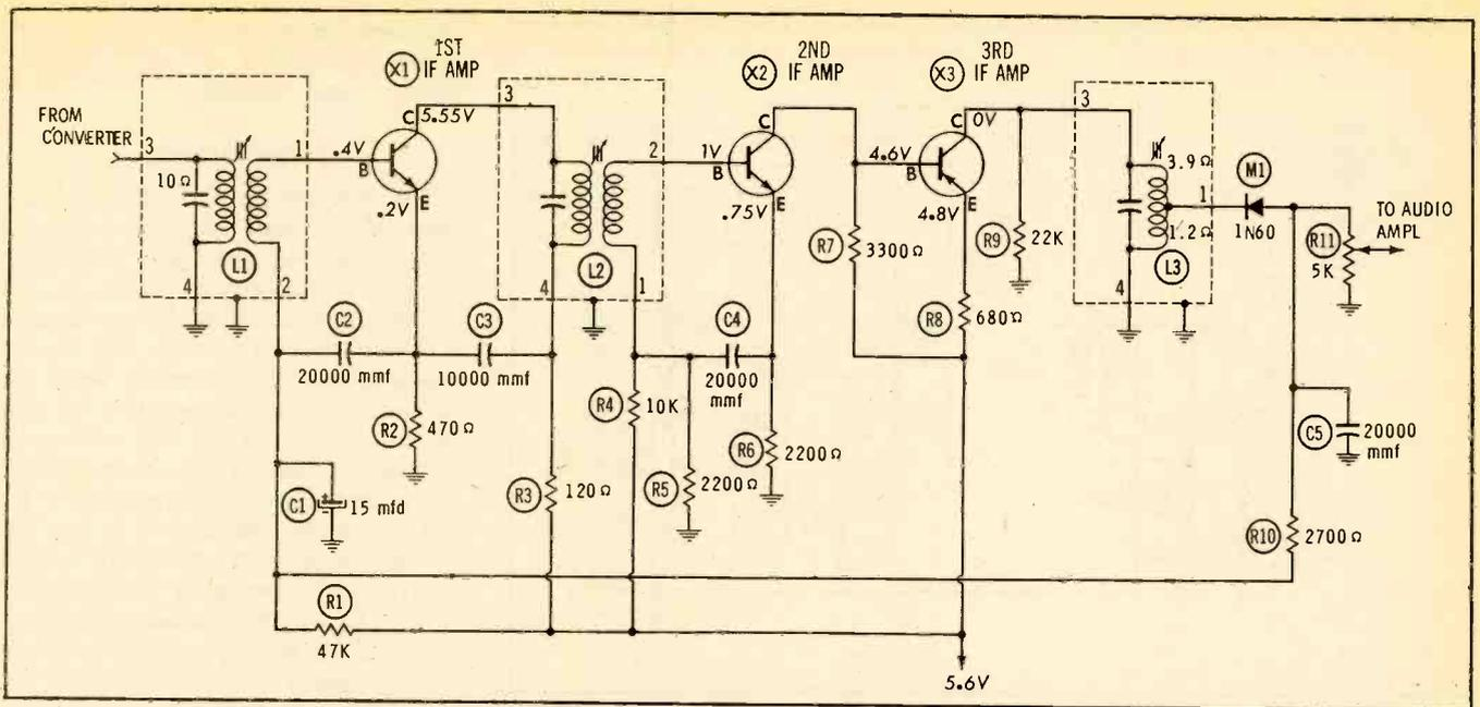
Fig. 15. IF system uses a wide variety of IF amplifier circuit configurations.
