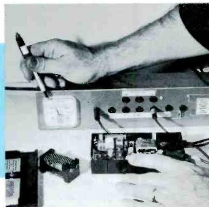
"I still have the home-made battery-operated power supply I started with," reports Wayne, "although I have since purchased two commercially - available units which are even better. One of the first tests I make, regardless of the trouble, is to measure total battery drain. Even if the radio seems to operate normally, excessive drain from a leaky transistor or capacitor may be running down the batteries too quickly."
