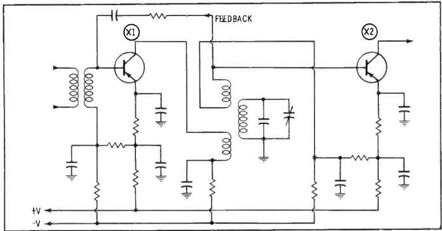
Fig. 3. Tunable high-IF stage is neutralized by feedback from transformer.
