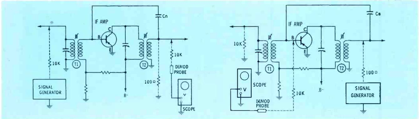
Fig. 1. Two-step setup to check the neutralization of a video IF stage.
