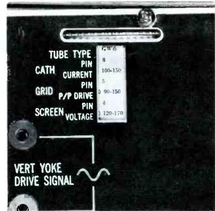
Fig. 3. Roll chart indicates important horizontal-output tube characteristics.
