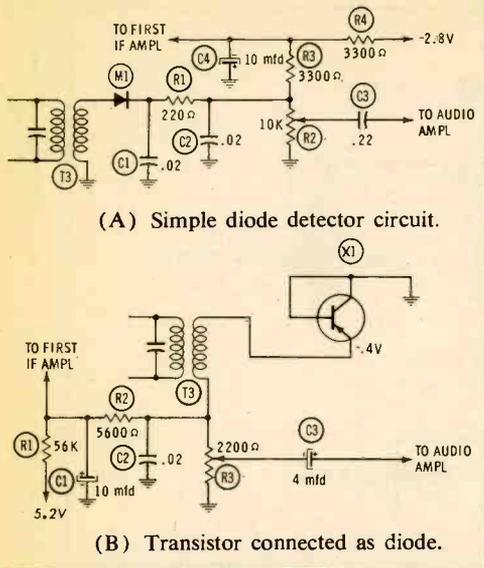
Fig. 12. Detectors in transistor radios.
