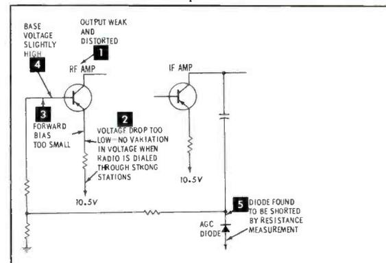
Fig. 5. Steps in troubleshooting an AGC fault in all-transistor car radio.
