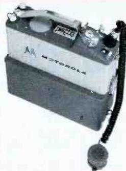
Portable FM "Handie-Talkie" by Motorola uses tubes only in RF section of transmitter. Switch on top of case selects one of two channels.
