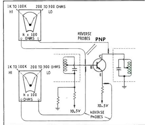
Fig. 4. Transistor can be checked with ohmmeter in same way as crystal diode.
