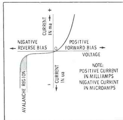
Fig. 2. Voltage-vs-current curve for conventional germanium crystal diode. slope obtained when the diode is operating in the *avalanche* region.
