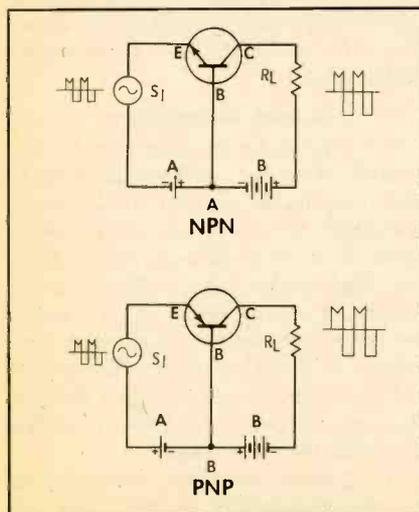
Fig. 7. Common-base circuits amplify without reversing phase of the signal.
