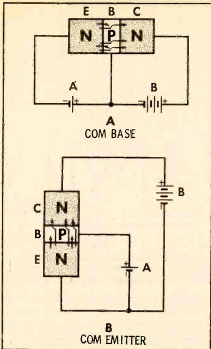
Fig. 4. Common-base and -emitter bias configuration of NPN transistor.
