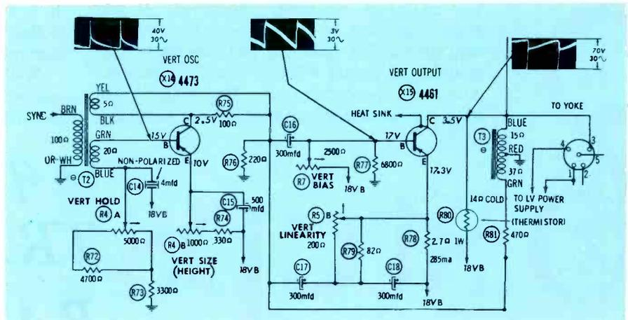
Fig. 4. Most transistorized vertical sweep systems use blocking oscillators.
