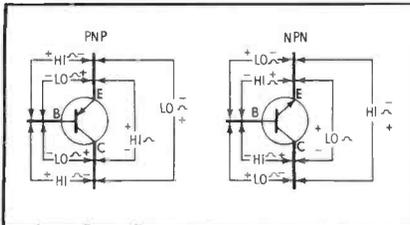
Fig. 8. Expected results of ohmmeter reading between two transistor leads.
