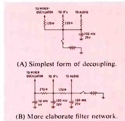
Fig. 3. Decoupling networks keep signals from entering improper circuits.
