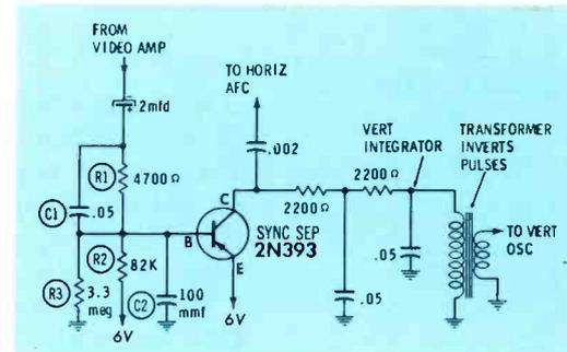
Fig. 3. Simple sync-separator circuit produces positive pulses at collector.
