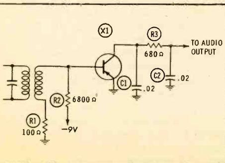
Fig. 14. This detector amplifies audio.
