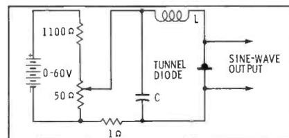
Fig. 6. This tunnel-diode oscillator produces output at approximately 11 mc.
