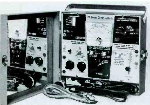
Fig. 1. New instrument simplifies the troubleshooting of deflection circuits.
