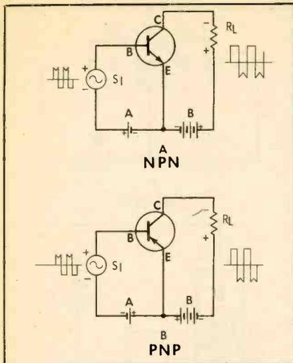
Fig. 6. Common emitter amplifier causes signal inversion in output load.
