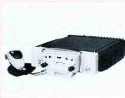
"Extender" circuit, controlled by switch on front panel of this Motorola mobile set, is used to increase effectiveness of noise rejection.
