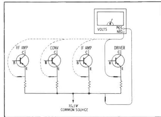
Fig. 3. Voltage drop across emitter resistors gauges transistor conduction.
