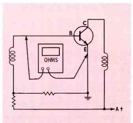
Fig. 3. An ohmmeter is connected between base and emitter in open-lead-test.
