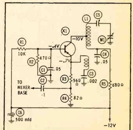
Fig. 16. Common-base oscillator uses a tickler coil for feedback to emitter.
