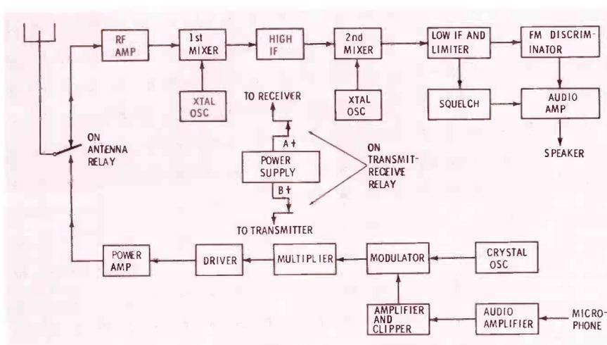
Fig. 1. Block diagram of two-way set with double superheterodyne receiver.
