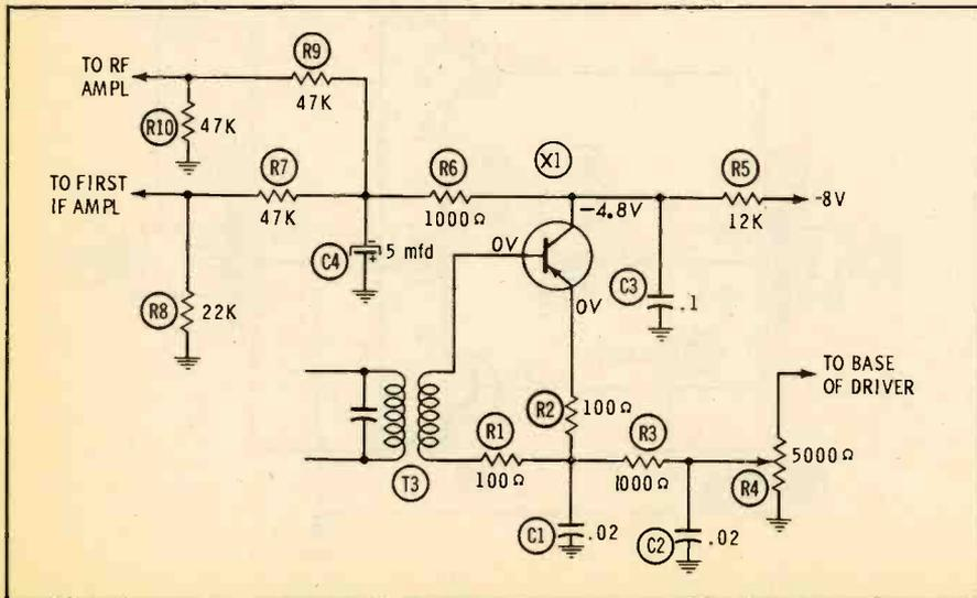
Fig. 13. Transistor detector includes an unusual AVC-circuit arrangement.
