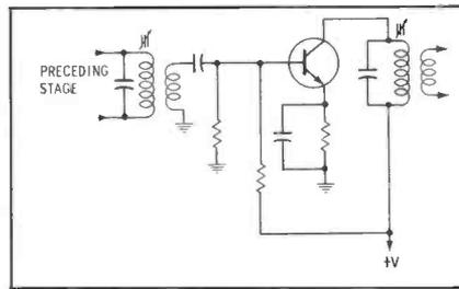
Fig. 6. Class-C stage for transmitter uses combined external and signal bias.
