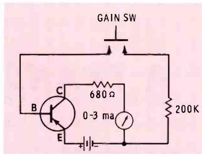
Fig. 1. A method for obtaining leakage and transistor relative-gain checks.
