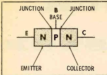
Fig. 2. Construction of an NPN transistor showing elements and junctions. emitter bias current causes the base-collector junction to conduct, and a large collector current flows from the negative to the positive terminal of voltage B.
