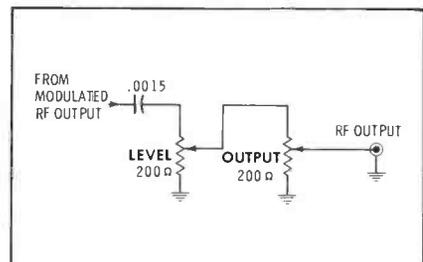
Fig. 5. Output-control system helps to prevent stray radiation from the unit.
