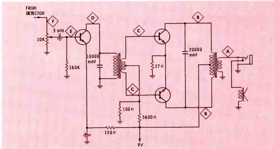
Fig. 4. Key test points form basis of step-by-step troubleshooting procedure.
