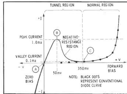
Fig. 4. High peak at B characterizes voltage-current curve of tunnel diode.
