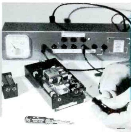
Wayne is constantly on the alert for tools and other devices especially designed for working with miniature portables. We found him already using two special drivers that hadn't been on the market more than a week or so. "Removing and replacing earphone nuts and jacks used to be tricky. I even went to the trouble of grinding down a screwdriver. These subminiature drivers are just what I needed."
