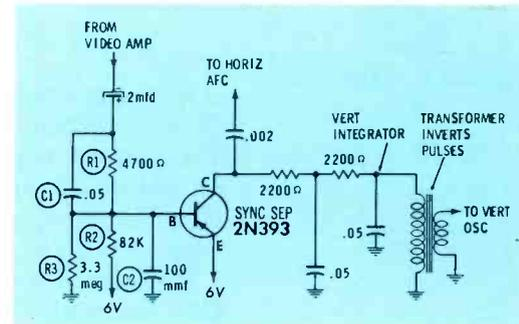
Fig. 3. Simple sync-separator circuit produces positive pulses at collector.
