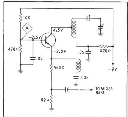
Fig. 6. Typical oscillator circuit is normal if tuning varies bias voltage. Develop some operating fault, or a defective transistor may just refuse to sustain oscillation. Voltage measurements and component tests will lead you to the trouble in short order.
