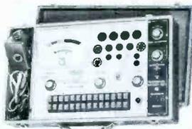
A new dynamic mutual conductance tube tester from Mercury is characterized by push-button settings. Known as the Model 1200, the unit will test tube types with all basing arrangements, plus black-and-white picture tubes, transistors, and batteries. In addition to transconductance tests, the
