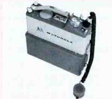
Portable FM "Handie-Talkie" by Motorola uses tubes only in RF section of transmitter. Switch on top of case selects one of two channels.
