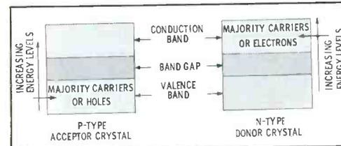
Fig. 3. Current carriers in a diode occupy two different energy levels.
