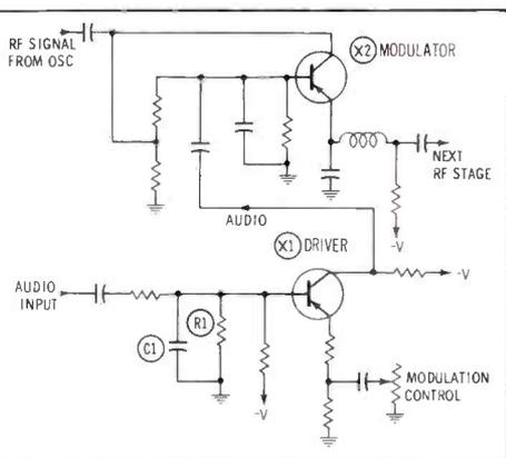
**Fig. 7. Driver prepares audio signal for application to phase modulator X2.**
