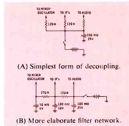
Fig. 3. Decoupling networks keep signals from entering improper circuits.
