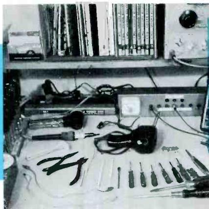
Just what does it take to put yourself in business? According to Wayne, "If you already service tube radios, you probably have most of the necessary equipment. The rest can be purchased for \$100 or less." Included in this array photographed at his shop are a power supply, VOM, signal-tracer, grid-dip meter, regular- and miniature-size tools, substitute transistors and batteries, and of course all the pertinent service data.
