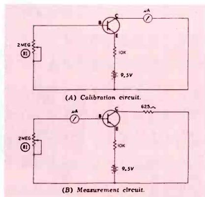
Fig. 2. A typical circuit for obtaining an actual reading of transistor beta.
