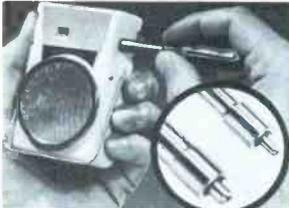
Designed to release the spanner nut found on external antenna and earphone jacks of many imported transistor radios, a special wrench manufactured by **Xcelite** is available in two sizes. Both the 1/4" and the 5/16" size have a plastic handle and a pocket clip. A guide pin centers the tool and two projecting keys fit slots in the spanner nut, which must be removed before the chassis can be lifted from the case for servicing. Price is 80c for either size.
