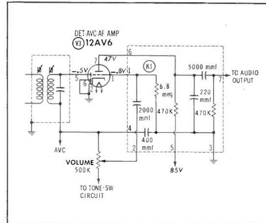
conductor between lead 1 of K1 and pin 1 of the 12AV6.
