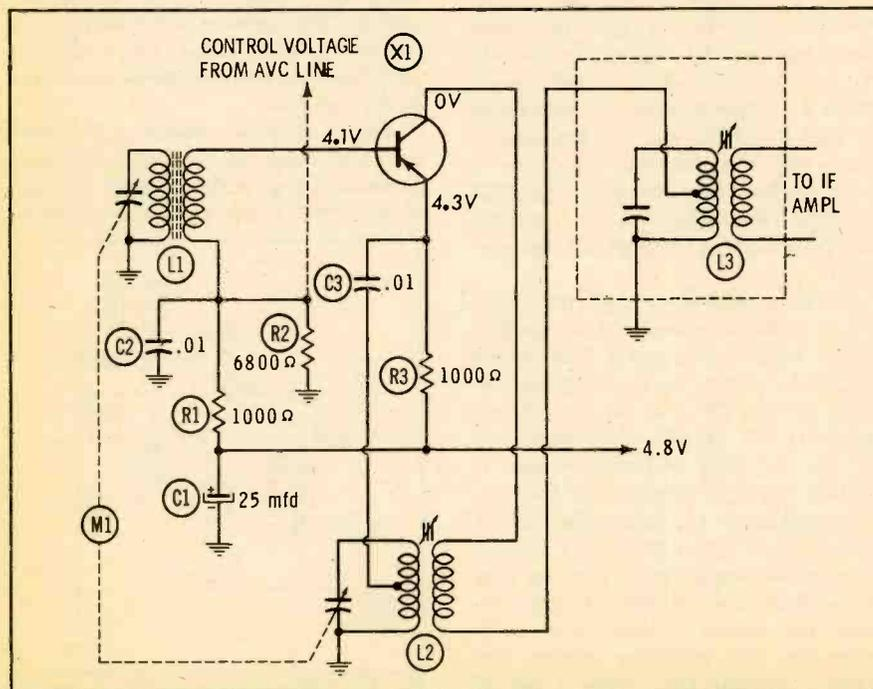
Fig. 18. One transistor serves as an oscillator, mixer and RF amplifier.
