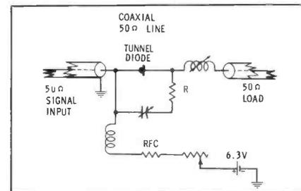
Fig. 7. Resistor is used in this 30-mc amplifier to prevent oscillations.
