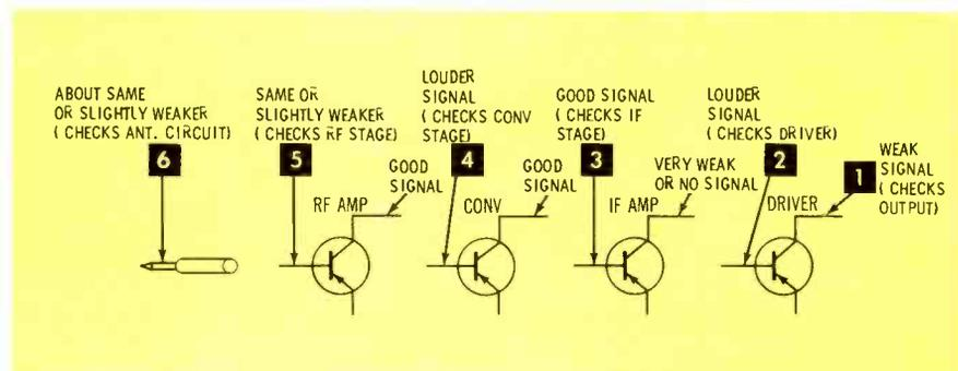
Fig. 1. Results expected in progressive steps of signal-tracing procedure.
