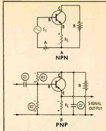
Fig. 8. There is no gain in a common-collector amplifier and no inversion.
