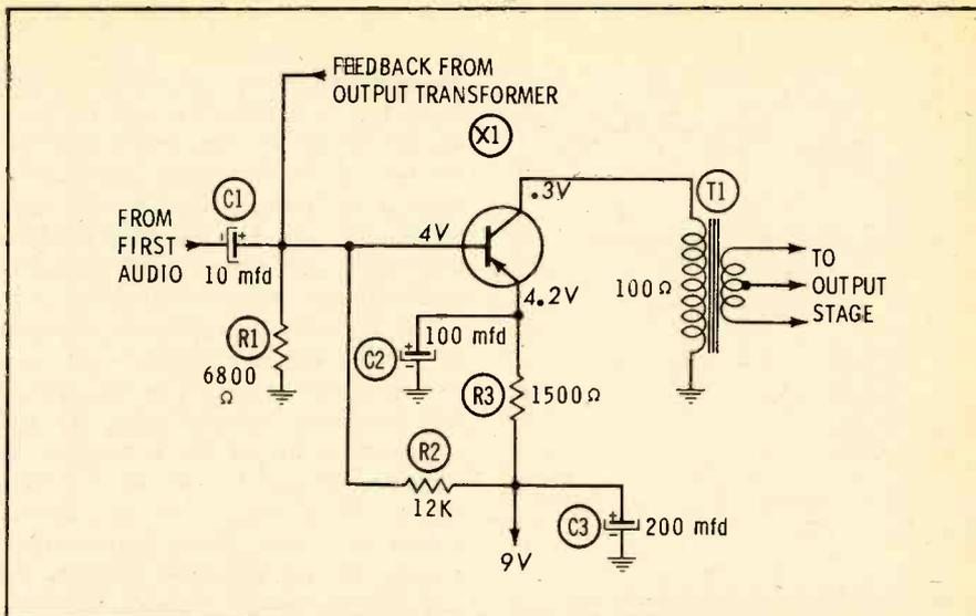
Fig. 10. Driver stage furnishes power by keeping current high in the load.
