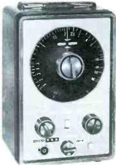
Capacitors can be checked either in or out of circuit with the **EICO Model 955**. The tester includes a Wien bridge to allow in-circuit capacitor measurements even when shunt resistances are comparatively low. Capacity is read from a 4" lucite dial after it has been adjusted to a "null" by an RC Balance Control. The control is calibrated in RC product, and has two ranges—.6 to 10.5, and 7.0 to infinity. Price of the kit is \$19.95; the wired unit is \$39.95.
