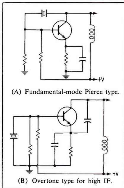
Fig. 5. Crystal oscillator circuits.
