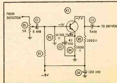
Fig. 9. This voltage-type amplifier is found very often in transistor radios.
