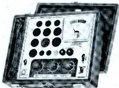
Fig. 1. Small tube tester contains sockets for latest receiving types.
