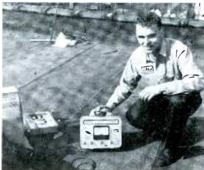
Official tests at receiving sites include measurements with UHF-VHF field-strength meter.
