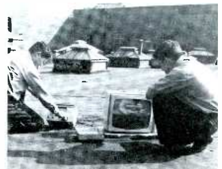
In addition to field-strength tests, signals are monitored on TV sets to check picture quality.
