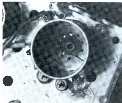
(A) Crack caused "intermittent."
