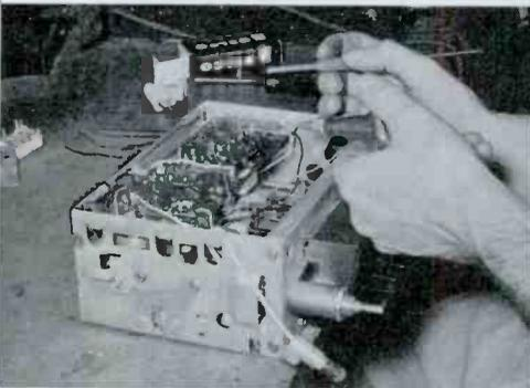
After using a soldering iron to heat the contacts until the solder melts, this technician uses an air gun to clear the solder away from the component contacts. A fine wire brush finishes the job.
