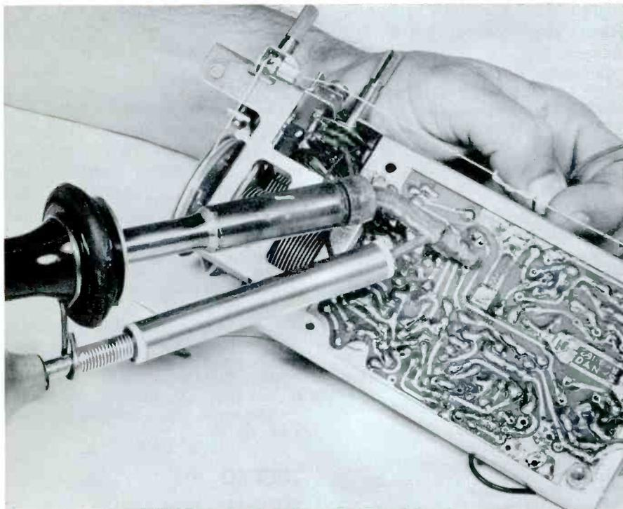
This photo shows one of the methods you might try for easier removal of multiple-lead components, such as the miniature transformers found in transistor radios, or IF cans in television sets. This job requires a bit of caution. Some technicians run into trouble because they apply too much heat to a small area of the board, unbonding the foil; others damage components by pulling too hard in trying to rock them loose.
