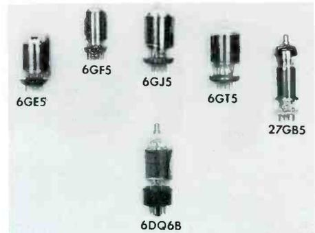
Fig. 2. Compactron and novar horizontal output tubes compared to a 6DQ6B.
