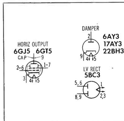
Fig. 3. Several 1963 models contain one or more of these novar tube types.
