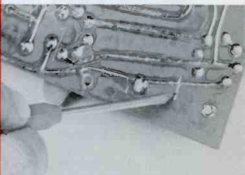
To isolate an individual component for testing, without dismantling it from the board, try cutting the printed foil with either a razor blade or the special tool shown. The cut is easily repaired later.
