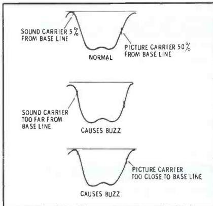
Fig. 4. Buzz may occur if sides of IF response curve have incorrect slope.
