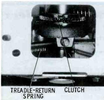
Fig. 3. Close-up of clutch and treadle.
