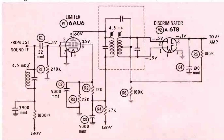
Fig. 2. Discriminator depends on limiter to suppress buzz in input signal.
