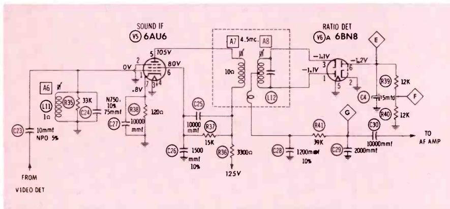
Fig. 1. Electrolytic capacitor in ratio detector filters out buzz.
