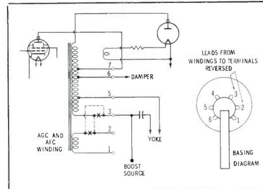
Fig. 4. Wrong connection in this flyback was located by ohmmeter check.
