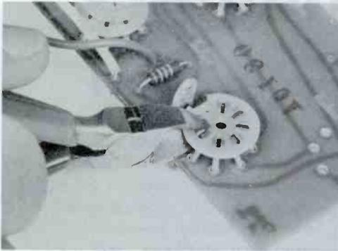
A relatively simple method of removing a defective tube socket without special adapters is shown here. After crushing the socket's phenolic wafer material, heat the individual pins and remove them with long-nose pliers.
