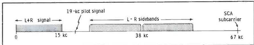
Fig. 6. The composite stereo signal is made up of several different signals.
