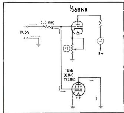
Fig. 2. Simplified schematic shows how grid-emission test is accomplished.
