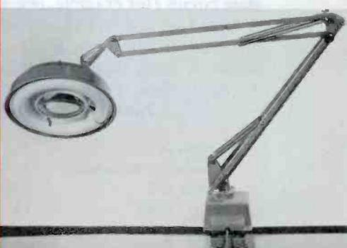
The adjustable light pictured here supplies shadowless lighting for printed-board work. It also has a built-in magnifying glass—a useful service aid for use with the miniature equipment now requiring the serviceman's attention.
