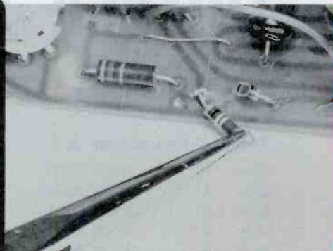
Shown here is the "hook" technique of replacing a resistor. Cut and crush the body of the old component to expose the full length of the leads. Form the old and new leads into hooks, clamp them together, and solder them carefully.
