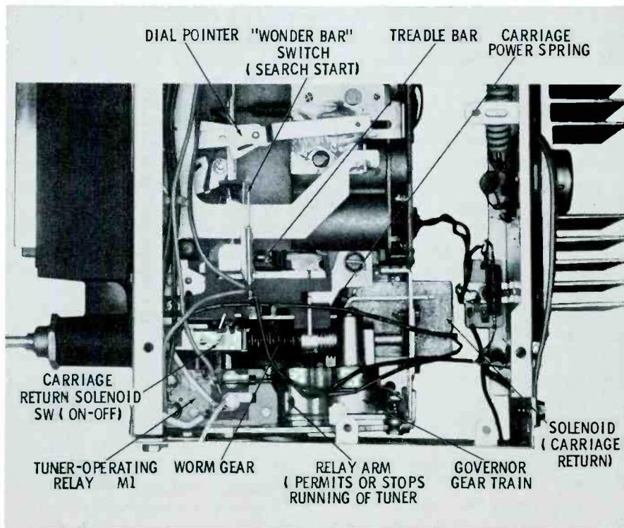
Fig. 2. Principal mechanical components of Delco F4-series search tuners.
