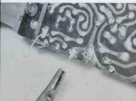
External connections for applying power or for testing purposes are easily provided by soldering one or more short wires to the printed board. Form them into a fish-hook pattern and clip on your leads, using miniature test clips.
