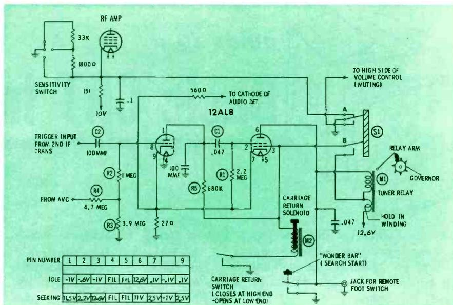
Fig. 1. Schematic of typical search-tuning system using solenoid return.
