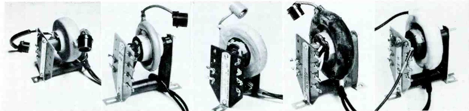
Fig. 2. Note similarity between original flyback (at left) and four different brands of replacements.
