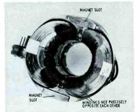
Fig. 3. Magnets can be installed in slots to counteract pincushion effect.
