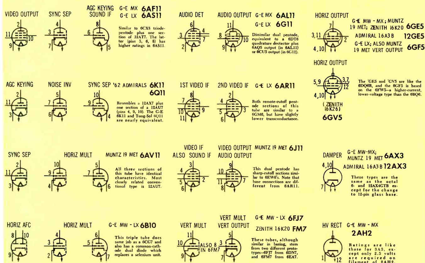
NOTE: ALL HEATERS ARE CONNECTED TO PINS 1 AND 12.
