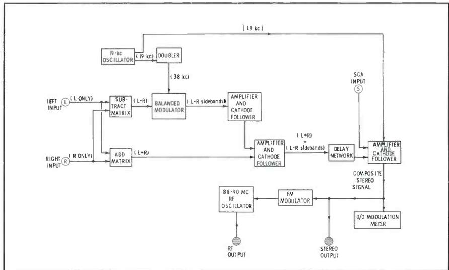
Fig. 5. Functional diagram shows how signals are developed within the unit.
