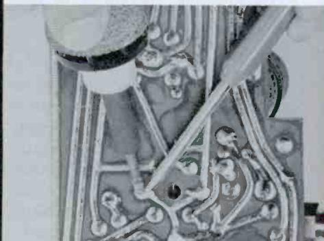
To prevent damage to an IF can, use the slotted end of a soldering aid to first straighten the ground tabs on the outer shield. With these tabs loose, the entire job of removal is made easier.
