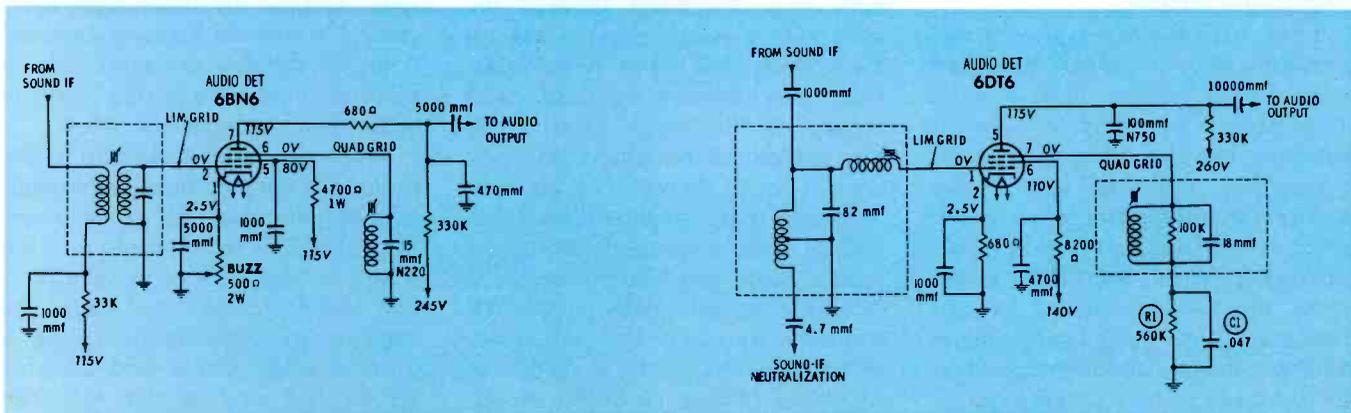
Fig. 3. Tube structure is main difference between 6BN6 and 6DT6 detectors.
