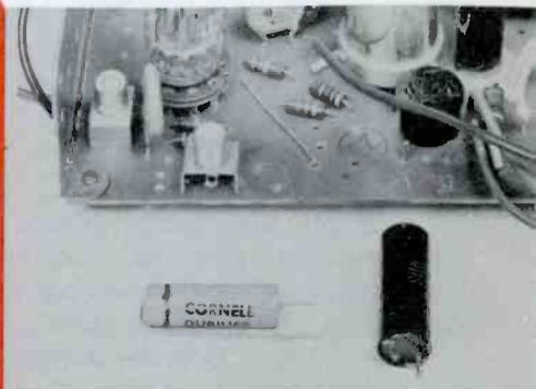
"Single-ended" components, such as the capacitor shown, can be replaced by the familiar "double-end" types, if you dress the leads on the new component in the manner shown here. Tape the wire close to the body of the unit.
