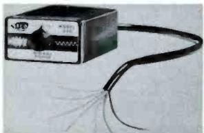
A dual high-mu triode and a dual diode are incorporated in an inverter circuit which clips noise impulses out of radio signals in **Seco's** Signal Filter. The unit reduces ignition interference, hash, and certain types of background noise. Adaptable to most tube-type Citizens-band receivers, the Signal
