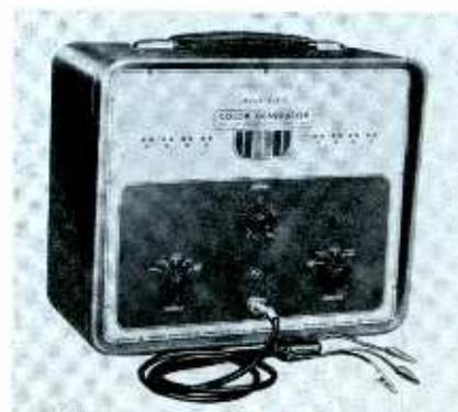
**Fig. 3. Newly developed keyed-rainbow signal generator for color servicing.**
