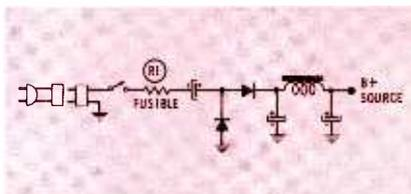
Fig. 1. Silicon rectifiers are commonly used in half-wave doubler circuit.
