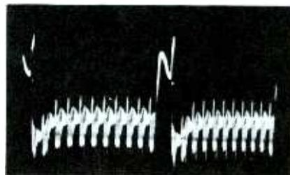
The output of the video amplifier stage is fed from this point to the chroma-bandpass and burst-amplifier stages. The waveform here shows us that the color signal is passing through the front-end stages in good shape. Loss of this signal, of course, would result in a "no-color" condition.
