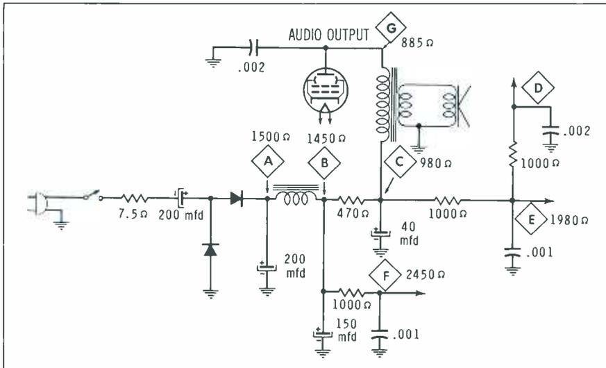
Fig. 4. Resistance method of localizing B+ shorts requires no unsoldering.
