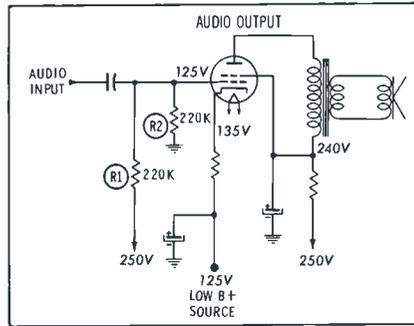
Fig. 5. Audio output tube serves as dropping resistor to develop low B+.
