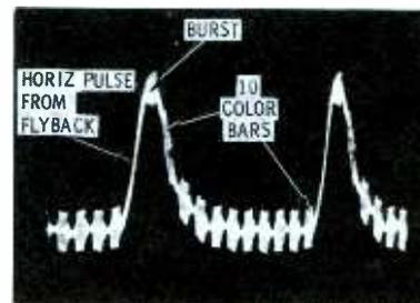
Look here for the presence of an incoming burst-and-color-bar signal combined with a keying pulse from a winding on the flyback. The burst signal can be seen sitting on the peak of the positive-going horizontal pulse, right where it belongs. The ten color bars produced by the generator are also well-defined.
