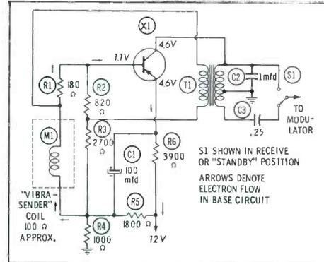
**Fig. 3. This transistorized oscillator drives a resonant-reed tone generator in the coil and thereby controls the operating frequency of the oscillator.**
