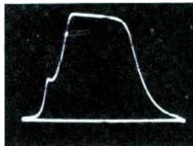
Fig. 3. Flat top on curve is too good to be true; the receiver is overloaded.
