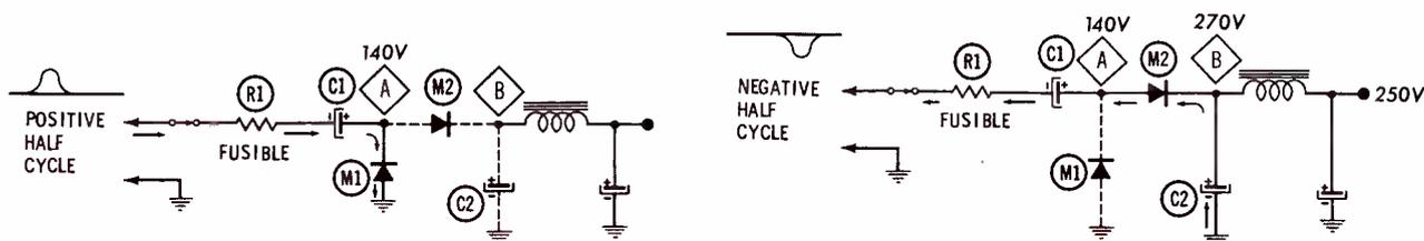
Fig. 2. DC output voltage of half-wave doubler is over twice the rms input.
