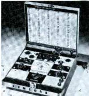
Two significant changes have been incorporated in all new **Sencore** Model TC114 "Mighty Mite" tube testers. An improved D'Arsonval meter is designed to provide increased reliability and damping. A large quick-setup chart, cemented inside the removable cover, eliminates the need to refer to the regular setup booklet for most-often-used tube types. Price of the Model TC114 is \$74.50 net.
