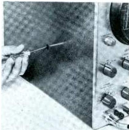
Fig. 2. Simple astigmatism adjustment.
