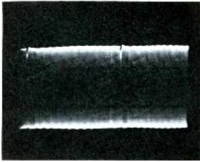
this CW signal is determined by the oscillator, and the relationship between it and the incoming burst signal sets the conduction of the phase detector. Loss of this feedback signal could result in wrong colors or out-of-sync color bars.
