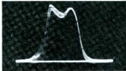
Fig. 5. Without capacitor, markers on wide-band scope may spread out.
