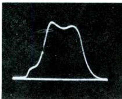
Fig. 2. Better ground connection from generator to receiver cured distortion.
