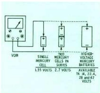
Fig. 1. Mercury cells are reliable as standards for DC voltage calibration.
