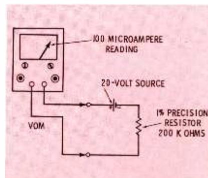
Fig. 2. Current through precision resistor is measured in milliammeter test.
