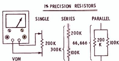
Fig. 3. Combination of precision resistors check accuracy of an ohmmeter.
