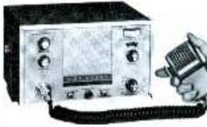
Receiver fine-tuning is provided for in the "Commaire" ED-276 transistorized Citizens-band transceiver manufactured by **Vocaline**. Other features of the unit include a signal-control squelch and RF gain, double-conversion receiver, and a three-stage AGC circuit. The ED-276 uses 22 transistors, 8 diodes,
