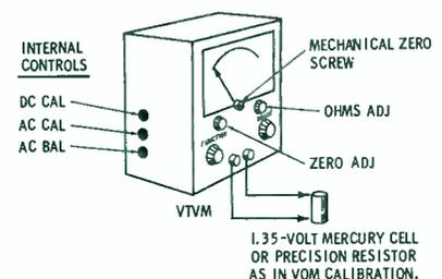
Fig. 4. These are the most important calibration points for typical VTVM.
