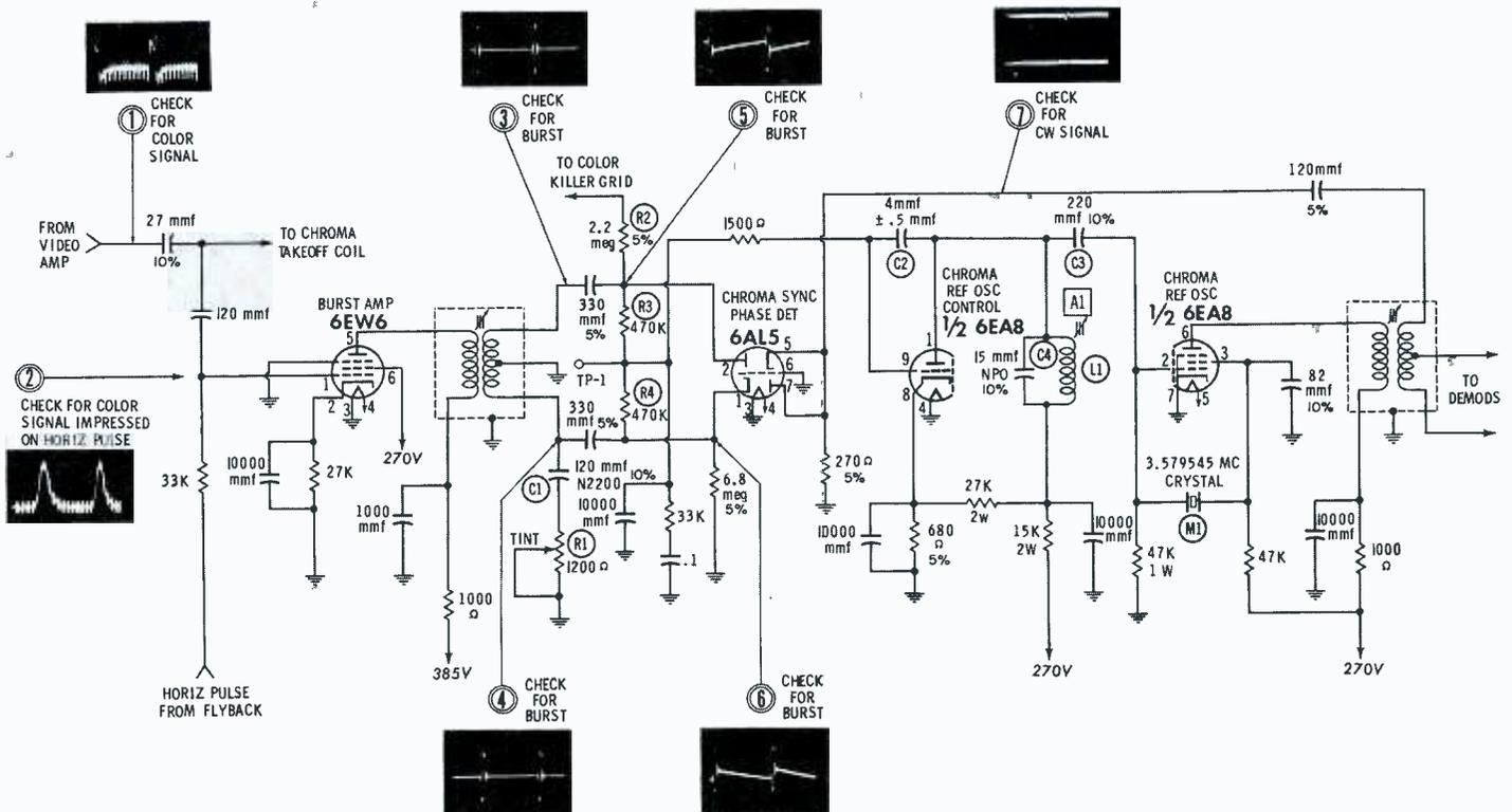
The transmitted color-TV signal contains a *color burst* (a sample of the chroma subcarrier) in addition to video, chroma, and deflection-sync modulation. In the receiver stages shown, the burst is amplified and compared with the 3.58-mc reference-oscillator signal. Any frequency error causes the chroma sync phase detector to apply a correction voltage to the grid of the oscillator-control tube, and the change in conduction of this tube makes the needed oscillator-frequency adjustment.
