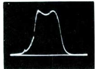
Fig. 4. The marker pip should be small and neat for best visibility on curve.
