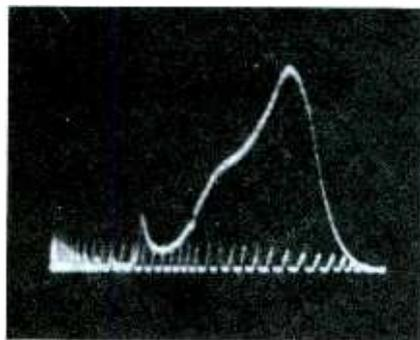
Fig. 1. Receiver is normal; distortion of curve is due to poor test setup.
