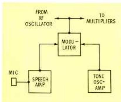
Fig. 1. Audio-frequency tone is applied to modulator stage in transmitter.
