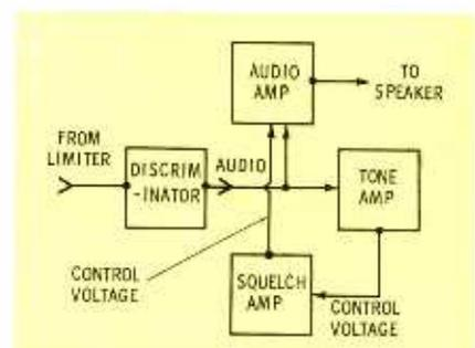
Fig. 2. In receiver, the tone circuit obtains its input from discriminator.
