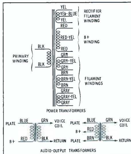
Fig. 4. EIA standard color codes for power and audio-output transformers.
