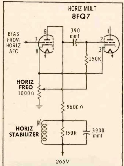
All the new chassis afford a novel and interesting method of varying horizontal-multivibrator frequency. As shown in the schematic, the common cathode resistor is a potentiometer, and the ground return for the second section of the multivibrator is completed through the arm of this control—providing adjustable bias and feedback.
