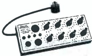
Five- and seven-pin nuvisitors, novars, compactrons, and 10-pin miniature tubes can be tested on any manually-operated tube tester that has an octal socket, when it is equipped with Hickok's CA-4 universal adapter. Each of 14 possible pin locations is controlled by eight individual selector switches, thereby providing facilities for testing future tube types.
