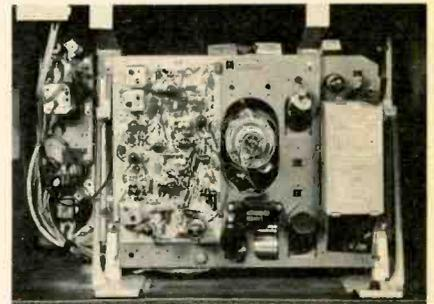
The chassis has one large printed board, marked with "road map" lines on the component side, and with *See-Matic* component symbols on the wiring side. In 19" models, the chassis can be pivoted back (after several screws are removed) and operated in a horizontal position.
