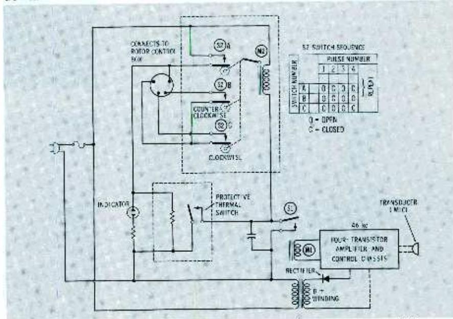
Fig. 4. Remote-control circuits used to start and stop antenna rotation.
