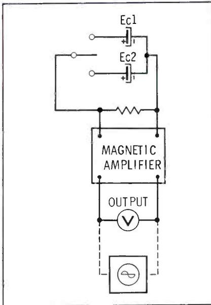
Fig. 3. Long time-constants are measured with a stop watch and indicator. in output brought about by a change in control current.
