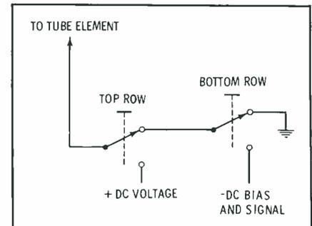
Fig. 10. Unique push-button arrangement provides DC to tube elements.
