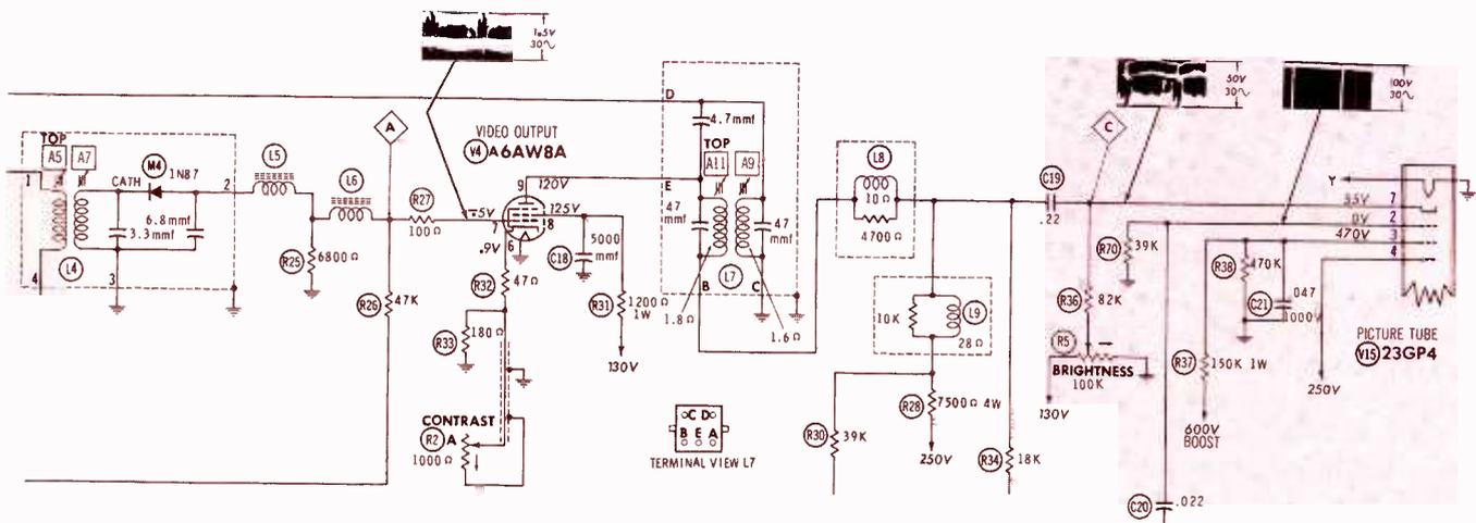
Fig. 2. Most TV receivers obtain adequate picture-signal gain from a one-stage video amplifier.
