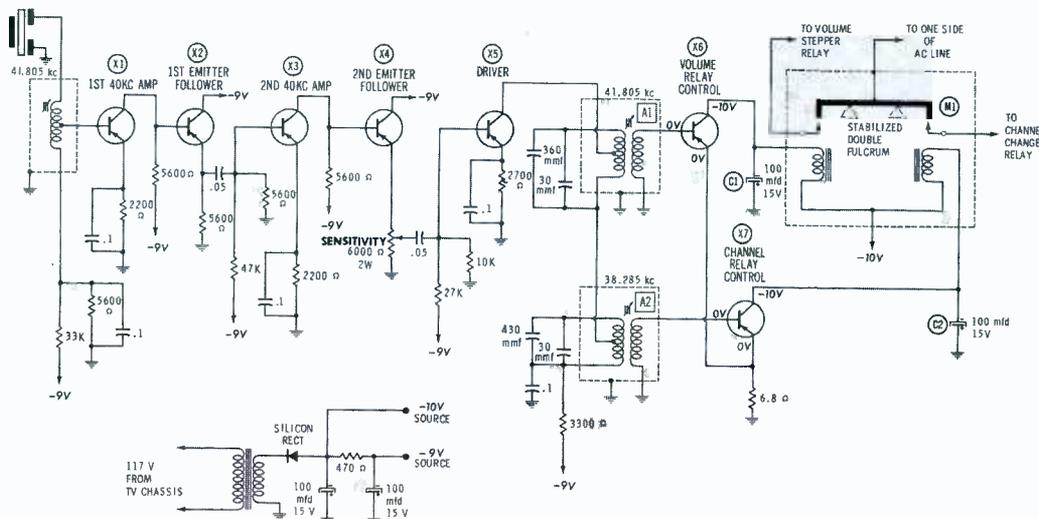
Fig. 2. Received signal is amplified to high enough level to drive relay-control transistors into conduction.
