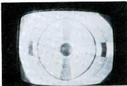
Fig. 5. Nearly open coupling capacitor causes this type of picture smearing.
