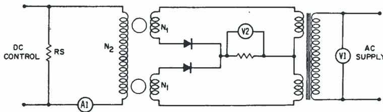
Fig. 1. Test arrangement for obtaining amplifier control characteristics.
