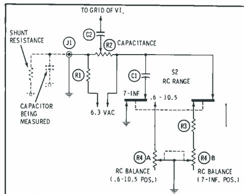
**Fig. 8. When bridge circuit is balanced, capacitance is shown on the dial.**
