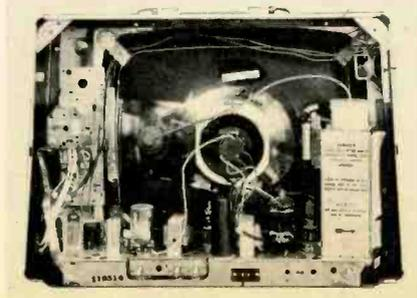
The deluxe "N" series continues to be used in high-end 23" models, retaining such features as a power transformer, 110° picture tube, keyed AGC, and 6DS4 *navistor* RF amplifier.
