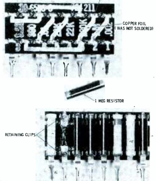
Fig. 2. Special printed component board used in noise-limiter and sync stage.
