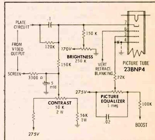
13N51 chassis series, which has several features in common with the 12N53 and -4 at the top end of the '62 line—for example, a 6HZ8 *Intensi-Tube* video amplifier, and horizontal retrace blanking.
