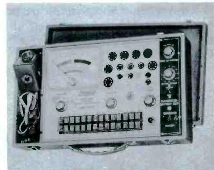
Fig. 9. Tubes and transistors both can be tested on the Mercury Model 1200.
