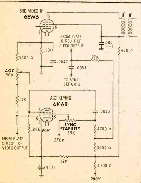
ITY control. Returning the grid of the AGC tube to ground through the cathode circuit of the third IF also contributes to noise cancellation.
