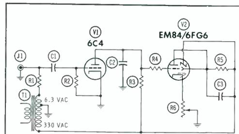
Fig. 5. Shorted capacitor across J1 removes cutoff voltage from grid of V1.
