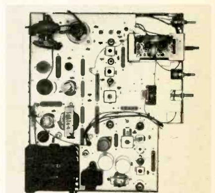
here is more nearly square in shape, and is mounted vertically on one side of the cabinet.
