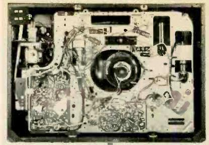
in this category use the "swing-out" style of vertical chassis shown in the photo, with tubes facing the CRT. The complement of 450-ma series-string tubes is the same as in last year's .51780 chassis, except that the new *shadow grid* tuner (equipped with a 3FS5 and a 6FG7) has been adopted in some models.
