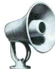
**SPECIFICATIONS:** Frequency Response 400-13,000 cps, Sound Pressure Level 119 db (at 4' on axis, 7.5 watts Input, 2-4 kc), Power Handling Capacity 7.5 watts, Impedance 8 ohms, Dispersion 120°, Size 6 3/4" diameter x 6" deep, Weight 2 lbs.
