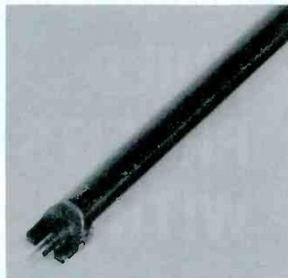
Fig. 4. Retrieving tool has pivoting blade section which grips slug tightly.
