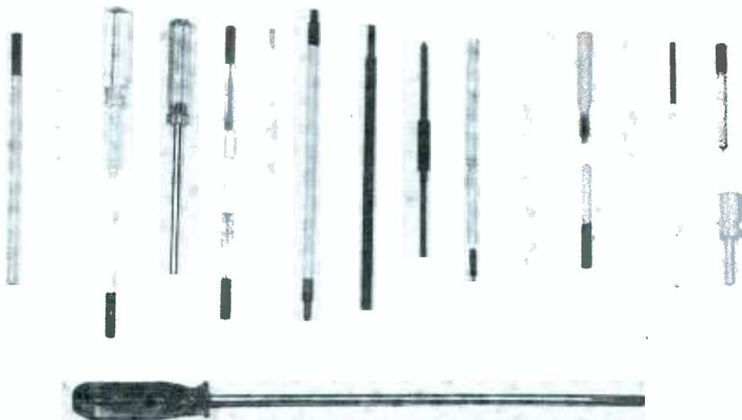
Fig. 2. Radio-TV service shops have uses for all these alignment tools.
