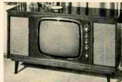
19" compact sets using Chassis 19M1, -2, -3; five 23" consoles equipped with Chassis 23M1, -2, -7; and two stereo combinations (including the "Saguenay" model shown) using Chassis 23M4, -6. Another 23" console series uses Chassis 23L1, -2, -3, and the "Corona" (a 19" compact) has Chassis 19L1. The "Instant Reflex" chassis used in 23" sets is a hand-wired horizontal type with a bonded 110° CRT attached.
