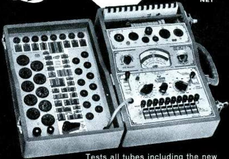
Tests all tubes including the new Nu-Vistors, Novars, Compactrons and 10-pin types.
