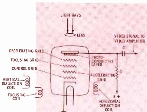
Fig. 1. Vidicon tube is very similar in general construction to ordinary CRT.
