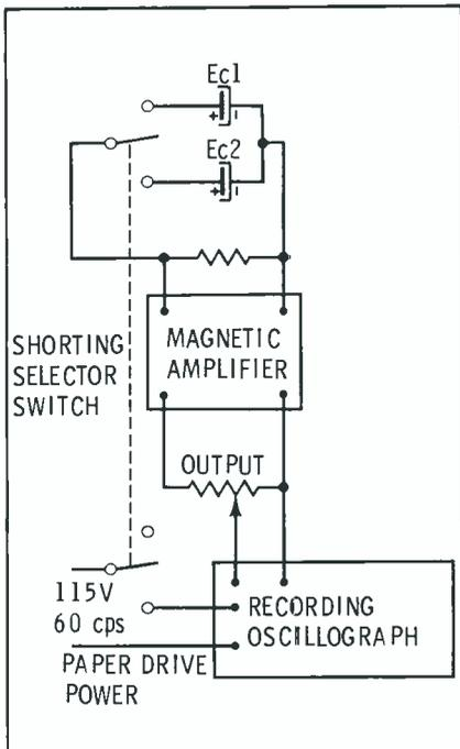
Fig. 4. A recording oscillograph is used to obtain an accurate measurement.
