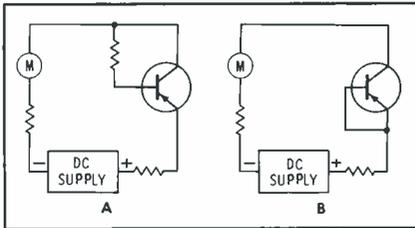
Fig. 11. Gain and leakage tests are performed by these simplified circuits.
