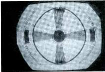
Fig. 7. Replacement of peaking coil with wrong value may cause ringing.
