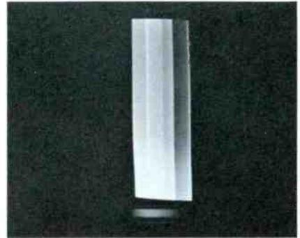
Fig. 4. Extreme loss of width caused by drastic rise in oscillator frequency.
