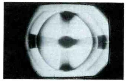
Fig. 6. Smear and loss of high frequencies, due to a defective peaking coil.
