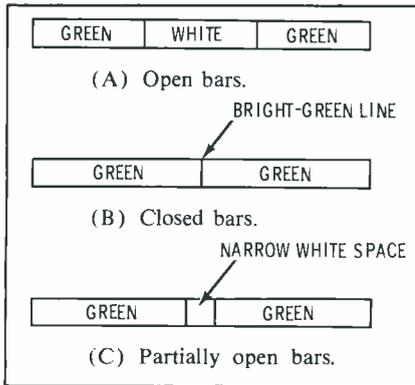
**Fig. 6. Indicator-tube bar patterns.** at J1. The test cable, together with L2, R1, and C3, is approximately one-quarter wavelength at 19 mc (the frequency of
