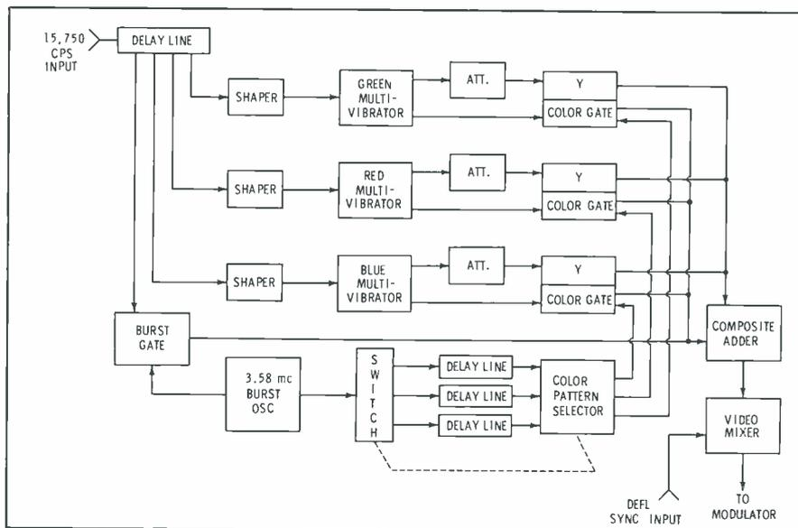
Fig. 3. Functional block diagram shows how the chroma signal is developed.
