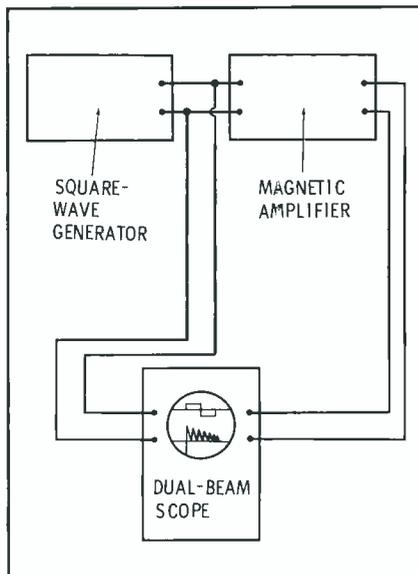
Fig. 5. This method uses a dual-beam scope and a square-wave generator.
