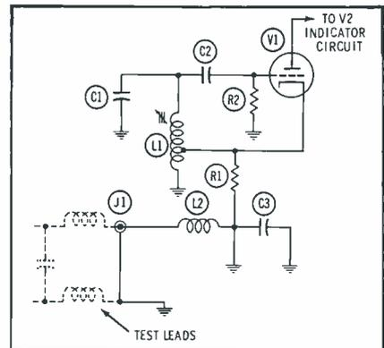
**Fig. 7. An open circuit across the test leads causes V1 to stop oscillating.**
