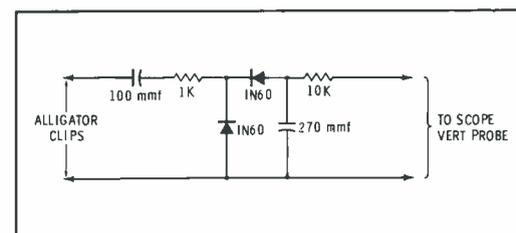
Fig. 5. Simple demodulator probe unit.
