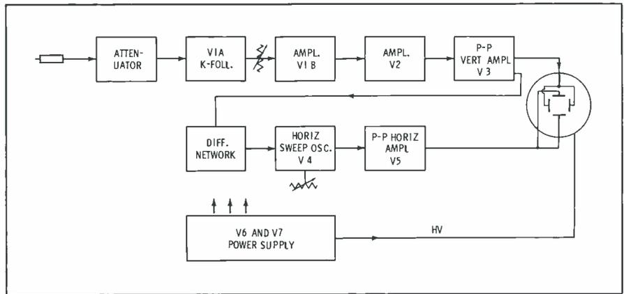
Fig. 4. Block diagram of PS120 scope.
