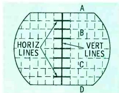
Fig. 3. Check for vertical dynamic convergence in this area of crosshatch.
