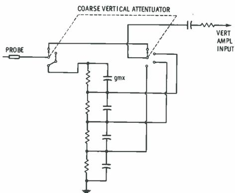
Fig. 3. Schematic showing compensation networks of vertical attenuator.
