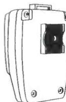
humidity, they will operate even if immersed in water. The ceramic transducer is neoprene encased, rendering it shock and impact-proof.
