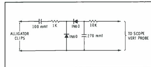
Fig. 5. Simple demodulator probe unit.
