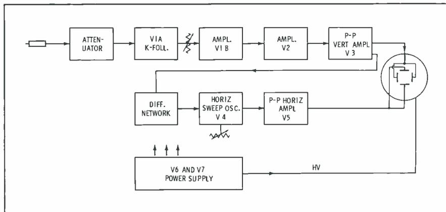
Fig. 4. Block diagram of PS120 scope.
