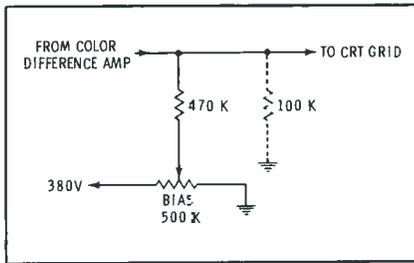
Fig. 1. 100K resistor disables CRT gun.
