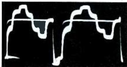
scale tracking adjustments; therefore, it is not usually necessary to analyze the cathode-signal waveforms in great detail. On the other hand, close attention to both the amplitude and the waveshape of the grid signals will often provide the key to locating trouble in the related circuits (Fig. 1).
