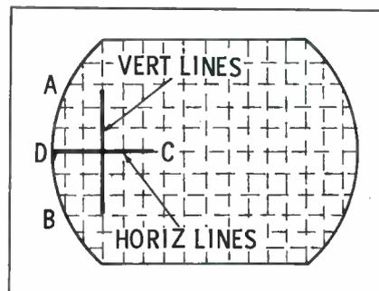
Fig. 6. Follow this pattern to adjust horizontal convergence at left side.
