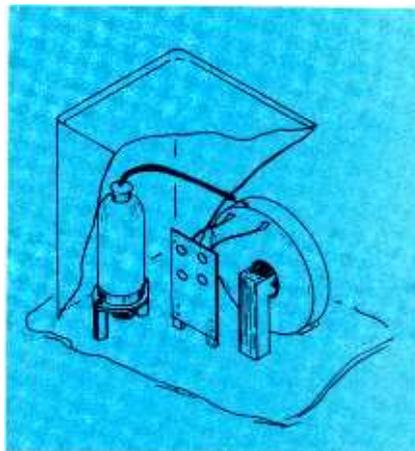
Fig. 1. Most common mounting for high-voltage sockets in older TV receivers.
