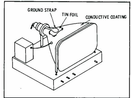
Fig. 3. Tin foil "patch" makes substitute for missing aquadag CRT coating.
