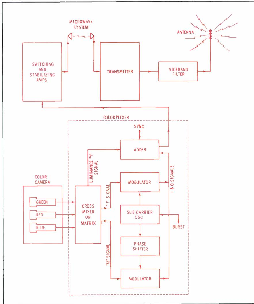
Simplified block diagram shows relationships between components and signals.
