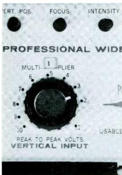
Fig. 2. Closeup of vertical attenuator showing multiplier reading in window.
