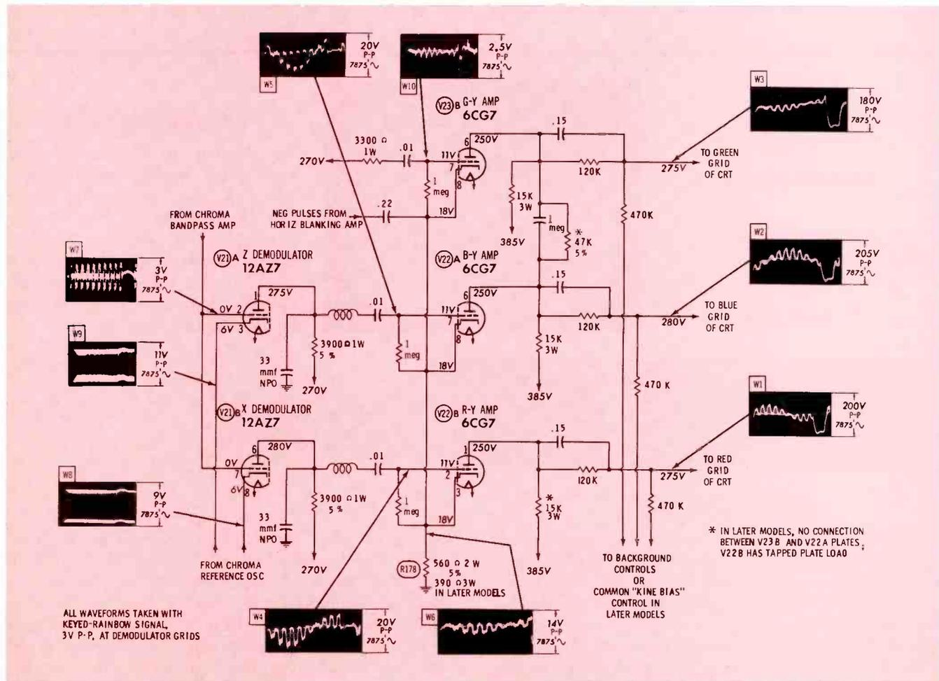
Fig. 1. Chroma demodulators and color-difference amplifiers of typical color TV (RCA Chassis CTC9).
