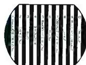
Generates full color rainbow display and color bar pattern to test color sync circuits, check range of hue control, align color demodulators. Demonstrates to customers correct color values.
