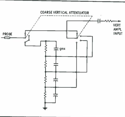
Fig. 3. Schematic showing compensation networks of vertical attenuator.
