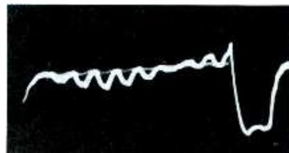
Fig. 3. Keyed rainbow with red, blue, and green grid inputs (W1, W2, W3).
