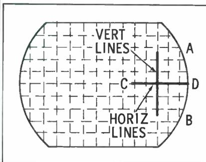
Fig. 5. Check convergence of both vertical and horizontal bars at right side.
