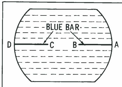
**Fig. 4. Straightening the blue bar is first step of horizontal convergence.**
