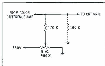
Fig. 1. 100K resistor disables CRT gun.
