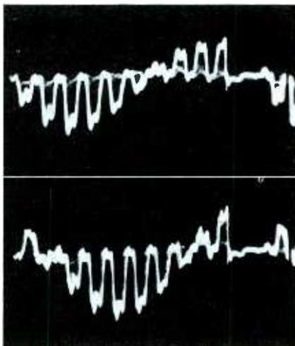
Fig. 4. Waveforms W4 and W5 applied to grids of R-Y and B-Y amplifiers.
