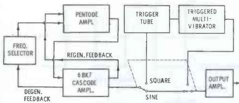
Fig. 5. Unusual method of frequency control is shown in block diagram.
