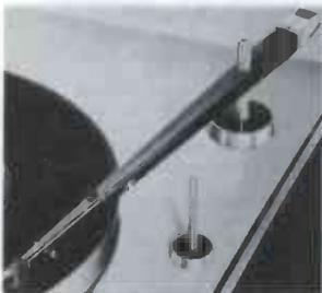
The Model M222 tone arm, which uses an N22D tubular stylus with a .0005" diamond point, is new from Shure. It has a tracking pressure of less than 1½ grams, frequency response from 20 cps to 20·kc, channel separation of more than 22.5 db at 1000 cps, and output voltage of 4.5 mv. Audiophile net price of the M222, including the N22D stylus, is
