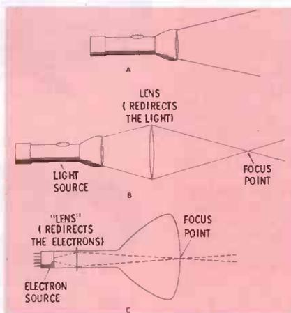
Fig. 1. Comparison between focusing of a flashlight beam and electron beam.
