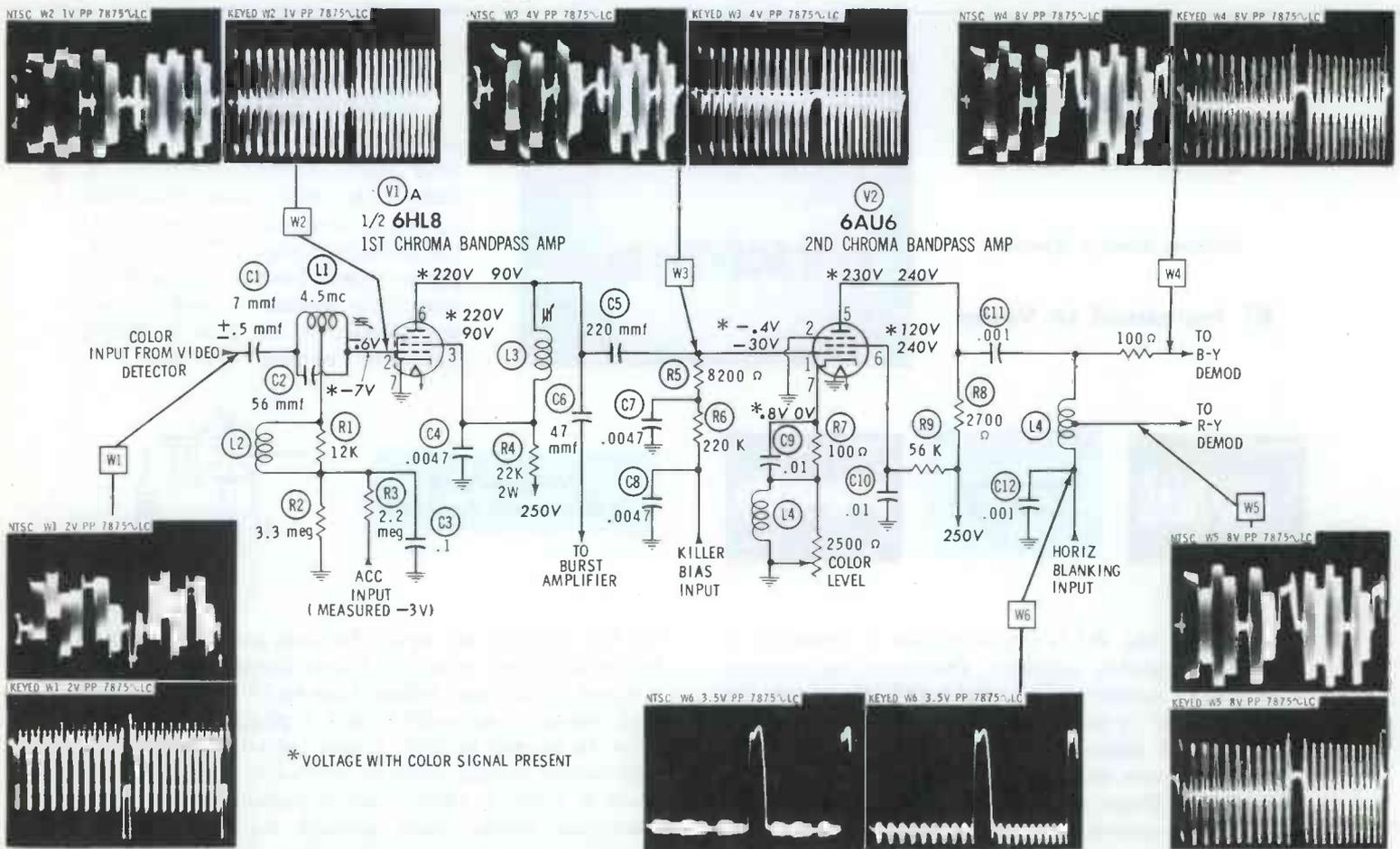
Fig. 1. Two-stage bandpass amplifier in Zenith Chassis 27KC20 receives input from video detector.
