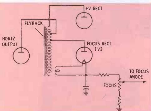
Fig. 2. Older circuit seldom used in monochrome sets, popular in color TV's.
