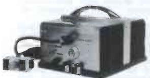
A transistorized converter, developed by Terado, changes 12 volts DC into 110 volts AC, and has a maximum continuous output capacity of 550 watts. This power capability makes it possible to use the unit in a "rolling service shop" to power test equipment, lights, a soldering gun, and the television set
