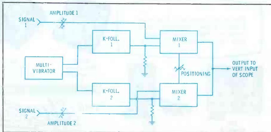
Fig. 2. Block diagram shows circuits that combine signals and switching.
