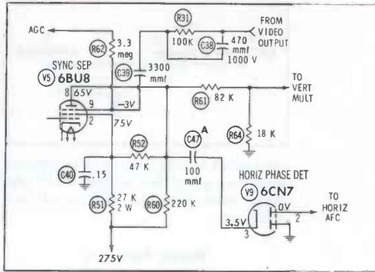
only waveform trouble is at the screen of the 6BU8; the scope trace looks fuzzy instead of having the shape shown on PHOTOFACT. Both horizontal and vertical hold are critical. Can you help?
