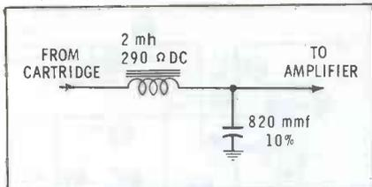
noise which usually consists of frequencies above this point. For sharper cutoff and greater attenuation, you can cascade two such circuits.
