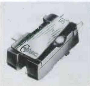
A series of ceramic replacement stereo cartridges, having a dual stylus for playing either stereo or monaural records, is now available. Made by **Euphonia**, the U-8 and U-9 feature a tracking force of 2 grams and high compliance. The U-8, with the sapphire dual stylus, carries a list price of \$9.95. The U-9, with a .0007" diamond and .003" sapphire stylus, lists for \$14.95.
