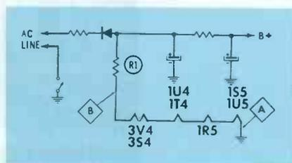
Fig. 1. Filament troubles are usual cause of fading in three-way portables.
