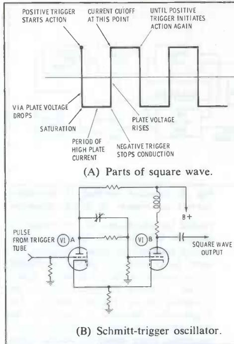
Fig. 6. Square-wave section of G-34.
