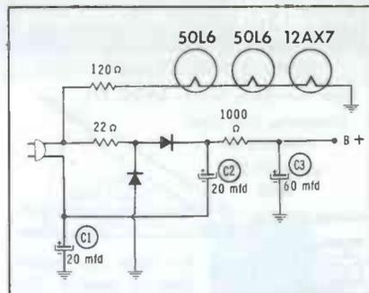
Fig. 5. "Different" method of obtaining DC voltage for hum-free operation.
