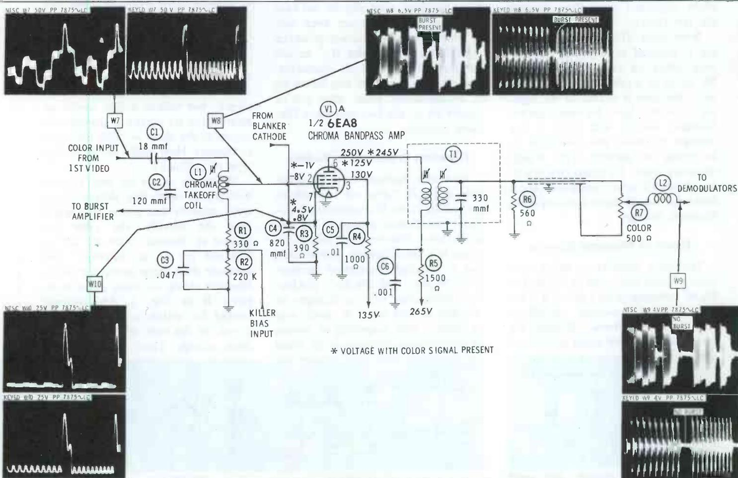
Fig. 2. In RCA Chassis CTC12, chroma signal passes through first video amplifier and one bandpass stage.
