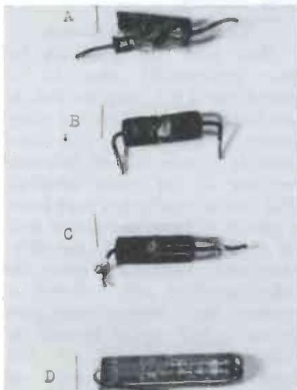
Fig. 8. Damage to filament chokes is usually spotted by visual inspection.
