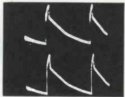
(A) Sawtooth modulating voltage.
