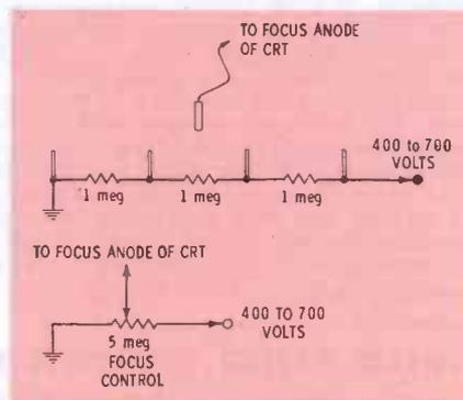
Fig. 3. Most modern receivers use one of these circuits for focusing the CRT.
