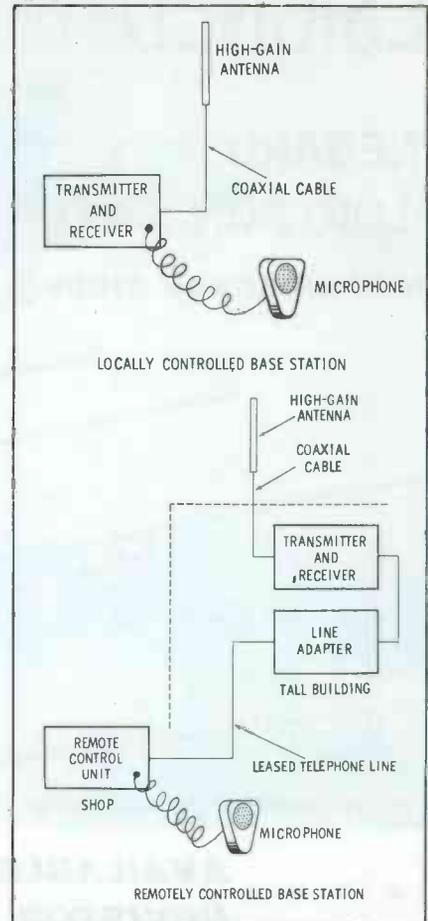
Fig. 3. Two ways in which two-way systems can be installed for best use.
