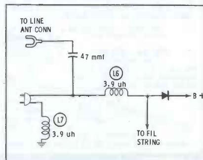
Fig. 6. Filament chokes in FM sets are usually at ends of series string.
