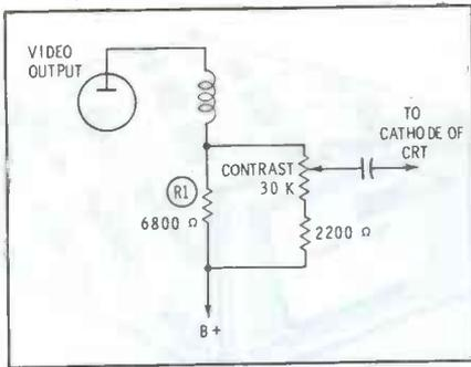
Fig. 4. Circuit with high-level contrast control causes unusual symptom.
