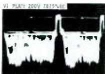
W1 is definitely weak: only 70 volts at maximum contrast. Obvious distortion is present, especially at 7875 cps — note exaggerated horizontal sync and compressed video. Normal signal is present at plate of video output tube, so signal loss must be occurring in CRT coupling circuit. Signal tracing reveals distortion on CRT side of C3-R5; C3 is suspect because it should pass signal without noticeable change in size or shape.
