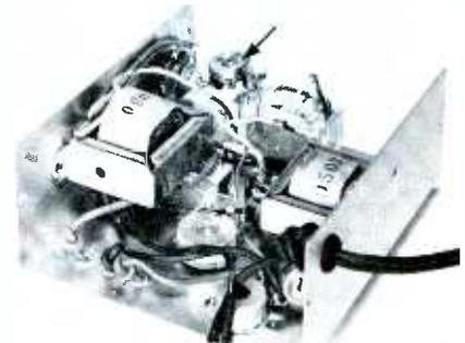
Fig. 3. Screwdriver control sets meter.
