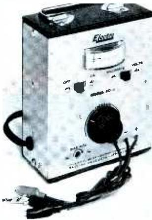
Fig. 1. Adjustable bias tap is special feature of this transistor power supply.
