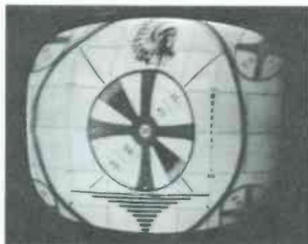
Visual indications are approximately same as in Symptom 2—picture pulls away from right edge of screen and may show phasing ghost at left. Attempt at correction makes sync less stable. Horizontal bending of picture varies with program material.
