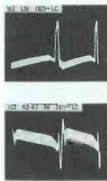
To avoid confusion in analyzing waveforms, picture should be made as stable as possible by keeping signal strength low and critically adjusting L1. W2 (shown), W1, and W3 look reasonably normal, but spurious 5 volt waveform is found at junction R2-R3, where less than 0.5 volt ripple should appear. Grid of V2 is free from ripple, indicating normal C6 and bad C5.
