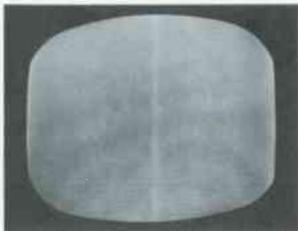
Trouble looks like blocked IF due to loss of AGC. Disconnecting antenna or switching to weak station brings in picture, but horizontal sync is very unstable. Grounding grid of V2 restores normal sweep and lets keyed AGC circuit operate properly, restoring video.
