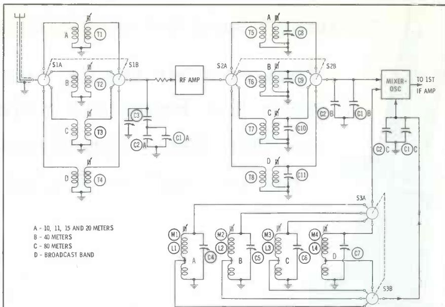
Fig. 3. Alignment points in typical four-band RF, and oscillator circuits.
