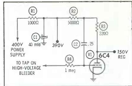
Fig. 3. Power supply includes 6C4 for voltage regulation of 150 volt line.
