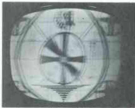
Multivibrator reacts normally to grid-grounding test. When ground lead is removed, AFC throws multivibrator off frequency. Sync can be restored by backing out L1 slug, but is extremely critical—picture soon begins to jitter, and falls out of sync.
