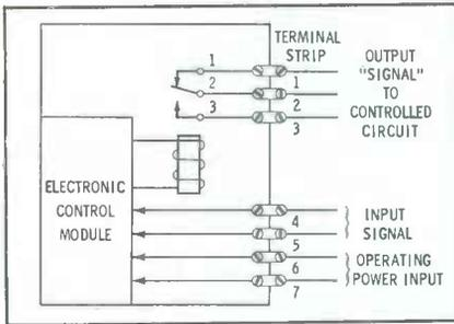
Fig. 8. Terminal strip simplifies the troubleshooting of this control device.
