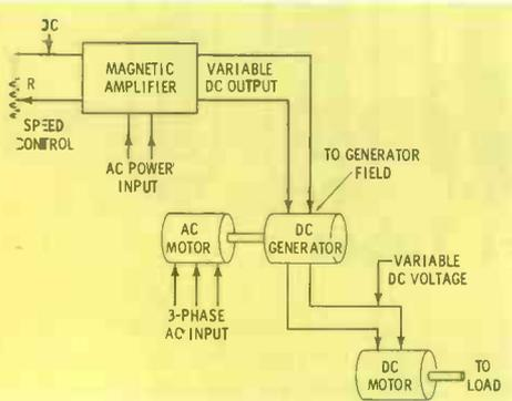
Fig. 3. An open-loop control system.
