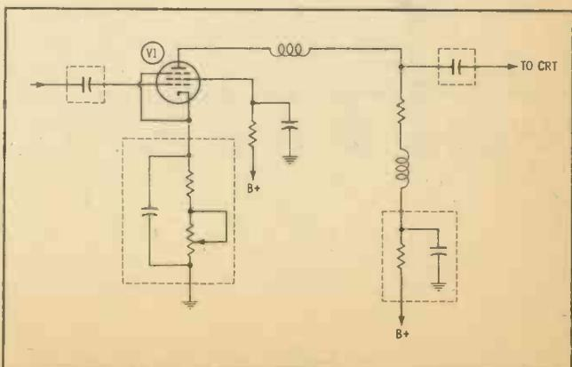
Fig. 3. Components that affect low-frequency response.
