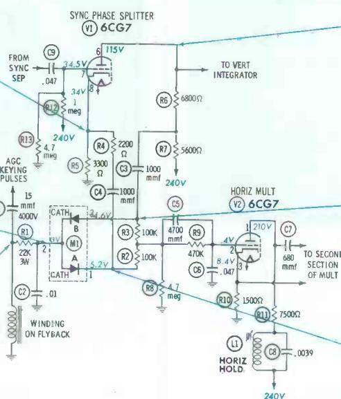
DC VOLTAGES taken with VTVM, on inactive channel; L1 adjusted for zero volts on grid of V2.
