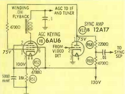
**Fig. 1.** Input to AGC tube in Westinghouse V-2313 is from a sync amplifier.
