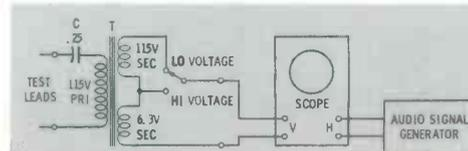
Fig. 5. This hookup results in a Lissajous figure for comparing frequencies.
