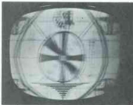
Multivibrator reacts normally to grid-grounding test. When ground lead is removed, AFC throws multivibrator off frequency. Sync can be restored by backing out L1 slug, but is extremely critical—picture soon begins to jitter, and falls out of sync.
