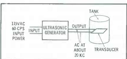
Fig. 9. Ultrasonic cleaning system is also common in watch-repair shops.
