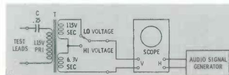
Fig. 5. This hookup results in a Lissajous figure for comparing frequencies.
