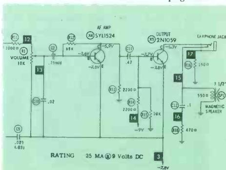
**Fig. 3.** This type of single-ended NPN driver and output circuit is widely used
