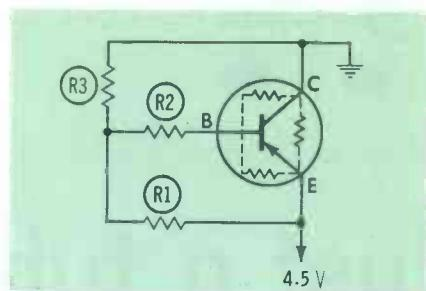
**Fig. 2.** Since a transistor is solid-state, it has resistance between electrodes.
