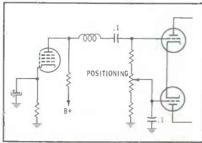
Fig. 2. Control in grid circuit of push-pull output adjusts trace positioning.
