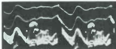
Fig. 9. Much worse distortion was apparent in video output plate waveform.
