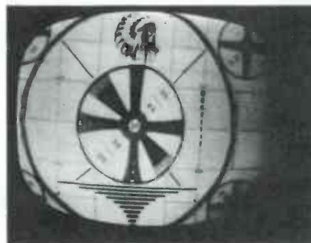
Picture locks in solidly, but L1 needs readjusting when set is turned on, and again after thorough warm-up. Tipoff to phasing fault is visible black border at right of screen, and milky phasing ghost at left. Attempt to correct it throws picture out of sync.
