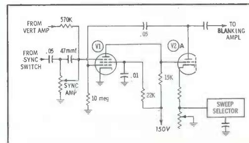
Fig. 4. Sync is injected into sweep multivibrator via suppressor of V1.
