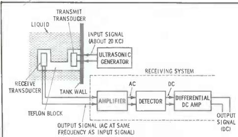
Fig. 10. Liquid-level detection system utilizes ultrasonics in special unit.
