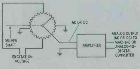
**Fig. 1. Shaft-position indicator produces AC or DC analog output signals.**
