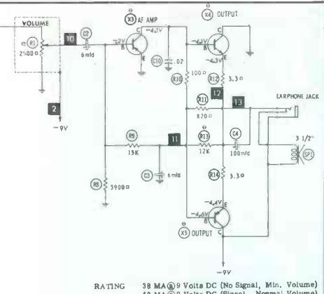
**Fig. 4. Common-collector outputs use this hookup to obtain operating bias.**ances extending from the 9-volt source to ground (X4 collector). Likewise, X4 and X5 base voltages are the result of divider action. (Notice that the collector of X3 and the base of X4 are DC coupled. This is possible because X3 is a PNP and X4 is an NPN.)
