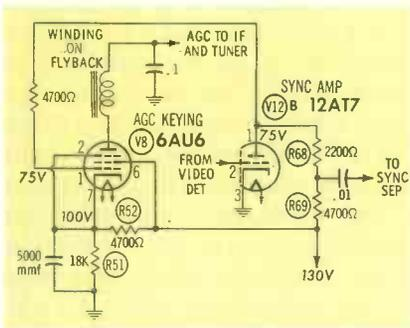
Fig. 1. Input to AGC tube in Westinghouse V-2313 is from a sync amplifier.
