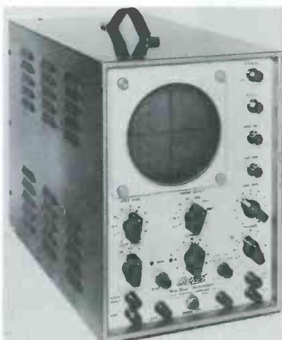
Fig. 1. Wideband scope includes frequency compensated vertical amplifier.
