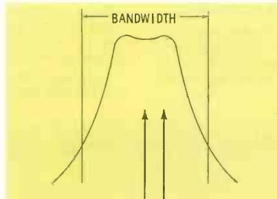
Fig. 2. Misalignment will widen bandwidth and ruin receiver selectivity.
