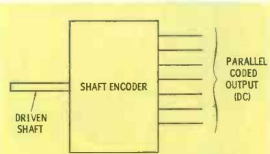
Fig. 2. Encoder unit develops digital information without analog converter.
