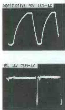
Reduced width is explained by weak, distorted drive signal at grid of horizontal output (should be 150 volts). AFC waveforms are not clear enough to be analyzed, until set operation is stabilized by connecting multivibrator grid to ground. Then W2 is nearly normal, but W1 is not—it has same shape as W4. Lack of sawtooth means M1A is not conducting. W3 is okay.
