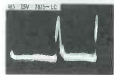
These waveforms were taken with contrast control at high setting, to aid in locating cause of horizontal twist. As anticipated, W1 is full of video. It's also somewhat stronger than normal, whereas W2 is weak; this unbalance explains phasing error. W5 is weak, and pulses in it fluctuate so much the waveform is hard to lock in. W4 (26 volts) contains much video. Something's wrong in circuit of V1, drastically upsetting its operation.
