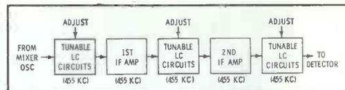
Fig. 4. Two IF tubes mean three adjustment points; three would indicate four.
