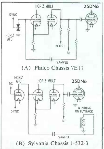
Fig. 12. Twist was caused by bad 25DN6 in circuit A, but not in circuit B.
