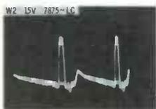
W3 is normal; this proves trouble is not due to reversed connections on flyback winding. Both W1 and W2 contain satisfactory sync pulses, but lack of sawtooth component in W1 and unusually strong sawtooth in W2 point to erratic operation of AFC. Wrong positioning of sync pulse on sawtooth portion of W2 is simply a consequence of phase error in horizontal sweep signal.
