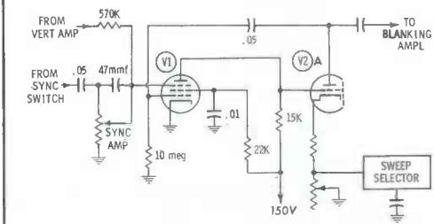
Fig. 4. Sync is injected into sweep multivibrator via suppressor of V1.
