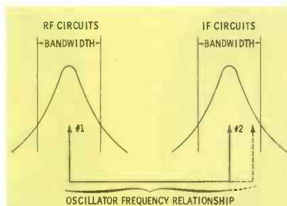
Fig. 1. Tracking is accurate only when oscillator-RF relationship is constant.
