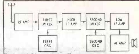
Fig. 5. Dual-conversion receiver is often called a double-superheterodyne.
