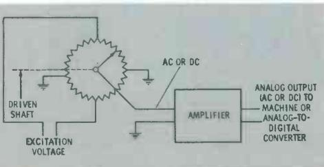
Fig. 1. Shaft-position indicator produces AC or DC analog output signals.
