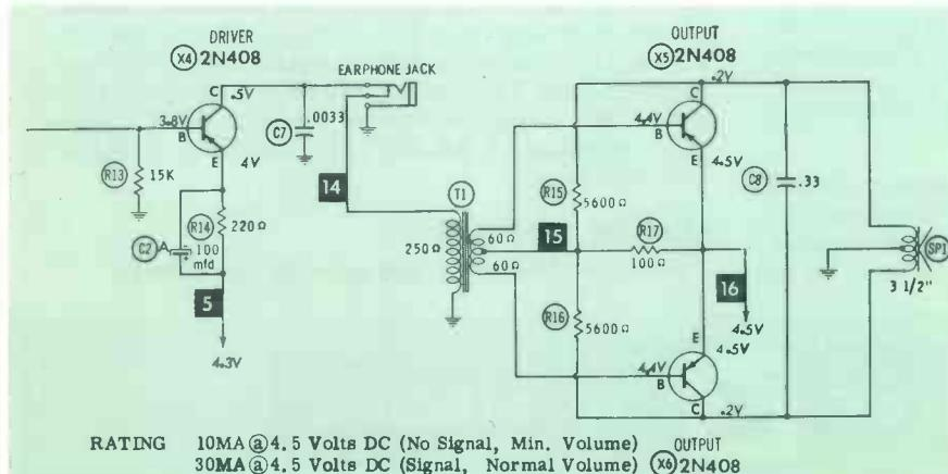
Fig. 1. PNP driver and output stages operating in the common-emitter mode.
