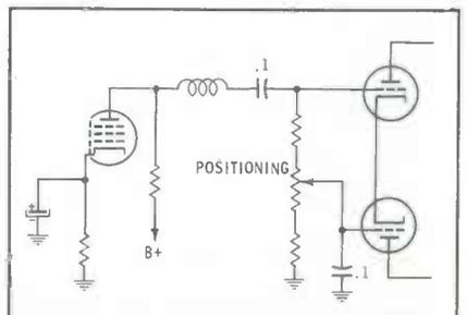
Fig. 2. Control in grid circuit of push-pull output adjusts trace positioning.
