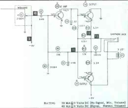
RATING 38 MA @ 9 Volts DC (No Signal, Min. Volume)
