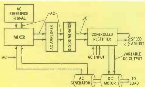
Fig. 4. A closed-loop control system.
