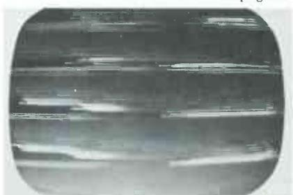
Fig. 7. Unusual form of horizontal squegging due to odd tube defects.
