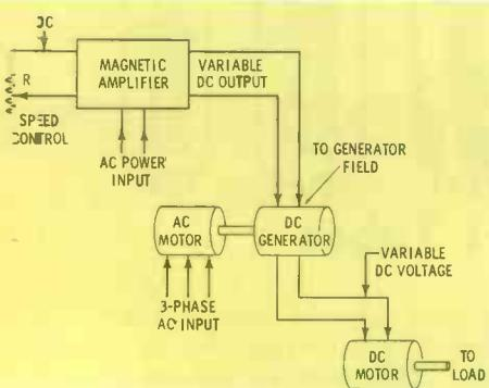
Fig. 3. An open-loop control system.
