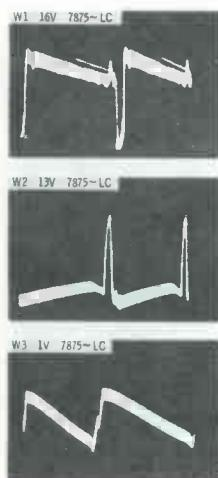
On weak station signals, picture can be held in sync long enough to view waveforms. W1 and W2 look almost the same as in Symptom 4, and display no definite evidence of trouble. Main clue is W3, which has approximately normal shape, but amplitude of only 1 volt. Considerable "hash" in W3 indicates high impedance from lead 2 of M1 to ground; thus, increased value of R1 is more likely cause of signal loss than shorted C2.
