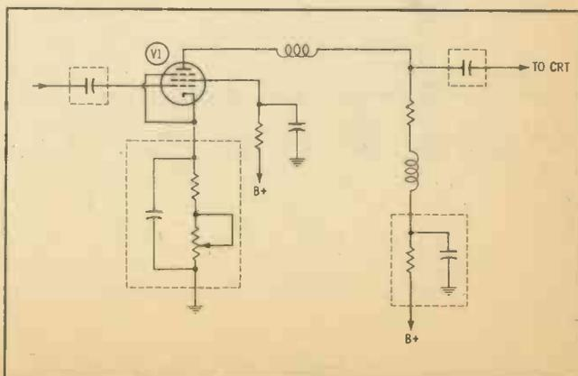
Fig. 3. Components that affect low-frequency response.
