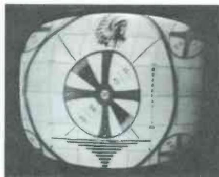
Visual indications are approximately same as in Symptom 2—picture pulls away from right edge of screen and may show phasing ghost at left. Attempt at correction makes sync less stable. Horizontal bending of picture varies with program material.
