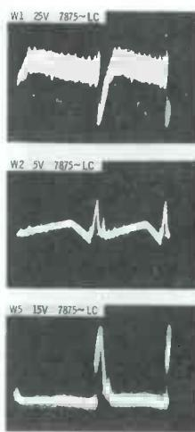
These waveforms were taken with contrast control at high setting, to aid in locating cause of horizontal twist. As anticipated, W1 is full of video. It's also somewhat stronger than normal, whereas W2 is weak; this unbalance explains phasing error. W5 is weak, and pulses in it fluctuate so much the waveform is hard to lock in. W4 (26 volts) contains much video. Something's wrong in circuit of V1, drastically upsetting its operation.
