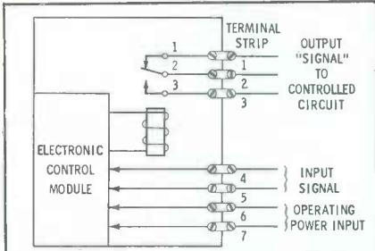
Fig. 8. Terminal strip simplifies the troubleshooting of this control device.
