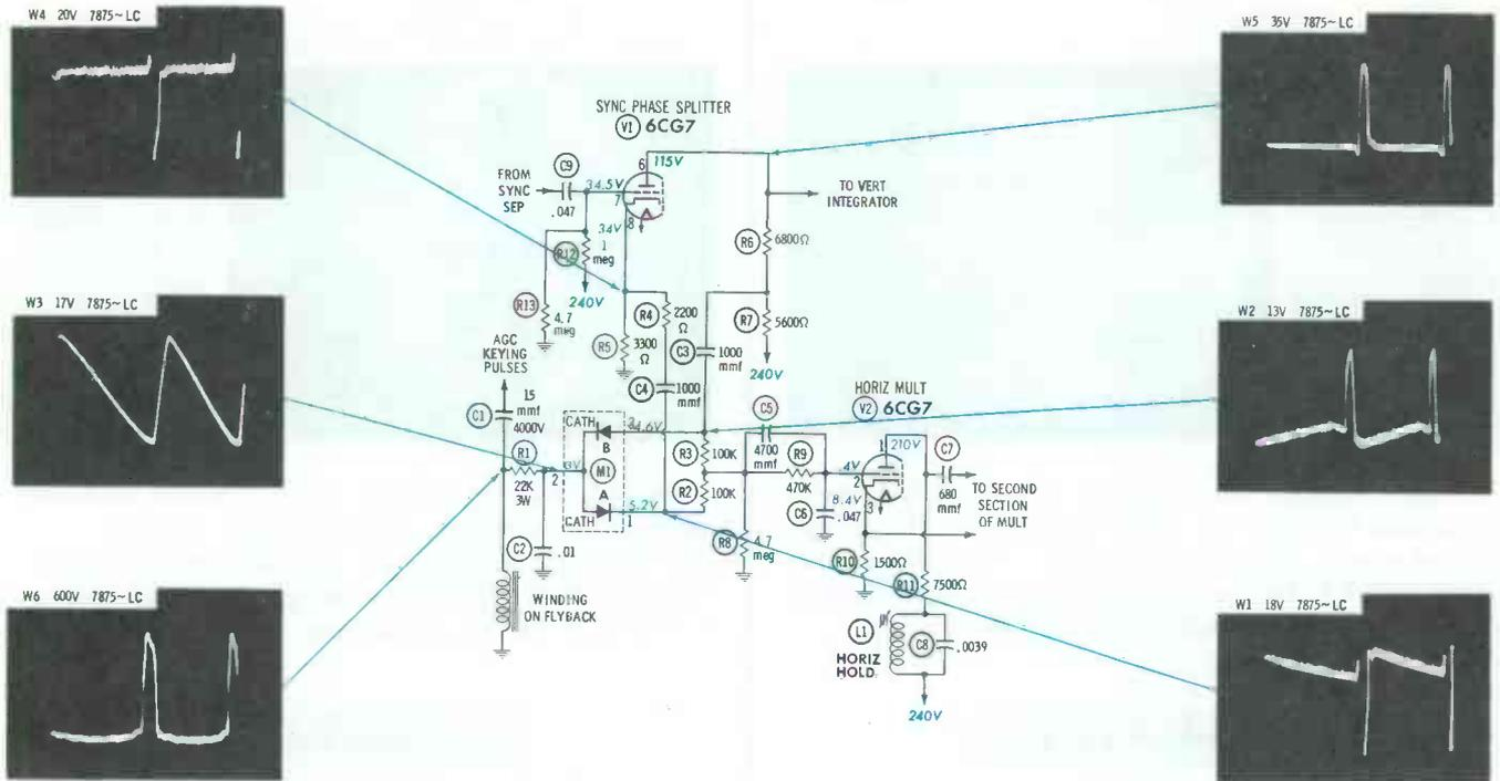
DC VOLTAGES taken with VTVM, on inactive channel; L1 adjusted for zero volts on grid of V2.
