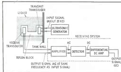
Fig. 10. Liquid-level detection system utilizes ultrasonics in special unit.
