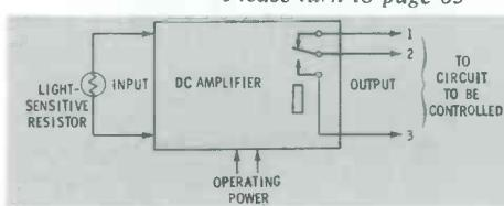
Fig. 7. Simple modular control circuit.
