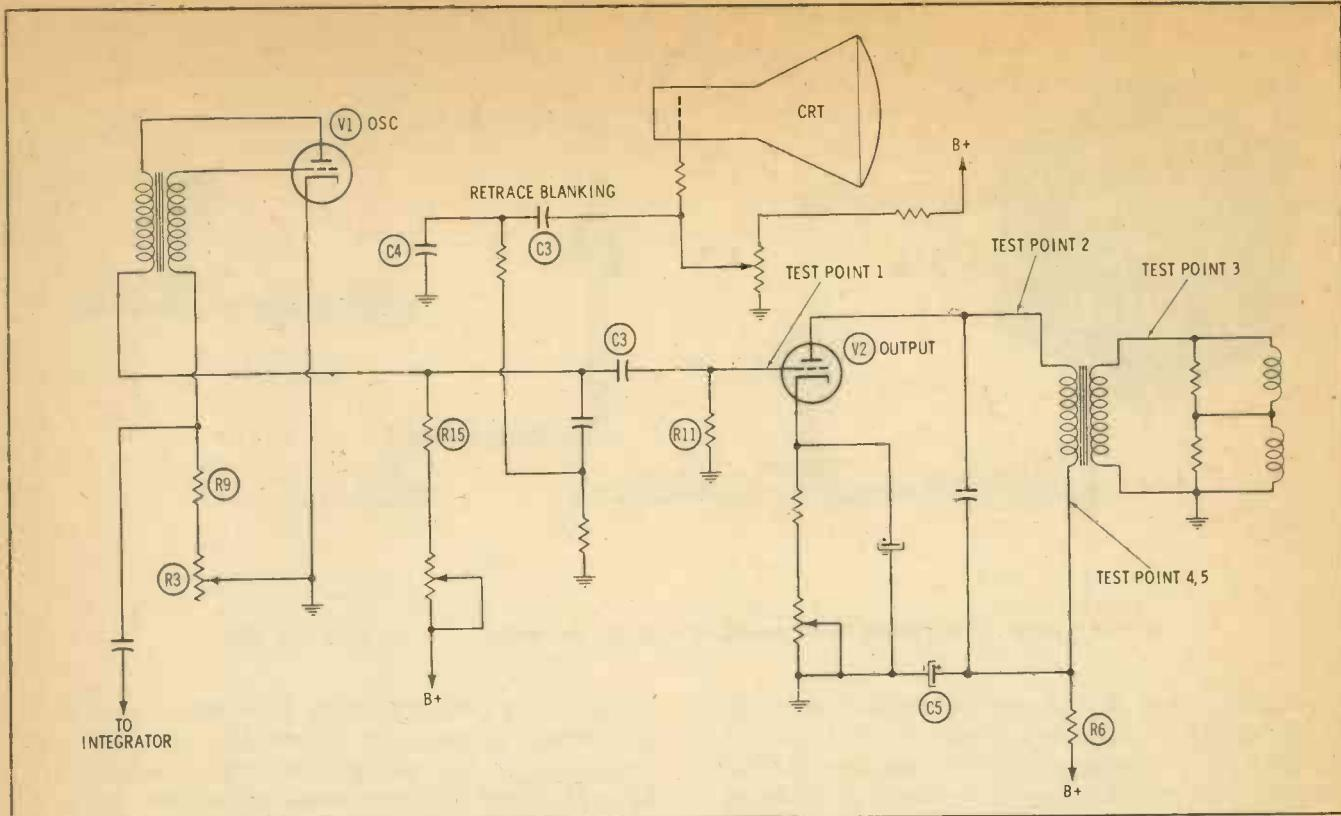
Fig. 1. Common blocking oscillator circuit used in a number of older receivers.
