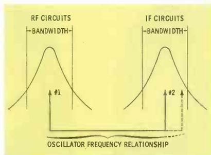
Fig. 1. Tracking is accurate only when oscillator-RF relationship is constant.
