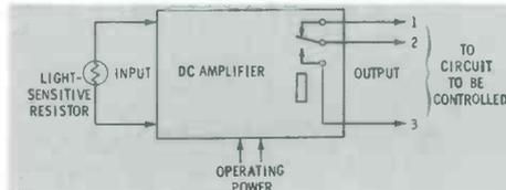
Fig. 7. Simple modular control circuit.
