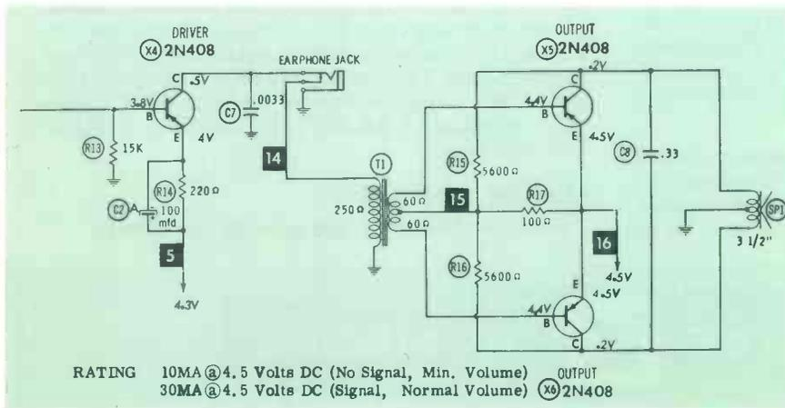
Fig. 1. PNP driver and output stages operating in the common-emitter mode.
