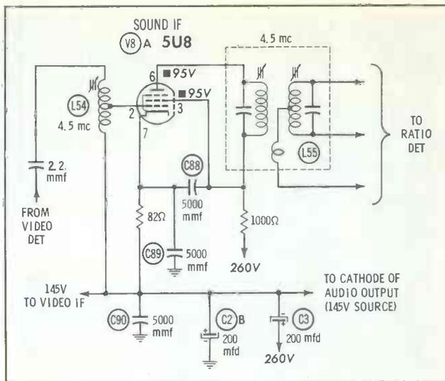
coupled into the sound circuits through faulty lead dress, or by leakage in the socket of V8 from the triode section (sync phase inverter) to the pentode section (sound IF).
