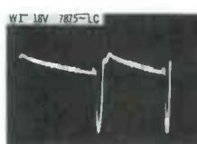
Normal amplitude of sync pulses in W1 and W2 isolates fault to AFC. W2, taken at point of most stable sync, shows pulse shifted to right of usual position on sawtooth. L1 can be adjusted to place pulse in W1 on negative peak of sawtooth, without losing sync; this point is beyond normal hold-in range. Waveforms call attention to phasing error, but do not pinpoint its cause.
