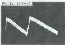
On weak station signals, picture can be held in sync long enough to view waveforms. W1 and W2 look almost the same as in Symptom 4, and display no definite evidence of trouble. Main clue is W3, which has approximately normal shape, but amplitude of only 1 volt. Considerable "hash" in W3 indicates high impedance from lead 2 of M1 to ground; thus, increased value of R1 is more likely cause of signal loss than shorted C2.
