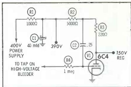
Fig. 3. Power supply includes 6C4 for voltage regulation of 150 volt line.
