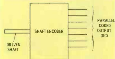
**Fig. 2. Encoder unit develops digital information without analog converter.**
