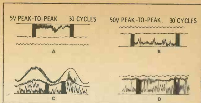
Fig. 2. Plate and grid waveforms of video output stages.
