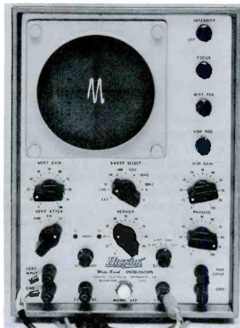
Another type of scope has a 1-volt peak to peak calibration terminal on the front panel. The vertical test lead, or a jumper, will apply the signal from this terminal to the vertical input, and you can adjust the vertical gain to obtain a trace of some arbitrary height—say one inch. Then with the same control settings, any signal corresponding to this same height is equal to 1 volt. The multiplier switch permits measuring larger voltages—as you'll see.
