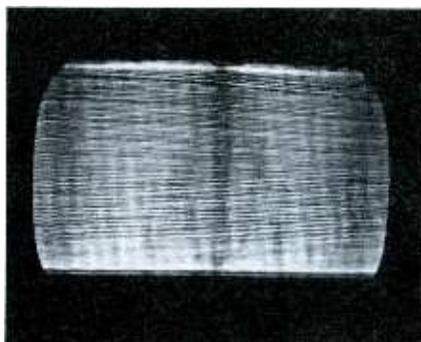
Raster fills one-half to three-fourths of screen, depending on R2 setting. Scanning lines are jittery and few in number. T1 emits faint high-pitched hum (several hundred cps). Hold and linearity controls have small effect. Details of picture are obscured.
