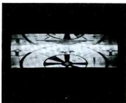
Raster height is one-third of normal, and is unaffected by turning R2. Both R1 and R4 have some effect on height; also, if either R1 or R3 is turned very far from counterclockwise limit, raster breaks into overlapping sections. Picture does not roll.
