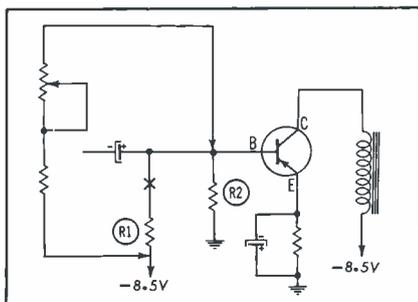
Fig. 4. Tester can substitute variable bias.
