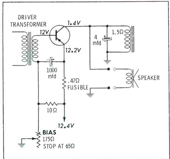
Installation of this radio requires the use of a 10-ohm rear-seat speaker to properly match the output impedance of the audio power transistor. Using a speaker with lower impedance would cause excessive current to be drawn by the output stage, thus burning out the bias control and/or the output transistor. The .47-ohm fusible resistor in the emitter circuit may also open.
