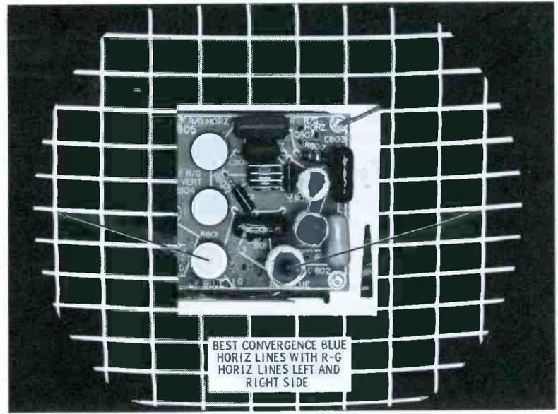
Use the blue horiz lines right (B-1) and blue horiz lines left (B-2) to converge blue horiz lines with red and green at the left and right center area.
