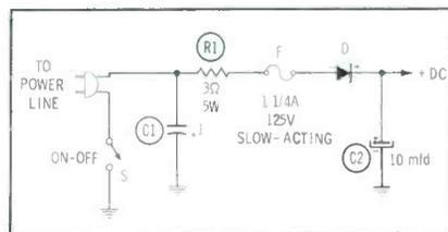
Fig. 3. Peak-limiting resistor in supply filter.
