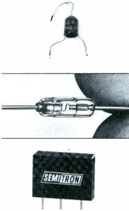
Fig. 4. Selenium diodes used in horizontal AFC circuits come in various shapes, sizes, of a few microamps, and extend to a few hundred milliamps. Peak inverse ratings—the amount of reverse voltage the unit can withstand—seldom exceed 150 volts, except in special units.
