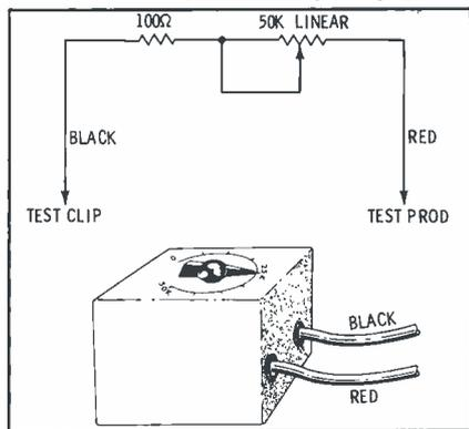
Fig. 3. "Bias-changer" will trace distortion.
