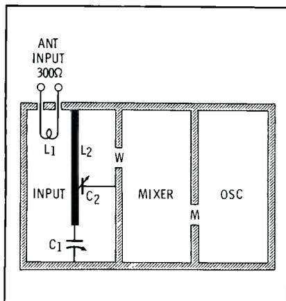
Fig. 4. Case configuration of typical tuner.
