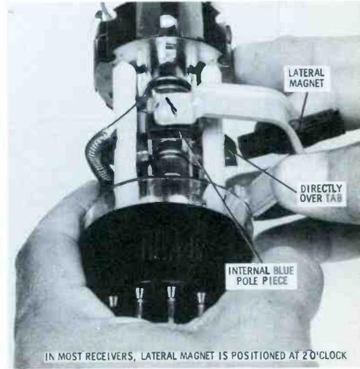
Poor convergence may result from improperly positioned elements; convergence yoke directly over pole pieces  $3\frac{7}{8}$ " from CRT base, purity ring  $\frac{5}{8}$ " rearward, and the lateral magnet over internal pole piece.
