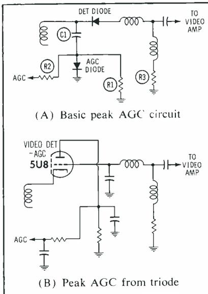
Fig. 10. Circuits in which AGC voltage is determined by peak level of video IF signal.
