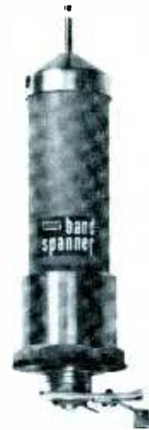
possible VSWR and then locking the barrel in place with a setscrew. Metal parts are chrome-plated solid brass. The transformer coil is moisture-proof, and the trapping of moisture within the antenna base is eliminated by a triple washer arrangement with a drain hole. The suggested list price is \$34.95.
