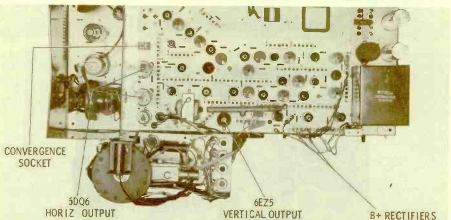
B+ is developed by two silicon rectifiers wired as a voltage doubler and protected by a circuit breaker. The parallel filament circuits are fused with #24 wire, except for the picture tube and high-voltage regulator which operate from a separate winding and are not protected.
