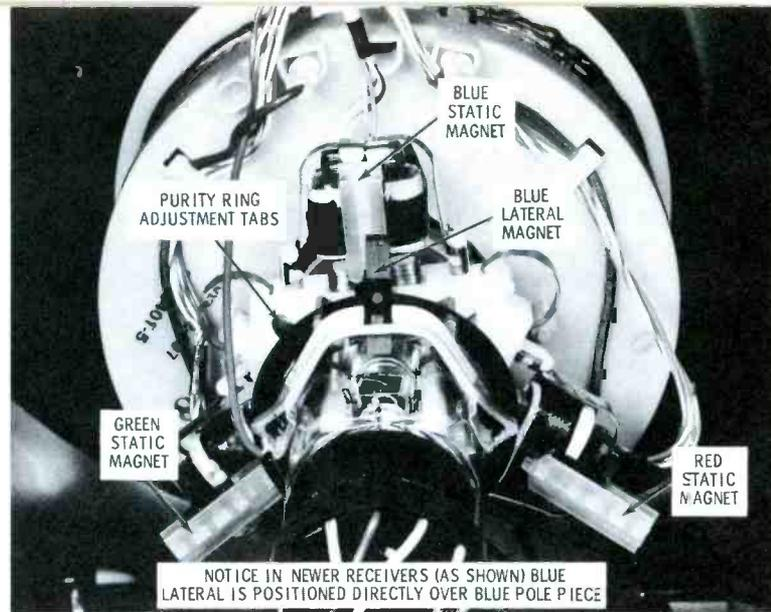
Black and white setup procedures, CRT degaussing, and purity checks should be performed previous to convergence. Use the red, green, and blue magnets and the lateral magnet for center dot convergence.
