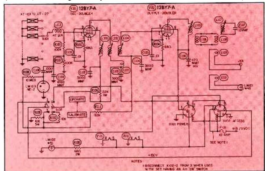
Fig. 3. Schematic of VHF transmitter. Separate modulator and power supply are required.
