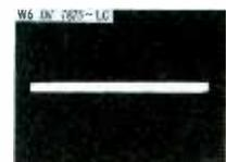
Absence of pulse in W6 hints strongly at trouble in oscillator circuit; eliminates need for further troubleshooting in driver or output stages. W4 offers more evidence of oscillator trouble. Normal p-p signal at this point is 8 volts. Collector-to-base feedback is necessary for oscillation. R17 and interstage winding of T1 can be disregarded. Possible faults are R16, X1 collector bias network, or winding of T1.
