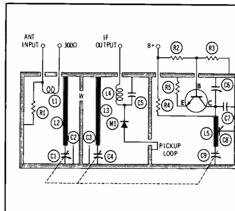
Fig. 5. Schematic of a typical UHF tuner. mixer, and an internally mounted transistor oscillator, the schematic will resemble that shown in Fig. 5. Other types of tuners are essentially similar—enough so that a single explanation should serve for most basic circuit functions.
