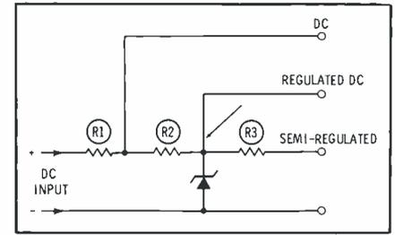
Fig. 3. Zener diode simple voltage regulator.
