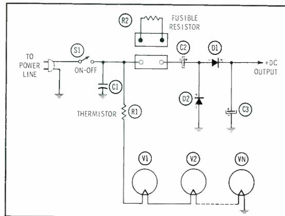
Fig. 4. Two types of protective resistors are often used in television power supplies.
