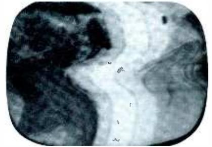
Fig. 9. Negative picture, poor sync resulting from gassy tubes in IF strip of TV receiver.
