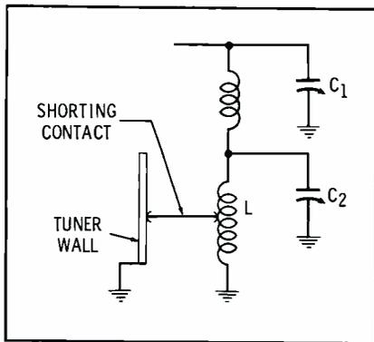
Fig. 3. Schematic of inductance-ring type.
