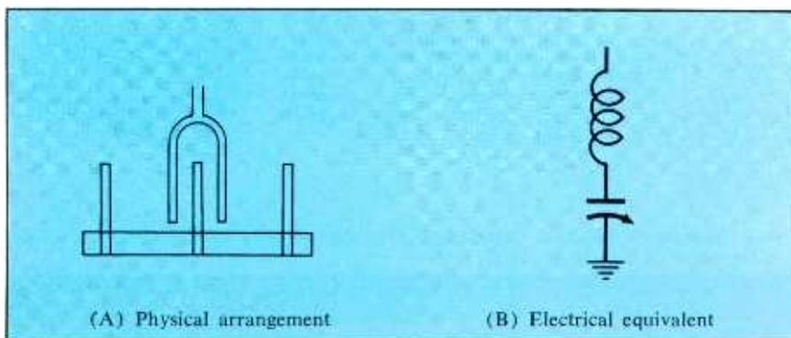
Fig. 1. Physical and electrical arrangement of a typical series-tuned UHF tank circuit.
