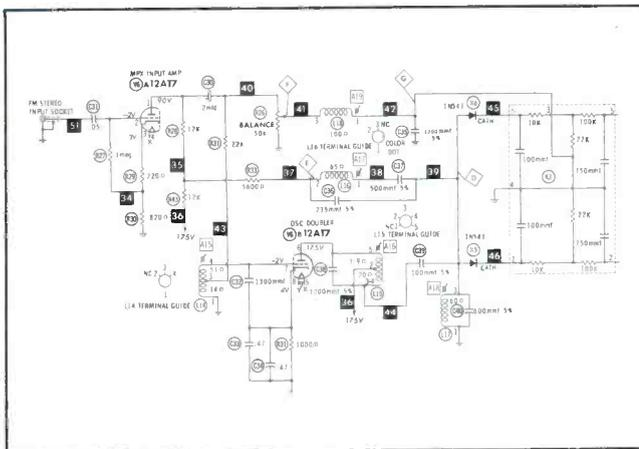
acteristics. (K3 is a most likely suspect.) If trouble still exists, very carefully adjust A19 and R26. Also make sure A15 is correctly adjusted. In some cases, the proper alignment of this coil can be most easily determined by connecting a scope to point D and adjusting A15 and A16 for maximum indication on the scope.
