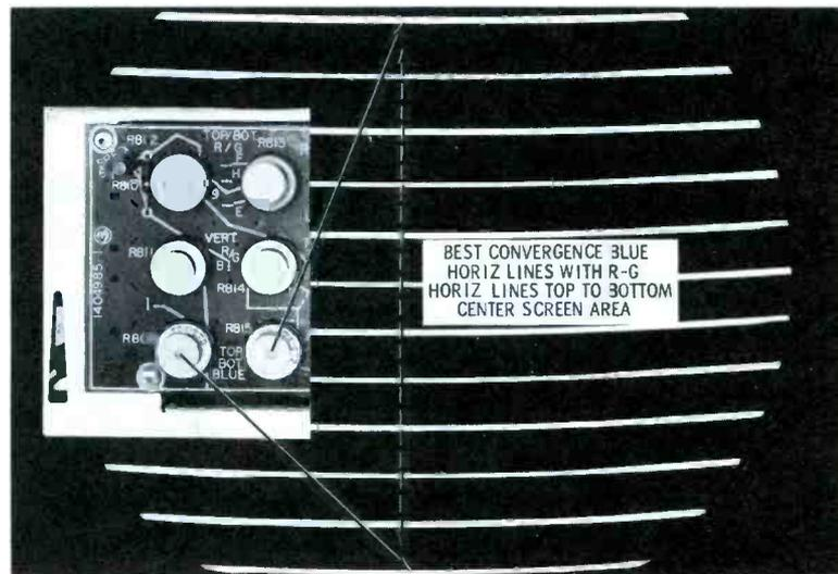
Use Blue horiz lines top (Blue Tilt) and Blue horiz lines bottom (Blue Amp) to converge blue horiz line with red and green lines at the center of the screen.
