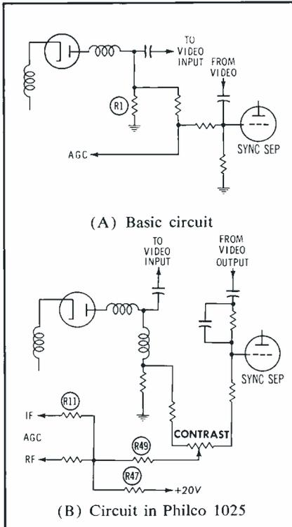
Fig. 8. Circuits producing supplemental AGC. grid of the sync separator resulted in excessive contrast along with disabling of the contrast control.
