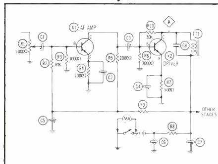
Fig. 5. Audio stages in transistor receiver.
