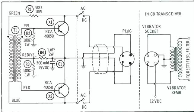
Fig. 3. Transistorized circuit replaces conventional vibrator.
