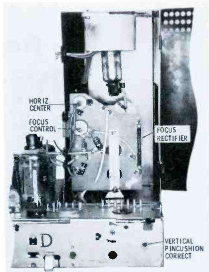
Fig. 4. Diode functions as focus rect.
