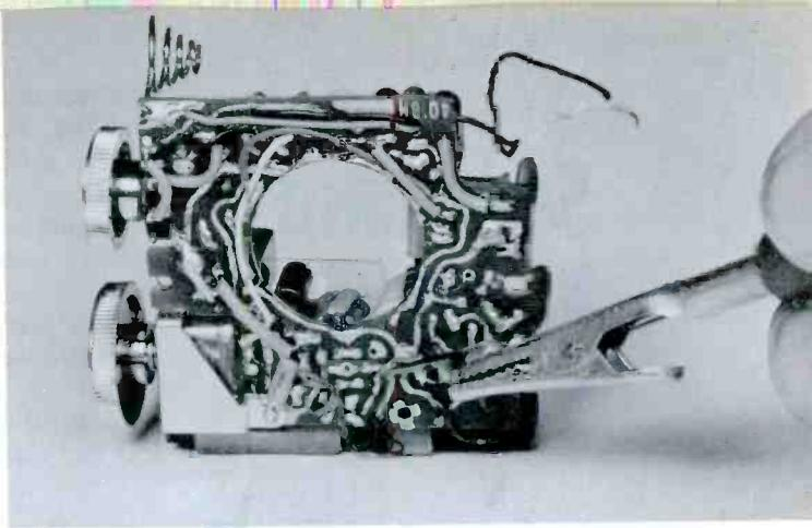
When replacing resistors or capacitors, use a pair of miniature long-nose pliers or small tweezers and a low wattage soldering iron—producing not more than 50 watts. When replacing components or making any repair to the printed board, use rosin-core solder; under no circumstances should an acid-core solder be used for repair.
