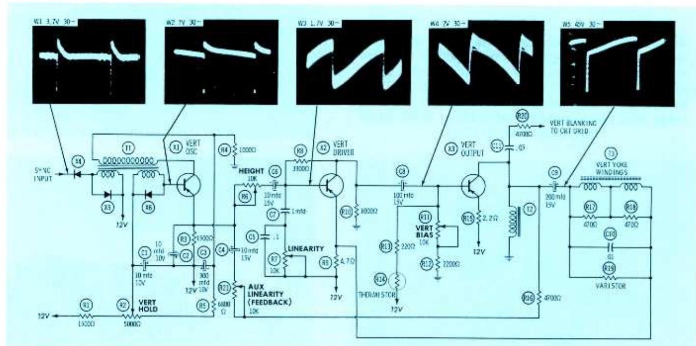
Fig. 1. Schematic diagram of common transistorized vertical deflection system shows basic blocking oscillator-driver-output.
