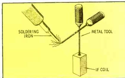
Fig. 12. Melting wax in a sealed IF can.
