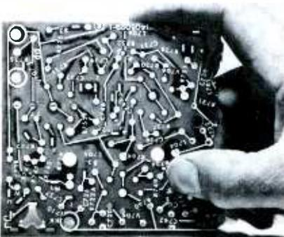
Fig. 1. Backlighting reveals wiring.
