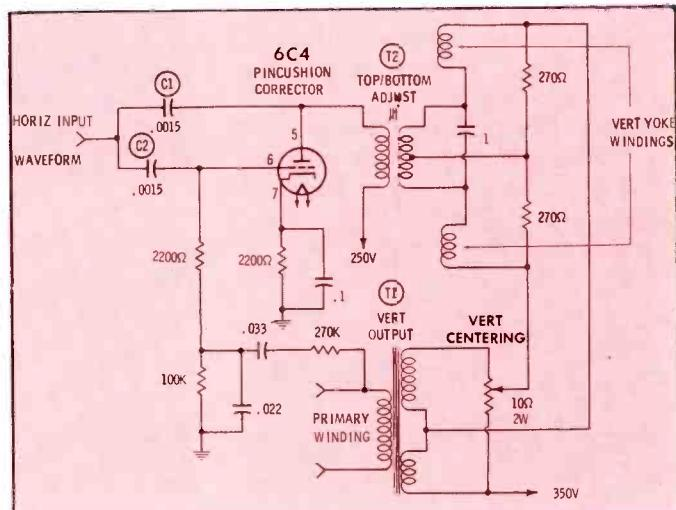
Fig. 6. Circuit compensates for vertical pincushioning.
