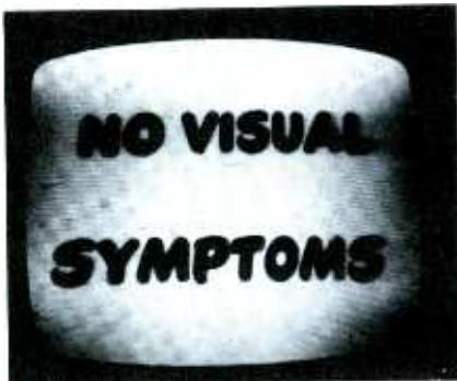
Normal volume is developed, but with volume control near maximum. High-frequency audio is slightly reduced. Symptom might suggest audio-circuit trouble, but any trouble there would generally cause more pronounced change.
