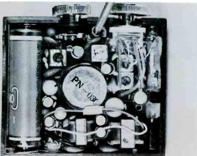
To disassemble these radios, a collection of miniature tools is needed. The set shown here requires a small Phillips screwdriver; however, for other makes and models you will need a set of jeweler's screwdrivers and a multitude of small-size spindrivers. Magnetized tools make the job considerably easier, especially during reassembly.
