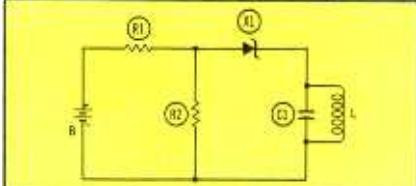
Fig. 4. Tunnel-diode oscillator circuit.
