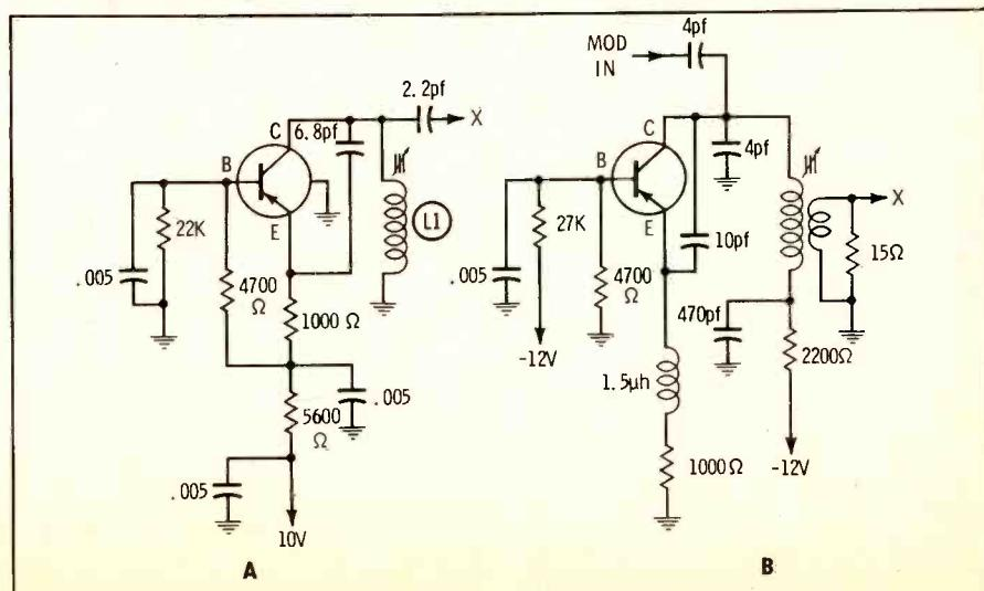
**Fig. 23.** C-B capacitance is responsible for sustaining oscillation at VHF.
