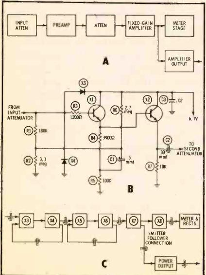
Fig. 18. Sectional arrangement and preamp schematic of audio voltmeter.
