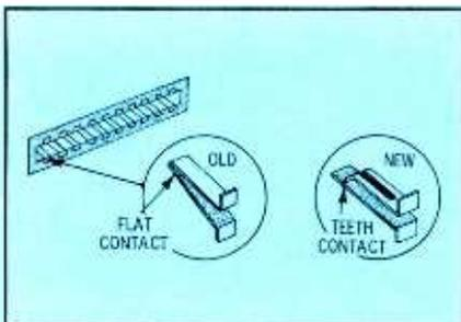
Fig. 2. New contact type solves fault.
