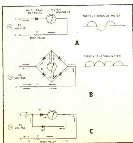
Fig. 1. Most common rectifier circuits.
