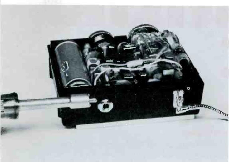
The terminal wrench (sometimes referred to as spanner wrench) is invaluable for removing the nut from tiny earphone jacks. This tool is available in two sizes —  $\frac{1}{2}$ " and  $\frac{5}{16}$ ". Once the screws and earphone jacks are removed, the only thing left is to disconnect the speaker wires. These wires will break quite easily—be careful.
