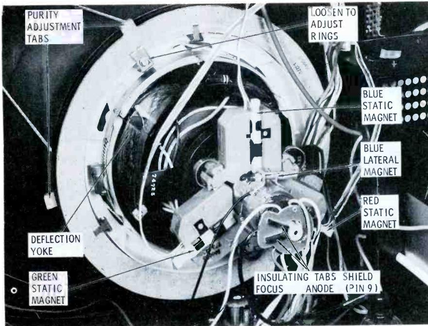
Fig. 3. Purity ring is in front of deflection yoke on 25" color receivers.
