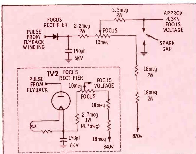
Fig. 5. Focus circuit for the 21" and 25" color receivers.
