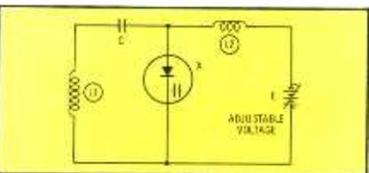
Fig. 5. Varactor diode in tuned circuit.
