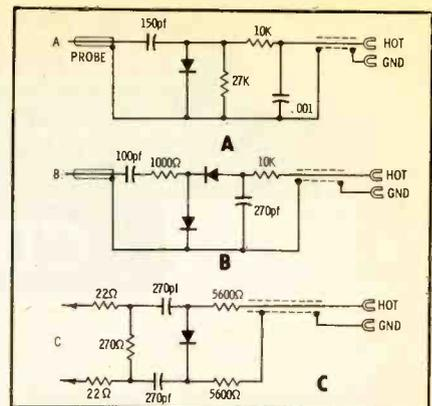
Fig. 5. Demod probes for scope, VTVM.
