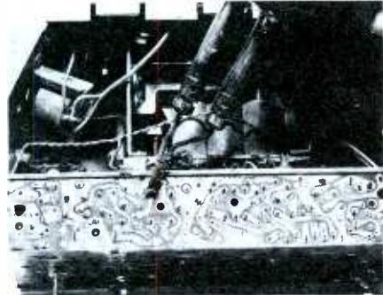
Fig. 8. With foil on both top and bottom of etched board, extra heat is required.
