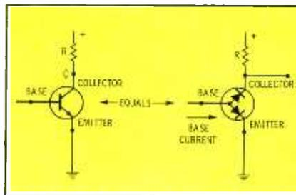
Fig. 1. Switch equivalent of transistor.
