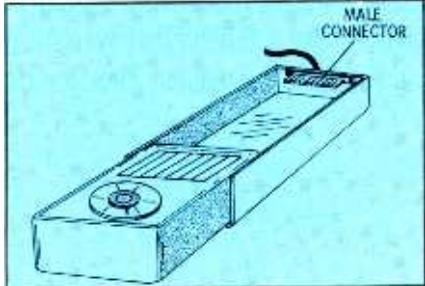
**Fig. 8. Don't insert radio upside down.**
