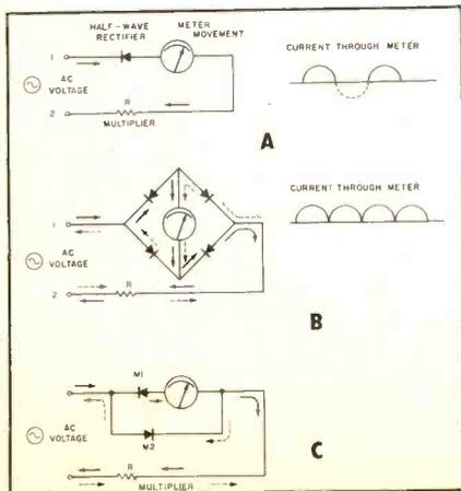
Fig. 1. Most common rectifier circuits.
