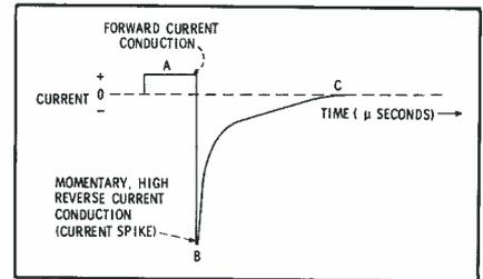
Fig. 8. PIN-diode characteristic curve.
