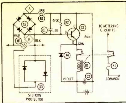
Fig. 7. Elaborate protection for VOM.
