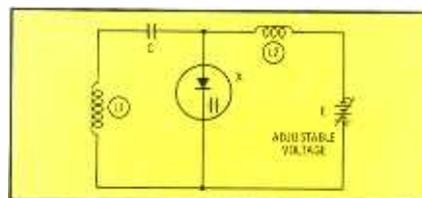
Fig. 5. Varactor diode in tuned circuit.
