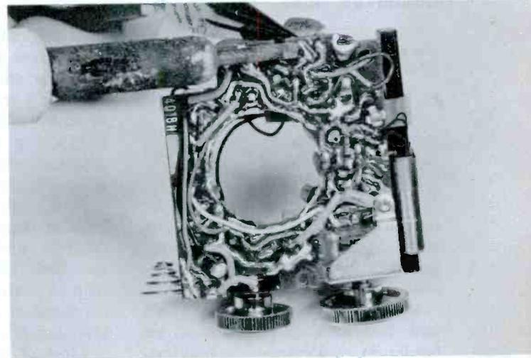
When replacing coils or transformers with multiple connection lugs, a desoldering iron makes the job much easier, quicker, and neater. This type of iron removes all the solder from around the connection point and leaves the hole open so that the defective component can be removed and the new one reinserted without trouble.
