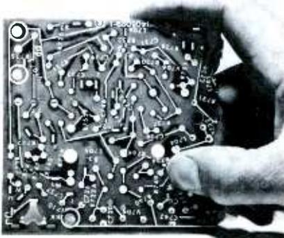
Fig. 1. Backlighting reveals wiring.
