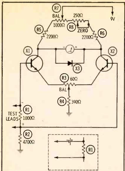
Fig. 17. A bridge-type voltmeter that uses differential-amplifier principles.
