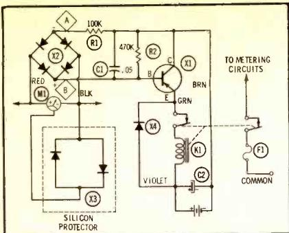
**Fig. 7. Elaborate protection for VOM.**
