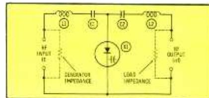
Fig. 6. Varactor used as RF multiplier.
