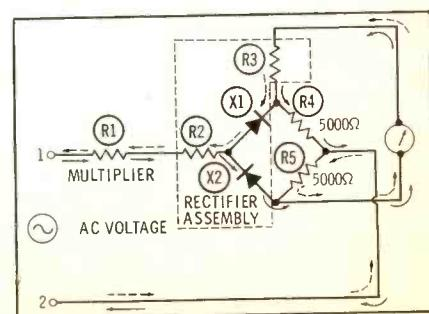
Fig. 2. Full-wave with only two diodes.
