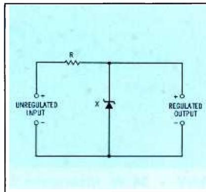
Fig. 2. Zener diode used as regulator.
