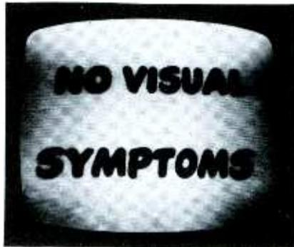
Volume control must be set close to maximum for normal listening level. Along with audio, slight background noise and distortion are heard. Trouble doesn't seem to be in ratio detector circuit, since fault there would probably cause more distortion.
