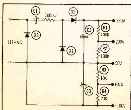
Fig. 4. Voltage tripler; note GND point.
