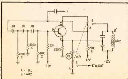
**Fig. 26. Unusual combination makes circuit either Colpitts or phase-shift.**
