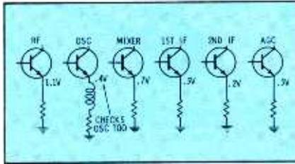
Fig. 7. Emitter test for open transistor.
