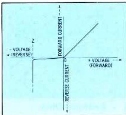
Fig. 1. Voltage-current curve of zener.
