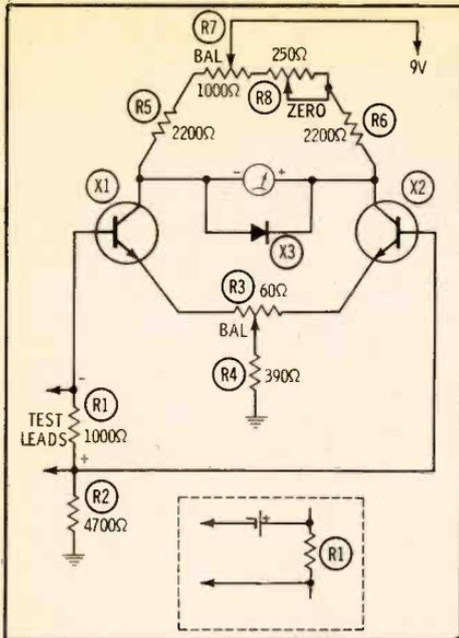
Fig. 17. A bridge-type voltmeter that uses differential-amplifier principles.
