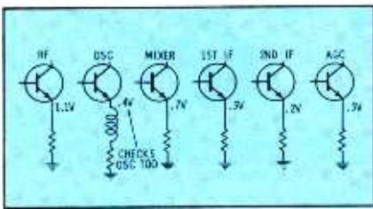
**Fig. 7. Emitter test for open transistor.**
