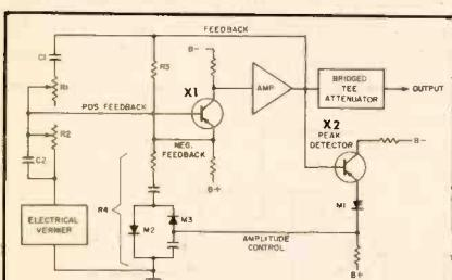
**Fig. 25.** A Wien-bridge oscillator with added circuit to stabilize output level.
