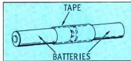
**Fig. 9. Tape stops crackling sound.**
