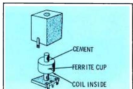
Fig. 5. Loose collar shifts frequency.
