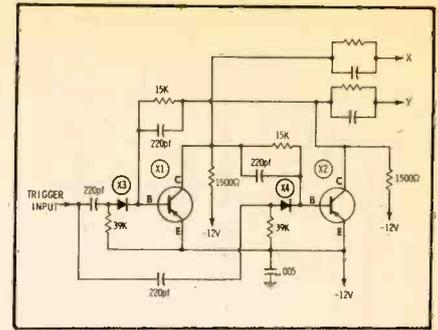
**Fig. 27. Bistable multivibrator is cut off during every second cycle of input.**
