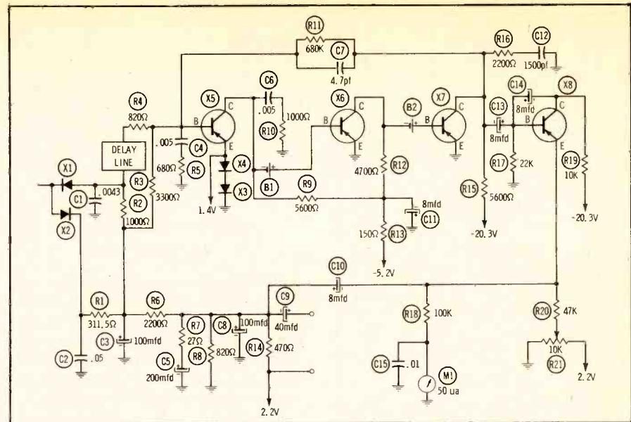
Fig. 14. Deviation-reading section contains both discriminator and voltmeter.
