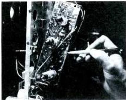
Fig. 5. Notice loose grounding eyelet.
