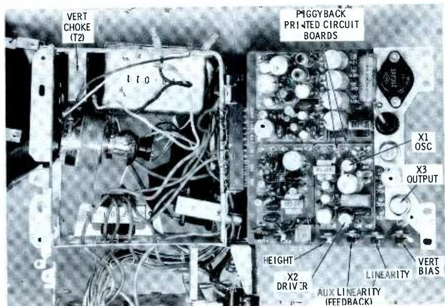
Fig. 2. View of transistorized vertical-sweep section shows typical components.
