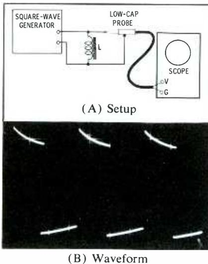
Fig. 2. Iron-core test results differ.
