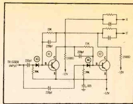
**Fig. 27.** Bistable multivibrator is cut off during every second cycle of input.
