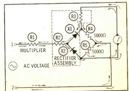
Fig. 2. Full-wave with only two diodes.
