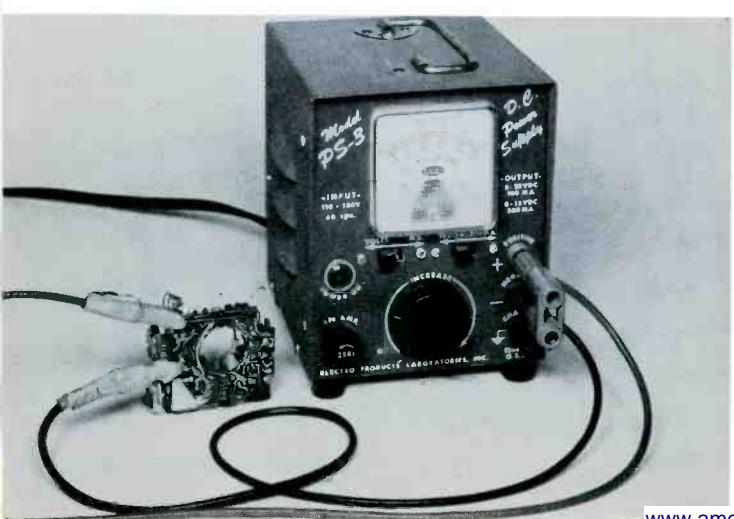
Many small radios operate on a single 1.5-volt battery. A DC power supply capable of supplying from 1.5 to 12 volts is suitable for practically any transistor radio. Before connecting the external power source, check to see if the radio requires a positive or negative voltage. Improper supply connection can damage the transistors.
