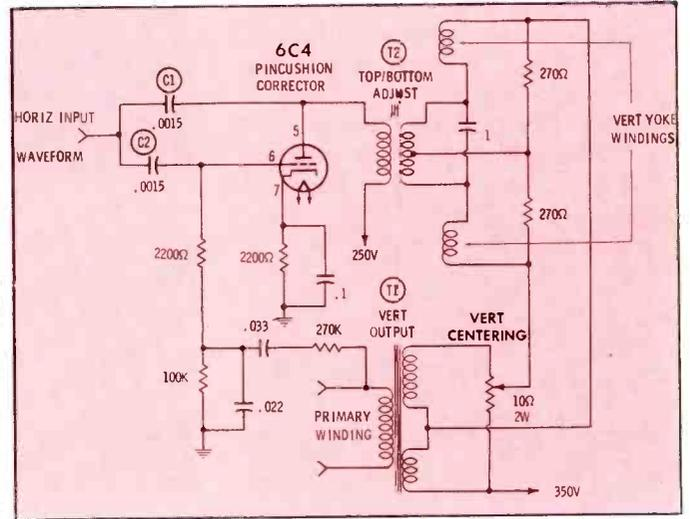
Fig. 6. Circuit compensates for vertical pincushioning.
