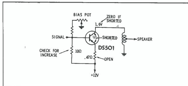
Fig. 13. Watch for these possible faults in power stage. 0 and 70 ohms when the leads are flexed.
