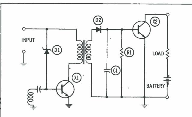
Fig. 2. Transistor oscillator keys switch in this circuit.
