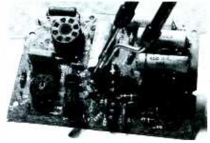
Fig. 3. "Looping" new part to board.
