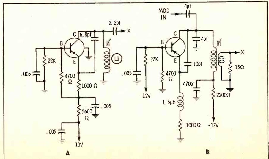
**Fig. 23. C—B capacitance is responsible for sustaining oscillation at VHF.**
