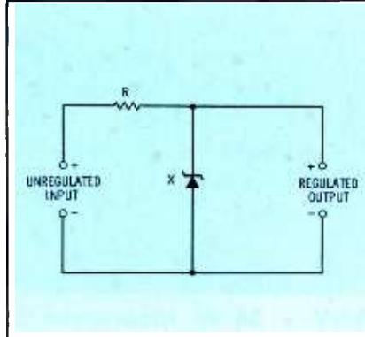
Fig. 2. Zener diode used as regulator.
