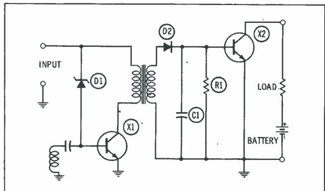
Fig. 2. Transistor oscillator keys switch in this circuit.
