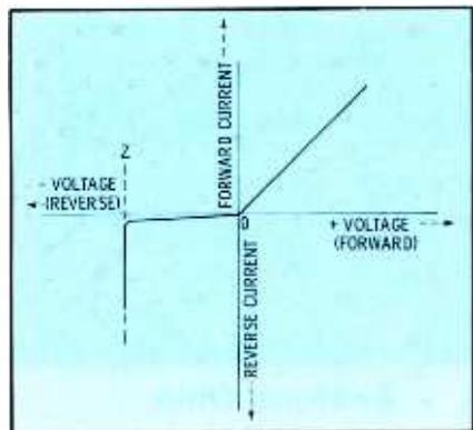
Fig. 1. Voltage-current curve of zener.
