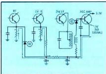
Fig. 3. Emitter volts clue to leakage.
