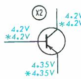
Base voltage is up .2 volt; collector voltage is 1.5 volt high; emitter voltage has increased .15 volt. Potential difference between emitter and collector is down 1.35 volt, reduces conduction of X2. Base-emitter potential difference is down .05 volt; reduced forward bias also decreases conduction. Remember X2 conduction has decreased; voltage at collector has increased, pointing to R7. Resistance check shows R7 to have increased in value. Good idea would be to replace X2 and R6 as well as R7.
