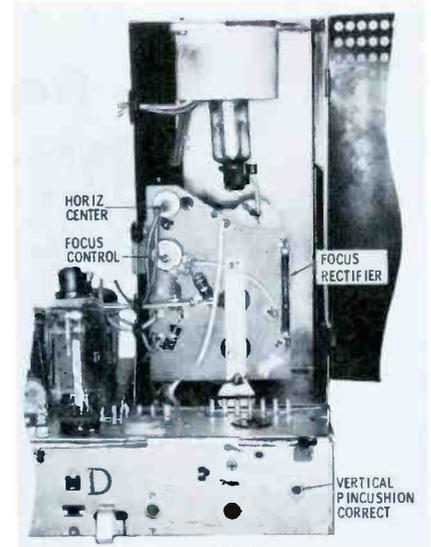
Fig. 4. Diode functions as focus rect.
