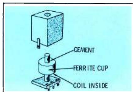
Fig. 5. Loose collar shifts frequency.
