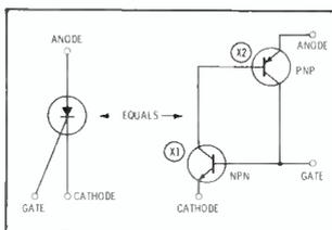
Fig. 4. Equivalent circuit.
