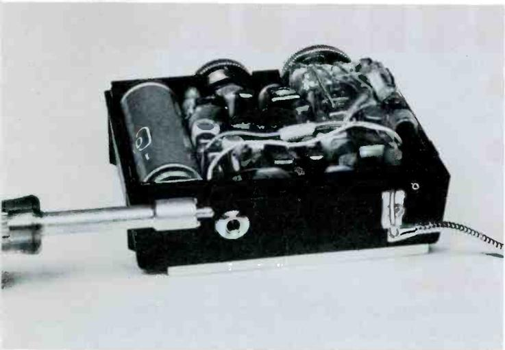
The terminal wrench (sometimes referred to as a spanner wrench) is invaluable for removing the nut from tiny earphone jacks. This tool is available in two sizes — 1/2" and 5/16". Once the screws and earphone jacks are removed, the only thing left is to disconnect the speaker wires. These wires will break quite easily—be careful.
