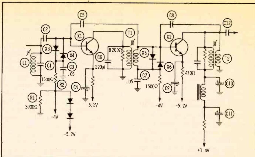
**Fig. 13. These IF stages operate much the same as any solid-state RF amp.**
