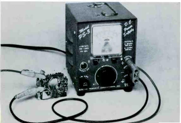
Many small radios operate on a single 1.5-volt battery. A DC power supply capable of supplying from 1.5 to 12 volts is suitable for practically any transistor radio. Before connecting the external power source, check to see if the radio requires a positive or negative voltage. Improper supply connection can damage the transistors.
