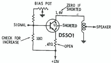
Fig. 13. Watch for these possible faults in power stage. 0 and 70 ohms when the leads are flexed.
