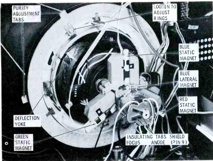
Fig. 3. Purity ring is in front of deflection yoke on 25" color receivers.
