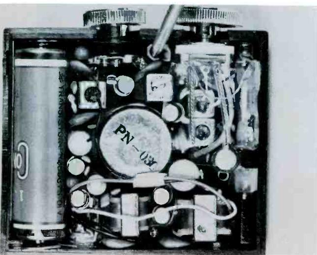
To disassemble these radios, a collection of miniature tools is needed. The set shown here requires a small Phillips screwdriver; however, for other makes and models you will need a set of jeweler's screwdrivers and a multitude of small-size spindrivers. Magnetized tools make the job considerably easier, especially during reassembly.
