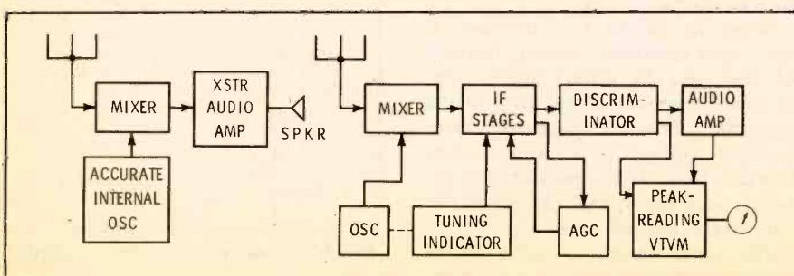
**Fig. 12. Simple and elaborate frequency meters using heterodyne principle.**
