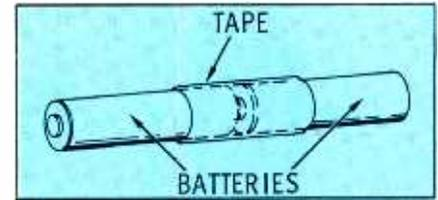
Fig. 9. Tape stops crackling sound.
