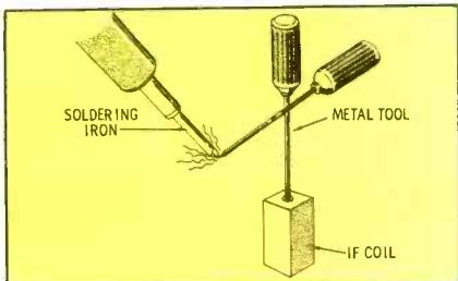
Fig. 12. Melting wax in a sealed IF can.
