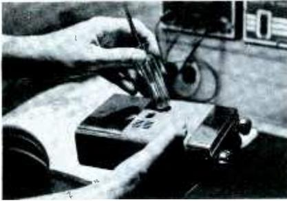
Fig. 6. Tapping case aggravates fault.
