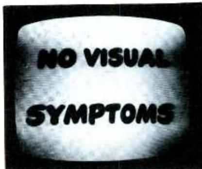
Normal volume can only be obtained by setting volume control almost to maximum. Since audio is so low at normal setting, noise and vertical buzz are heard with higher setting. Such noise is most likely to be picked up in stages where audio is weak.
