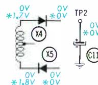
Voltages at X4 anode, X5 cathode are over twice normal. No voltage is measured at X4 cathode, X5 anode, nor at top of C11 (best clue). For voltage to be applied to C11, current must flow through X4. Path for RF current is from ground, up through R11 and R10, left through R8 and X4, down through secondary of T3, and right through X5 and R9 to ground. (Additional path is through tertiary winding of T3 and down through C12.) X4 tests good. Continuity checks show T3 secondary open.
