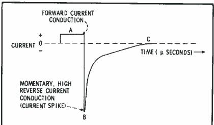
Fig. 8. PIN-diode characteristic curve.
