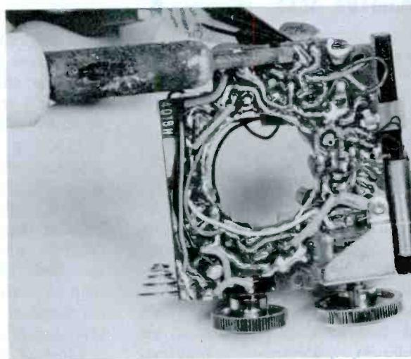
When replacing coils or transformers with multiple connection lugs, a desoldering iron makes the job much easier, quicker, and neater. This type of iron removes all the solder from around the connection point and leaves the hole open so that the defective component can be removed and the new one reinserted without trouble.
