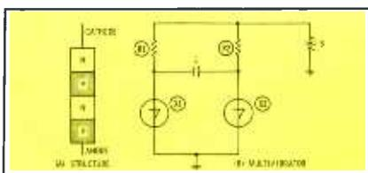
Fig. 7. Circuit using four-layer diode.
