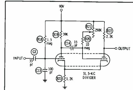
Fig. 3. Schematic is typical of the six multivibrator frequency-divider stages.
