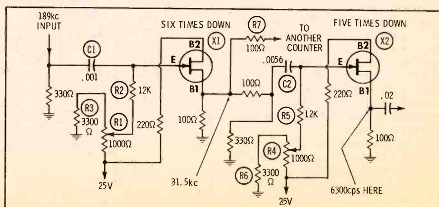
**Fig. 28.** Latest development for counting circuits is the unijunction transistor.
