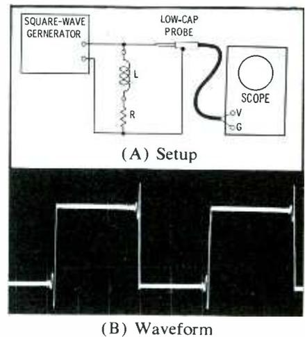
Fig. 4. Shunted inductance will ring. shoot or ringing, because the IF coil rings at a frequency which is practically out of the scope's passband. On the other hand, a 15-mc triggered-sweep scope has usable response at 20 or even 25 mc—which permits a useful ringing test.
