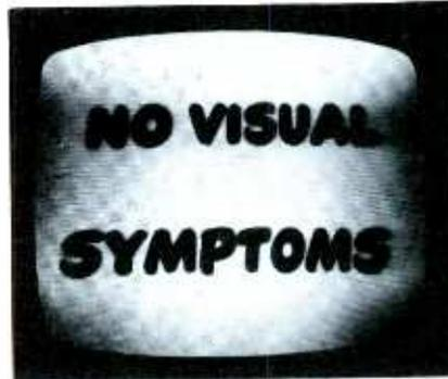
Normal volume can only be obtained by setting volume control almost to maximum. Since audio is so low at normal setting, noise and vertical buzz are heard with higher setting. Such noise is most likely to be picked up in stages where audio is weak.
