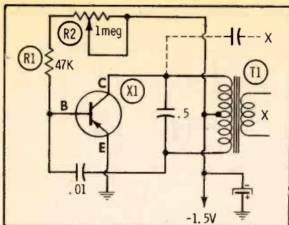
**Fig. 24.** Hartley form of audio oscillator uses tapped choke or transformer.
