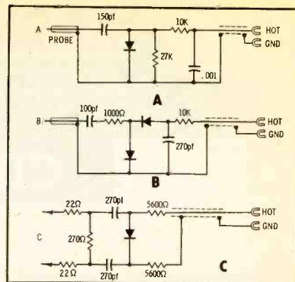
Fig. 5. Demod probes for scope, VTVM. sistance; the tap is brought out to a third terminal on the meter case, and the protective diode unit is connected across the armature only. With this arrangement (Fig. 6B), greater surges can be withstood without damage to either the protector or the meter.
