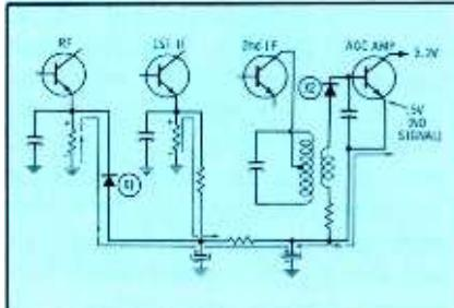
Fig. 3. Emitter volts clue to leakage.
