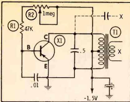
**Fig. 24. Hartley form of audio oscillator uses tapped choke or transformer.** tion of the transistor, the signal energy is self-sustaining—a requirement for oscillation. Note that output is via a capacitor at X for phase-shift operation, with capacitor C1 as an emitter bypass. For 67-kc oscillation, C1 is switched to the 67-kc output line, and the stage acts as an emitter follower.
