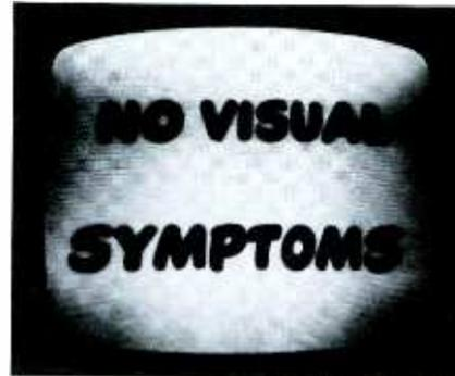
Normal volume can be obtained only by setting volume control almost to maximum. When this is done, buzz becomes quite loud. Slight distortion of audio also is evident. Most likely location of trouble is in stages prior to audio, so tests can be limited to IF and detector.
