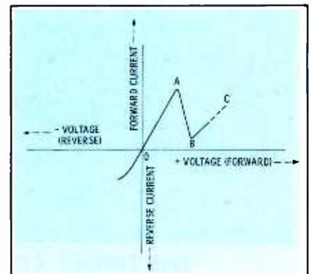
Fig. 3. Characteristic of tunnel diode.
