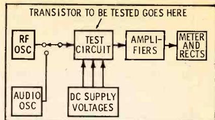
Fig. 19. Standard transistor circuits can be used to test other transistors.
