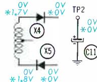
Voltages at X4 anode, X5 cathode are over twice normal. No voltage is measured at X4 cathode, X5 anode, nor at top of C11 (best clue). For voltage to be applied to C11, current must flow through X4. Path for RF current is from ground, up through R11 and R10, left through R8 and X4, down through secondary of T3, and right through X5 and R9 to ground. (Additional path is through tertiary winding of T3 and down through C12.) X4 tests good. Continuity checks show T3 secondary open.
