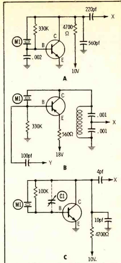
**Fig. 22.** Three crystal-controlled transistor oscillators of the Pierce variety.
