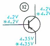
Base voltage is up .2 volt; collector voltage is 1.5 volt high; emitter voltage has increased .15 volt. Potential difference between emitter and collector is down 1.35 volt, reduces conduction of X2. Base-emitter potential difference is down .05 volt; reduced forward bias also decreases conduction. Remember X2 conduction has decreased; voltage at collector has increased, pointing to R7. Resistance check shows R7 to have increased in value. Good idea would be to replace X2 and R6 as well as R7.
