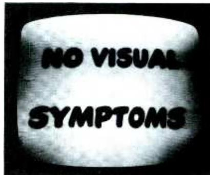
With volume control at maximum, slight buzz and background noise are heard; no audio signal is present. Since noise and buzz are heard from speaker, audio stages must be good. Noise is low in volume, so suspected stage is near end rather than near beginning of sound IF strip.
