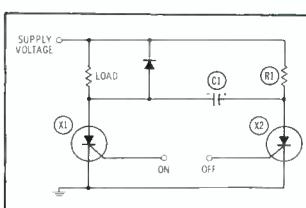
**Fig. 5. Two-SCR gate stage.**
