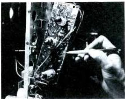
Fig. 5. Notice loose grounding eyelet.
