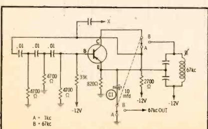
**Fig. 26.** Unusual combination makes circuit either Colpitts or phase-shift.
