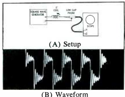
Fig. 1. Ringing test for air-core coil.
