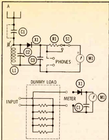
**Fig. 11. Field-strength meter and power meter are basically same circuit type.**
