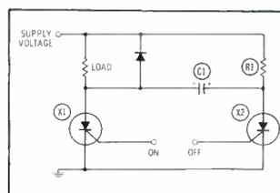
Fig. 5. Two-SCR gate stage.
