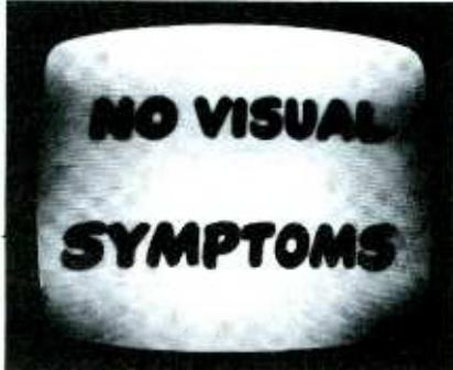
No audio at all. With volume control at maximum, low-level buzz is heard. Output stage is okay since rotating volume-control changes buzz level. Fine-tuning control can be rotated to show sound bars in picture; presence of audio at input to sound IF is indicated.
