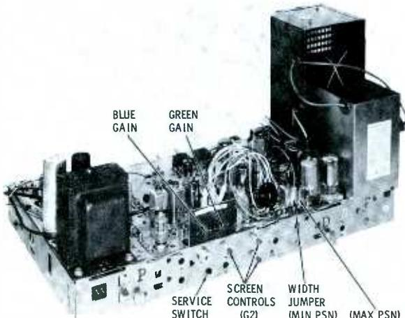
Fig. 1. Zenith's 25" color chassis contains a width jumper.
