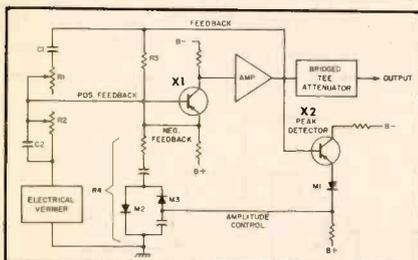
**Fig. 25. A Wien-bridge oscillator with added circuit to stabilize output level.**
