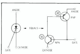
**Fig. 4. Equivalent circuit.**
