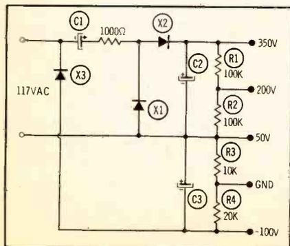
Fig. 4. Voltage tripler; note GND point.
