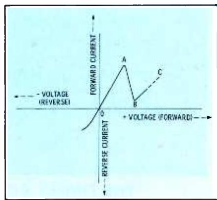
Fig. 3. Characteristic of tunnel diode.
