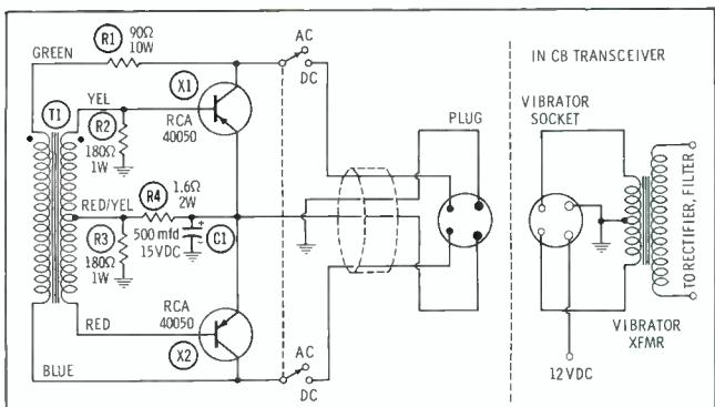
**Fig. 3. Transistorized circuit replaces conventional vibrator.**
