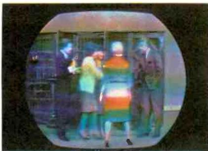
Color is out of lock on this network color broadcast. Use a generator to check whether the trouble is in the receiver or at the station. Remember not to use a strong output signal from the color-bar generator; some sets which exhibit out-of-lock symptoms will display proper sync on a strong signal from the generator. Suspected tubes are the burst amplifier, chroma-sync phase detector, 3.58-mc oscillator, and oscillator control.
