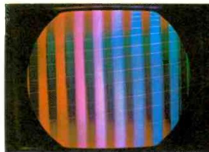
These lines are caused by hum at the cathode of the "X" demodulator on an RCA CTC12, CTC15, CTC16, or CTC17 chassis. No hum is visible on a b-w picture with the color control turned counter-clockwise—a good test to determine if the hum is in the color or b-w stages. Notice the color-bar pattern displays correct colors—that is, the fourth bar is magenta, as it should be. Demodulator tubes in these sets are 6GY6's.
