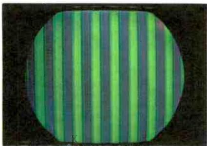
No 3.58-mc oscillator carrier; b-w picture is normal. This condition occurs in RCA chassis CTC12, CTC15, CTC16, and CTC17. In RCA CTC7 to CTC11, the bars are purple. The tint control has no effect on the bars; the color control will reduce their intensity. These bars are caused by demodulator overload on color sidebands. Zenith sets show no color bars; the screen is bluish green. Check the 3.58-mc oscillator and reference-control tubes.
