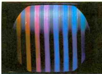
This distorted color-bar pattern was caused by hum in the cathode circuit of the R-Y, B-Y, and G-Y amplifiers. The hum also could be seen on a b-w picture. The cathodes of all three difference amplifiers are connected together, and a common cathode resistor is used; thus, all colors are distorted. Such hum can appear on any RCA chassis from CTC7 up. Zenith and some Motorola receivers do not use difference-amplifier stages.
