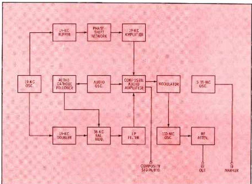
Fig. 2. Simulated stereo signal generation similar to FM station exciter unit.
