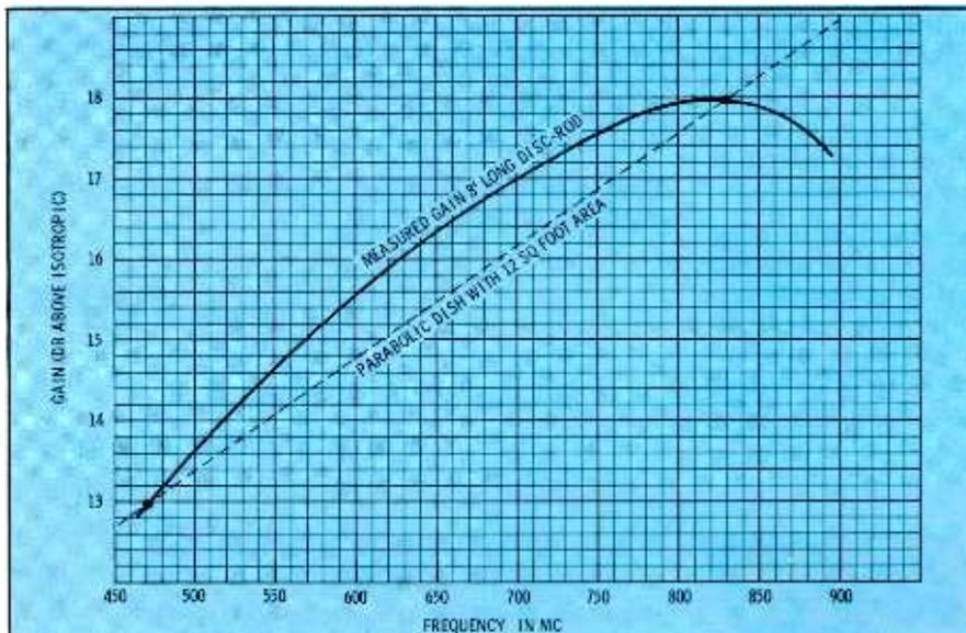
Fig. 1. Gain-frequency characteristics, disc-rod and parabolic type antennas.
