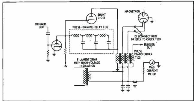
Fig. 6. Mag current is "zero" with maggie disconnected.
