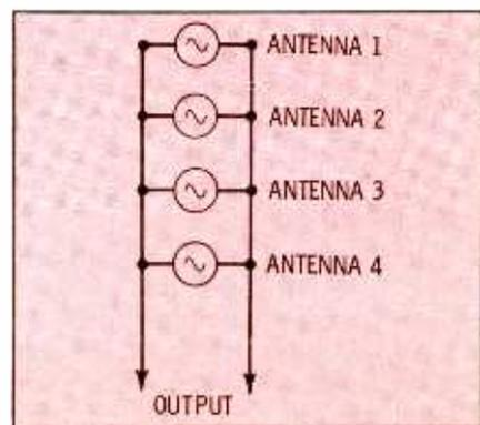
**Fig. 8. Analogy comparing four antennas to four parallel wired generators.**
