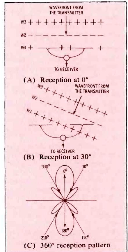
Fig. 4. Reception patterns of 1/2-wave dipoles spaced one wavelength apart.
