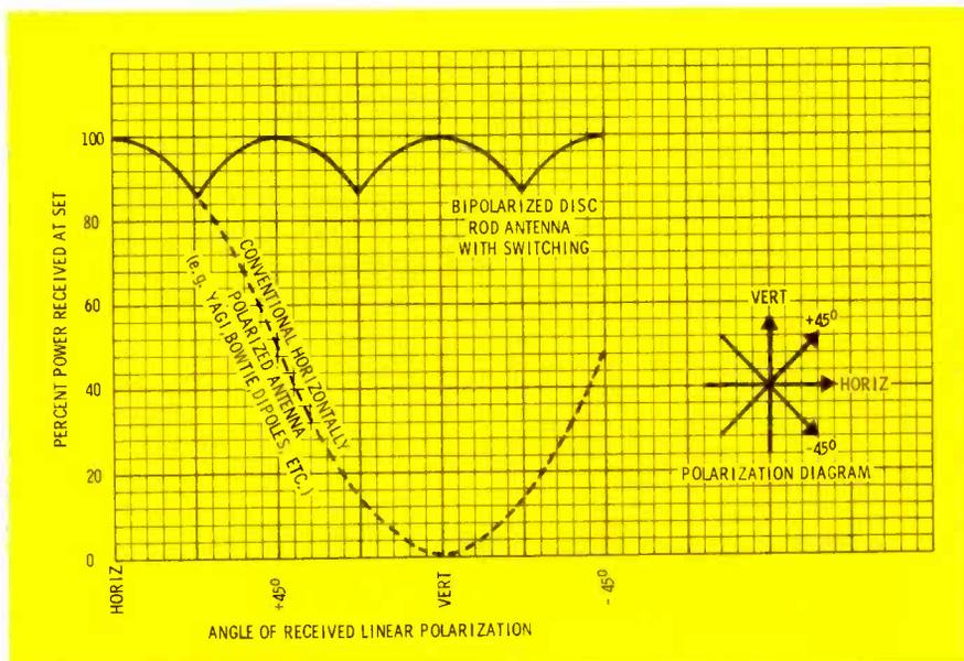
Fig. 3. Performance comparison under various conditions of polarization.
