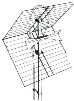
Two screens meet to make a corner and reflect the signal toward a wideband driven element to form the *corner-reflector* antenna.
