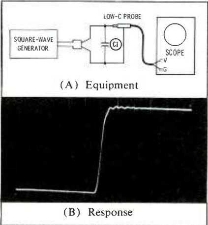
Fig. 1. The capacitor inductance test.
