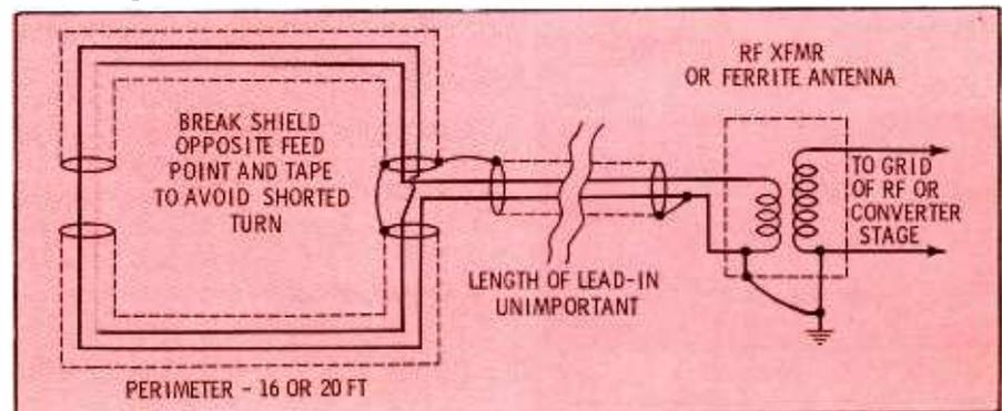
Fig. 5. Low-impedance, shielded loop antenna made of cable.
