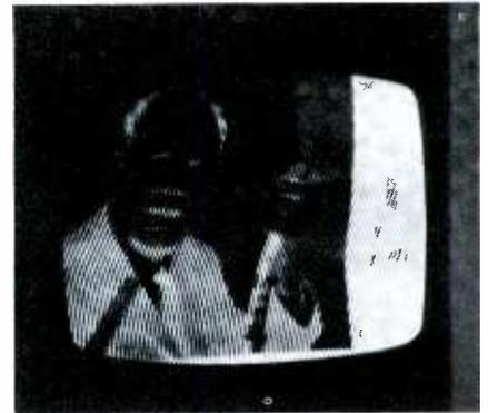
Fig. 4. RF overload, negative picture.
