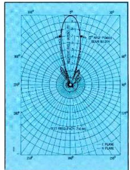
Fig. 2. Directional characteristics of a single-bay disc-rod type antenna.
