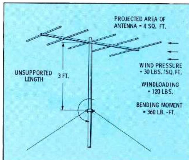
Fig. 3. Bending moment equals windload  $\times$  free length.
