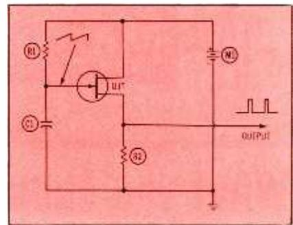
Fig. 7. Simplified UJT timer circuit.
