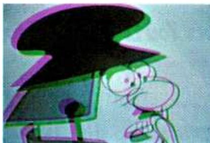
Displaced color is normally caused by the misconvergence of one color—in this case, green. In all cases of misconvergence, first be sure to position the static convergence magnets correctly; also, these should be double checked after the vertical convergence controls have been adjusted but before the horizontal controls are aligned. Without these static checks, you may be working for nothing and have to readjust dynamic convergence.
