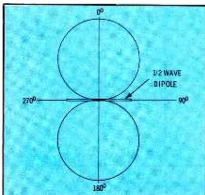
Fig. 1. Sensitivity of simple  $\frac{1}{2}$ -wave dipole plotted for horizontal plane.
