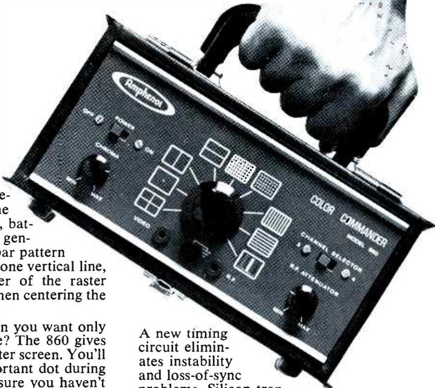
A new timing circuit eliminates instability and loss-of-sync problems. Silicon transistors maintain built-in precision and stability indefinitely. RF output is on channel 3 or 4, switch selected. An attenuator simulates weak-signal conditions. It has gun killer circuit. Uses 9 penlight cells. Weighs 3½ lbs. in compact leatherette carrying case. \$149.95. Optional AC power supply, \$19.95.
