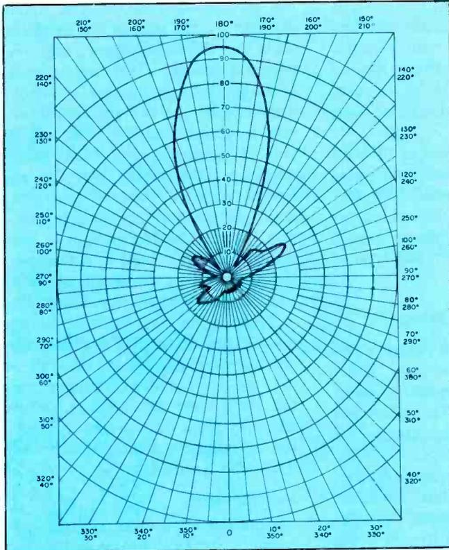
Fig. 2. Yagi antenna pattern plotted in horizontal plane.
