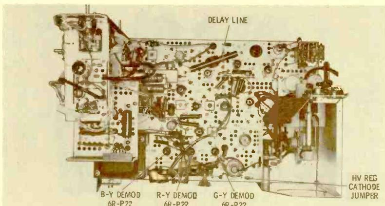
In the color circuits, there are a two-stage chroma bandpass amplifier and three independent demodulators; 6R-P22 tubes are used to demodulate R-Y, B-Y, and G-Y separately. All the other tubes are common types, with the exception of the 5642 focus rectifier.
