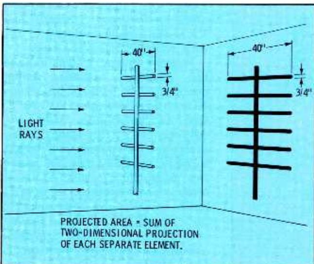
Fig. 2. Projected area of antenna is equivalent to shadow.
