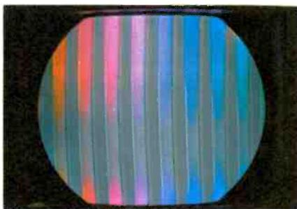
Distortion is due to hum at the cathode of the bandpass amplifier. This distorted color-bar pattern may appear on any color receiver utilizing only one bandpass amplifier stage. In this case the chassis was an RCA CTC16. The distortion isn't visible during monochrome reception, since the bandpass stage is cut off by action of the color killer. In many cases, defects in the bandpass amplifier will result in a complete loss of color.
