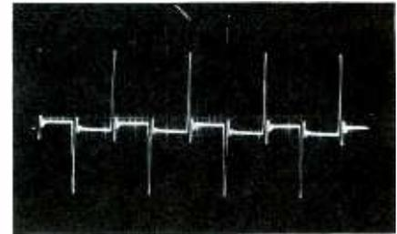
Fig. 7. Testing low-voltage filter cap.
