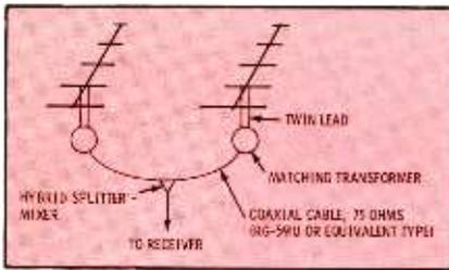
Fig. 5. Proper method of connecting horizontally stacked yagis is shown.
