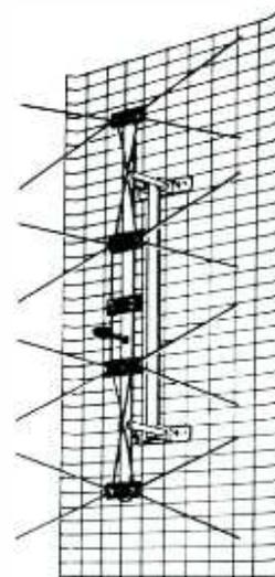
The *bow-tie* antenna provides high gain and broad response in a light-weight and compact unit.
