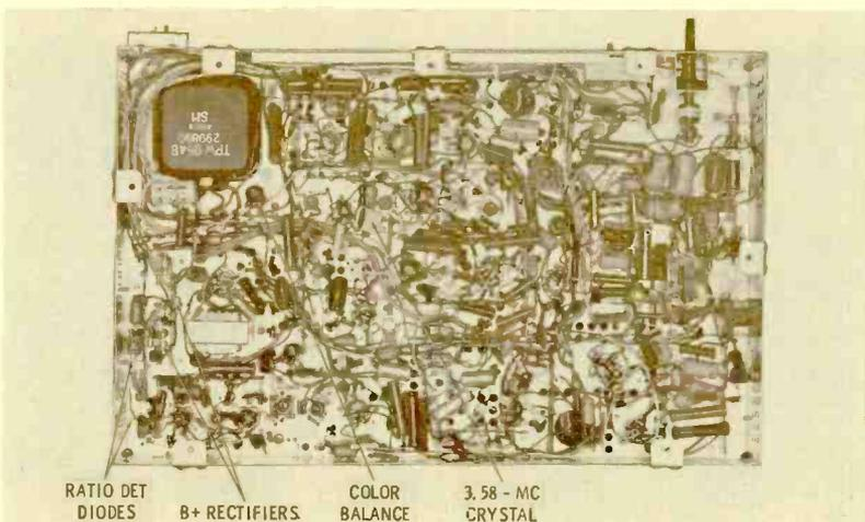
This hand-wired, transformer-powered chassis has a conventional low-voltage power supply—two silicon rectifiers operating in a full-wave voltage-doubler circuit.
