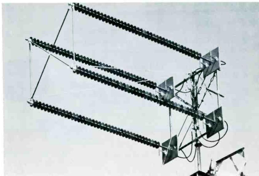
Fig. 4. One of the disc-rod antenna arrays used by Lincoln Laboratories.
