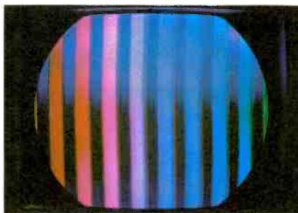
Hum at the cathode of the "Z" demodulator will usually display itself as shown in the above photo. (The b-w picture was free of any symptoms.) This is particularly true of RCA chassis CTC12, CTC15, CTC16, and CTC17. In just about all cases of hum in the video (b-w and color), the trouble is filament-to-cathode leakage in some tube that handles the video signal. First determine if hum is present in b-w, color, or both.
