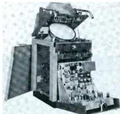
Fig. 1. Typical marine radar indicator showing accessibility for service work.
