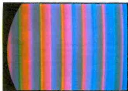
Bars are blurred by misalignment. The fine tuning was detuned, and the generator output and color control were advanced to give full color. Similar bars can be caused by poor IF alignment. Almost as bad a symptom can occur because of poor chroma alignment, multiple sets on the same antenna, poor distribution system, etc. A bar generator provides the best proof, but be sure to disconnect the antenna before connecting the generator.
