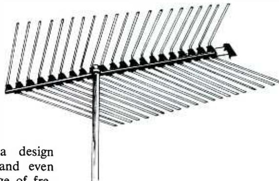
The *log-periodic* antenna design provides high efficiency and even response over a wide range of frequencies.
