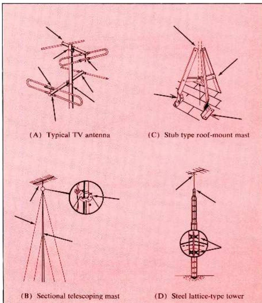
Fig. 2. Beware of these potential antenna trouble spots when making inspection.
