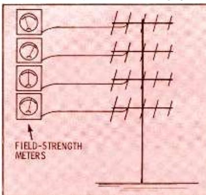
**Fig. 7. Signal strength varies from antenna to antenna on vertical stack.**
