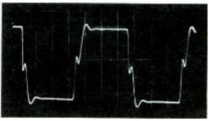
Fig. 2. Ringing caused by test leads.
