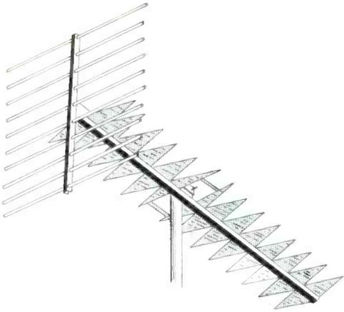
A lightweight, high-gain, and highly directive type is the *planar-helical* antenna (two types are shown).
