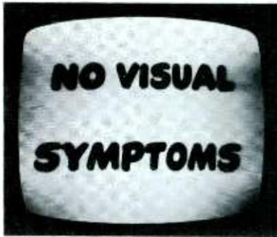
Absolutely no sound can be heard from speaker, even at maximum setting of volume control. Video and sync appear perfectly normal, which clears all circuits which precede sound takeoff. Audio output stage is definitely suspect whenever not even hum or buzz is audible.
