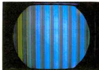
There is no "X" demodulation. Since "X" is closest to R-Y, red bars are missing on the screen, and the green bars are reversed in brightness compared to the blue bars. There is no change in the b-w picture. Loss of "Z" demodulation results in no blue being seen in the picture, since "Z" is close to B-Y. Any RCA chassis (or others using similar demodulator stages) from CTC7 until current models will display this symptom.
