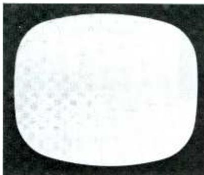
Picture and sound are missing on all channels. Brightness control affects, but can't extinguish, raster. Possibilities include defective CRT; malfunction in brightness circuit; trouble in B+ path which supplies cathode voltage to picture tube.
