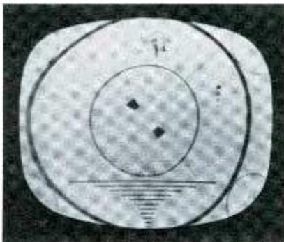
Picture shows video is weak though no snow is present. Sync is occasionally lost, especially when channels are changed. Sound is weak and slightly garbled. Contrast and brightness controls are operative. Loss of gain in IF, video, or output stage is indicated.
