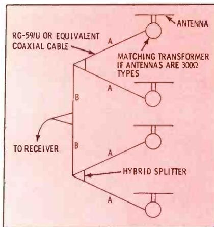
Fig. 9. Four-bay vertical stack antenna with hybrid mixing techniques.
