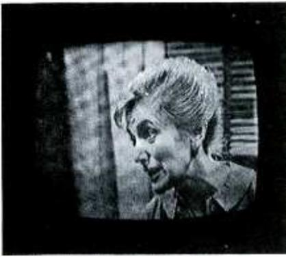
Fig. 3. Picture has weak interference.
