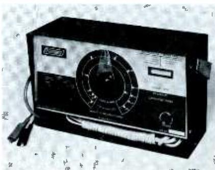
**Fig. 3. Handy capacitor checker can speed preliminary troubleshooting.**
