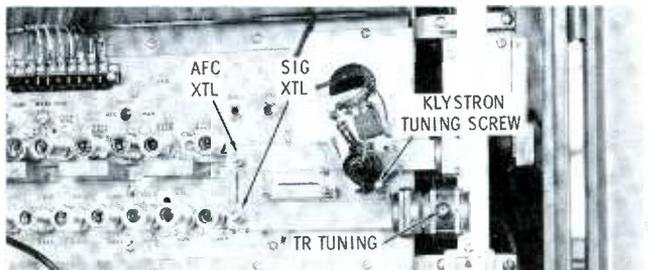
Fig. 7. Receiver "plumbing" shows klystron and TR tuning.
