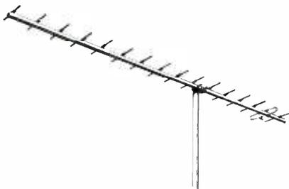
The many parasitic elements of the *yagi* antenna provide for high gain and sharp directivity.
