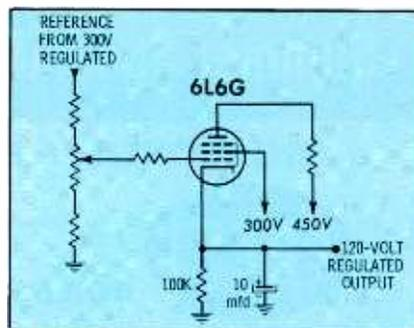
Fig. 4. Simplified schematic. In actual supply, two tubes are used in parallel.
