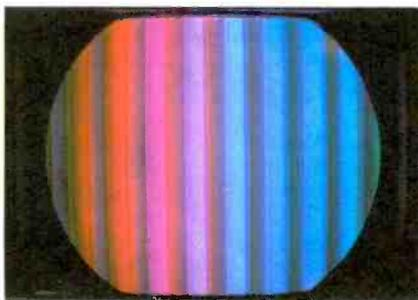
Improper color bars can be caused by a number of tubes and components. In this case, the .01-mfd capacitor shunting the 100K resistor in series with the red grid of the picture tube was open; this caused the R-Y amplifier to have poor high-frequency response. Incorrect colors may also be caused by malfunctions in the burst amplifier, the difference amplifier, and in some cases even the bandpass amplifier stages.
