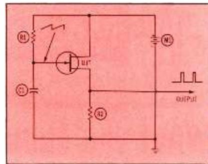
Fig. 7. Simplified UJT timer circuit.
