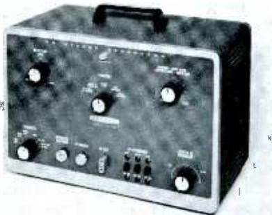
Fig. 1. Crystal-controlled oscillators generate a composite stereo signal.
