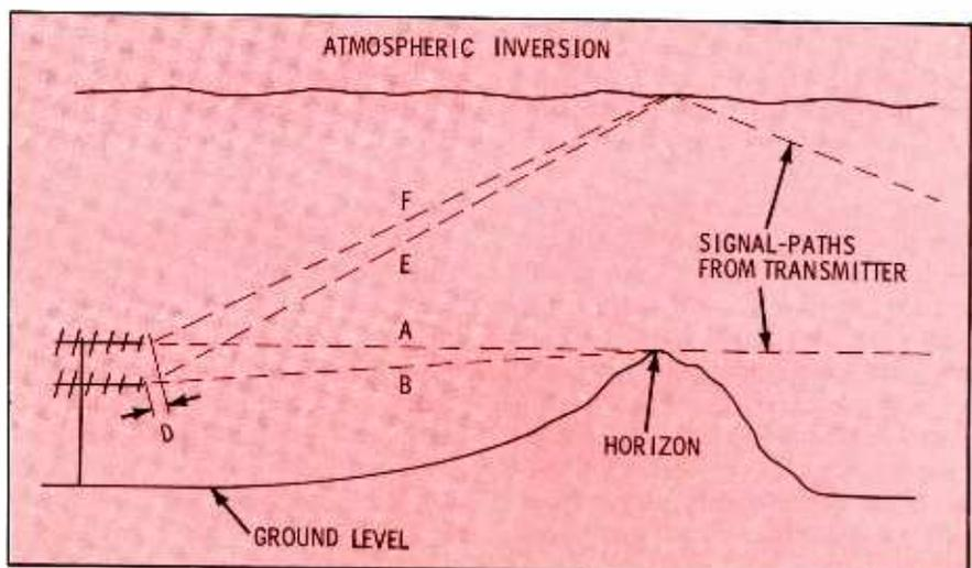
Fig. 6. Multiple signal paths are involved in reception over the horizon.
