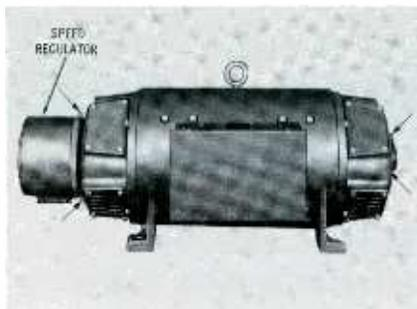
Fig. 3. Cover at left end is removable to expose speed regulator for servicing.
