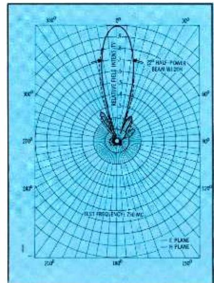
Fig. 2. Directional characteristics of a single-bay disc-rod type antenna.
