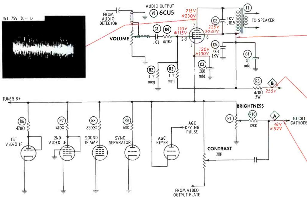
DC VOLTAGES taken with VTVM, on inactive channel; antenna terminals shorted. \*Indicates voltage taken with signal present — see "Operating Variations."
