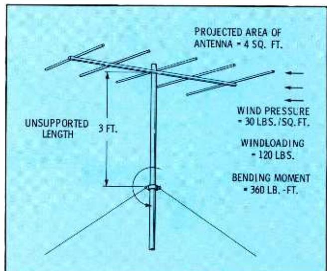
Fig. 3. Bending moment equals windload  $\times$  free length.
