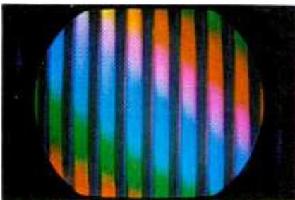
Loss of color sync is a quite common trouble. Notice there is color present only where the color bars should be; however, the color is displaced diagonally across the screen. In this photo the oscillator frequency error is only slight—the greater the error, the more diagonal bars are present (smaller error means fewer bars or stripes). This symptom is indicative of trouble in either the 3.58-mc oscillator or reactance-control stages.
