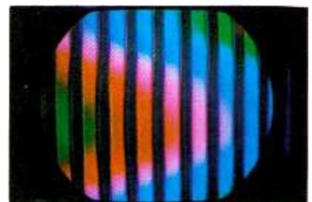
This distorted color-bar pattern was caused by hum being introduced at the cathode of the chroma reference-oscillator control tube in an RCA CTC16 chassis. (However, the same basic symptom will appear on nearly all recent color receivers.) The hum wasn't visible on a black-white picture. Notice the color bars are bent in the shape of a sine wave. In most receivers, the oscillator and oscillator-control tubes are in the same envelope.
