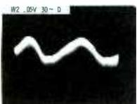
Waveform (W4) is only 25 volts p-p (normal is 100 volts p-p). Loss of gain in preceding stages is responsible for weak picture and poor sync. Plate signal of audio output tube (W1) is reduced almost 50% (p-p amplitude is only 40 volts). Scope has given clue (W4) that decreased B+ voltage supplying IF tubes may be responsible. Amplitude of ripple in W2 is greatly reduced suggesting increase in value of R5 could be responsible for trouble.
