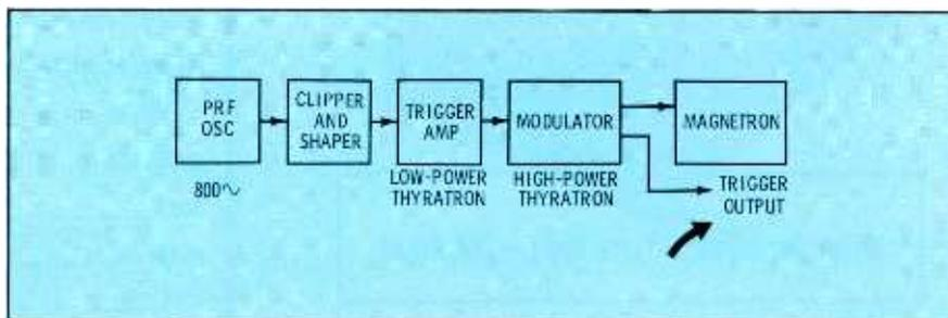
Fig. 5. The pulse-repetition-frequency oscillator sets timing via the trigger.
