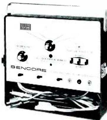
Fig. 4. Color-bar generator has gun interrupters and storage compartment.
