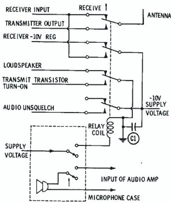
Fig. 8. Switching in 5w solid-state unit.
