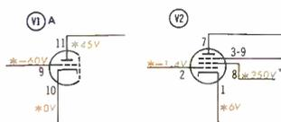
Grid of V1A measures -60 volts. V2 must be conducting more, providing greater feedback, causing increased bias of 6BA11. Pin 8 6GK6 has insignificant voltage change, but pin 1 voltage has dropped 50%, reducing bias on V2. This permits conduction to start on lower nonlinear portion of drive pulse and explains stretched top portion of picture. Negative voltage on pin 2 V2 indicates grid drawing current, resulting in foldover at bottom. Resistance check at pin 1 shows C1 has 100-ohm leakage.
