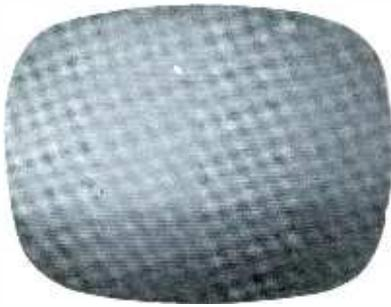
Fig. 5A. AGC faults cause white raster.
