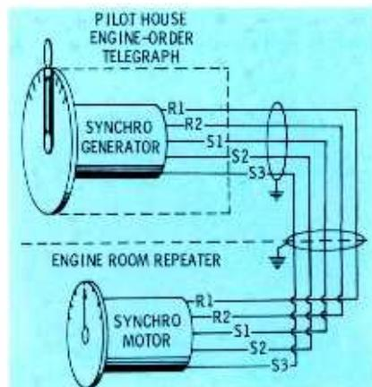
Fig. 1. Synchro system relays information from pilot house to engine room.
