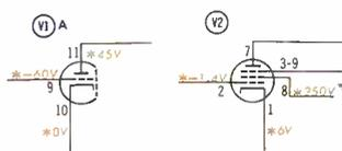
Grid of V1A measures -60 volts. V2 must be conducting more, providing greater feedback, causing increased bias of 6BA11. Pin 8 6GK6 has insignificant voltage change, but pin 1 voltage has dropped 50%, reducing bias on V2. This permits conduction to start on lower nonlinear portion of drive pulse and explains stretched top portion of picture. Negative voltage on pin 2 V2 indicates grid drawing current, resulting in foldover at bottom. Resistance check at pin 1 shows C1 has 100-ohm leakage.
