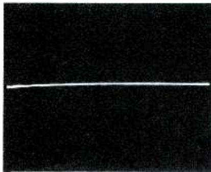
Narrow horizontal line through center of screen indicates absence of vertical sweep. Vertical linearity or size controls have no effect on bright horizontal line. Turning vertical hold produces no change. Rotation of controls renders no helpful hints.
