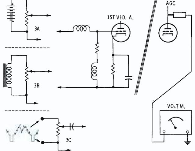
Fig. 2. Amplified-AGC circuit used in early model RCA's. Fig. 3. How AC and DC potentials affect video amplifier.
