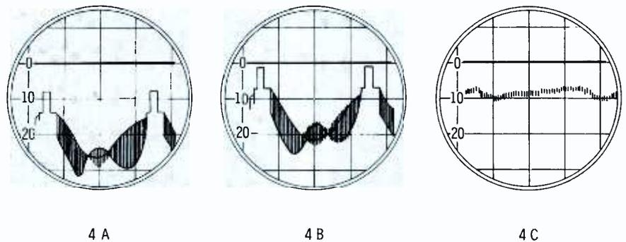
Fig. 4. Waveform as it appears at grid and cathode of AGC amplifier V15A.
