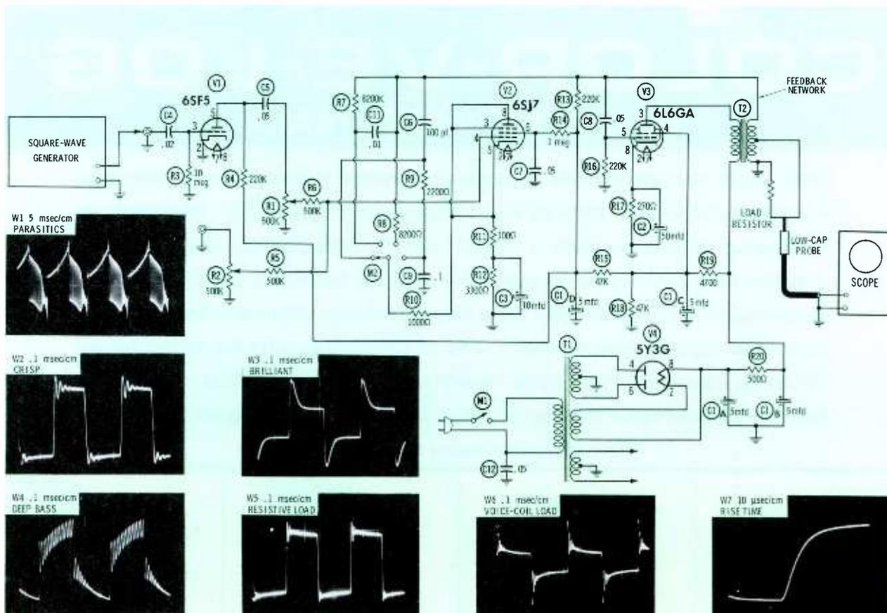
Fig. 2. Utility amplifier commonly used for public-address systems provides better reproduction than the two-tube type.
