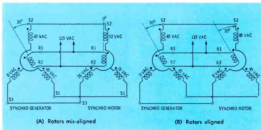
Fig. 5. High current flows until both rotors are aligned—residual current remains.
