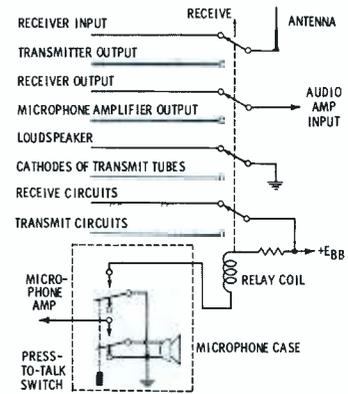
Fig. 9. Switching in vacuum-tube unit.
