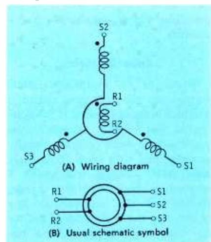
Fig. 2. Wiring and schematic diagrams for the synchro generator or motor.
