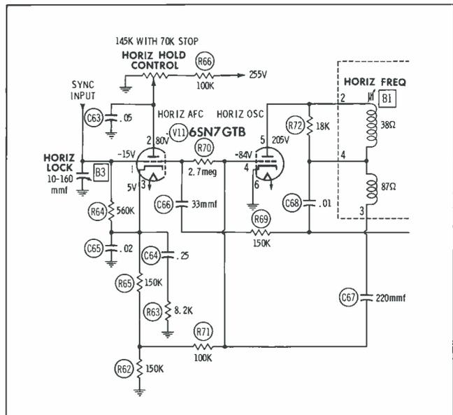
*It sounds as though a component, probably a capacitor, is breaking down due to heat. This occurs only when the chassis is in the cabinet because the components are exposed to a lower temperature if the set is operating on the service bench. With the set on the bench, you can use a heat lamp, directed toward the chassis, to simulate the heat conditions that exist within the cabinet.*
