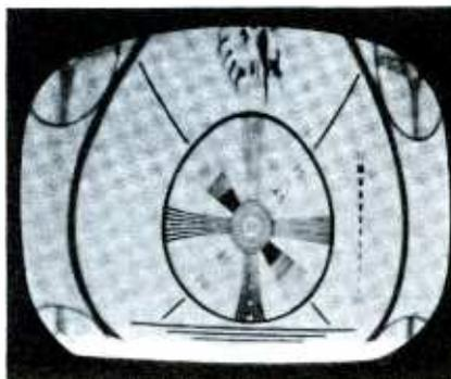
Vertical hold will sync picture but must be positioned near one end of rotation. Height control affects bottom of picture; however, vertical linearity has no influence on top of raster. Adjustment of either size or linearity controls causes uncontrollable roll.
