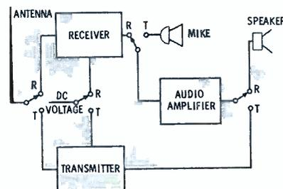
Fig. 2. Transceiver switching operation.
