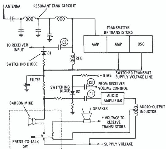
Fig. 11. Electronic switching used in Raytheon TWR-7.
