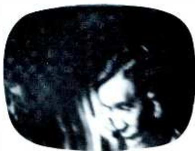
Fig. 1B. Overloaded picture from AGC
