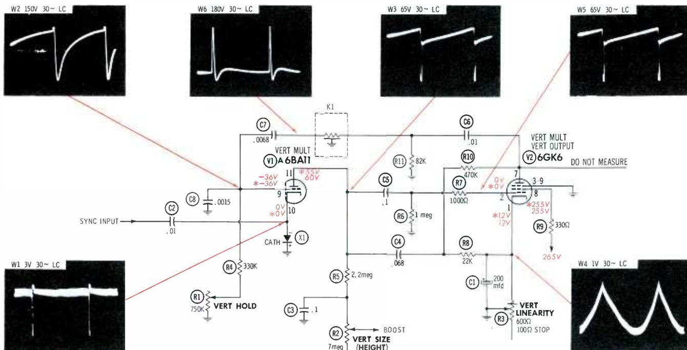
DC VOLTAGES taken with VTVM, on inactive channel; antenna terminals shorted. \*Indicates voltages taken with signal present—see "Operating Variations."
