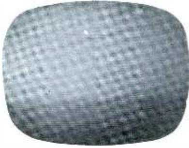
Fig. 5A. AGC faults cause white raster.
