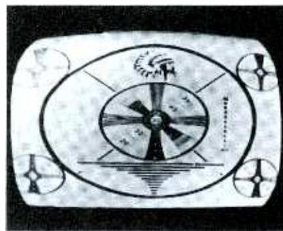
Raster equally compressed at top and bottom. Vertical hold has ample range and syncs picture at center of rotation. Height and linearity controls adjustable so picture fills screen linearly. Even though controls compensate for trouble, component breakdown indicated.
