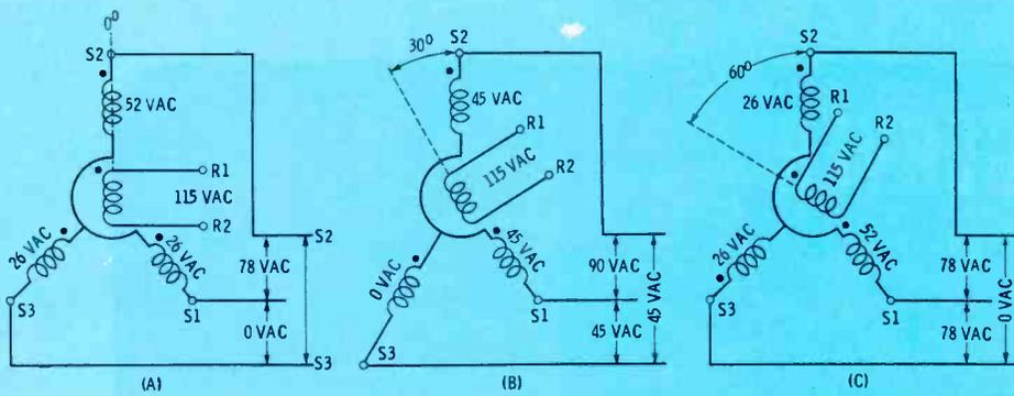
Fig. 3. Synchro stator voltages change as the rotor is turned from 0° to 60°.
