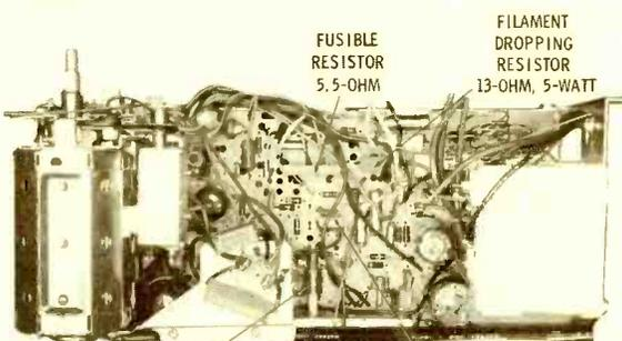
FUSIBLE RESISTOR 5.5-OHM    FILAMENT DROPPING RESISTOR 13-OHM, 5-WATT
