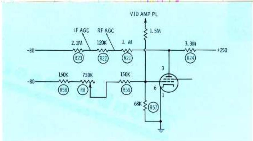
Fig. 8. Simplified schematic of 'BU8 AGC circuit—noise-cancelling grid not shown.
