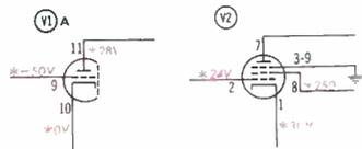
Bias voltage on grid V1A shows increase to  $-50$  volts while pin 10 voltage remains zero. 6BA11 plate reads 28 volts, 50% down. This decreased voltage could be result of increased tube conduction—larger negative voltage on V1A grid indicates greater feedback driving pulse—or defective component in V1A plate circuit. Cathode voltage of 6GK6 has jumped to 30 volts. Leaky C4 could cause voltage change on pin 1, but C4 checks okay. Pin 2 measures 24 volts. C5 suspected and found leaky.
