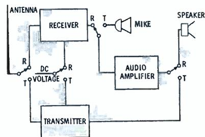
Fig. 2. Transceiver switching operation.
