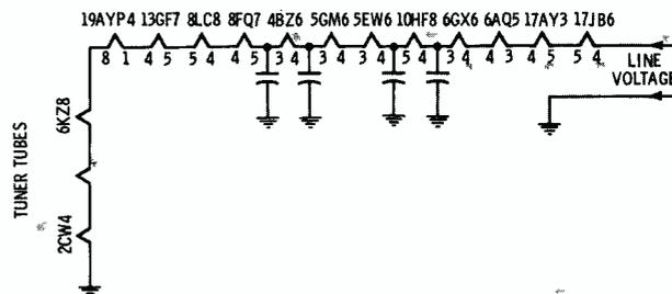
Fig. 2. Series filament circuit in modern-day receivers.
