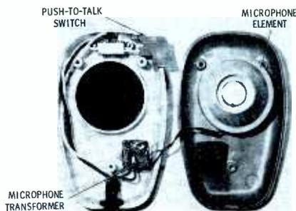
Fig. 1. Inside the microphone case.
