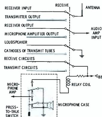
Fig. 9. Switching in vacuum-tube unit.
