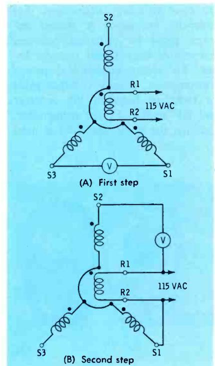
Fig. 6. Connections to locate zero.
