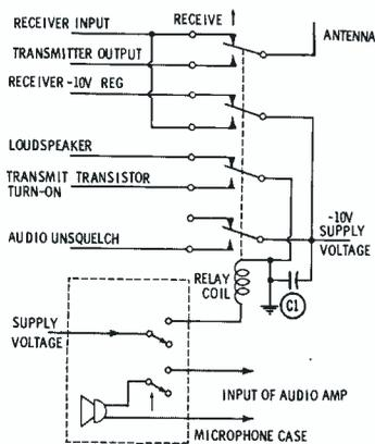
Fig. 8. Switching in 5w solid-state unit.
