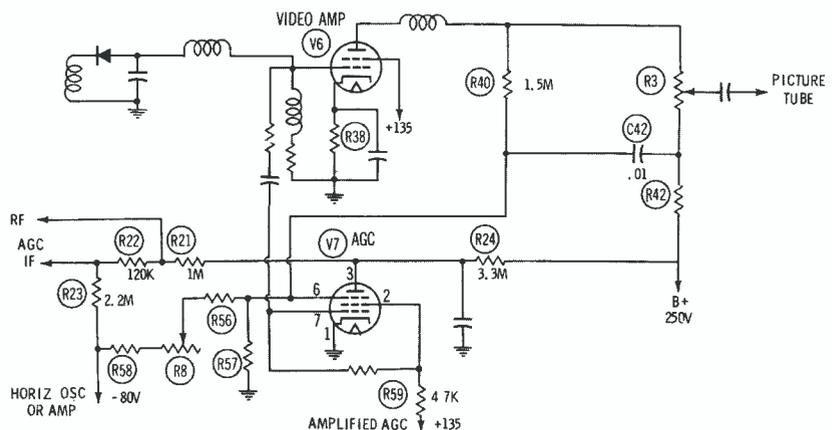
Fig. 7. This single tube amplified AGC circuit is used in Zenith Chassis 17Z30.
