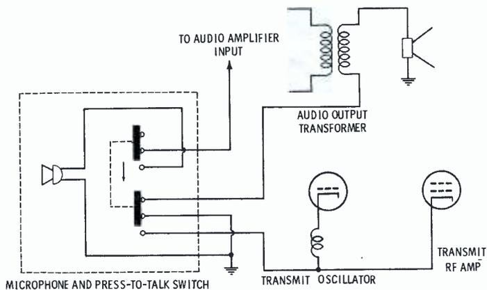
Fig. 3. A direct switching arrangement used in transceivers.
