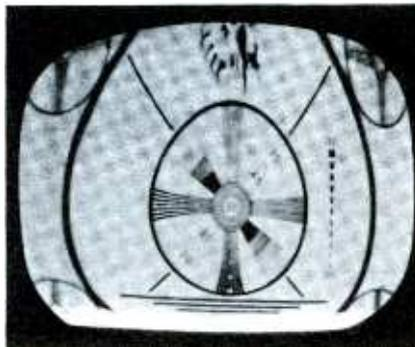
Vertical hold will sync picture but must be positioned near one end of rotation. Height control affects bottom of picture; however, vertical linearity has no influence on top of raster. Adjustment of either size or linearity controls causes uncontrollable roll.
