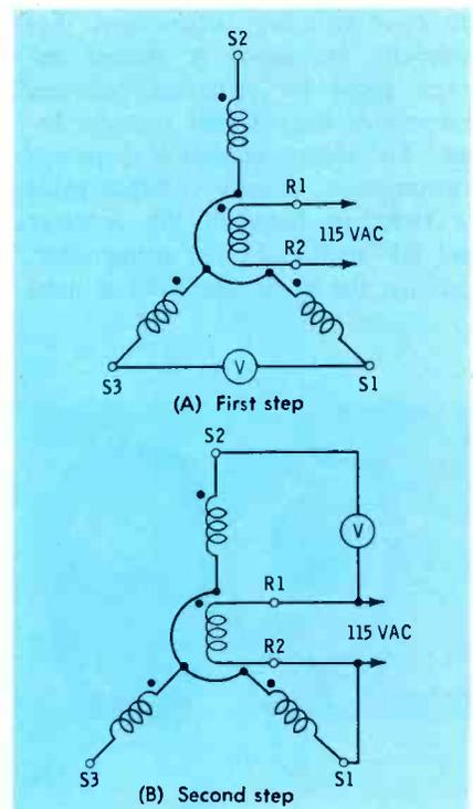
Fig. 6. Connections to locate zero.
