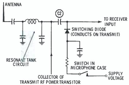
Fig. 10. Electronic antenna switching using a diode.
