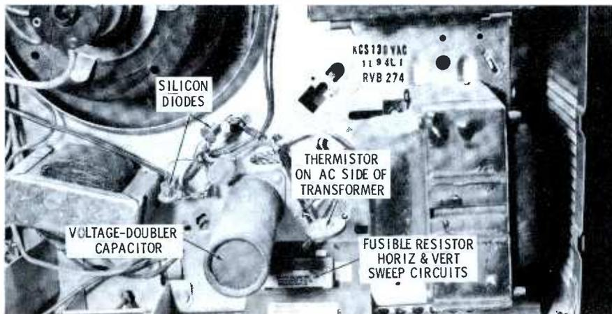
Fig. 3. Location of low-voltage power supply components used in an RCA portable.
