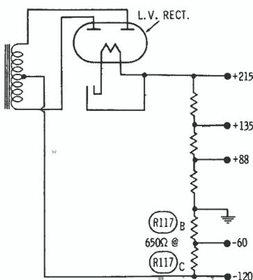
Fig. 6. Observe power-supply voltages.
