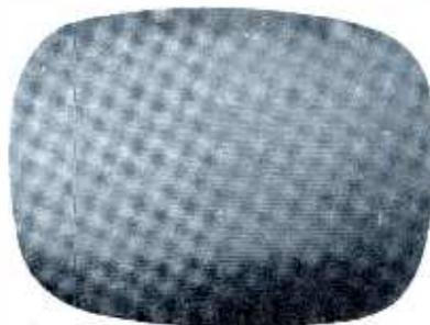
Fig. 9A. No picture—lines in raster.
