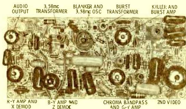
AUDIO OUTPUT 3.58mc TRANSFORMER BLANKER AND 3.58mc OSC BURST TRANSFORMER KILLER AND BURST AMP
