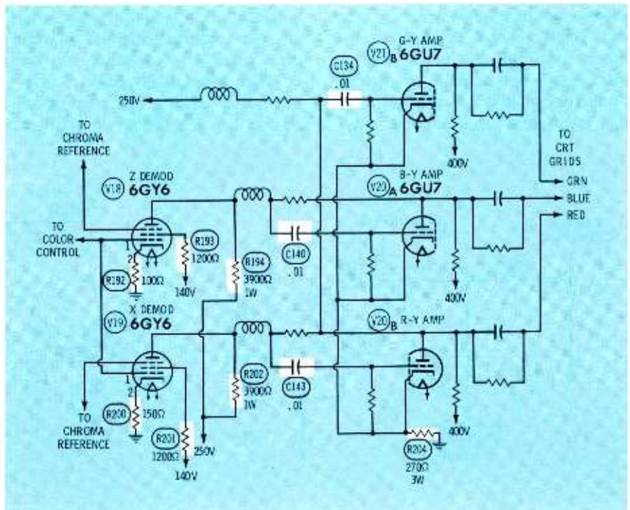
Fig. 1. RCA CTC17 circuit with most troublesome parts indicated.
