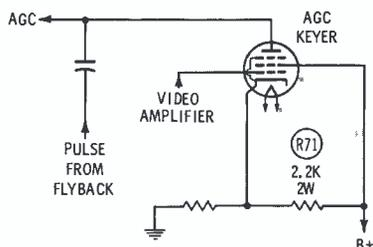
Fig. 10. Source of screen voltage.
