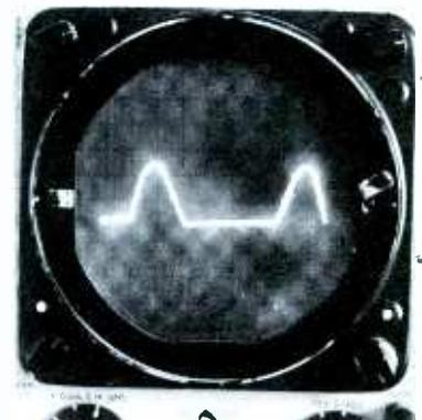
Fig. 2 Base waveform at Q2.
