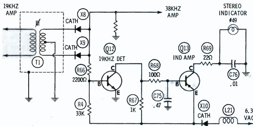
Fig. 1 Schematic Magnavox R204 EP chassis.
