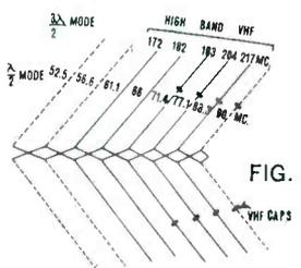
FIG. 2 However, by introducing parallel plate capacitors into the dipoles and by carefully adjusting the value of this capacitance and its position on the dipole, as shown in Figure 2, the resonant frequencies of the dipole can be shifted in the 3/2 wavelength mode. In this way, the dipole can be made to resonate at two desired frequencies: e.g., 88 and 216 mc.
