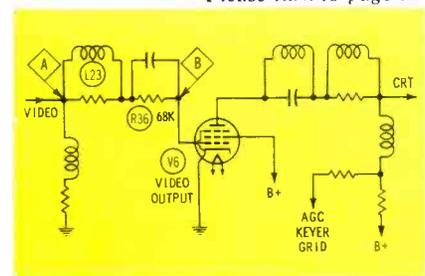
Fig. 9. Bad V6 produced odd symptom
