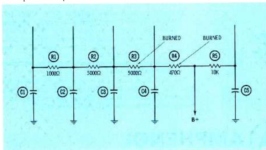
Fig. 2. Ohmmeter tests in this B+ feeder string quickly pinpoint exact fault.
