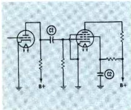
Fig. 1. Small-value coupling and bypass capacitors in a typical R-C amplifier.
