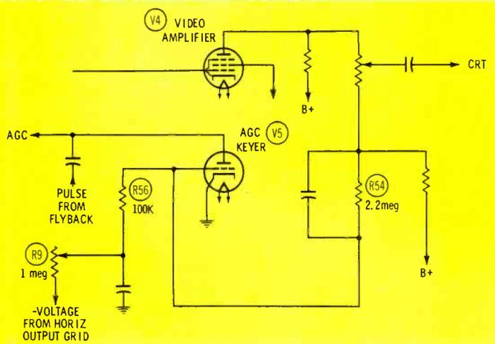
Fig. 5. Circuit with grounded cathode.
