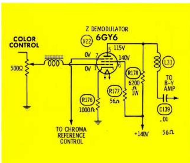
Fig. 2. Admiral 24E2 Z demodulator circuit.
