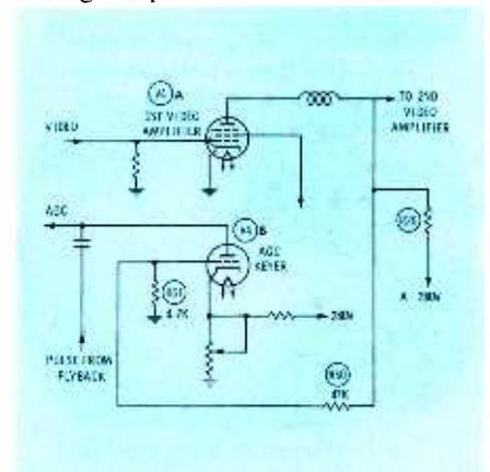
Fig. 4. Source of cathode voltage.
