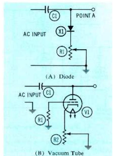
Fig. 2. Control of rectified voltage.
