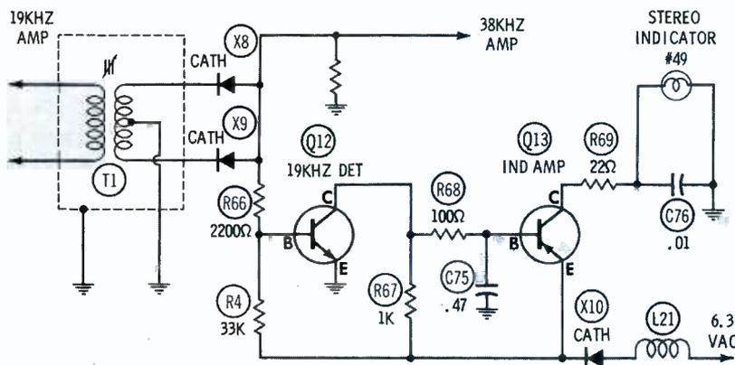
Fig. 1 Schematic Magnavox R204 EP chassis.
