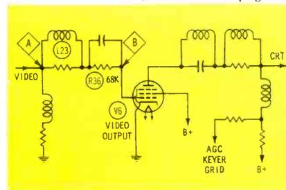
Fig. 9. Bad V6 produced odd symptom
