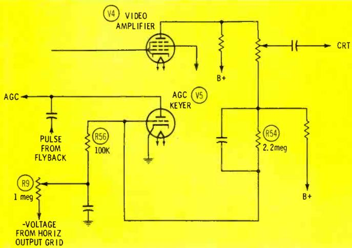
Fig. 5. Circuit with grounded cathode.
