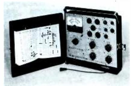
Fig. 2. Checks all modern tubes.
