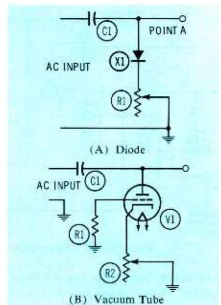
Fig. 2. Control of rectified voltage.
