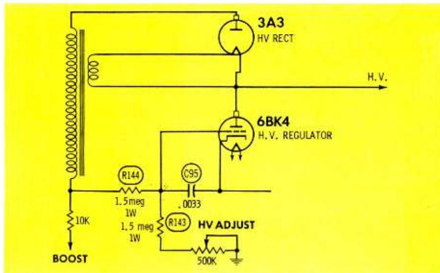
slipped and replacing the 6BK4 plate cap, we turned it on again. Oh, ho! Sure enough, the picture did come on for about 2 seconds, then went fuzzy. When it did, the 6BK4 plate current rose gently to about 3.0 ma!
