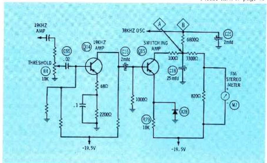
Fig. 4 Schematic Magnavox R201-05 chassis.
