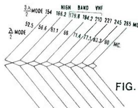
FIG. 1 (Note that only three dipoles resonate at frequencies in the high VHF band.)
