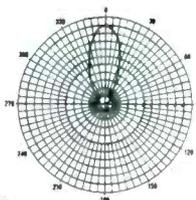
FIG. 3 Result: the active region in the high band extends over five of the eight original dipoles instead of three, as in Fig. 2, with a performance improvement of 66%. The new capacitor-coupled dipoles also present more capture area on the low band than ordinary dipoles. Thus LPV-TV antennas offer, on both bands, higher and more uniform gain, lower side-lobe levels, narrower beamwidths, for vastly improved ghost rejection (see Fig. 3).
