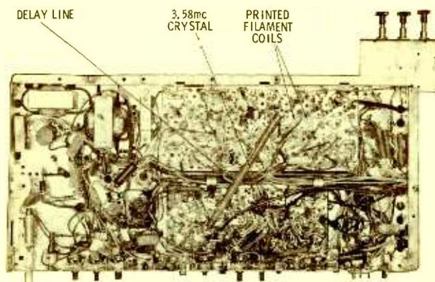
DELAY LINE 3.58mc CRYSTAL PRINTED FILAMENT COILS
