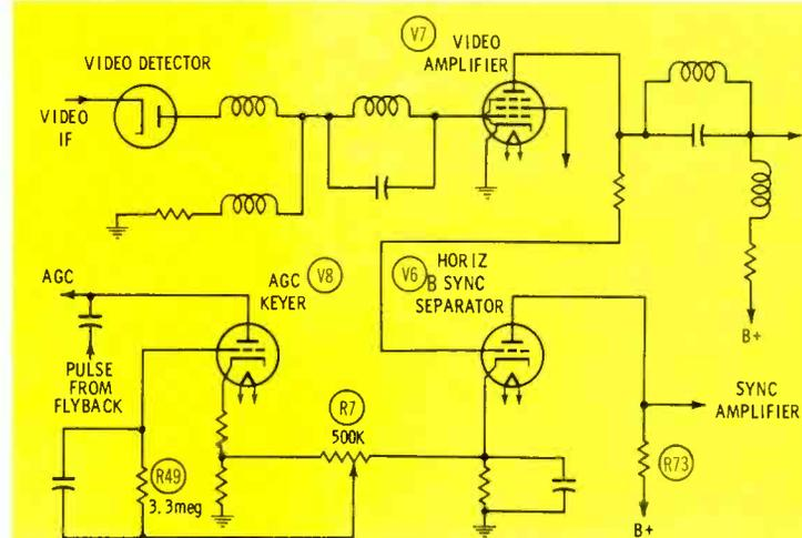
Fig. 6. Use of buffer and amplifier.
