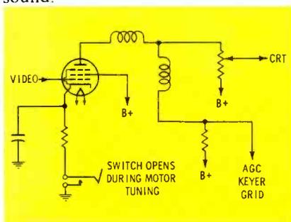
Fig. 8. Cathode lead opened during automatic tuning.
