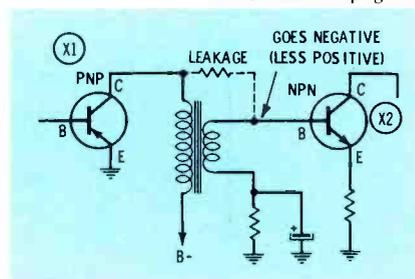
Fig. 9. Leakage has effect similar to leaky coupling capacitors.
