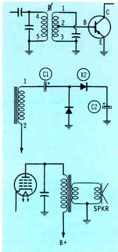
Fig. 8. A few of the many external circuits that affect transformer checks.
