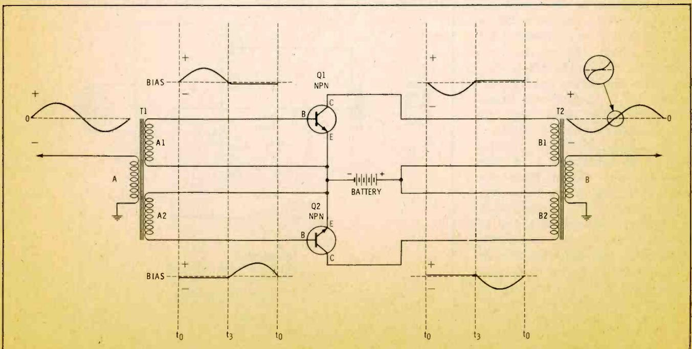
Fig. 14. A class-B output stage with current waveforms. (Waveforms are not drawn to scale.)
