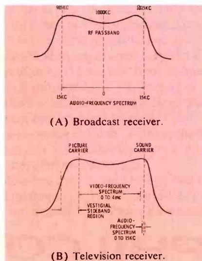
Fig. 1. Frequencies in the RF bandpass.
