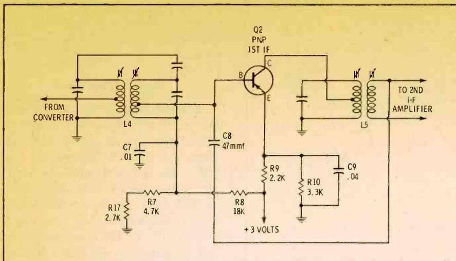
Fig. 11. An IF amplifier with double-tuned transformer.
