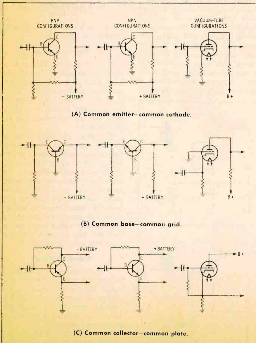
Fig. 1. The transistor circuit configurations and vacuum-tube counterparts.
