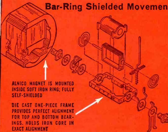
ALNICO MAGNET IS MOUNTED INSIDE SOFT IRON RING; FULLY SELF-SHIELDED
