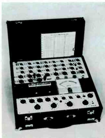
Fig. 1. High speed tube tester.
