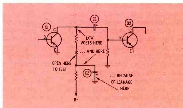
Fig. 7. If voltage becomes normal, C2 is bad. If not, trouble is in X1 or C1.
