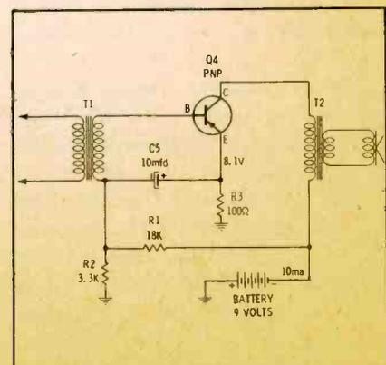
Fig. 13. A class-A output stage.
