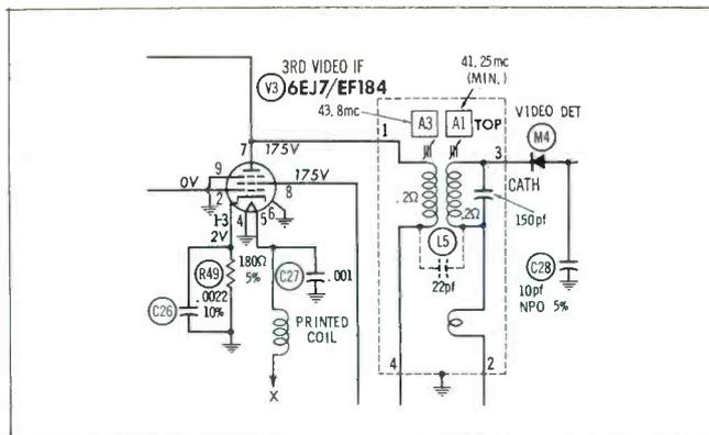
The heat pattern you are experiencing has also occurred in earlier RCA chassis and is a result of the 4th harmonic of the picture IF carrier, generated in the picture-detector circuit, being picked up by the 300-ohm lead associated with the UHF/VHF switch. The frequency of the interference is approximately 183 mHz, depending on the position of the fine-tuning control.
