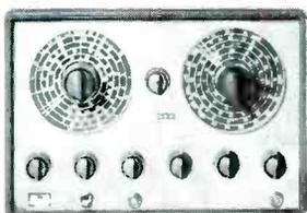
**Model 369** Sweep/Marker Generator for easiest, fastest visual alignment of color or B&W TV and FM RF and IF circuits. Five sweep ranges from 3-220mc. Four marker ranges from 2-225mc. Crystal marker oscillator. Post injection of markers. \$99.95 kit, \$149.95 wired.
