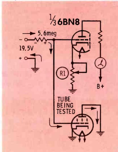
Fig. 2. Simplified schematic shows how grid-emission test is accomplished.
