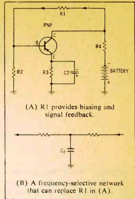
Fig. 4. Bias stabilization and feedback.
