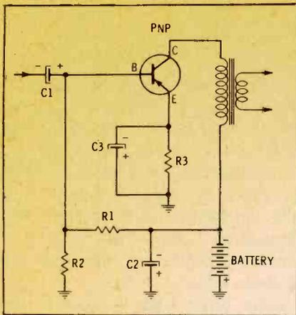
Fig. 5. Common R-C coupled circuit.
