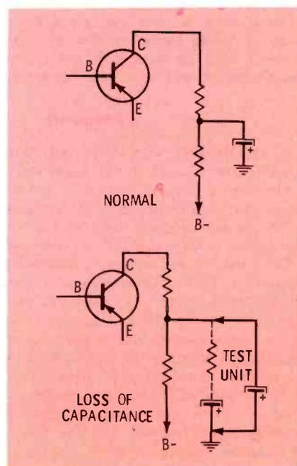
Fig. 4. Loss of capacitance has effect of resistor in series with electrolytic.
