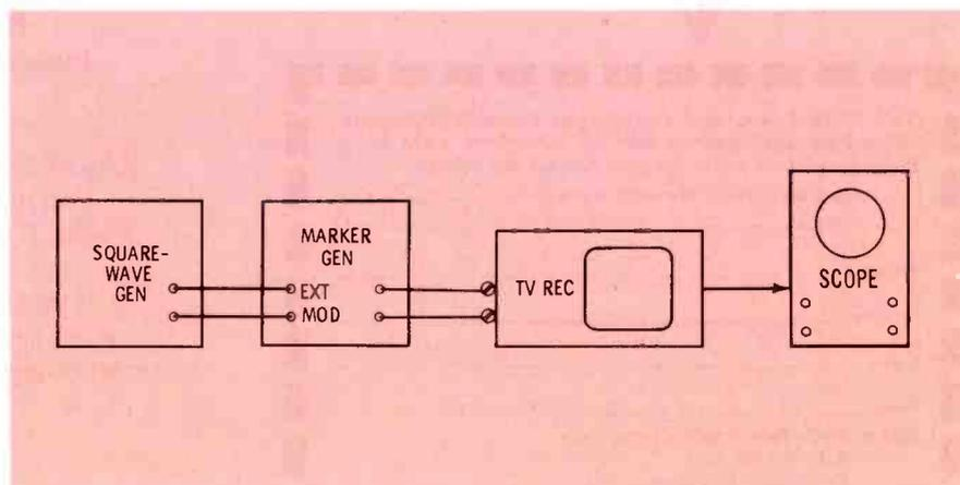
Fig. 2. Basic test setup.
