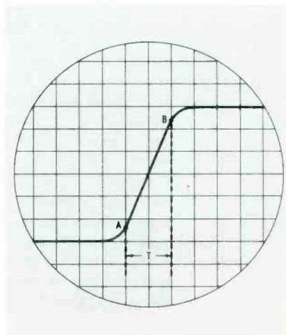
Fig. 9. Measure rise time from A to B.
