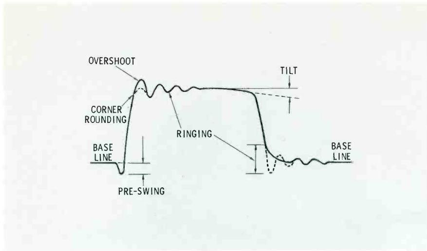
Fig. 7. Results of improper frequency.
