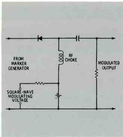
Fig. 3. Wide-band modulator found in good-quality marker generator.
