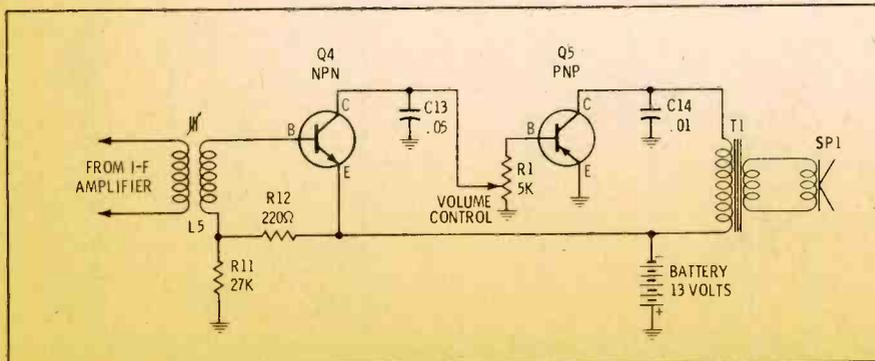
Fig. 9. A DC coupled amplifier employed in a receiver.
