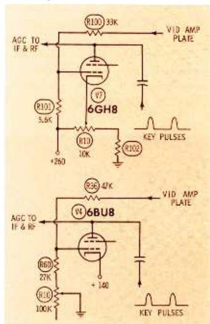
Fig. 1. Sensitivity of keyed AGC stage is controlled by either of these circuits in many designs.
