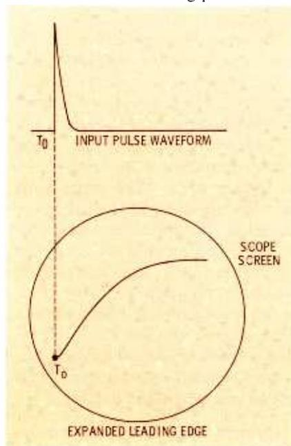
Fig. 6. Sweep must start at the beginning of the pulse.
