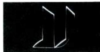
(B) 60Hz square-wave with excessive tilt.
