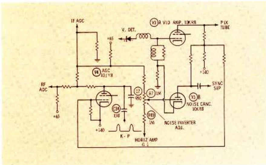
Fig. 3. Decreasing capacity of C-7 to 820 pf cured trouble in Philco.
