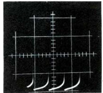
Fig. 5. Normal vertical-output pulses.
