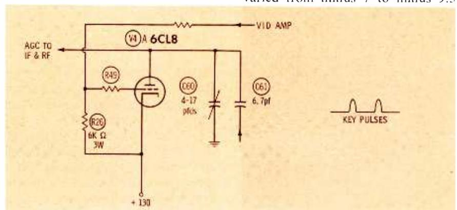
Fig. 2. Westinghouse controls levels of AGC voltage developed by varying amplitude of keying pulses via variable capacitor C-60.
