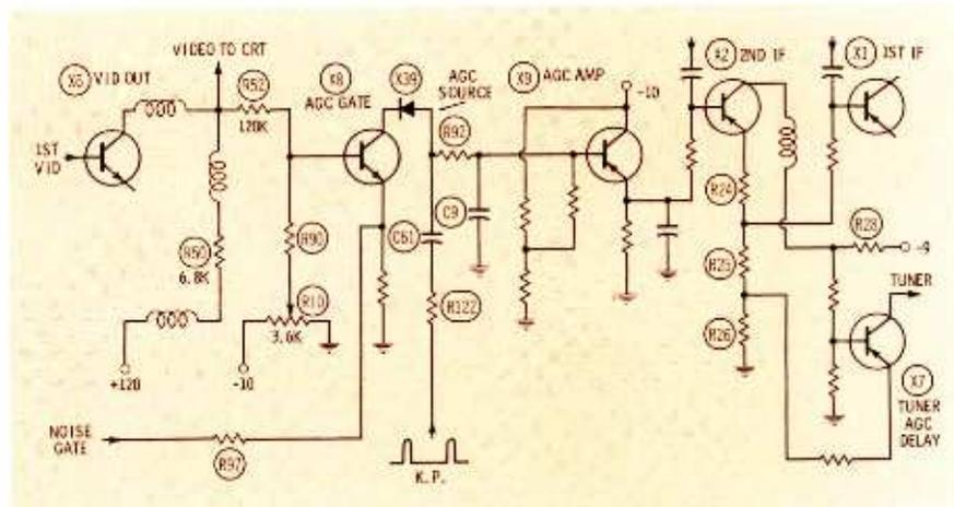
Fig. 5. Late transistorized TV by Zenith uses this keyed AGC circuit with some interesting features.
