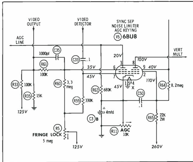
Thanks for sharing your solution with us. Without screen voltage V5 will not conduct, no AGC voltage will be developed, and the 1st video IF stage will become overloaded, causing the loss of both video and sound. However, it should be pointed out that the possible troubles described in the June Troubleshooter Column can result in the same symptoms—which just goes to show that there is always more than one side to every trouble, and in this case we overlooked one.
