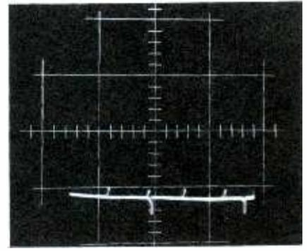
Fig. 4. Vertical oscillator out of sync.
