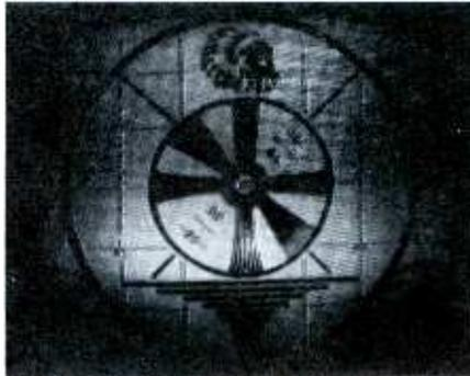
B-w picture and sound normal except for insufficient brightness—even with controls at maximum. Raster is full width, doesn't bloom, and focus is normal. Color picture is low in brightness, but chroma information is normal. Symptoms indicate loss of luminance signal.
