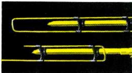
The BI MODAL parasitic elements combine two high band directors into a single director covering all low-band channels, plus the entire FM band. These directors are resonated to overcome the natural tendency for fall-off in gain at 108 MHz and 216 MHz. Thus, the Paralog-Plus is exceptionally flat across the entire VHF television and FM bands.
