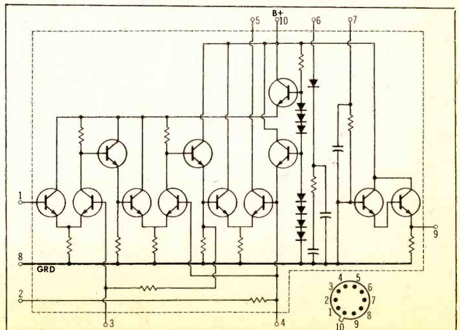
and video-output stage, it effectively controls the maximum conduction level of the CRT. This control is preset at the factory to provide maximum conduction desired in the video-output transistor and should not require adjustment unless one of the three video amplifiers changes characteristics or is replaced.
