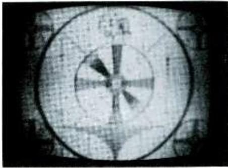
At times screen is dark at any brightness control setting. Other times, screen may be dark at maximum brightness, with almost normal picture at lower settings. Most of time, picture shows excessive brightness, impossible to focus, and retrace lines evident.
