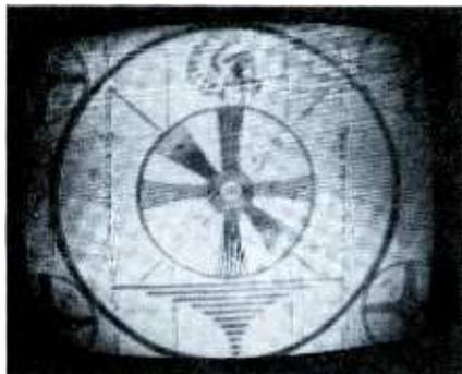
Vertical retrace lines all through picture during both color and b-w. More predominant in scenes with high brightness and low contrast. Lines can be eliminated by reducing brightness and increasing contrast controls, but picture too dark.
