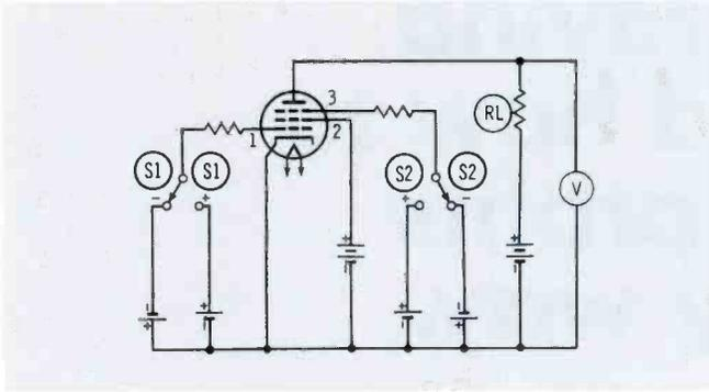
Fig. 1. AND gate using gated-beam tube.
