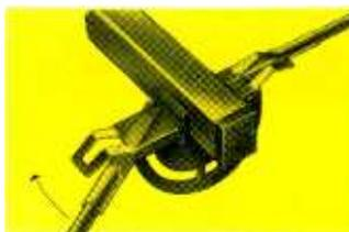
The wedge-snap lock actually tightens and improves with vibration. The spring pressure of the clamp jams the wedge aperture over the squared dipole's end. Since it cannot seat all the way down, a sharp pressure is maintained on the edges of the dipole. Vibration merely tightens the pressure, jamming the wedge into the dipole so that it is both self-cleaning and self-tightening.
