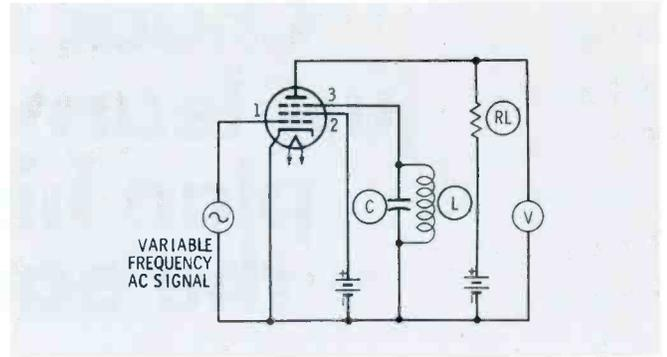
Fig. 2. Gated-beam frequency sensor.
