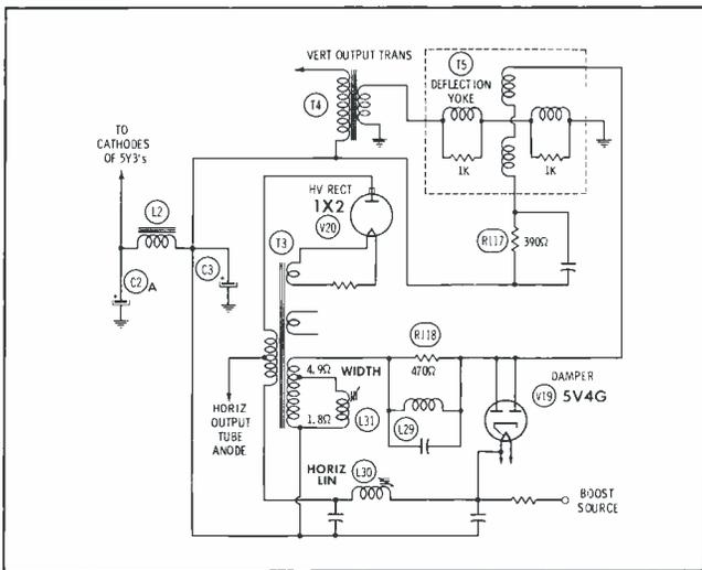
Your troubleshooting procedure is quite sound. The next step to take is resistance measurements of the yoke itself. All indications are a short between vertical and horizontal windings, as the vertical winding presents a ground at each end. There is a possibility of a mechanical short to ground anywhere along the wiring between the yoke and the horizontal output transformer.
