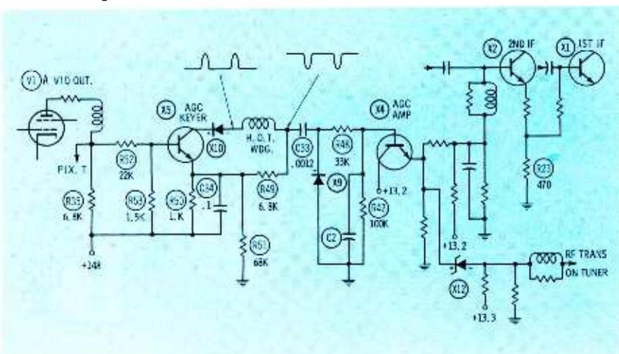
Fig. 7. Philco 16JT26 intermixes tubes and transistors but keyed AGC circuits uses transistors. Shop Talk Editor thinks three circuits are typical of future designs.
