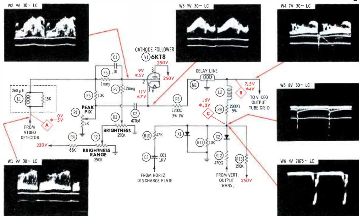
DC VOLTAGES taken with VTVM, on inactive channel; antenna terminals shorted. \*Indicates voltage taken with signal present — see "Operating Variations."
