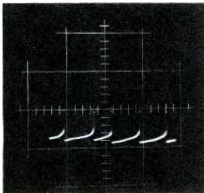
Fig. 3. Abnormal vertical-output pulse.
