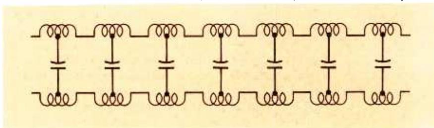
Fig. 8. Basic delay-line circuit.
