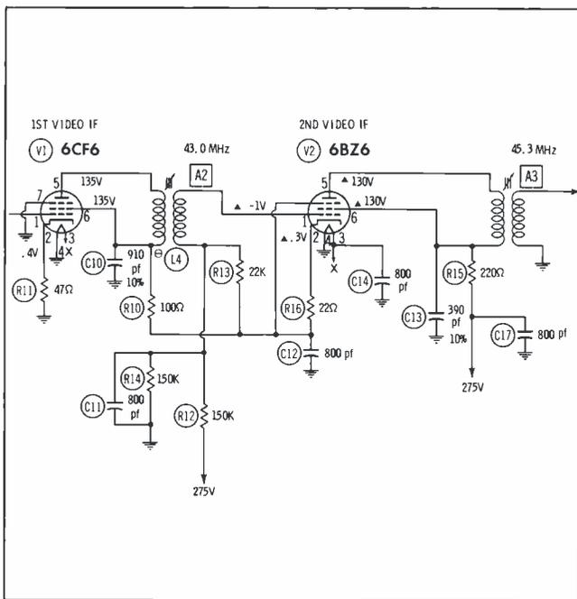
Note that most of the voltage readings around V2 have a small symbol ▲ beside them. This indicates the foot note "▲ measured from pin 7 of V2." The plate of V2 is actually 265 volts above ground, the cathode 135.3 volts, and the grid 134 volts. A heater-to-cathode short in V2 would make the cathode 0 volts, G1 134 volts and the plate 265 volts, and the tube would draw very excessive current. If C12 or C10 shorted the effect would be much the same.
