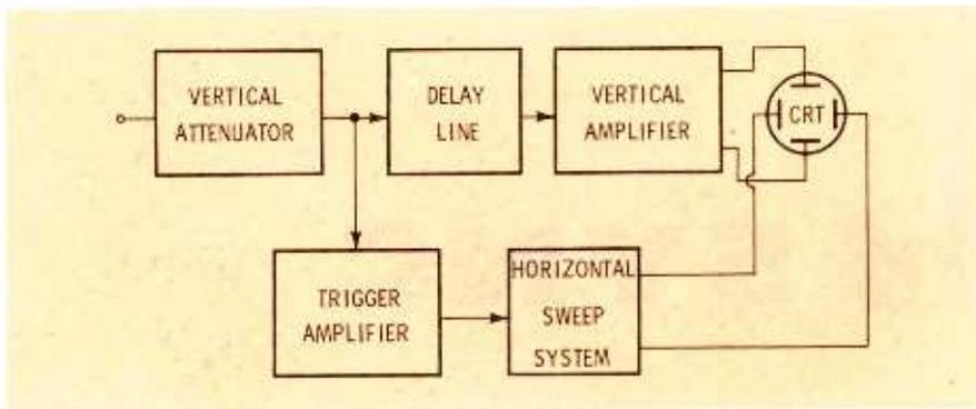
Fig. 7. Delay line permits early triggering of sweep.
