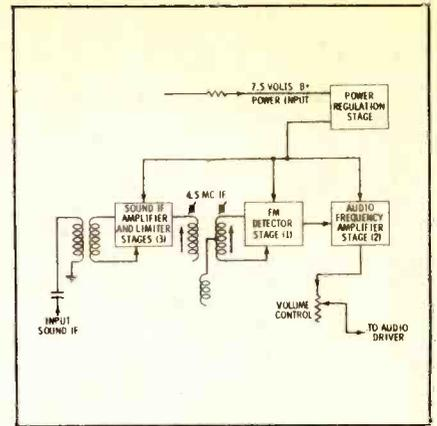
former, rather than by a winding on the horizontal-output transformer, as was the case in the 16JT26 chassis. The AGC circuit in this chassis is basically the same as that used in the 16JT26. Two transistors are used, one as the AGC gate and the other as the AGC amplifier.
