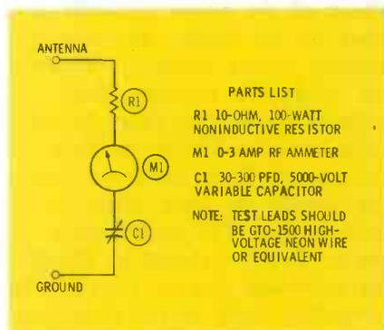
Fig. 1. Circuit diagram of dummy load.
