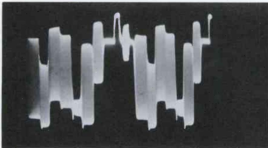
Fig. 13. Composite color waveform.
