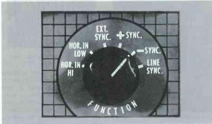
Fig. 10. Negative slope setting.
