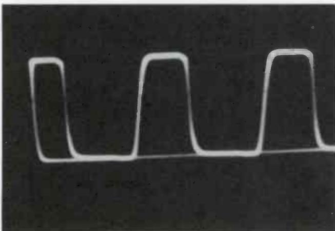
Fig. 4. Semi-square wave on free-running oscilloscope.
