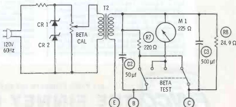
Fig. 3. Simplified schematic of the beta tester.
