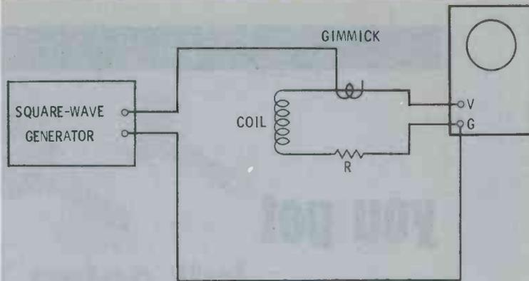
Fig. 3. Test setup with arbitrary resistance connected in series with coil.
