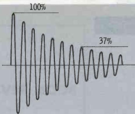
Fig. 2. Damped sine wave with 7 cycles between amplitude level of 100% and 37%.
