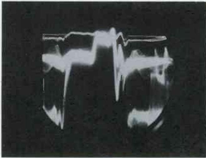
Fig. 7. Horizontal-sync pulse on free-running sweep.
