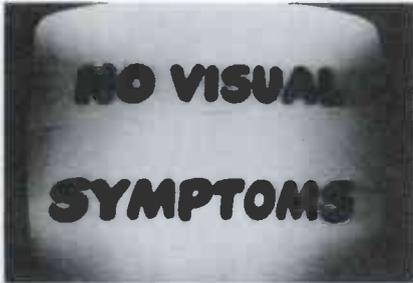
AM and phono operation is normal. FM is weak on normally strong stations—normally weak stations almost lost. Stereo FM same as FM, separation is poor. Stereo indicator lights on stereo station signal. All symptoms point to stereo FM circuitry.
