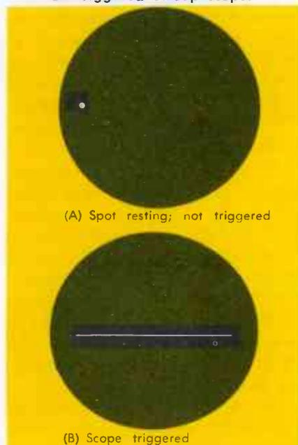
Fig. 2. Trigger control of CRT beam.
