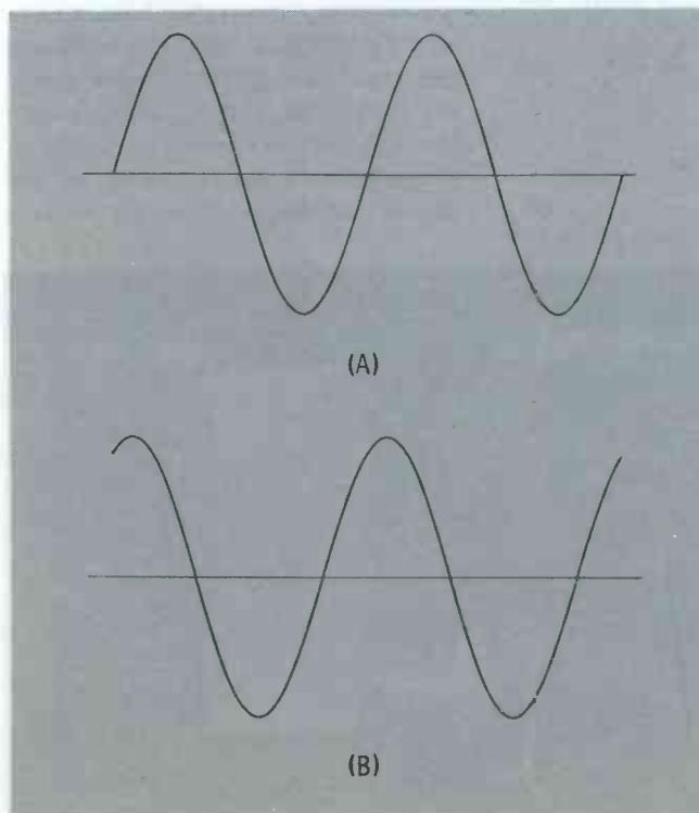
Fig. 11. Triggered higher on the leading edge with + sync.
