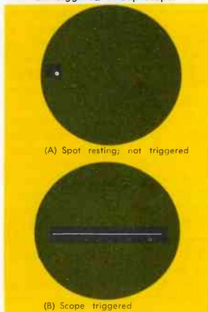
Fig. 2. Trigger control of CRT beam.
