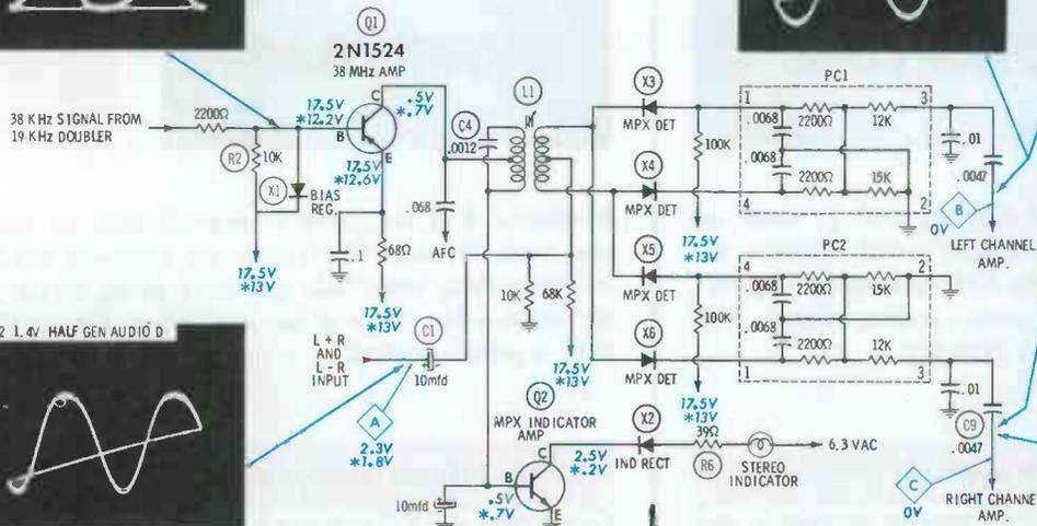
DC VOLTAGES taken with VTVM; receiver off station. \*Indicates voltage taken with signal from stereo generator present — see "Operating Variations."
