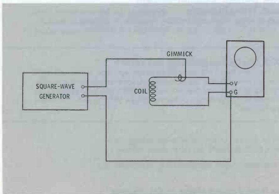
Fig. 1. Equipment setup to measure Q.
