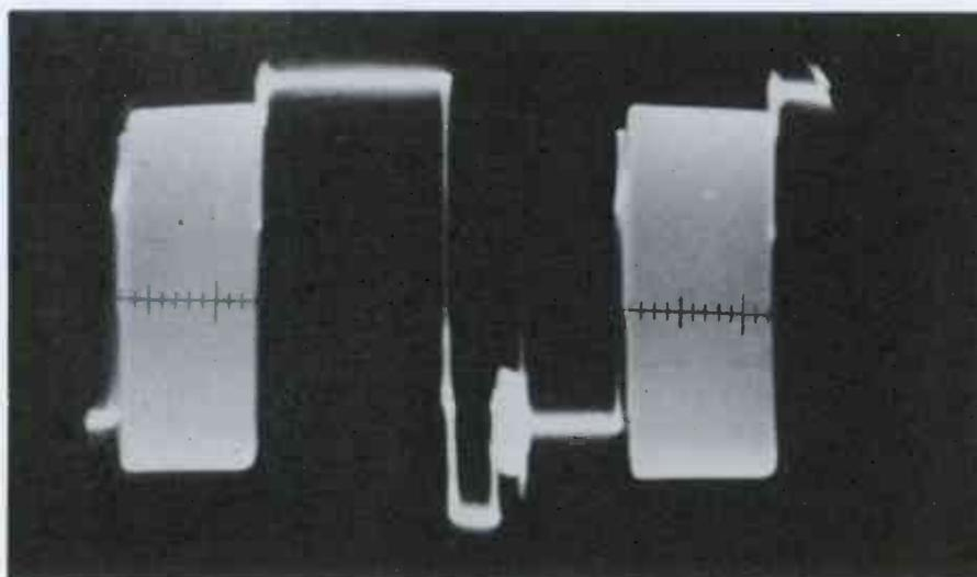
Fig. 15. Color burst located in negative portion of waveform.
