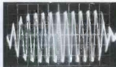
Fig. 14. Triggered-sweep scope display of color burst.
